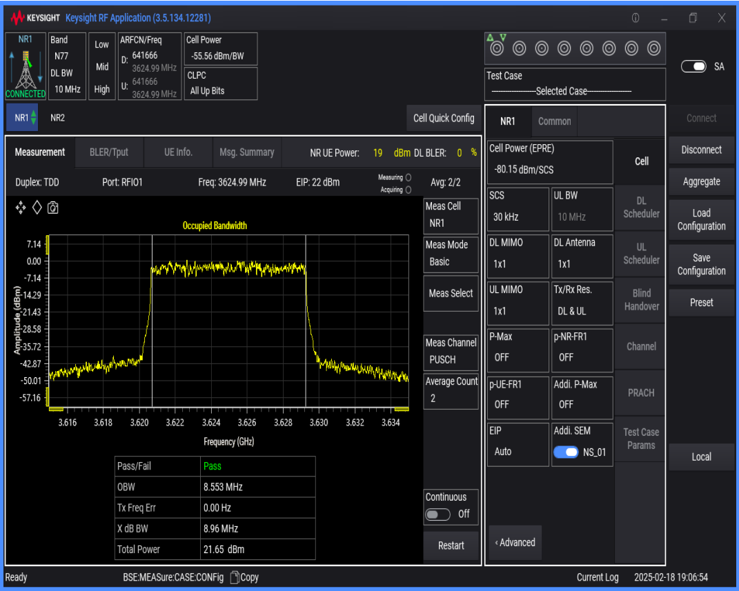
n77(3550-3700) SCS=30kHz DFT_QAM64 BW=15MHz Channel=641666 RB=36@0
