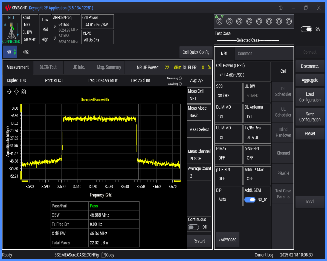
n77(3550-3700) SCS=30kHz DFT_QAM16 BW=40MHz Channel=641666 RB=100@0
