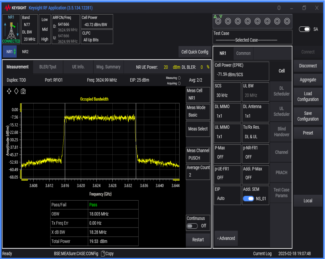
n77(3550-3700) SCS=30kHz DFT_QAM256 BW=60MHz Channel=641666 RB=162@0
