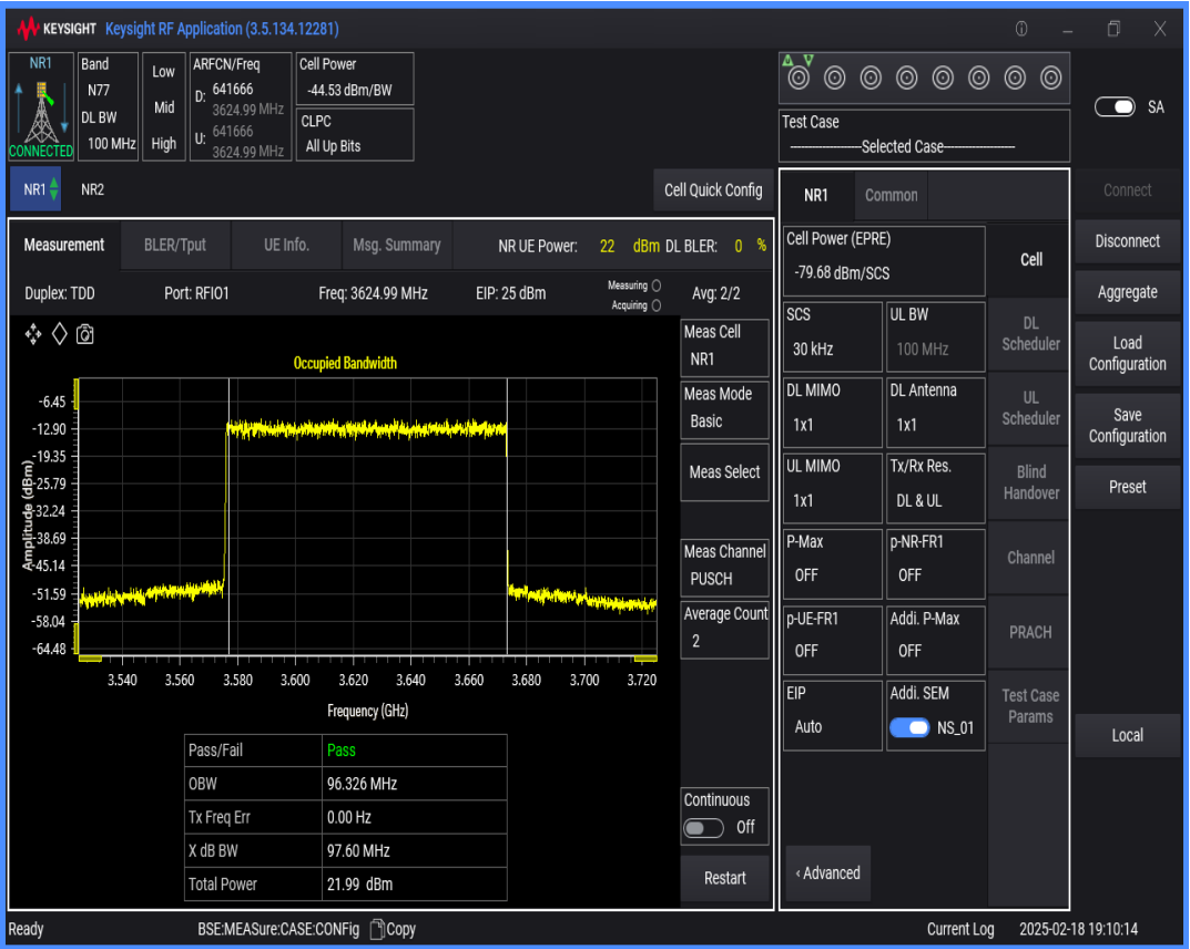
n77(3550-3700) SCS=30kHz DFT_BPSK BW=90MHz Channel=641666 RB=240@0
