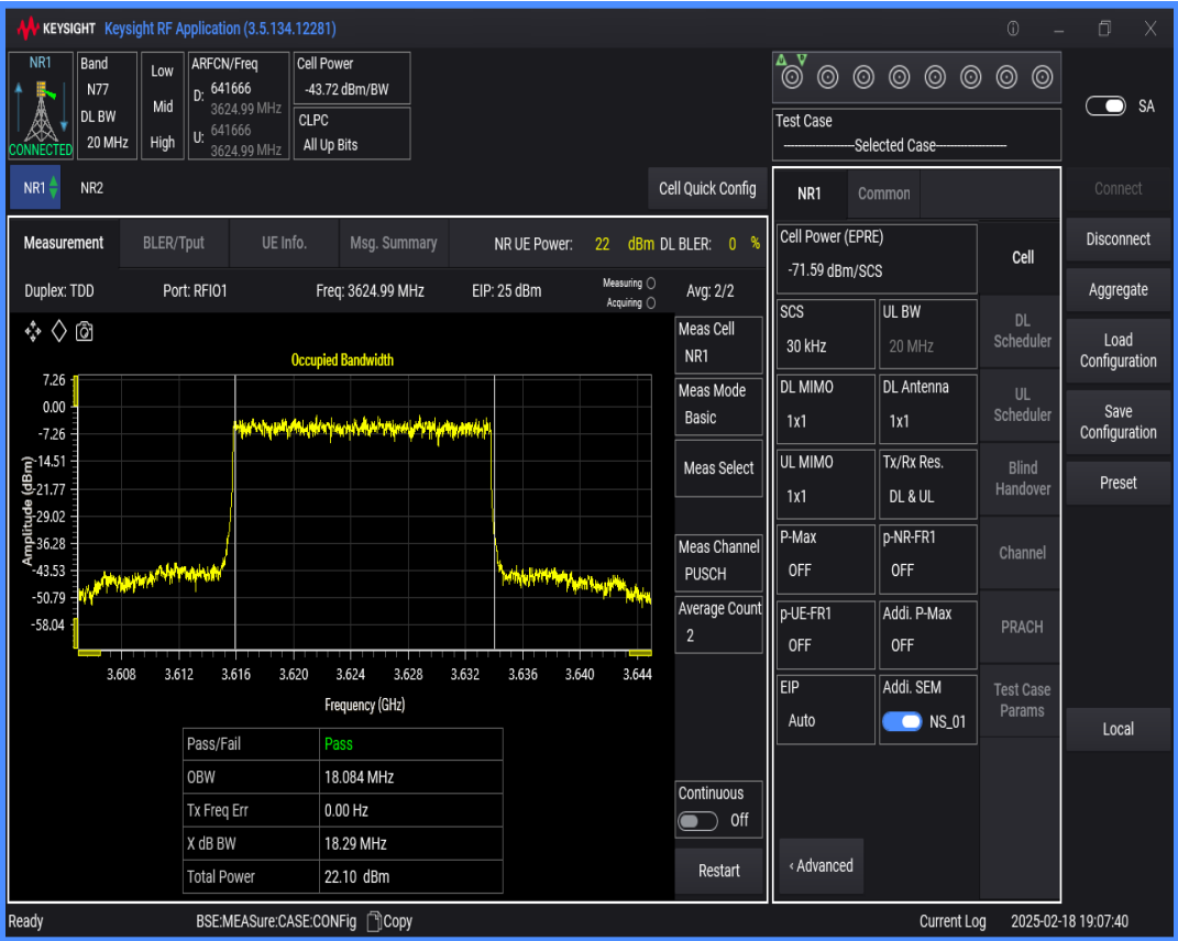
n77(3550-3700) SCS=30kHz DFT_QAM16 BW=15MHz Channel=641666 RB=36@0
