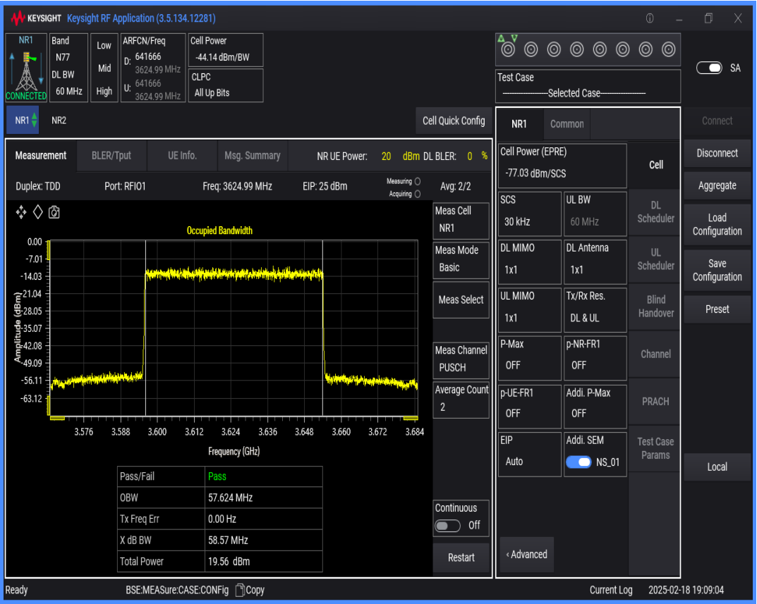
n77(3550-3700) SCS=30kHz DFT_QAM256 BW=80MHz Channel=641666 RB=216@0
