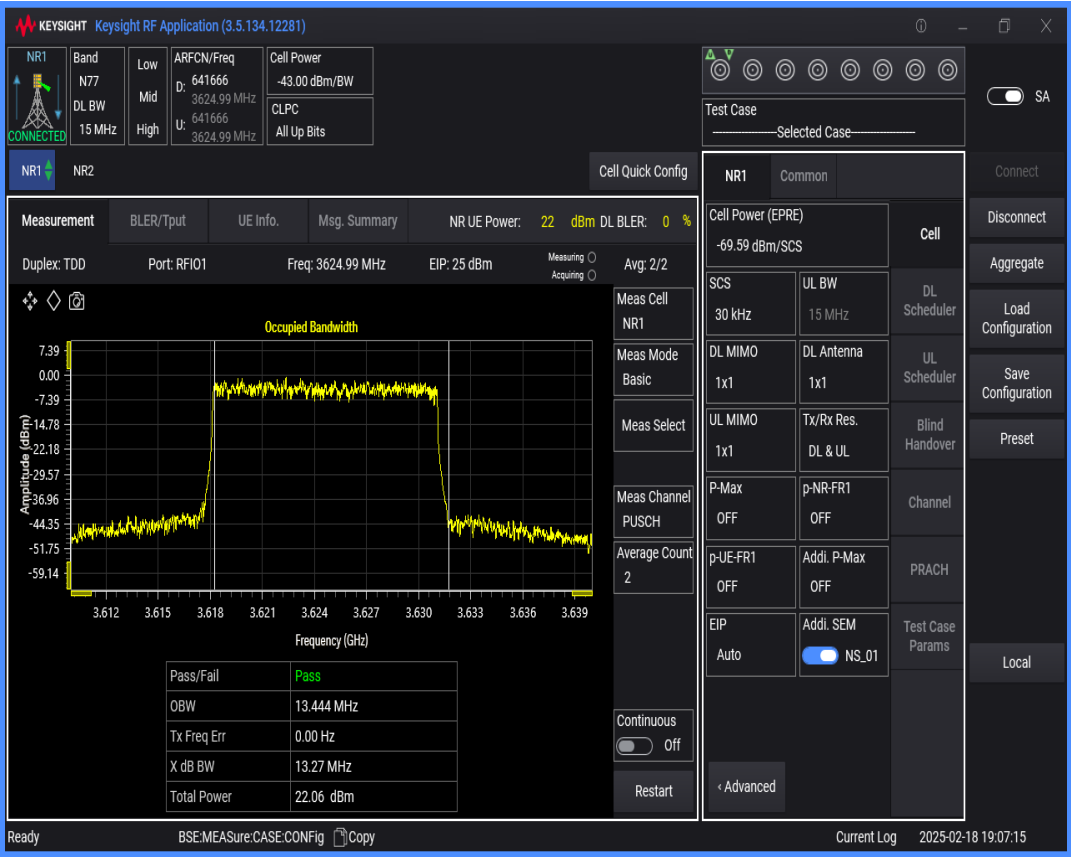
n77(3550-3700) SCS=30kHz DFT_QAM16 BW=60MHz Channel=641666 RB=162@0
