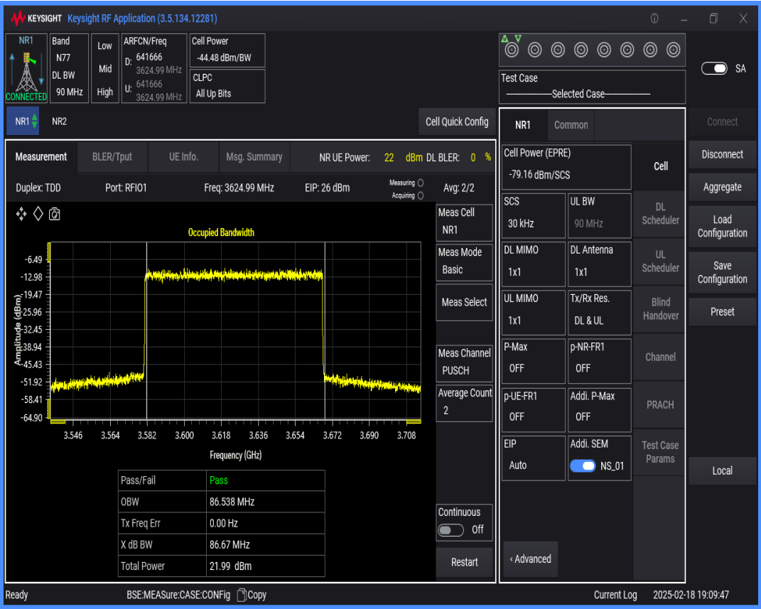
n77(3550-3700) SCS=30kHz DFT_QAM16 BW=80MHz Channel=641666 RB=216@0
