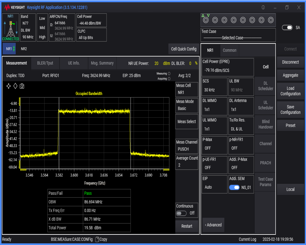
n77(3550-3700) SCS=30kHz DFT_QAM64 BW=100MHz Channel=641666 RB=270@0
