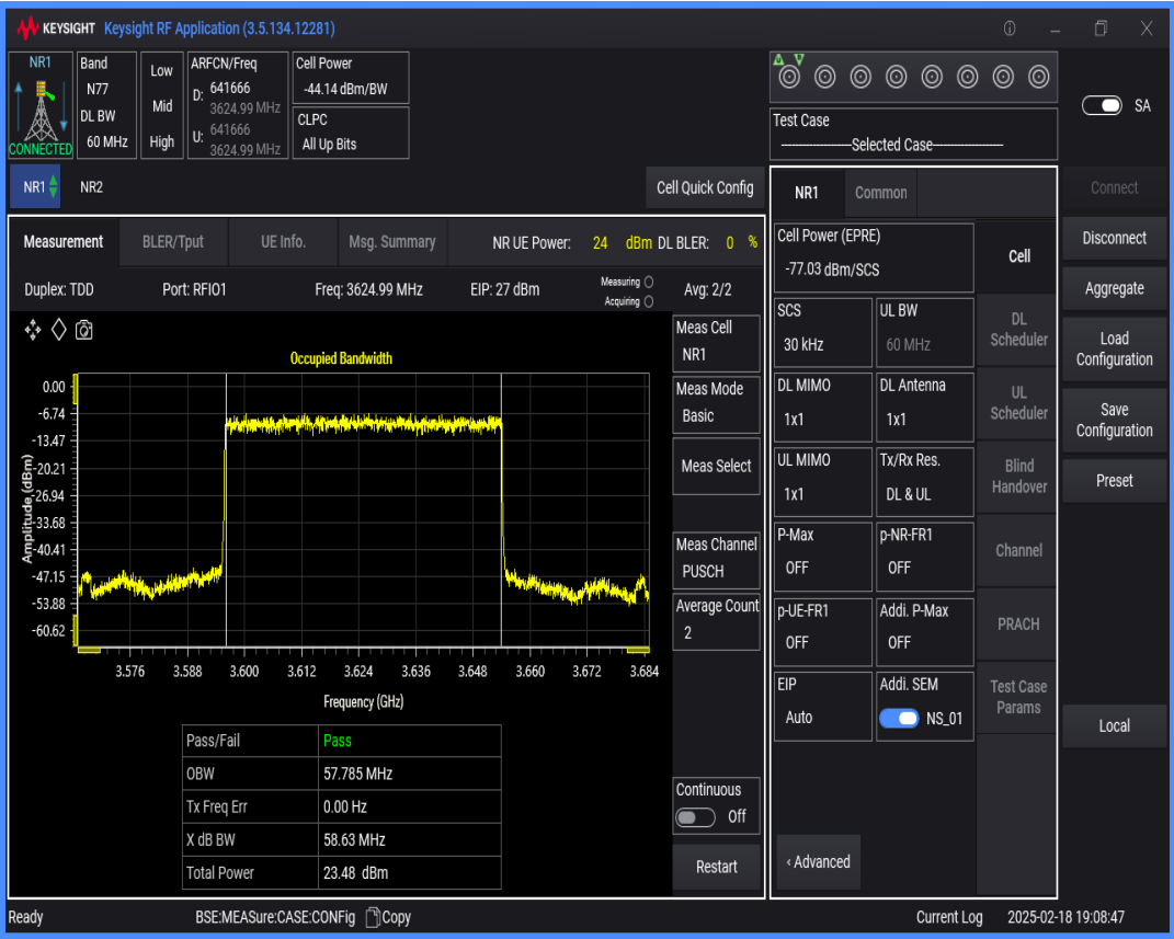
n77(3550-3700) SCS=30kHz DFT_BPSK BW=80MHz Channel=641666 RB=216@0
