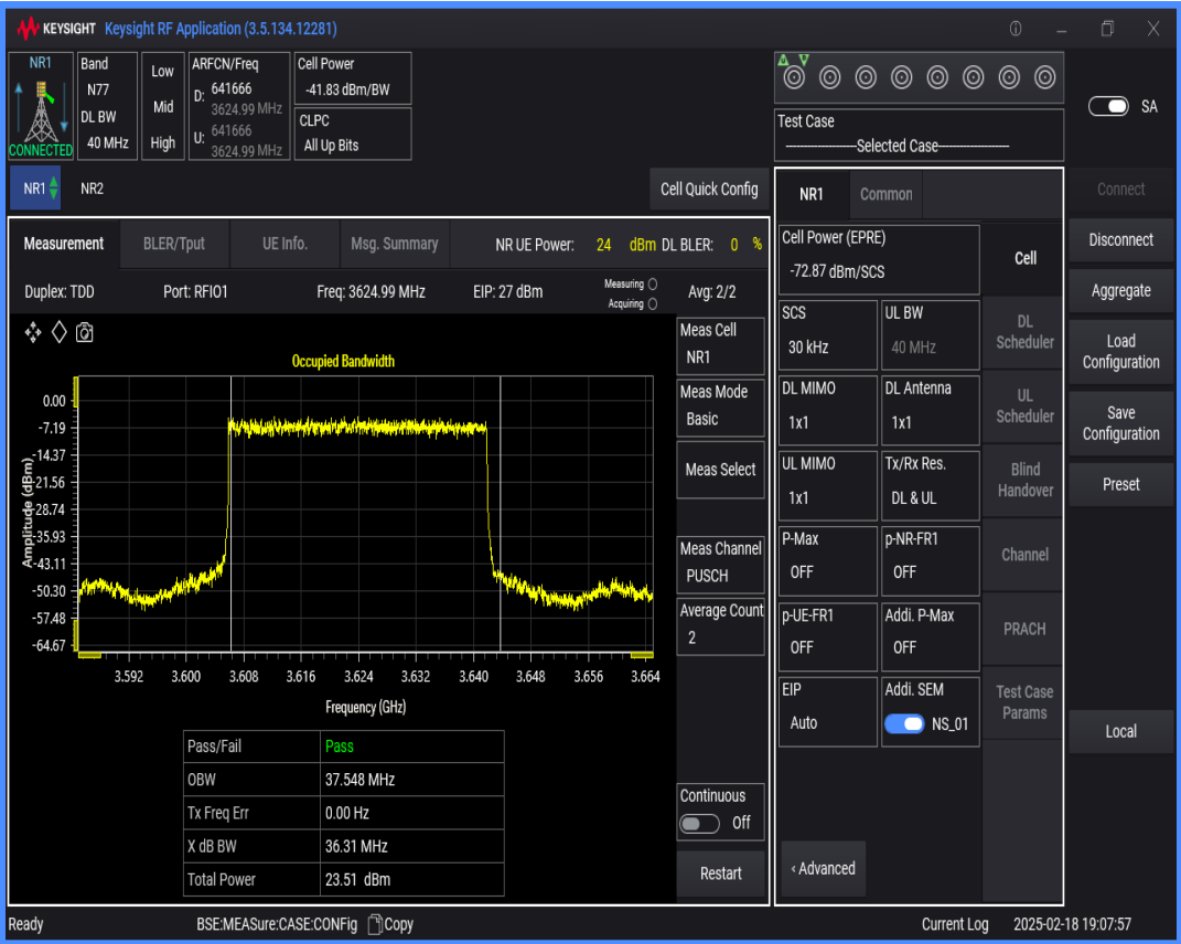
n77(3550-3700) SCS=30kHz DFT_BPSK BW=60MHz Channel=641666 RB=162@0
