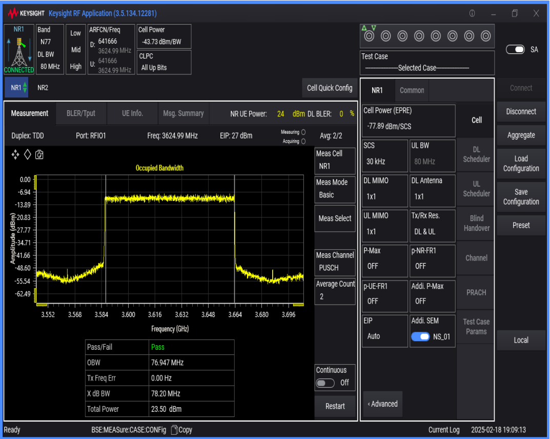
n77(3550-3700) SCS=30kHz DFT_QAM16 BW=10MHz Channel=641666 RB=24@0
