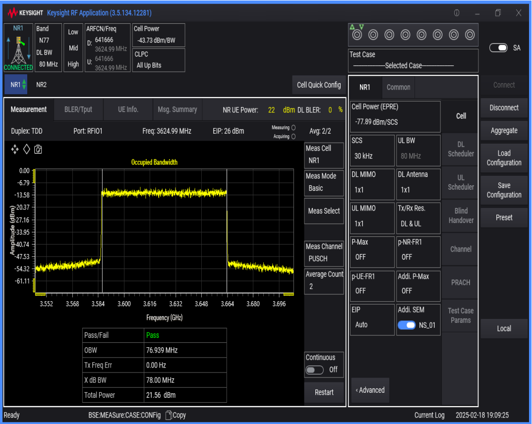
n77(3550-3700) SCS=30kHz DFT_QAM64 BW=50MHz Channel=641666 RB=128@0
