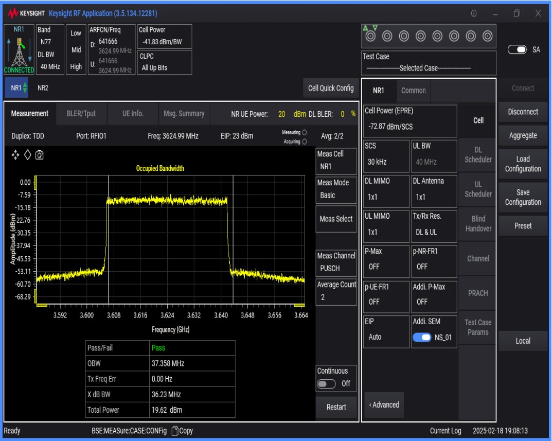
n77(3550-3700) SCS=30kHz DFT_QAM256 BW=50MHz Channel=641666 RB=128@0
