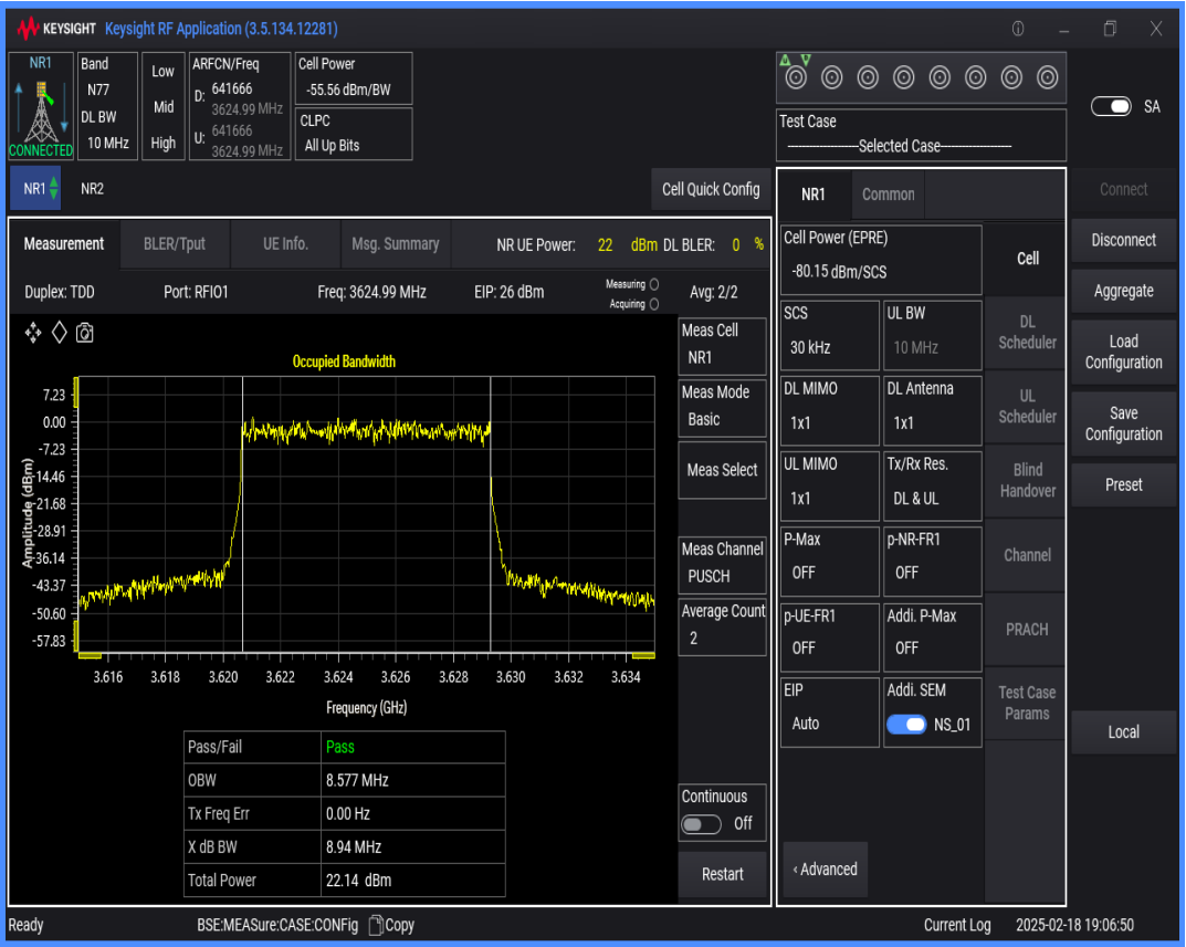
n77(3550-3700) SCS=30kHz DFT_QAM16 BW=100MHz Channel=641666 RB=270@0
