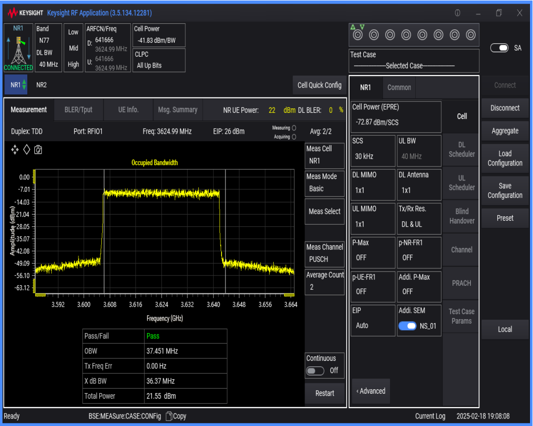
n77(3550-3700) SCS=30kHz DFT_QPSK BW=10MHz Channel=641666 RB=24@0
