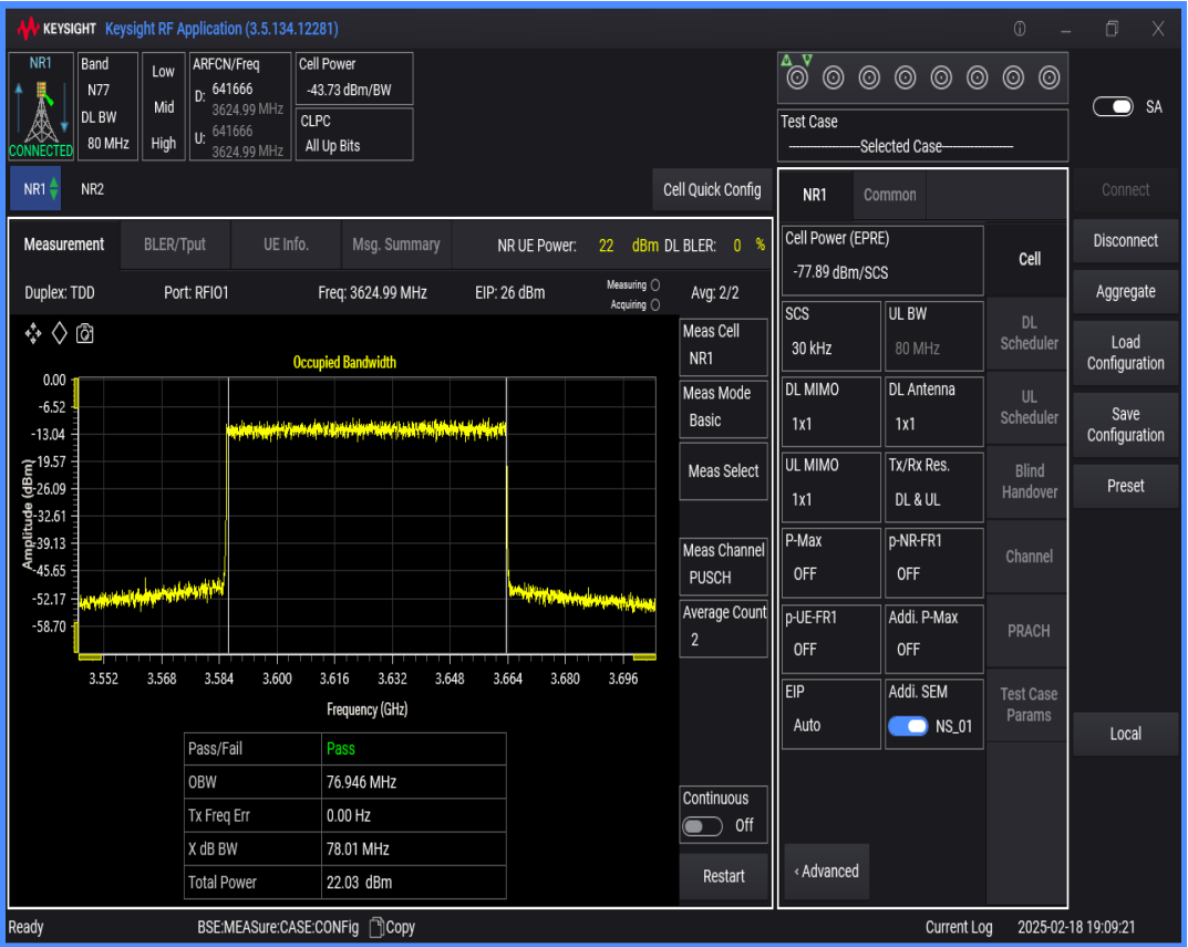
n77(3550-3700) SCS=30kHz DFT_QAM256 BW=15MHz Channel=641666 RB=36@0
