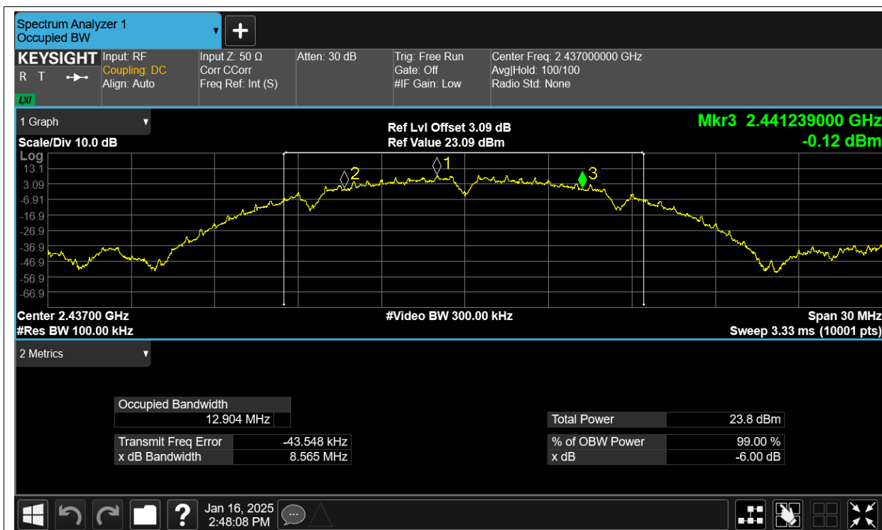
-6dB Bandwidth NVNT b 2462MHz Ant12
