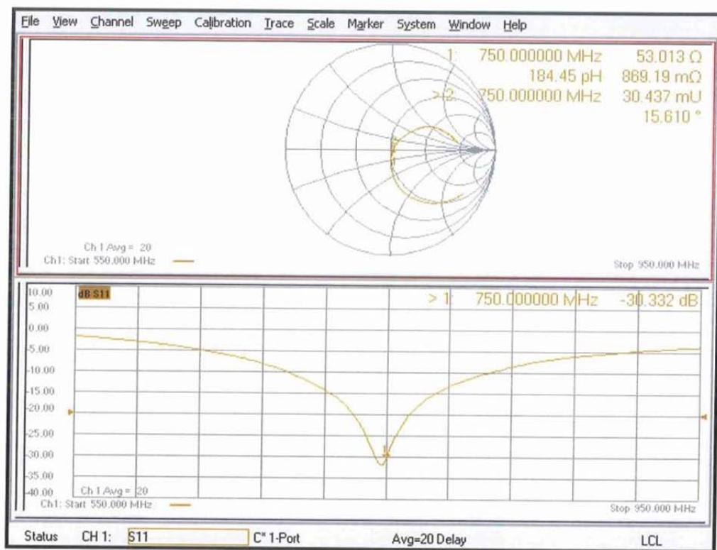
**D750V3 - SN:1230 Extended Dipole Calibrations**
