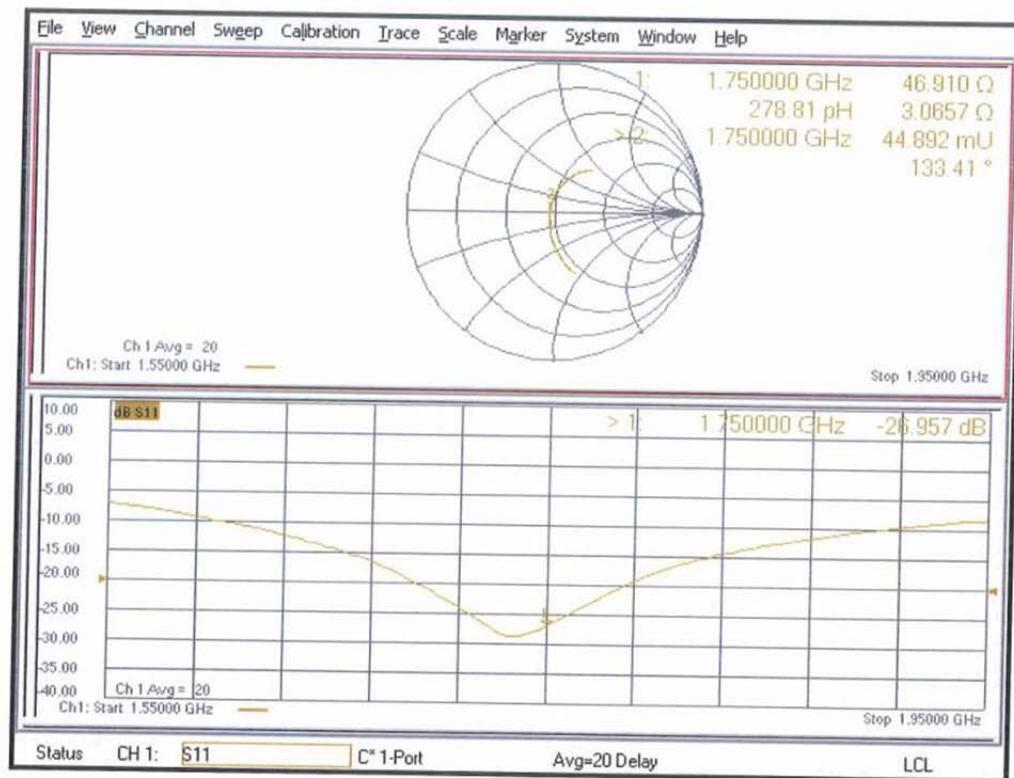
**D1750V2 - SN:1200 Extended Dipole Calibrations**
