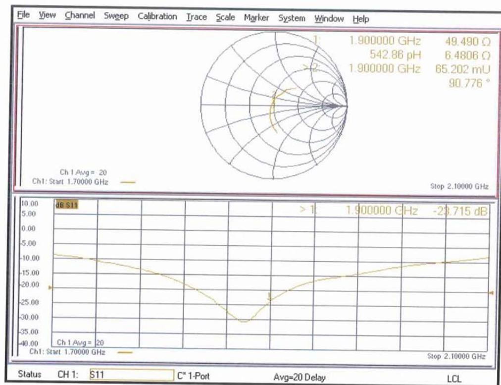
**D1900V2 - SN:5d251 Extended Dipole Calibrations**
