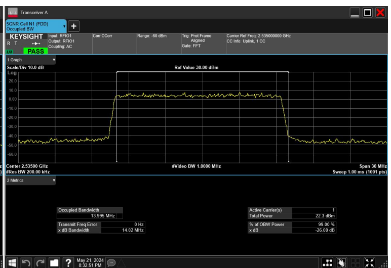
15MHz_15kHz_2535MHz_DFT-s-OFDM \pi/2 BPSK_RB75@0
