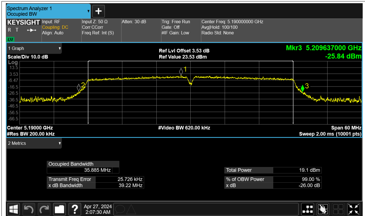
-26dB Bandwidth NVNT ac40 5230MHz Ant14
