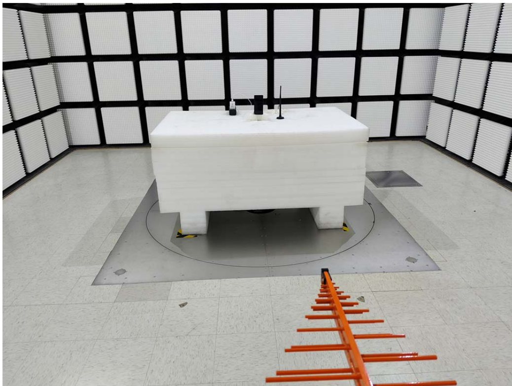
Radiated Emission 30 MHz-1 GHz View
