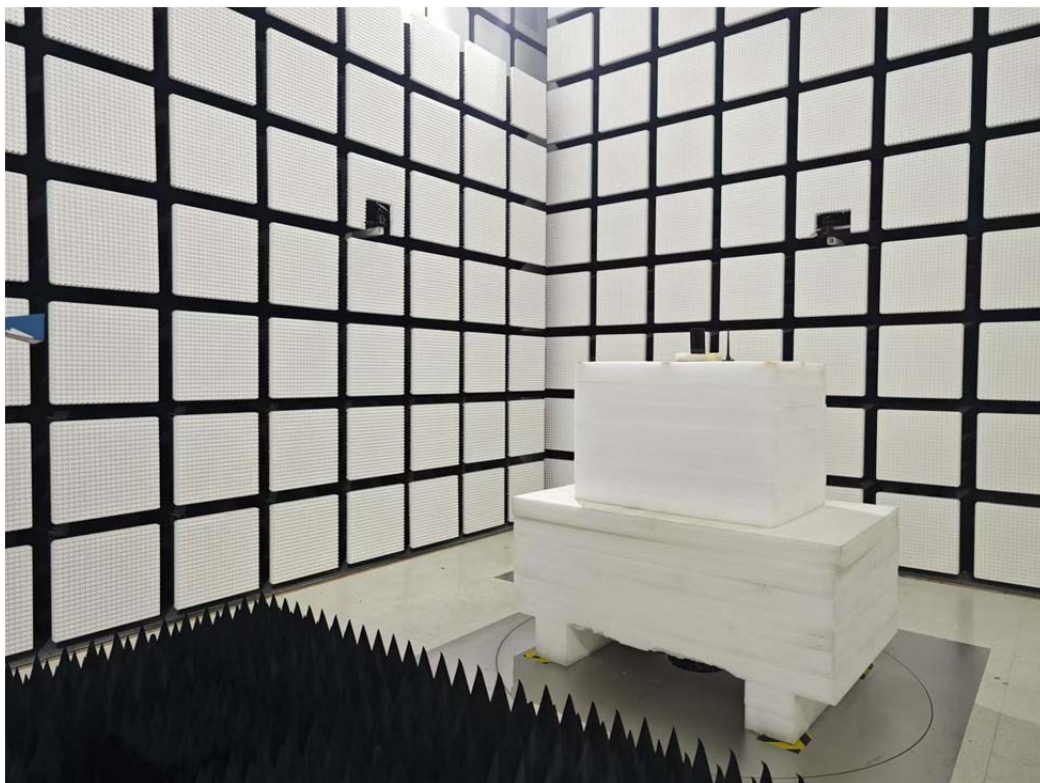
Radiated Emission Above 18-26.5GHz View
