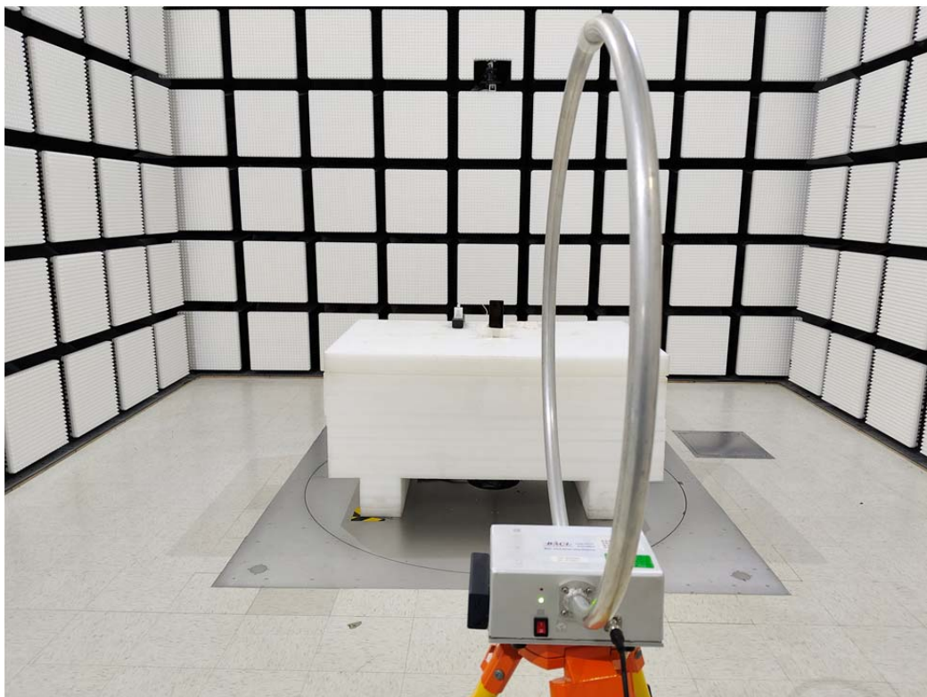
Radiated Emission 9 kHz-30 MHz Perpendicular View
