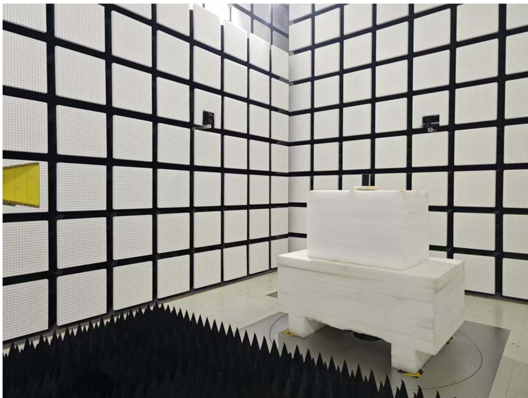
Radiated Emission Above 1-18GHz View
