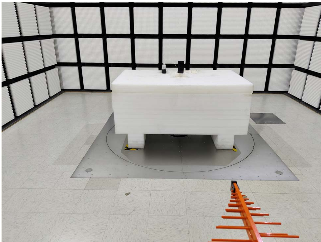
Radiated Emission 30 MHz-1 GHz View
