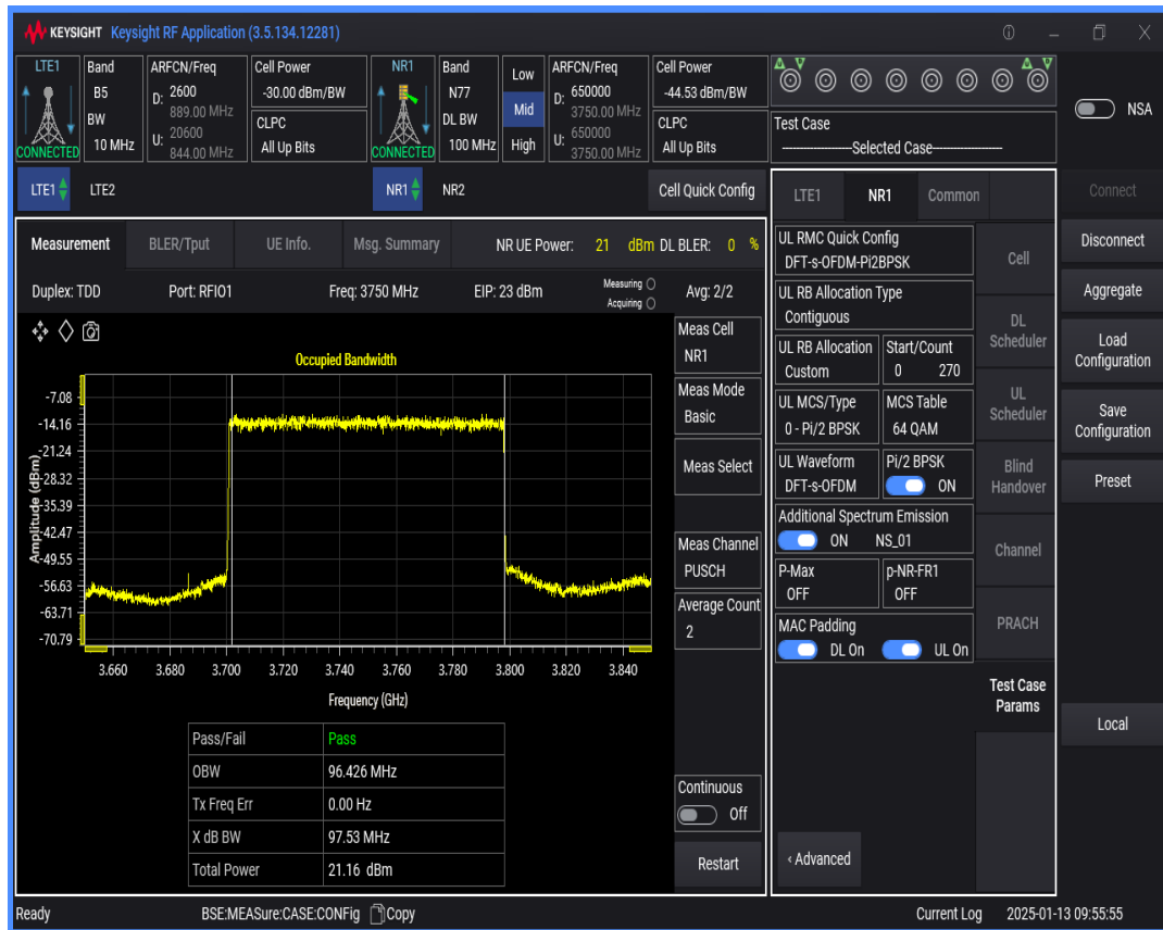
n77 SCS=30kHz DFT_BPSK BW=15MHz Channel=650000 RB=36@0
