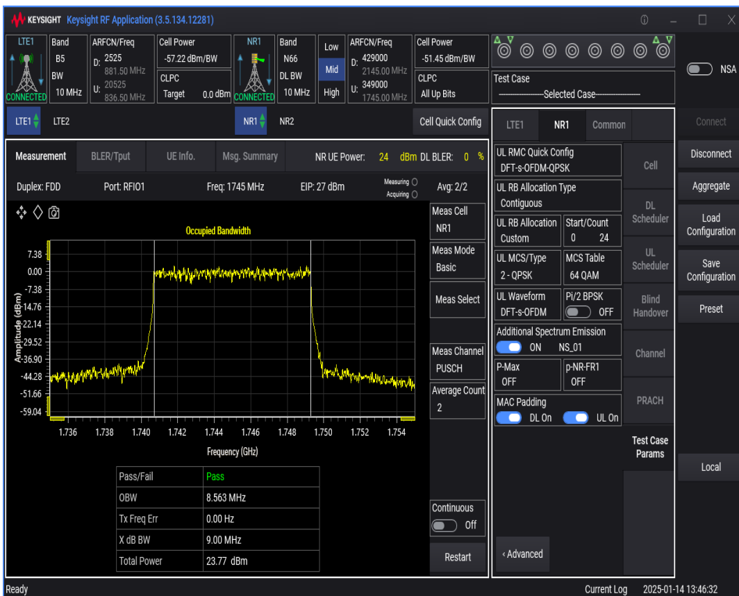
n66 SCS=30kHz DFT_QPSK BW=15MHz Channel=349000 RB=36@0
