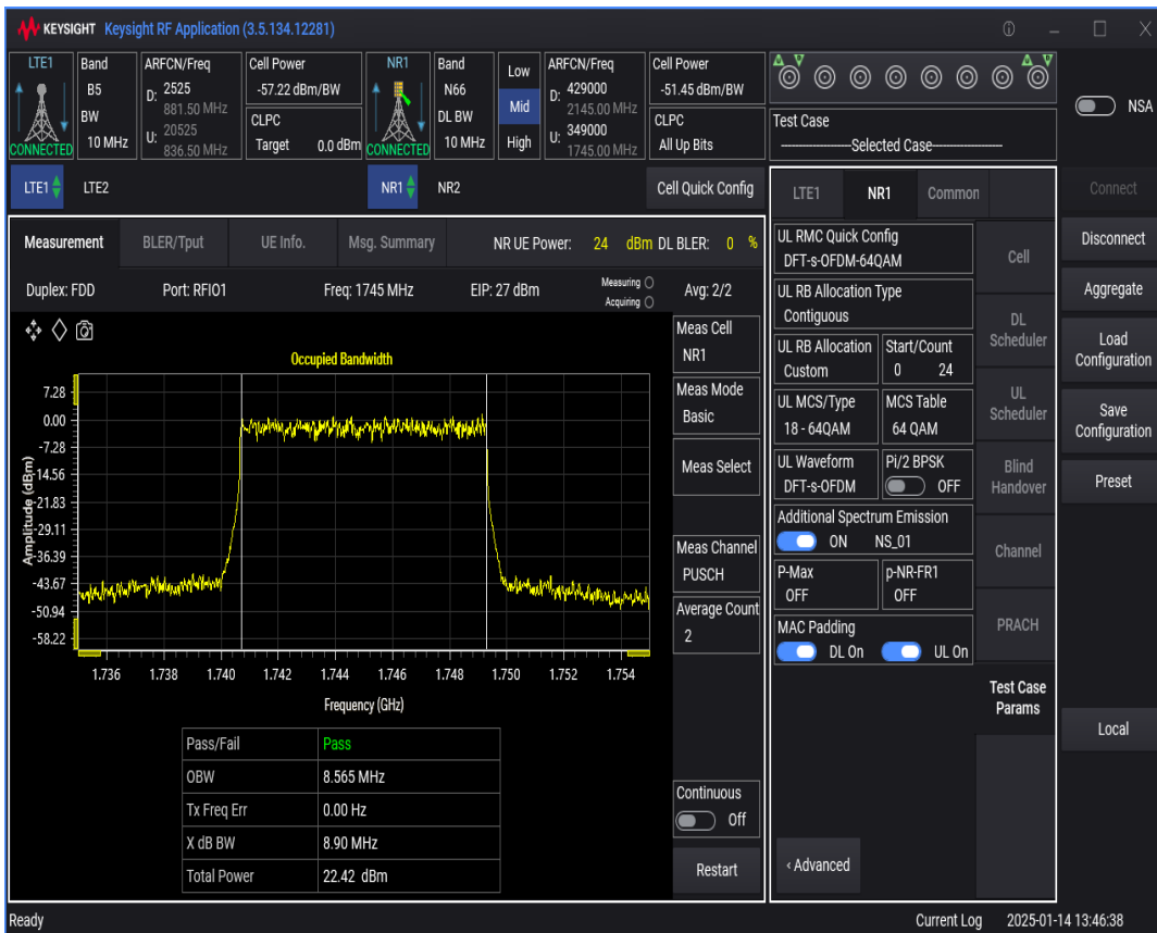
n66 SCS=30kHz DFT_QAM64 BW=15MHz Channel=349000 RB=36@0
