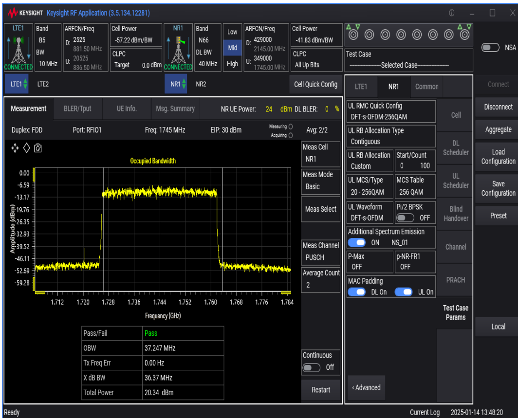
n66 SCS=30kHz DFT_QAM64 BW=10MHz Channel=349000 RB=24@0
