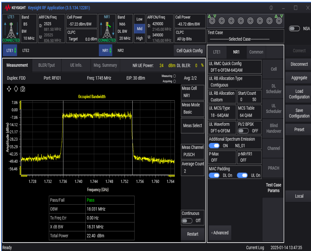
n66 SCS=30kHz DFT_QAM64 BW=40MHz Channel=349000 RB=100@0
