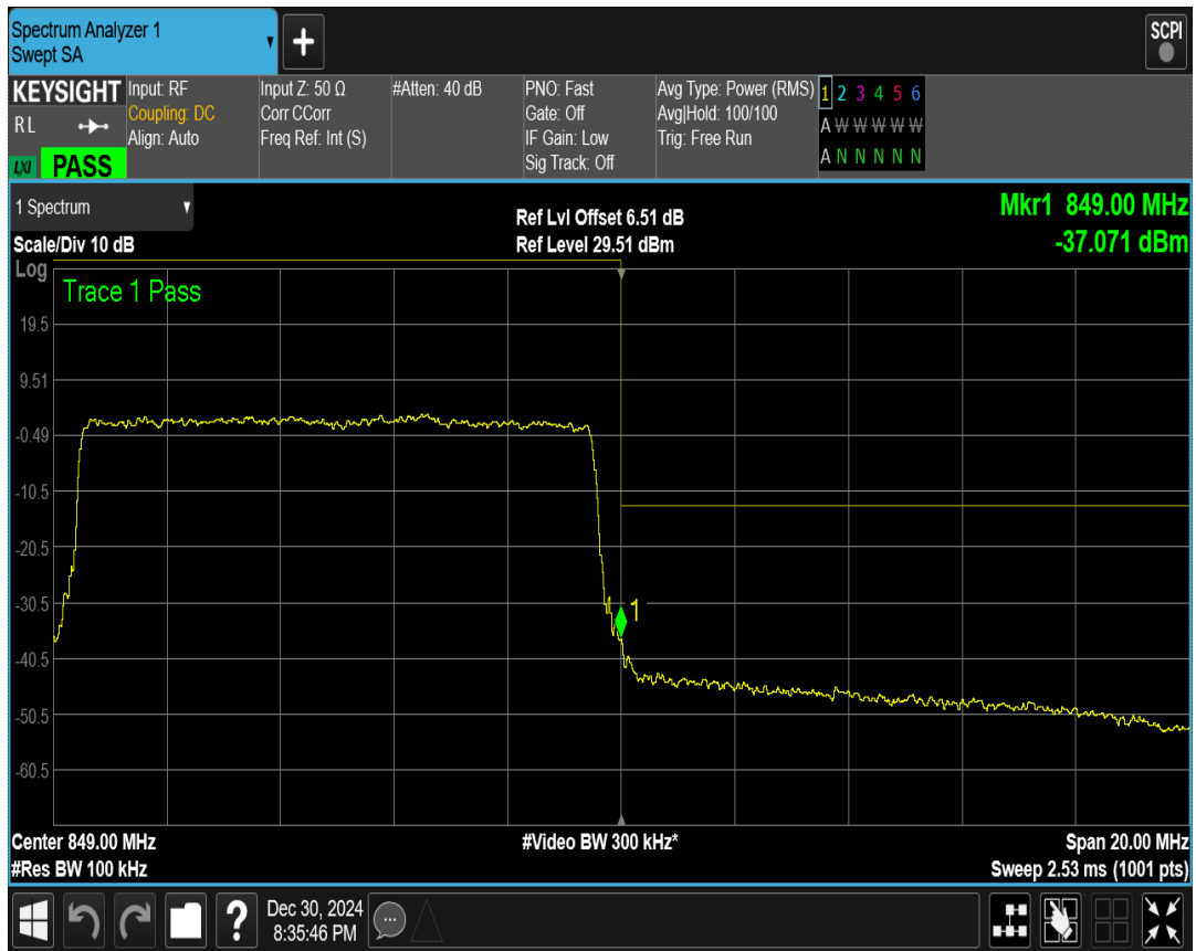
Band5 QPSK BW=3MHz Channel=20635 RB Size=15 Position=#0
