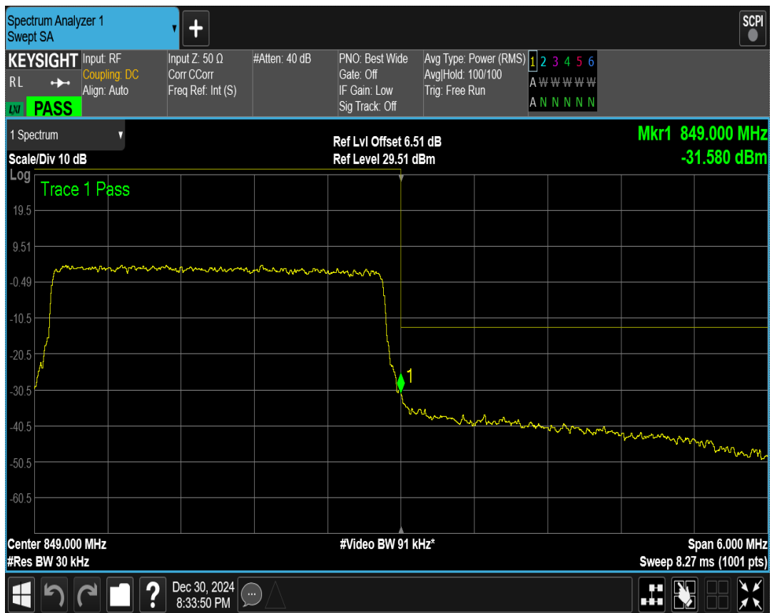
Band5 QPSK BW=3MHz Channel=20415 RB Size=15 Position=#0
