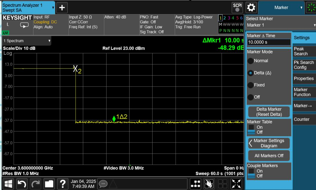
Setup with frequency 3610-3630MHz and power level 5dBm/MHz
