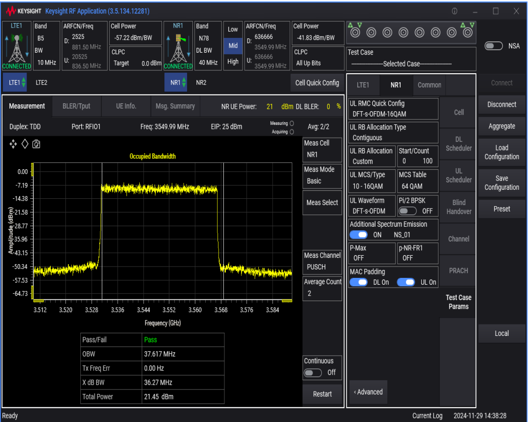
n78 SCS=30kHz DFT_QAM16 BW=60MHz Channel=636666 RB=162@0
