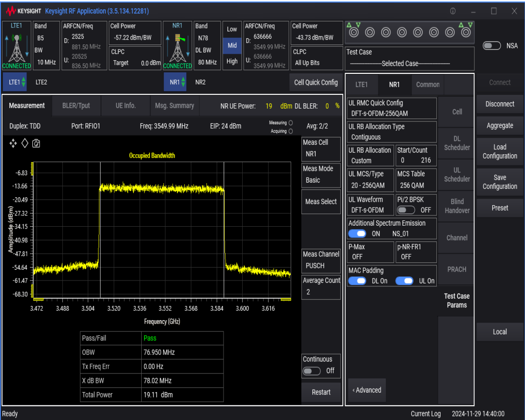
n78 SCS=30kHz DFT_QAM256 BW=40MHz Channel=636666 RB=100@0
