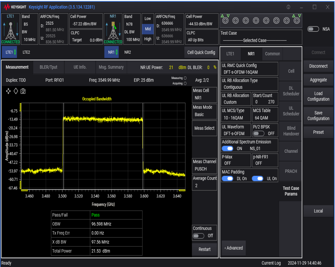
n78 SCS=30kHz DFT_BPSK BW=90MHz Channel=636666 RB=240@0
