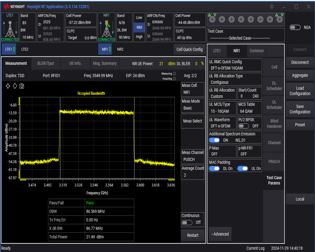
n78 SCS=30kHz DFT_QAM16 BW=80MHz Channel=636666 RB=216@0
