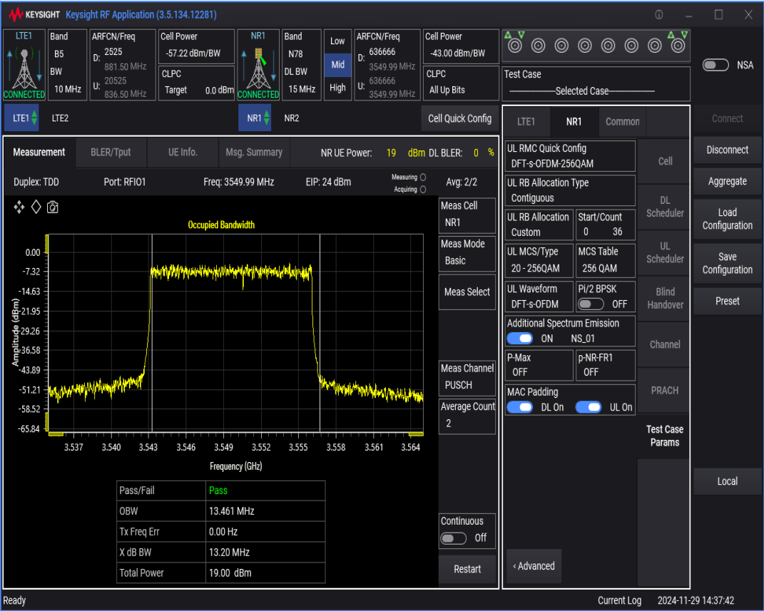
n78 SCS=30kHz DFT_QAM64 BW=60MHz Channel=636666 RB=162@0
