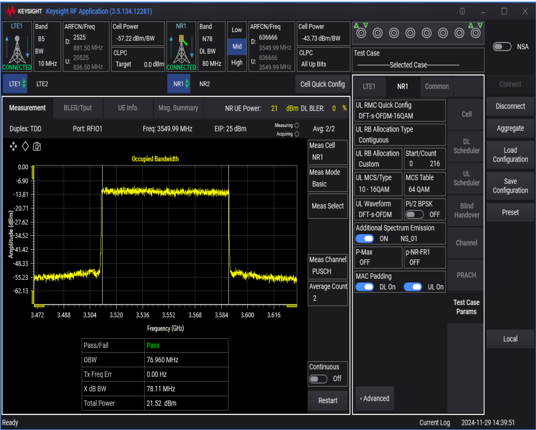
n78 SCS=30kHz DFT_QAM16 BW=100MHz Channel=636666 RB=270@0
