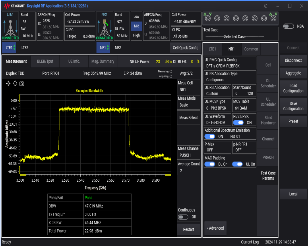
n78 SCS=30kHz DFT_BPSK BW=40MHz Channel=636666 RB=100@0
