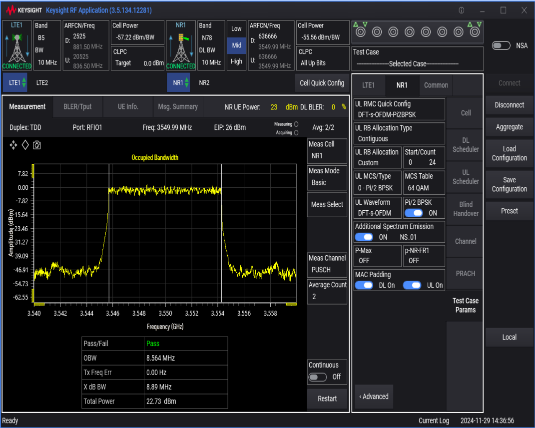
n78 SCS=30kHz DFT_BPSK BW=100MHz Channel=636666 RB=270@0
