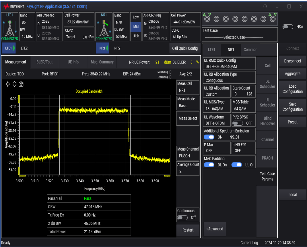
n78 SCS=30kHz DFT_QAM64 BW=80MHz Channel=636666 RB=216@0
