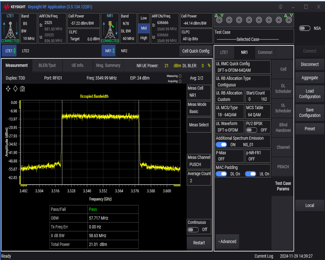
n78 SCS=30kHz DFT_QAM64 BW=50MHz Channel=636666 RB=128@0
