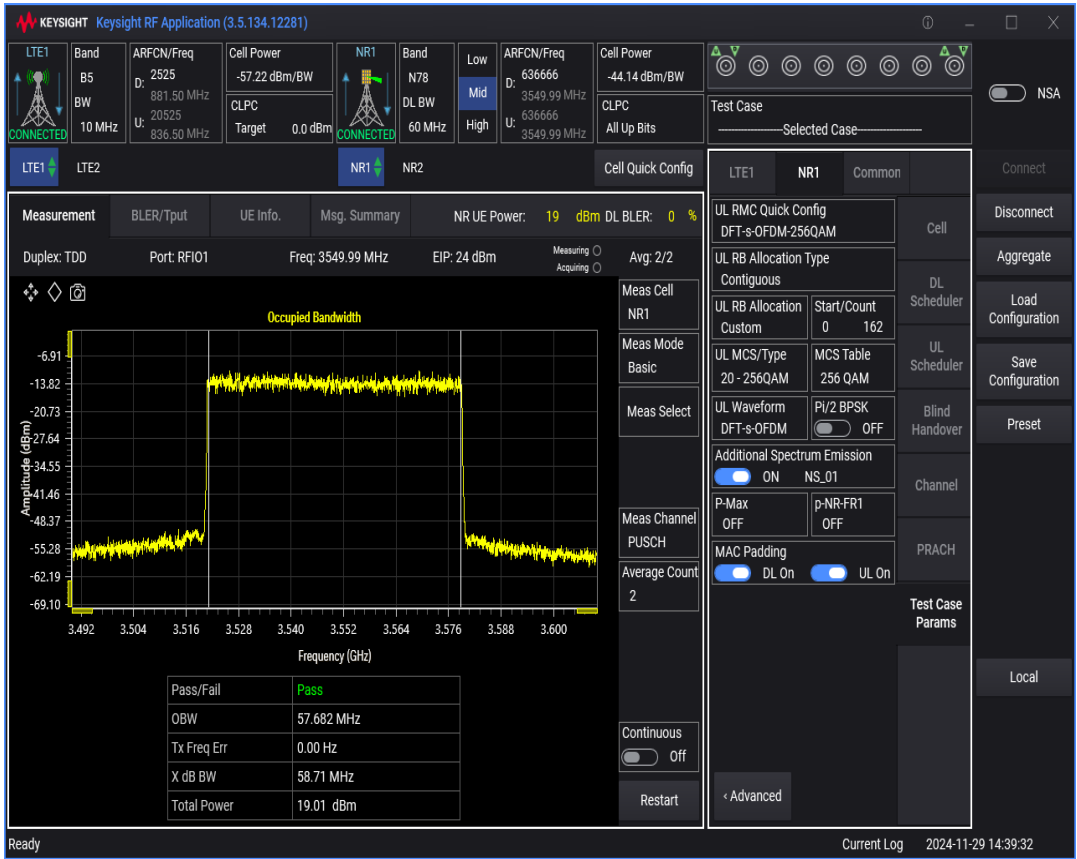
n78 SCS=30kHz DFT_QAM256 BW=50MHz Channel=636666 RB=128@0
