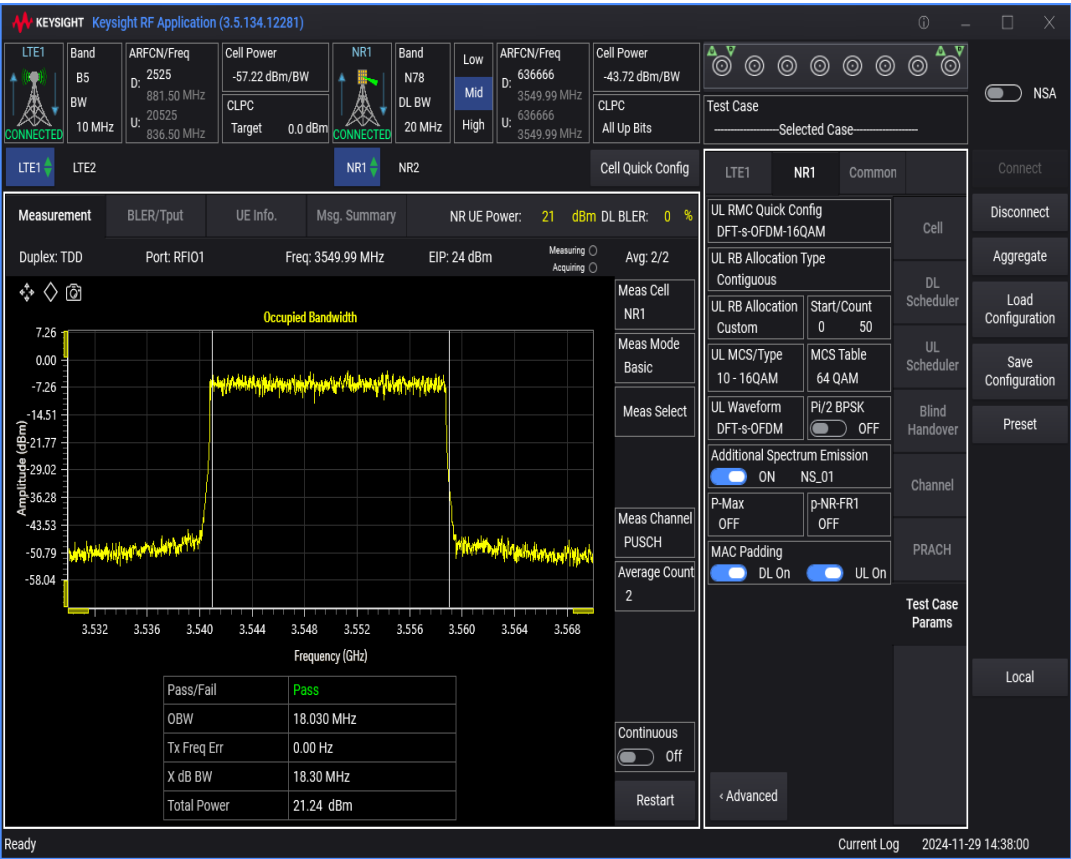
n78 SCS=30kHz DFT_QAM16 BW=15MHz Channel=636666 RB=36@0
