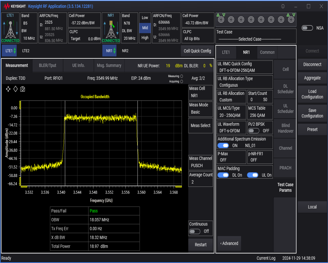
n78 SCS=30kHz DFT_QAM256 BW=15MHz Channel=636666 RB=36@0
