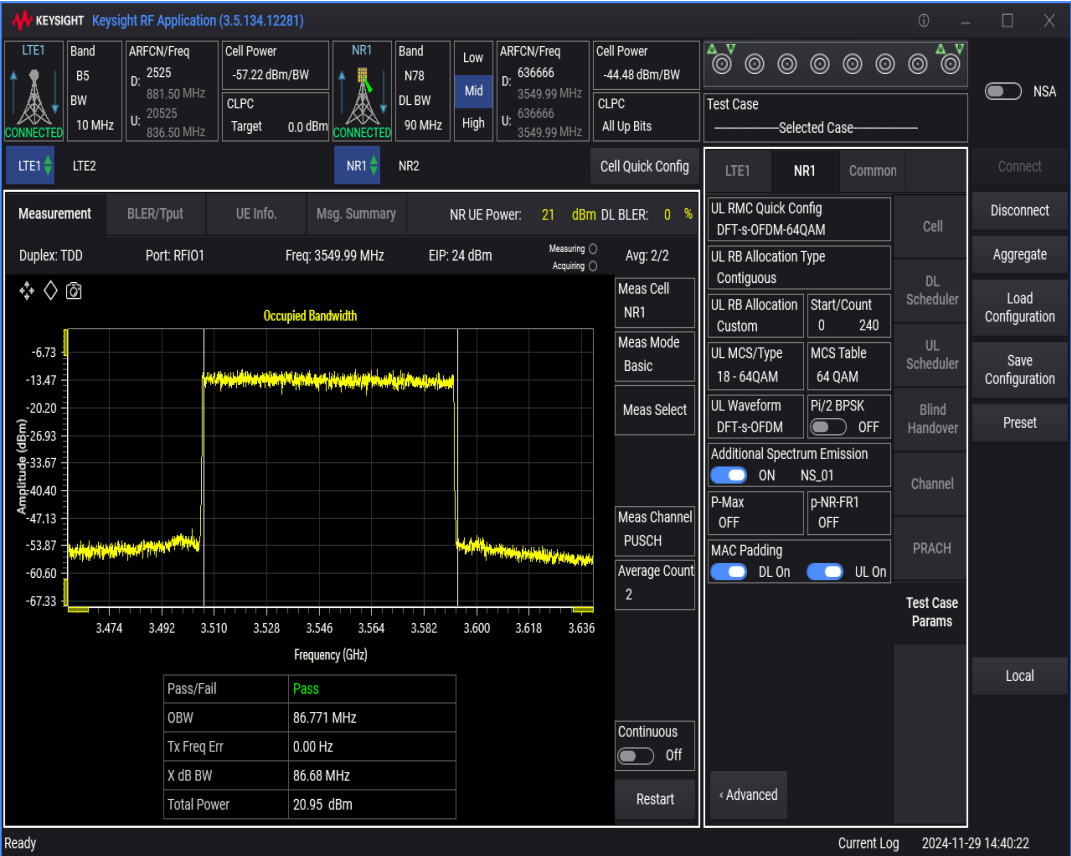
n78 SCS=30kHz DFT_QAM64 BW=10MHz Channel=636666 RB=24@0
