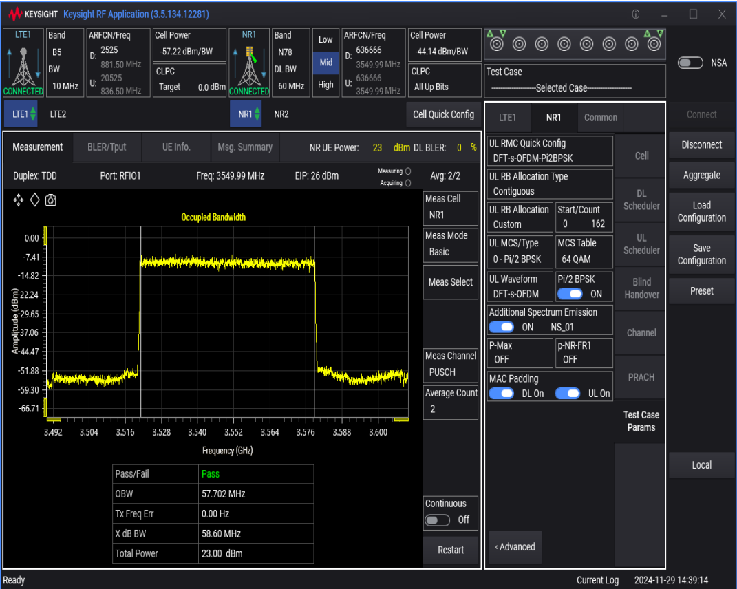
n78 SCS=30kHz DFT_BPSK BW=10MHz Channel=636666 RB=24@0
