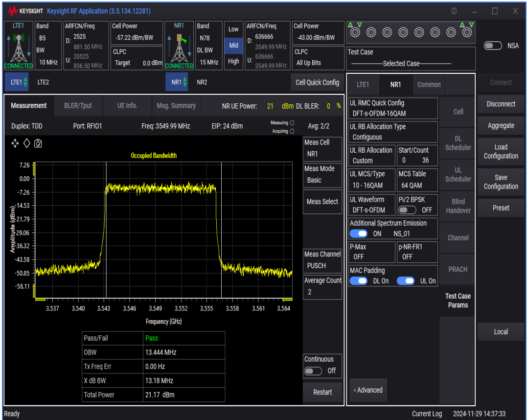
n78 SCS=30kHz DFT_QAM256 BW=60MHz Channel=636666 RB=162@0
