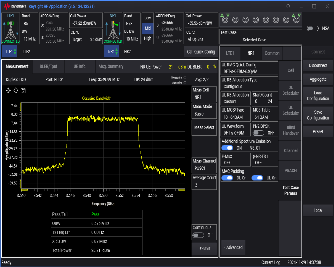
n78 SCS=30kHz DFT_QAM64 BW=100MHz Channel=636666 RB=270@0
