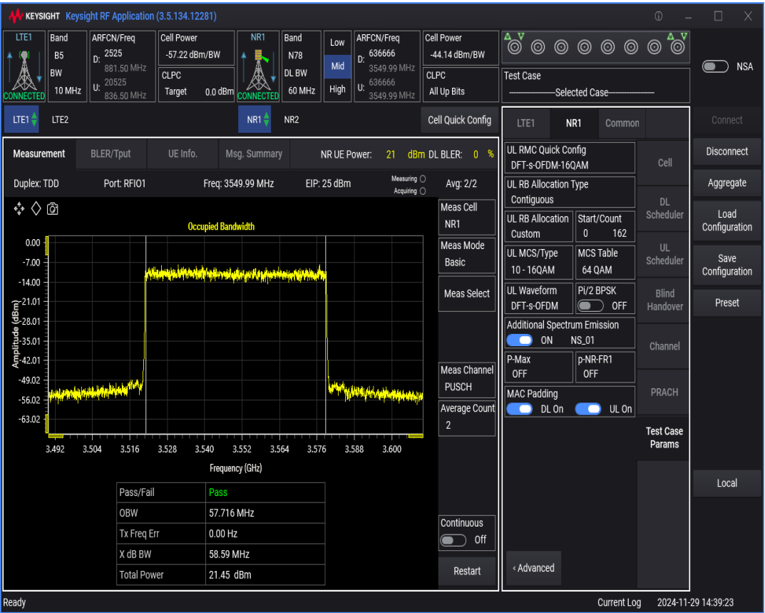
n78 SCS=30kHz DFT_QAM16 BW=90MHz Channel=636666 RB=240@0
