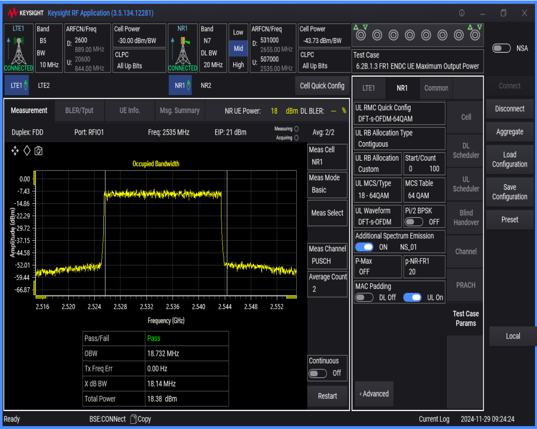
n7 SCS=15kHz DFT_QAM64 BW=15MHz Channel=507000 RB=75@0
