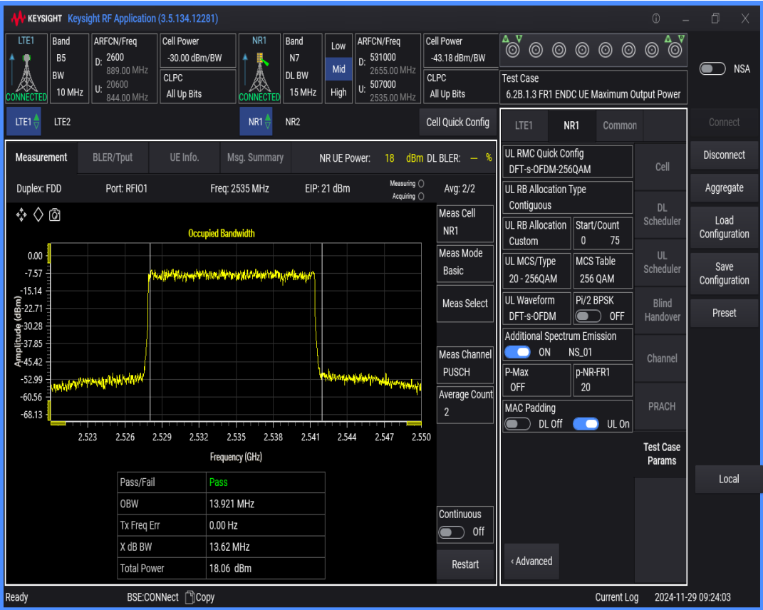
n7 SCS=15kHz DFT_QAM64 BW=20MHz Channel=507000 RB=100@0
