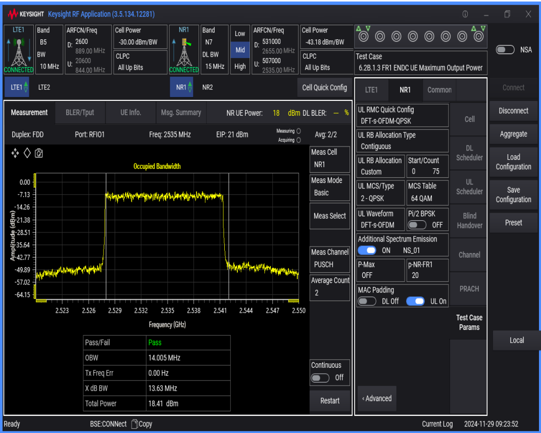
n7 SCS=15kHz DFT_QAM64 BW=5MHz Channel=507000 RB=25@0
