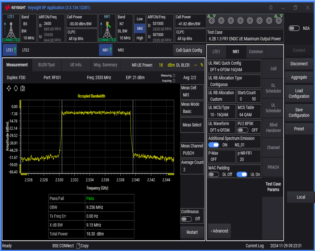
n7 SCS=15kHz DFT_QAM16 BW=15MHz Channel=507000 RB=75@0
