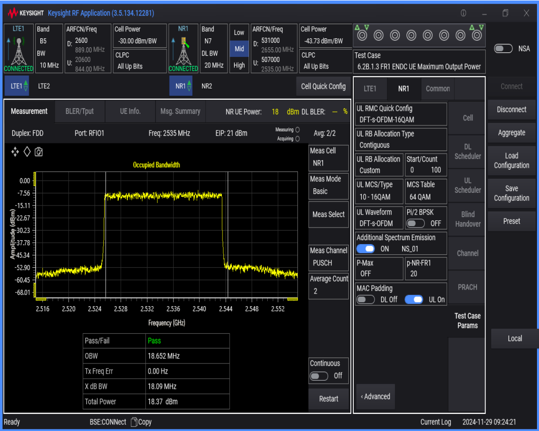
n7 SCS=15kHz DFT_BPSK BW=5MHz Channel=507000 RB=25@0
