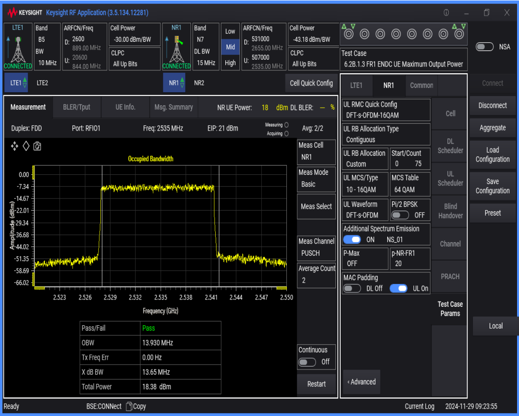
n7 SCS=15kHz DFT_QAM16 BW=20MHz Channel=507000 RB=100@0
