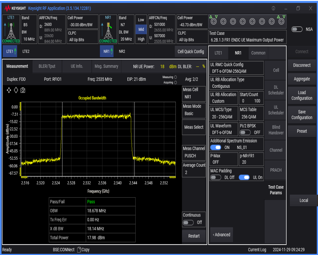
n7 SCS=15kHz DFT_QAM256 BW=5MHz Channel=507000 RB=25@0
