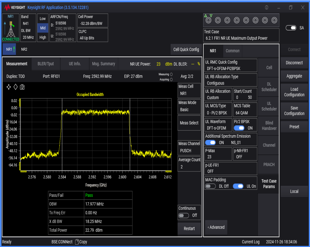
n41 SCS=30kHz DFT_BPSK BW=60MHz Channel=518598 RB=162@0
