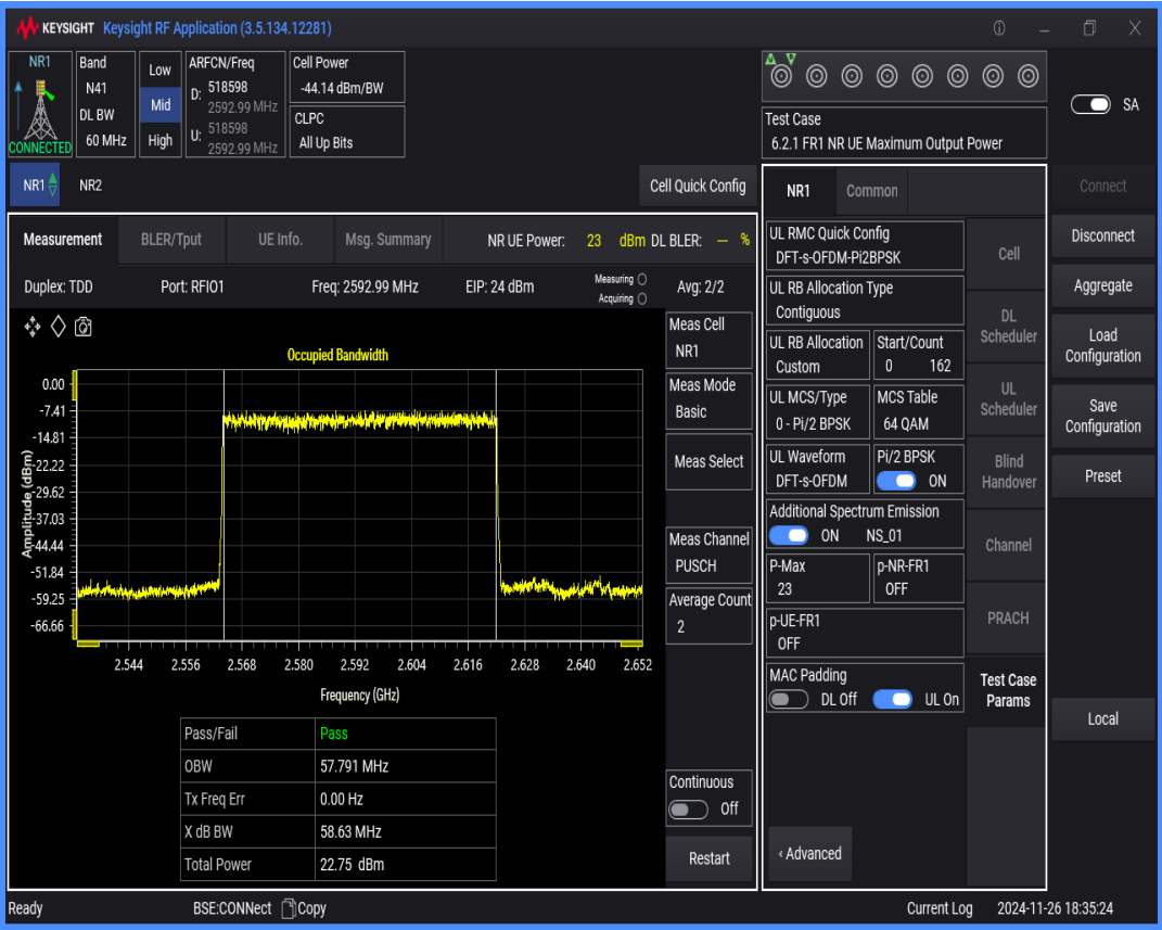
n41 SCS=30kHz DFT_BPSK BW=50MHz Channel=518598 RB=128@0
