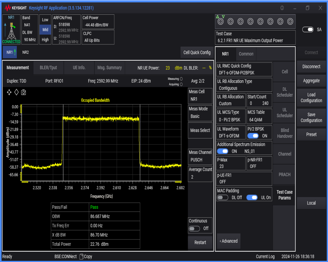
n41 SCS=30kHz DFT_BPSK BW=80MHz Channel=518598 RB=216@0
