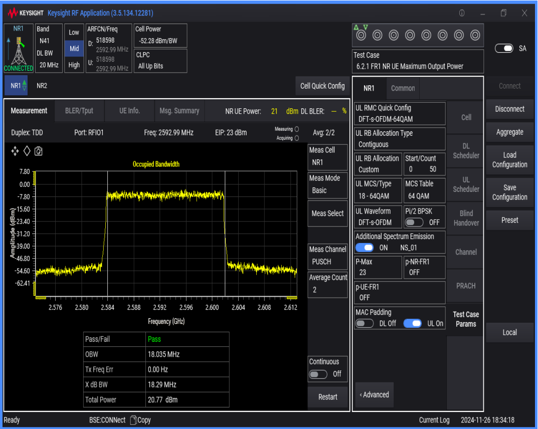
n41 SCS=30kHz DFT_QAM64 BW=100MHz Channel=518598 RB=270@0
