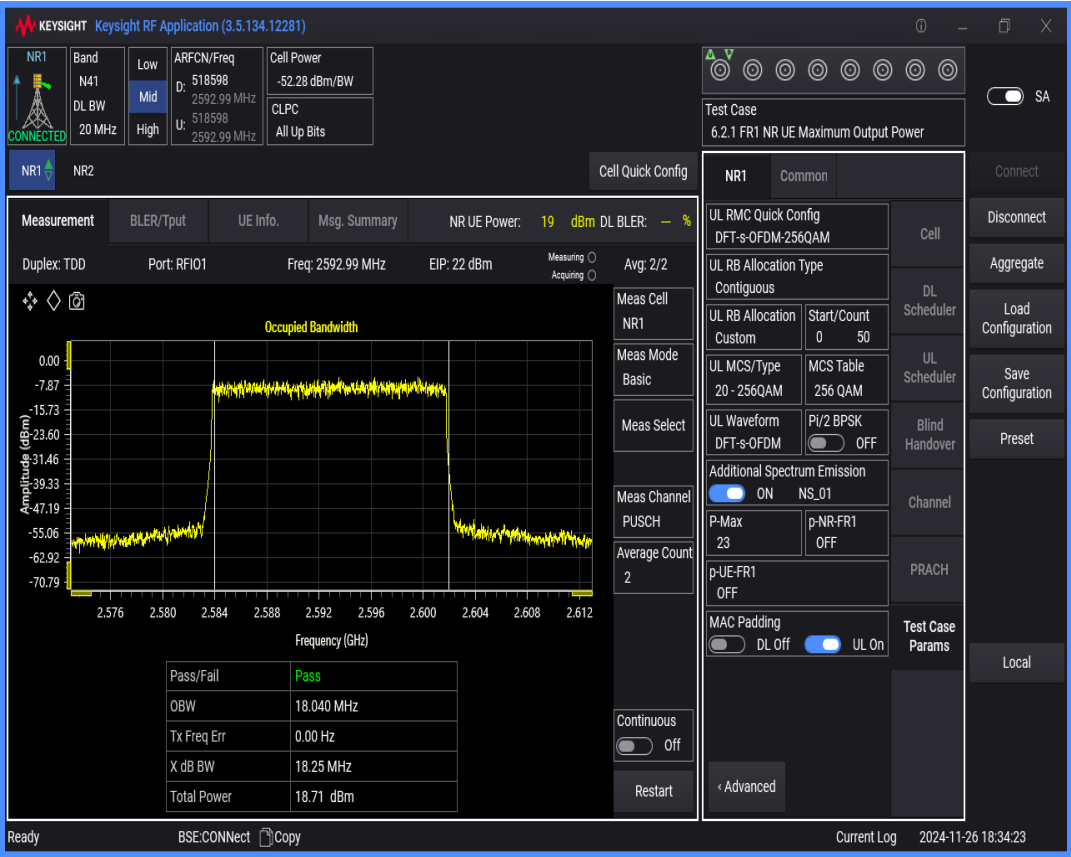
n41 SCS=30kHz DFT_QAM256 BW=50MHz Channel=518598 RB=128@0
