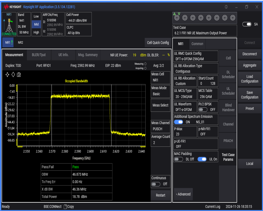
n41 SCS=30kHz DFT_QAM256 BW=40MHz Channel=518598 RB=100@0
