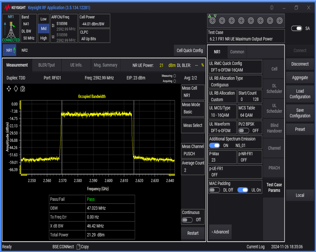
n41 SCS=30kHz DFT_QAM16 BW=40MHz Channel=518598 RB=100@0
