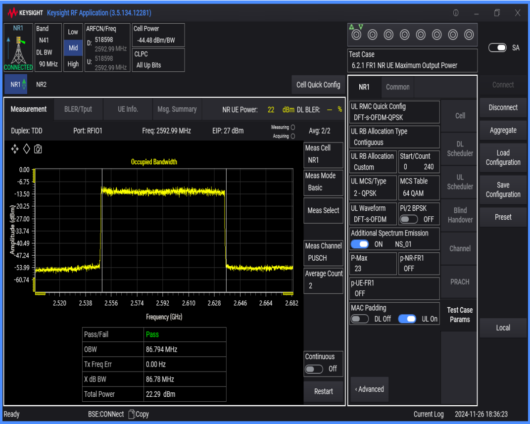
n41 SCS=30kHz DFT_QPSK BW=60MHz Channel=518598 RB=162@0
