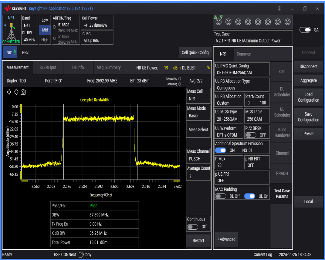
n41 SCS=30kHz DFT_QAM256 BW=90MHz Channel=518598 RB=240@0
