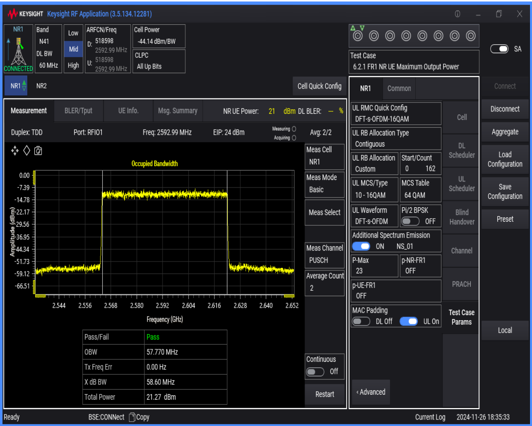
n41 SCS=30kHz DFT_QAM16 BW=80MHz Channel=518598 RB=216@0
