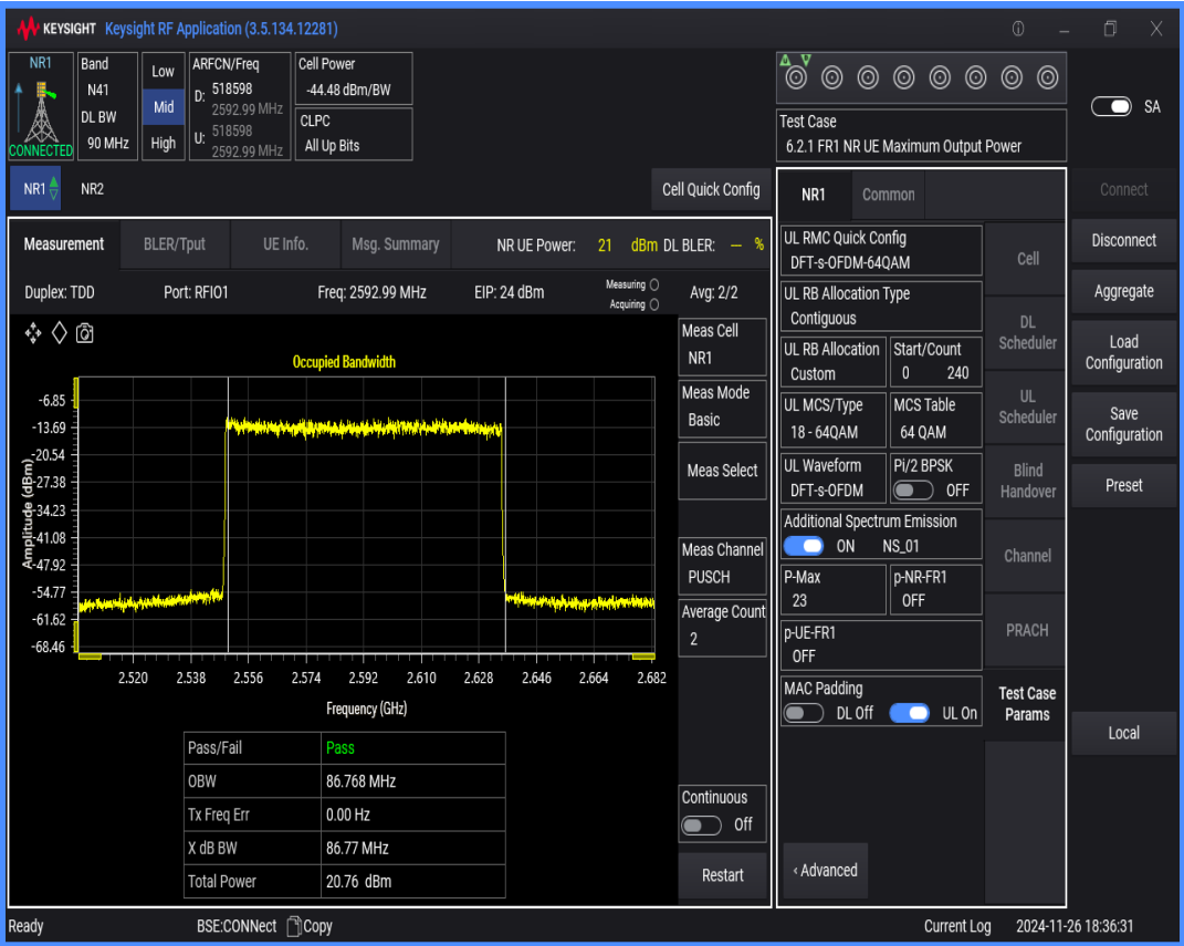
n41 SCS=30kHz DFT_QPSK BW=100MHz Channel=518598 RB=270@0
