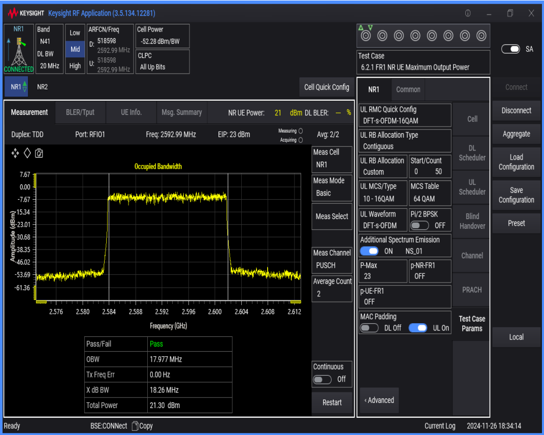
n41 SCS=30kHz DFT_QAM16 BW=60MHz Channel=518598 RB=162@0
