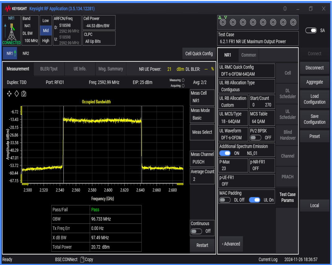
n41 SCS=30kHz DFT_QAM64 BW=90MHz Channel=518598 RB=240@0
