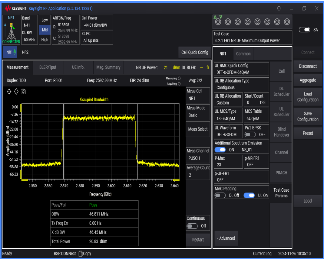
n41 SCS=30kHz DFT_QAM64 BW=60MHz Channel=518598 RB=162@0
