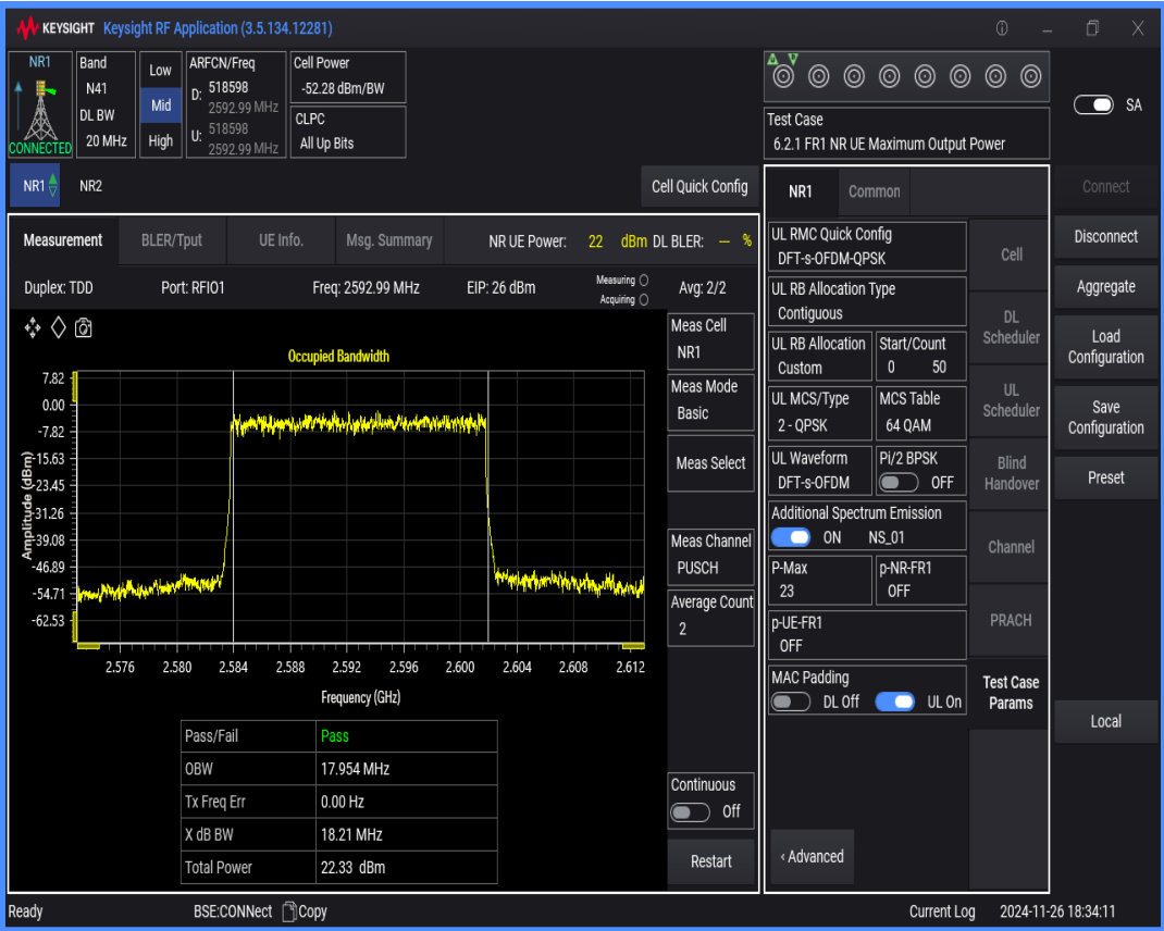
n41 SCS=30kHz DFT_QAM64 BW=50MHz Channel=518598 RB=128@0
