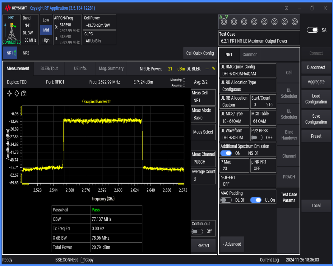
n41 SCS=30kHz DFT_QPSK BW=80MHz Channel=518598 RB=216@0
