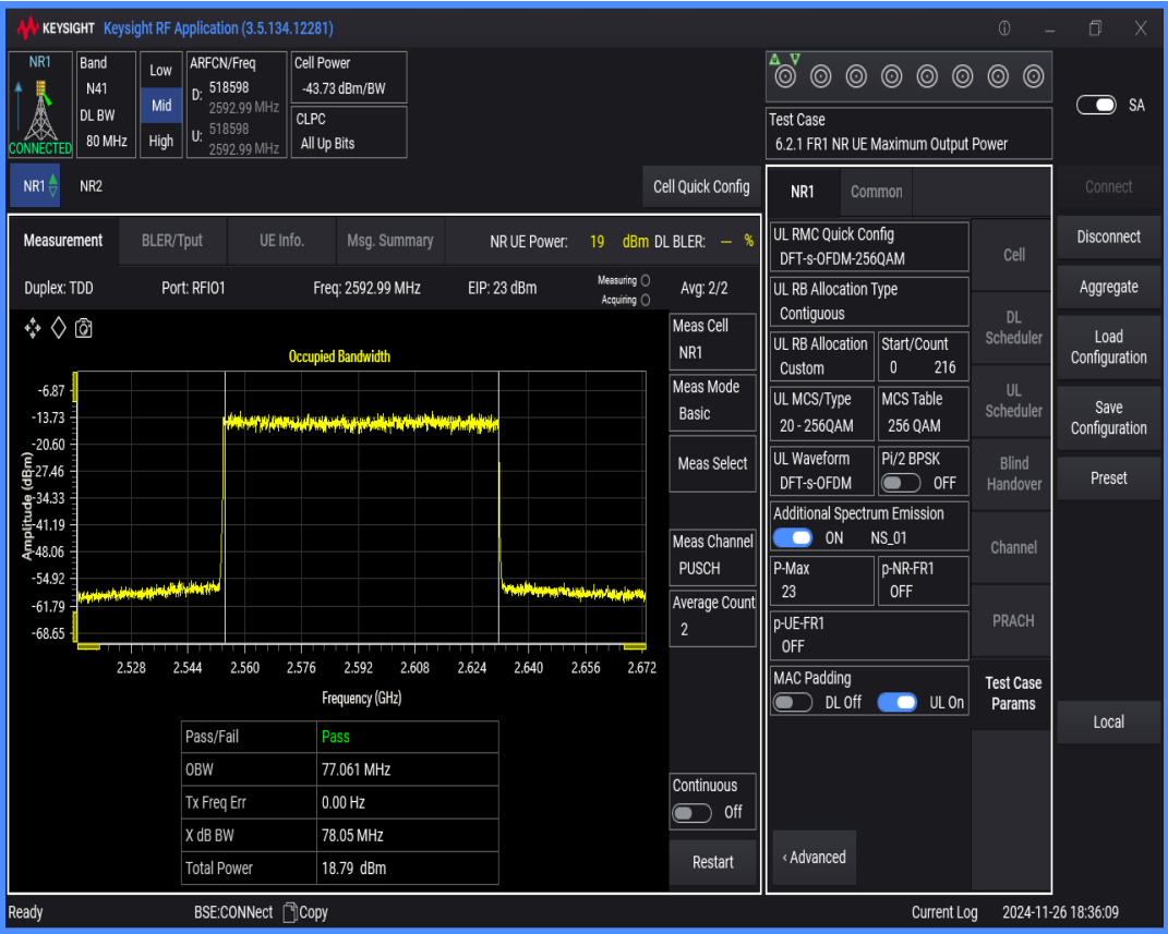
n41 SCS=30kHz DFT_QAM256 BW=60MHz Channel=518598 RB=162@0
