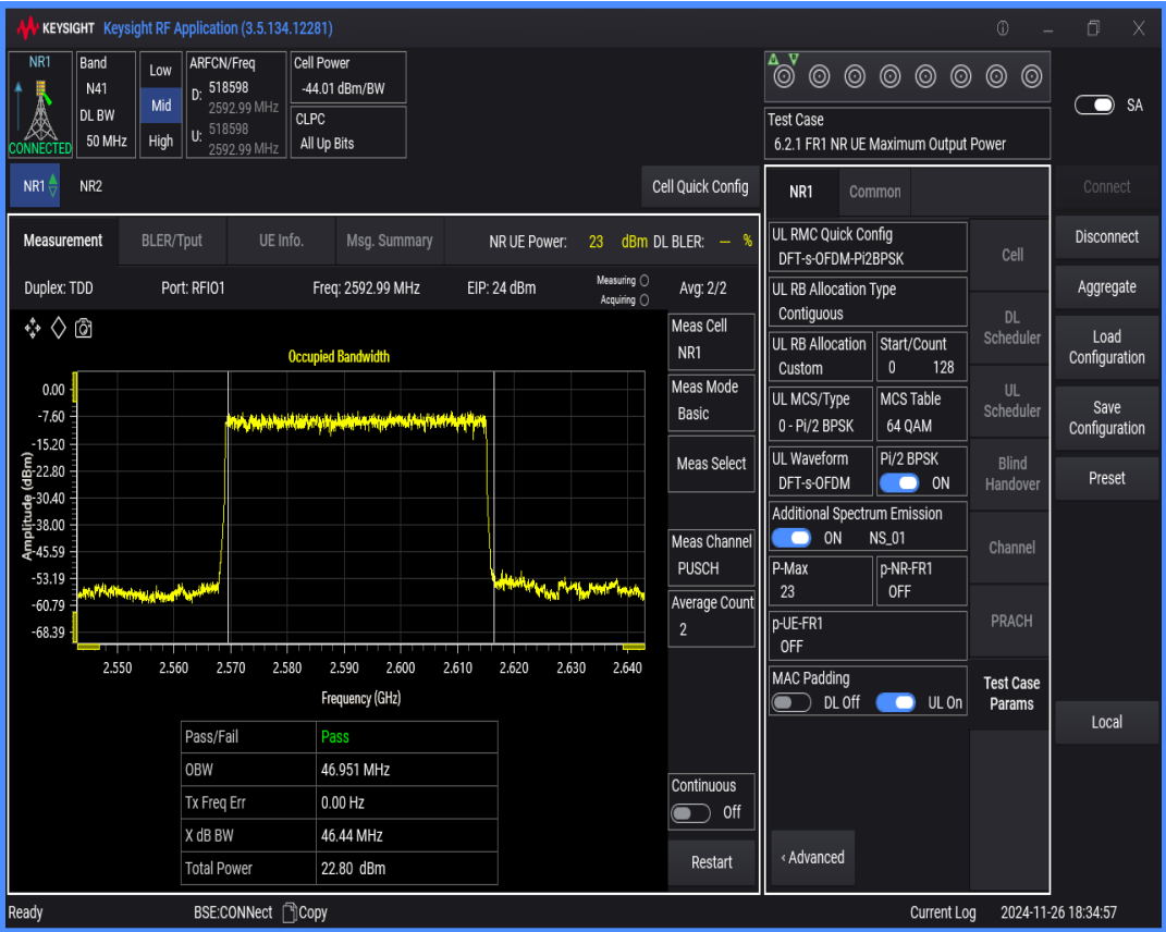
n41 SCS=30kHz DFT_QAM16 BW=100MHz Channel=518598 RB=270@0
