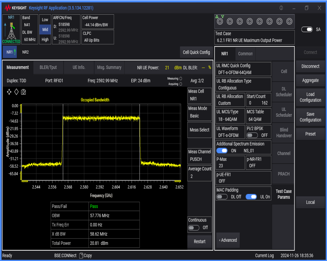
n41 SCS=30kHz DFT_QAM64 BW=80MHz Channel=518598 RB=216@0
