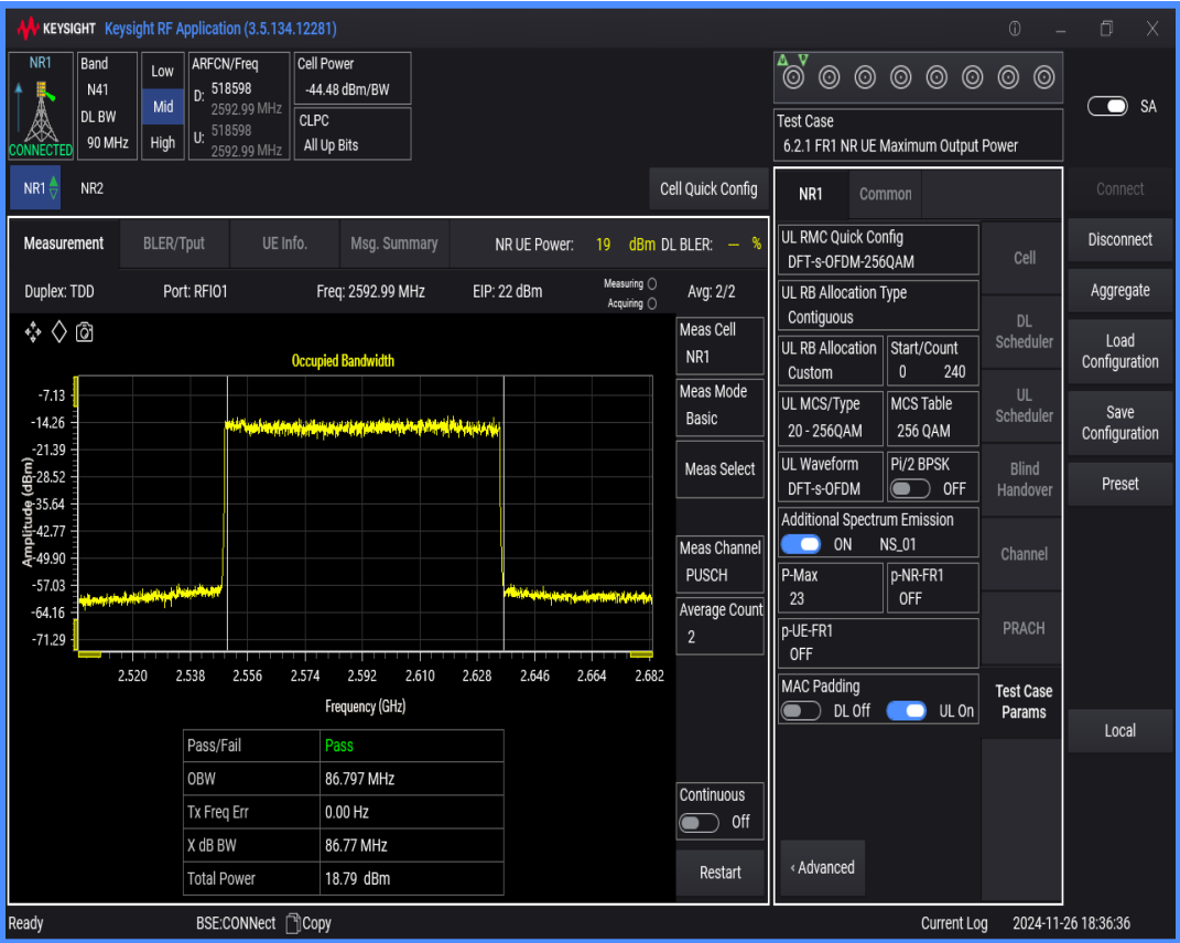
n41 SCS=30kHz DFT_QAM256 BW=80MHz Channel=518598 RB=216@0
