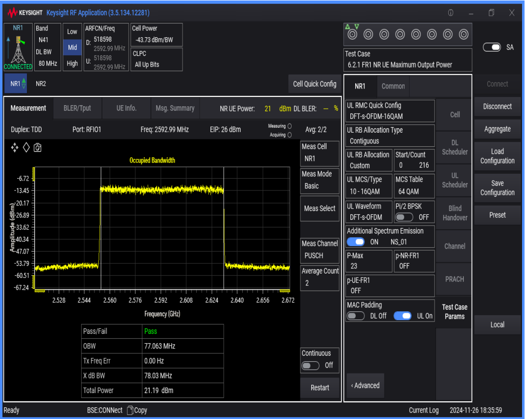
n41 SCS=30kHz DFT_QAM16 BW=90MHz Channel=518598 RB=240@0
