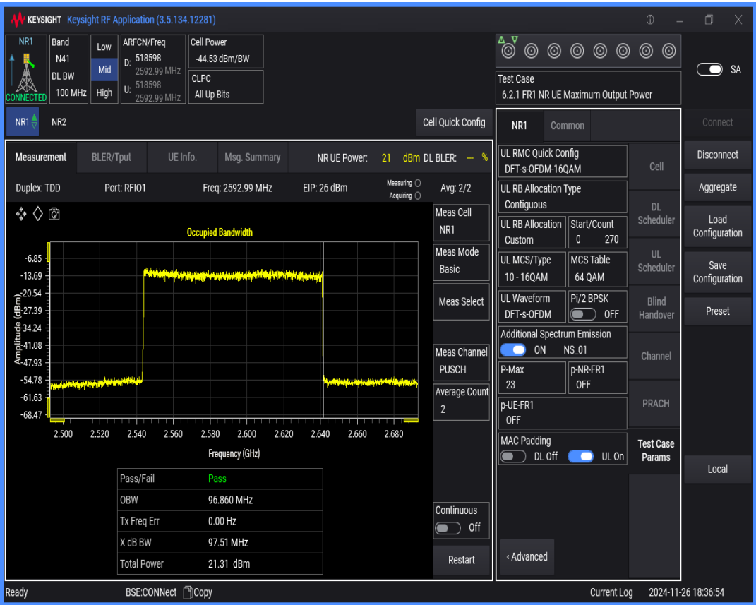
n41 SCS=30kHz DFT_BPSK BW=90MHz Channel=518598 RB=240@0
