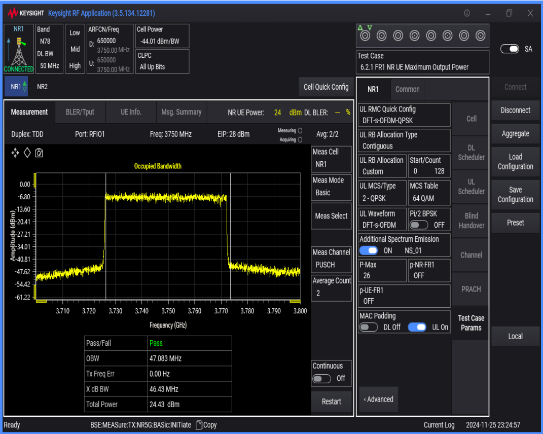
n78(3700-3800) SCS=30kHz DFT_QPSK BW=40MHz Channel=650000 RB=100@0
