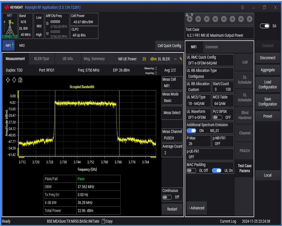
n78(3700-3800) SCS=30kHz DFT_QAM64 BW=50MHz Channel=650000 RB=128@0
