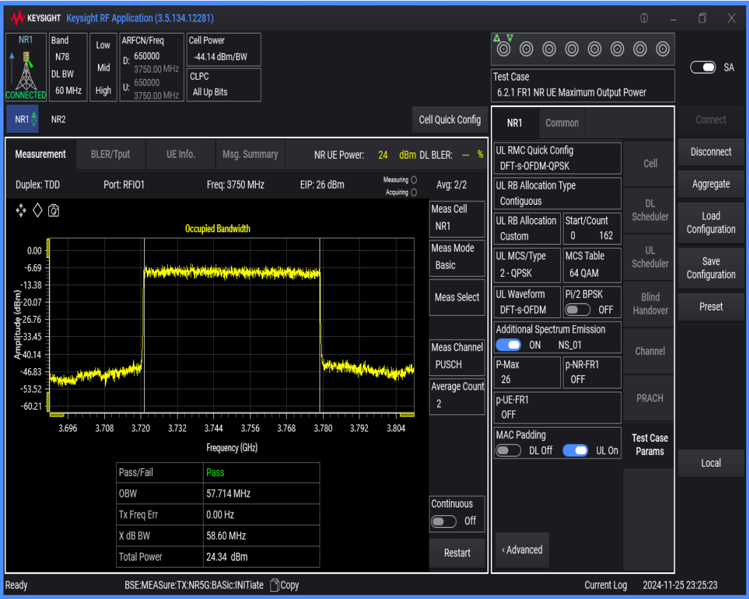
n78(3700-3800) SCS=30kHz DFT_QPSK BW=90MHz Channel=650000 RB=240@0
