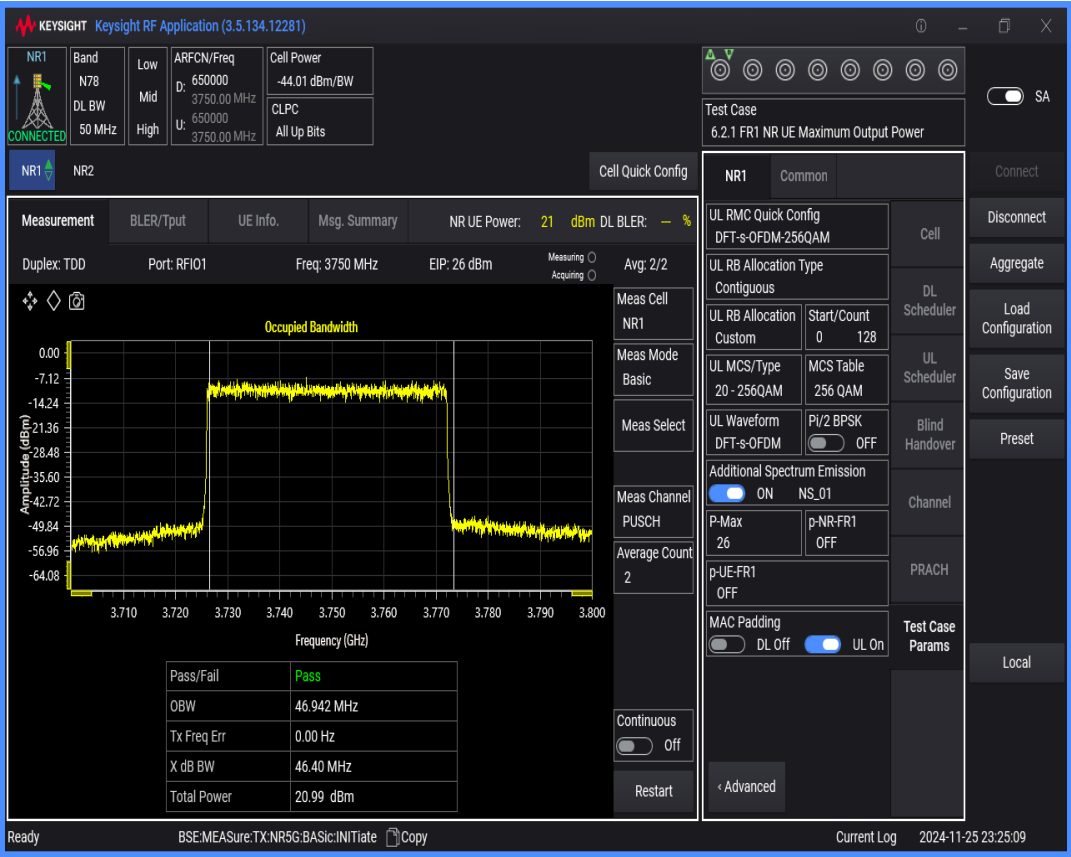
n78(3700-3800) SCS=30kHz DFT_QAM64 BW=100MHz Channel=650000 RB=270@0
