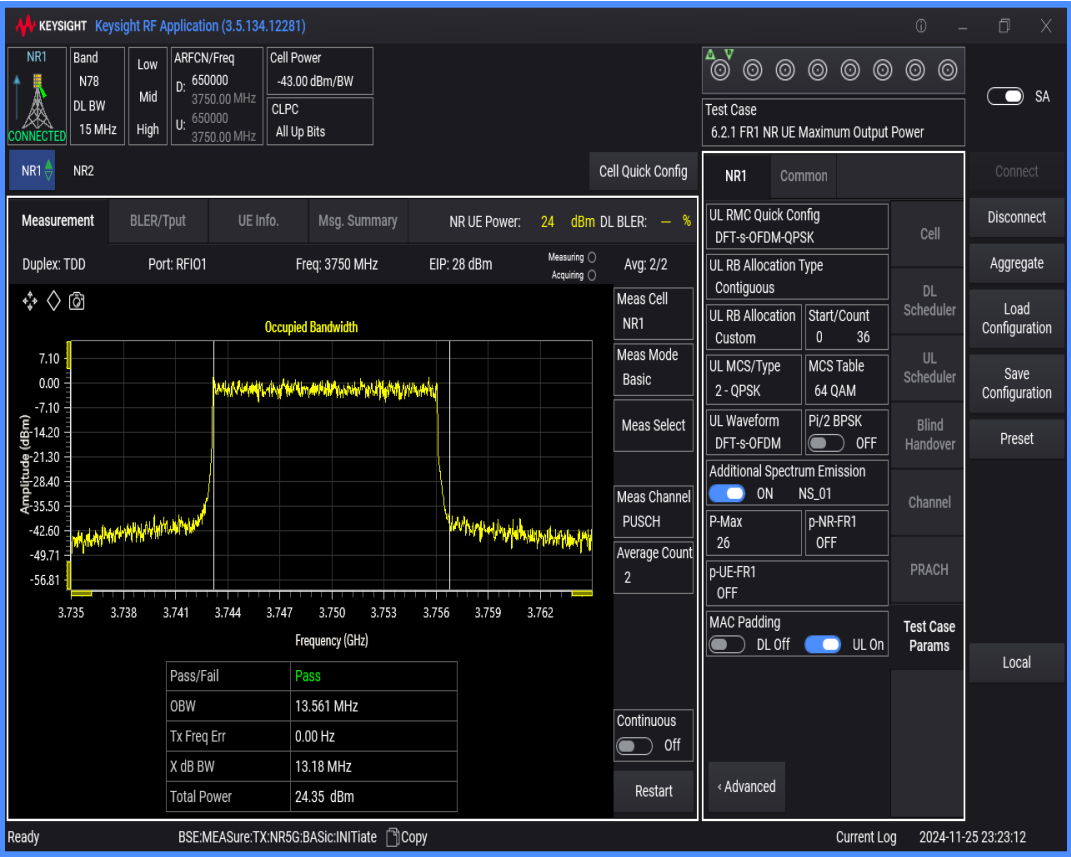
n78(3700-3800) SCS=30kHz DFT_QPSK BW=10MHz Channel=650000 RB=24@0
