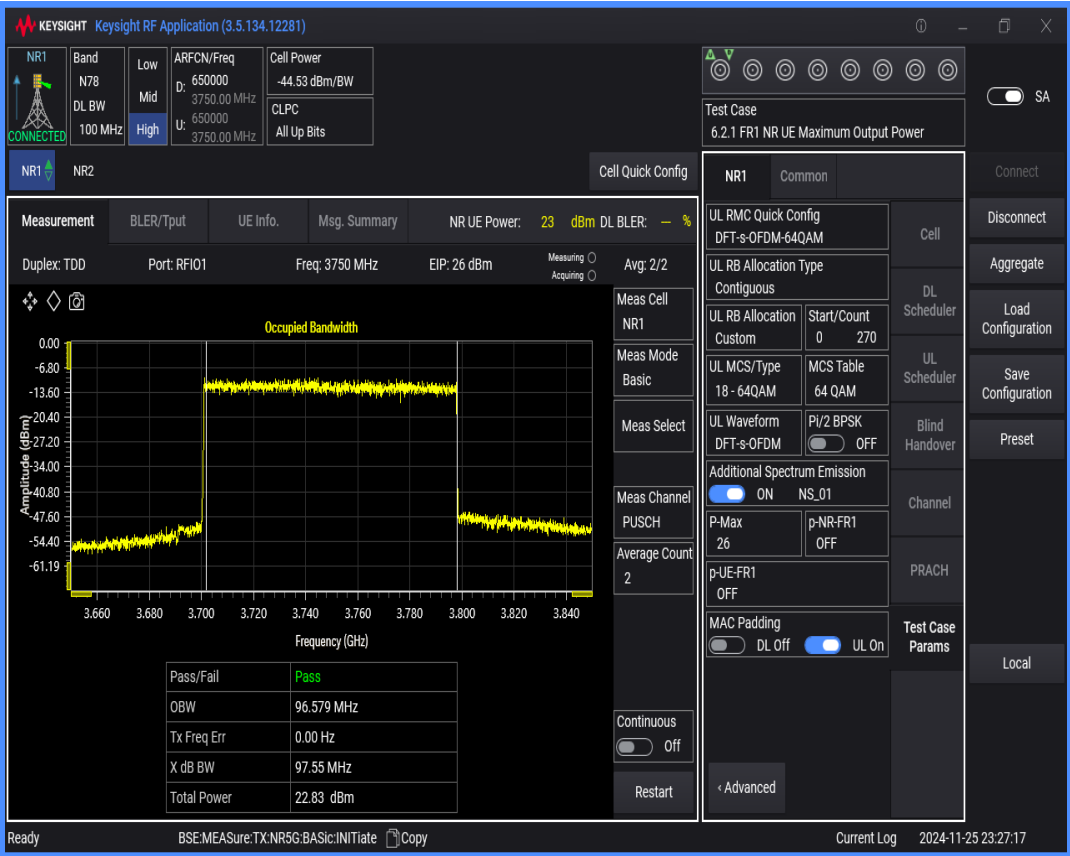
n78(3700-3800) SCS=30kHz DFT_QAM256 BW=90MHz Channel=650000 RB=240@0
