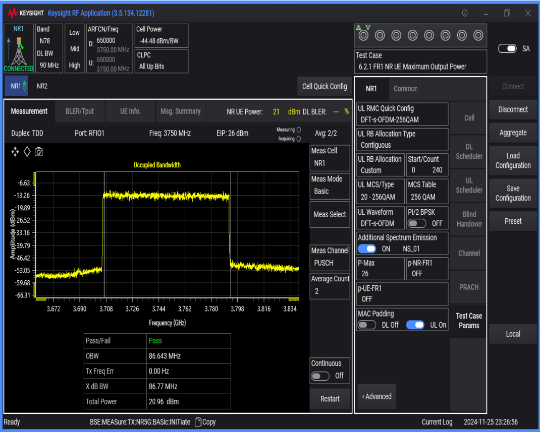
n78(3700-3800) SCS=30kHz DFT_QAM256 BW=80MHz Channel=650000 RB=216@0
