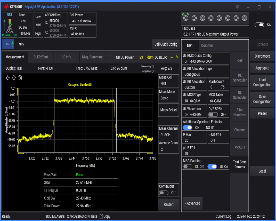
n78(3700-3800) SCS=30kHz DFT_QAM64 BW=15MHz Channel=650000 RB=36@0
