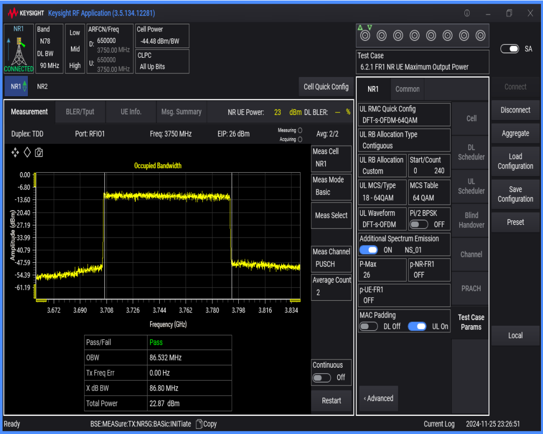
n78(3700-3800) SCS=30kHz DFT_QAM64 BW=80MHz Channel=650000 RB=216@0
