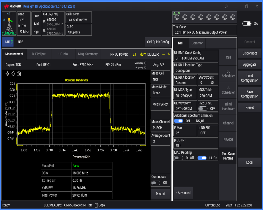
n78(3700-3800) SCS=30kHz DFT_QAM256 BW=60MHz Channel=650000 RB=162@0
