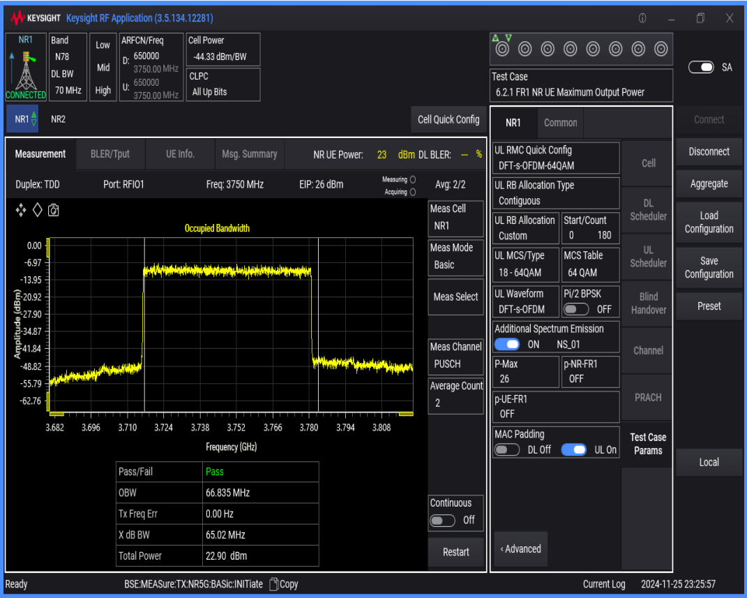
n78(3700-3800) SCS=30kHz DFT_QAM64 BW=60MHz Channel=650000 RB=162@0
