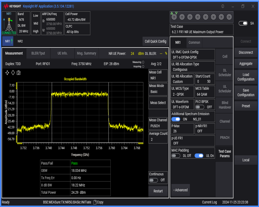
n78(3700-3800) SCS=30kHz DFT_QPSK BW=50MHz Channel=650000 RB=128@0
