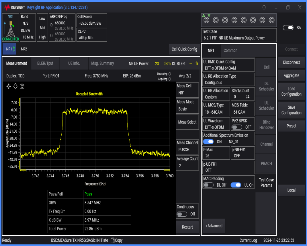
n78(3700-3800) SCS=30kHz DFT_QAM64 BW=40MHz Channel=650000 RB=100@0
