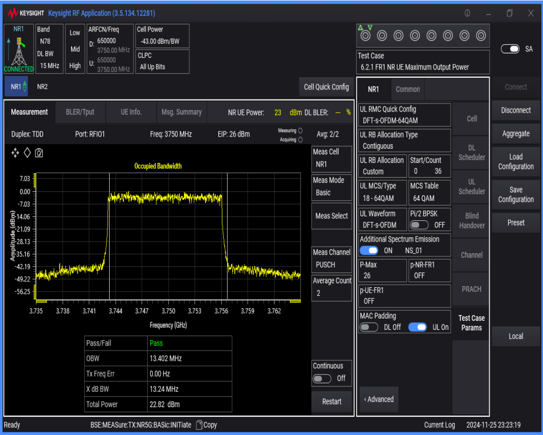
n78(3700-3800) SCS=30kHz DFT_QAM64 BW=20MHz Channel=650000 RB=50@0
