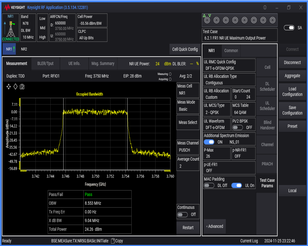
n78(3700-3800) SCS=30kHz DFT_QPSK BW=100MHz Channel=650000 RB=270@0
