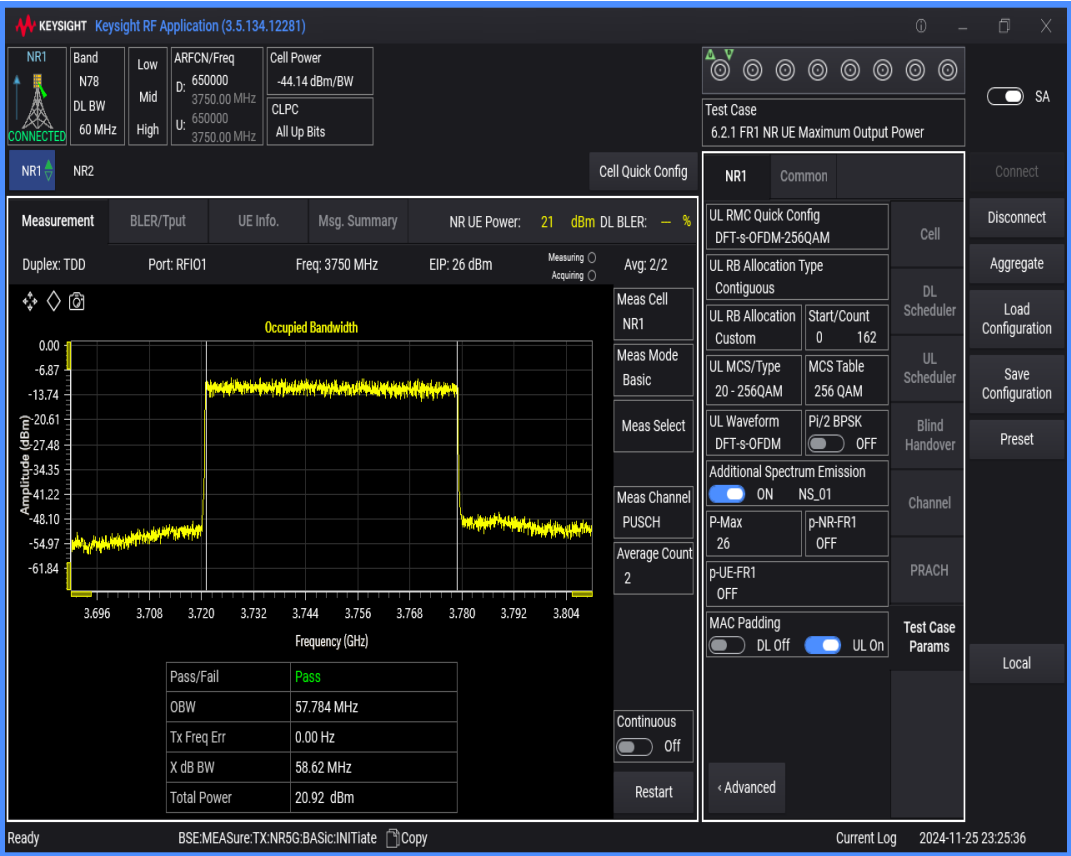
n78(3700-3800) SCS=30kHz DFT_QAM256 BW=70MHz Channel=650000 RB=180@0
