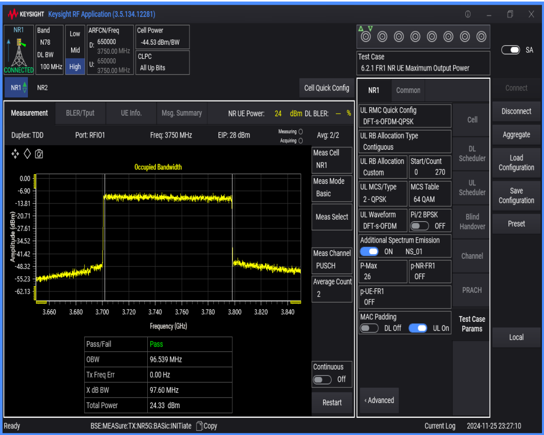
n78(3700-3800) SCS=30kHz DFT_QPSK BW=30MHz Channel=650000 RB=75@0
