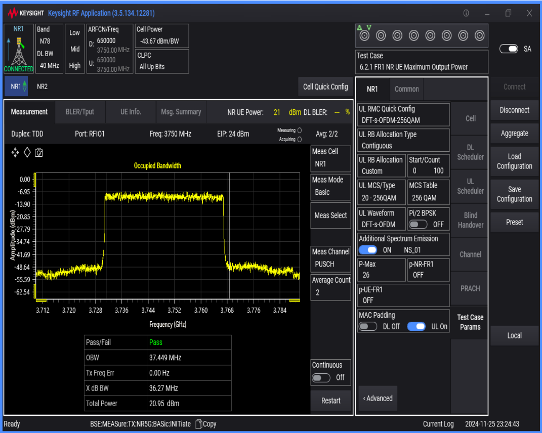
n78(3700-3800) SCS=30kHz DFT_QAM256 BW=50MHz Channel=650000 RB=128@0
