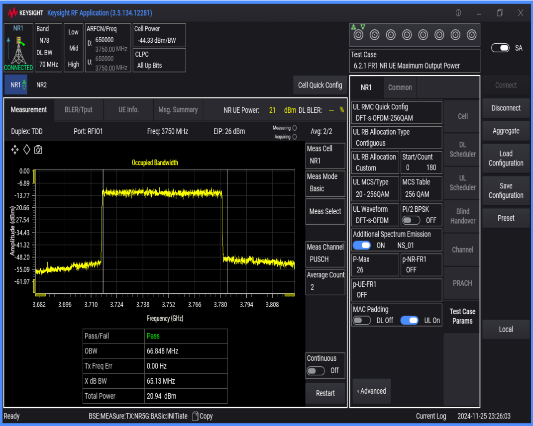
n78(3700-3800) SCS=30kHz DFT_QAM256 BW=40MHz Channel=650000 RB=100@0
