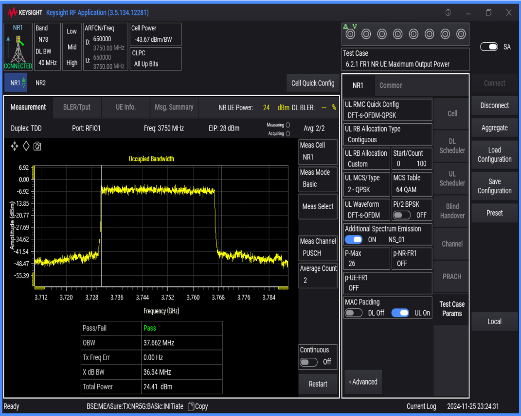
n78(3700-3800) SCS=30kHz DFT_QPSK BW=70MHz Channel=650000 RB=180@0
