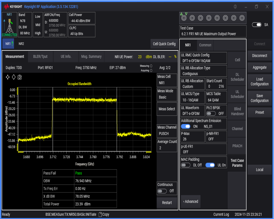
n78(3700-3800) SCS=30kHz DFT_QAM16 BW=70MHz Channel=650000 RB=180@0
