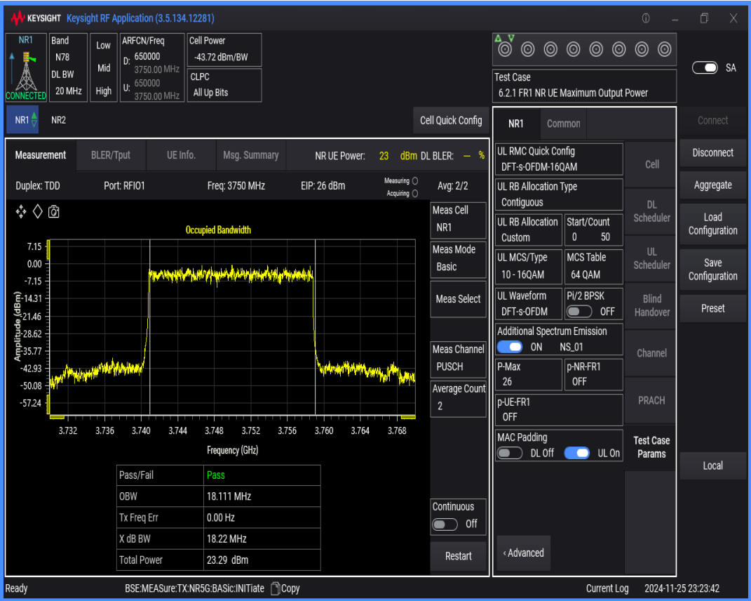
n78(3700-3800) SCS=30kHz DFT_QAM16 BW=15MHz Channel=650000 RB=36@0
