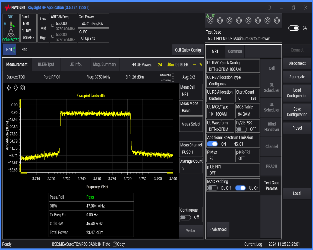
n78(3700-3800) SCS=30kHz DFT_QAM16 BW=80MHz Channel=650000 RB=216@0
