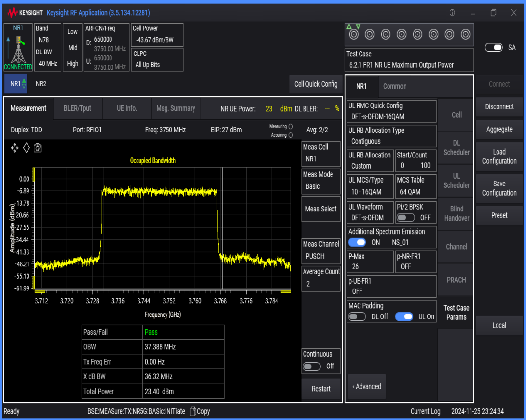
n78(3700-3800) SCS=30kHz DFT_QAM16 BW=30MHz Channel=650000 RB=75@0
