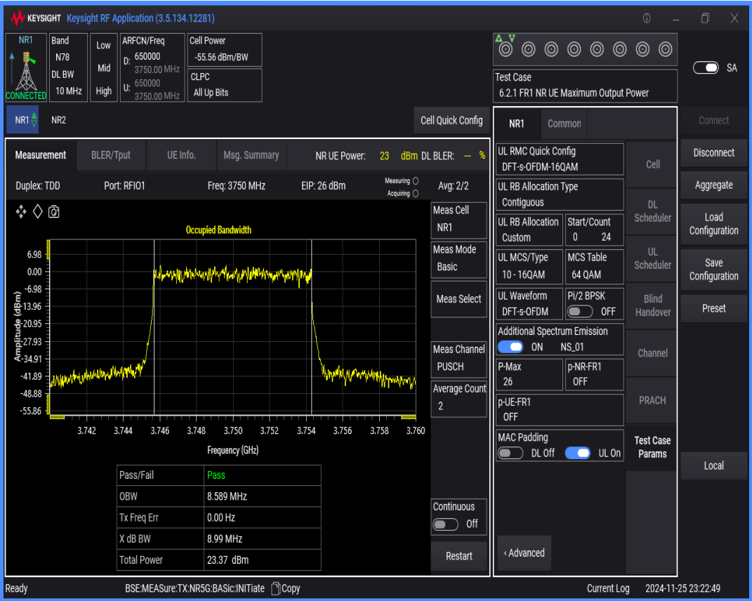
n78(3700-3800) SCS=30kHz DFT_QAM16 BW=100MHz Channel=650000 RB=270@0
