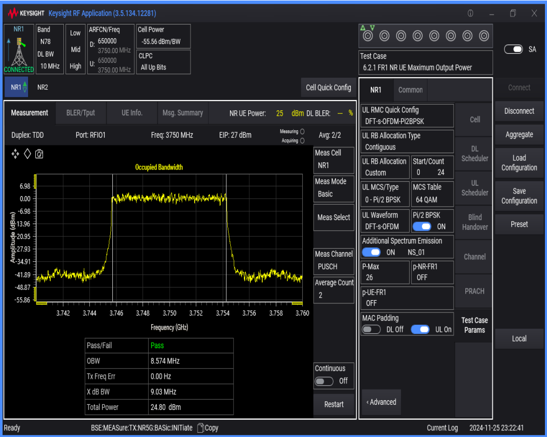
n78(3700-3800) SCS=30kHz DFT_BPSK BW=30MHz Channel=650000 RB=75@0
