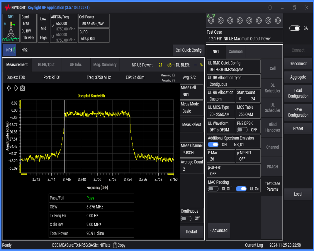
n78(3700-3800) SCS=30kHz DFT_QAM256 BW=30MHz Channel=650000 RB=75@0
