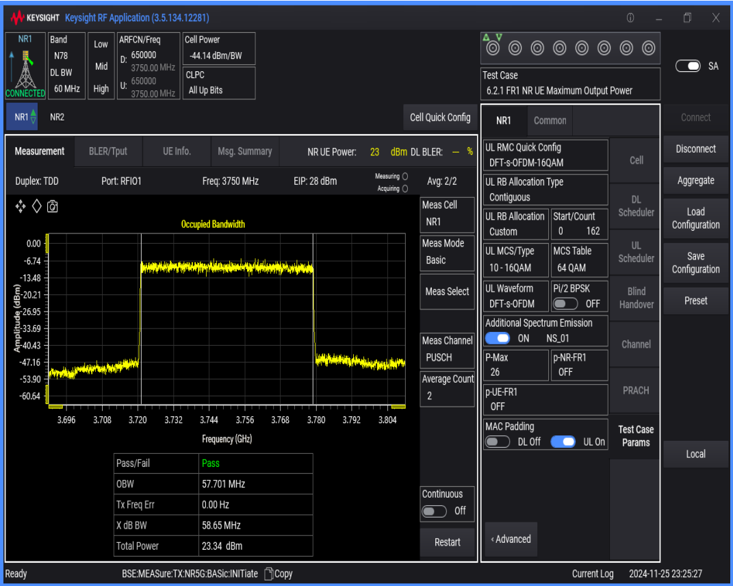
n78(3700-3800) SCS=30kHz DFT_QAM16 BW=50MHz Channel=650000 RB=128@0
