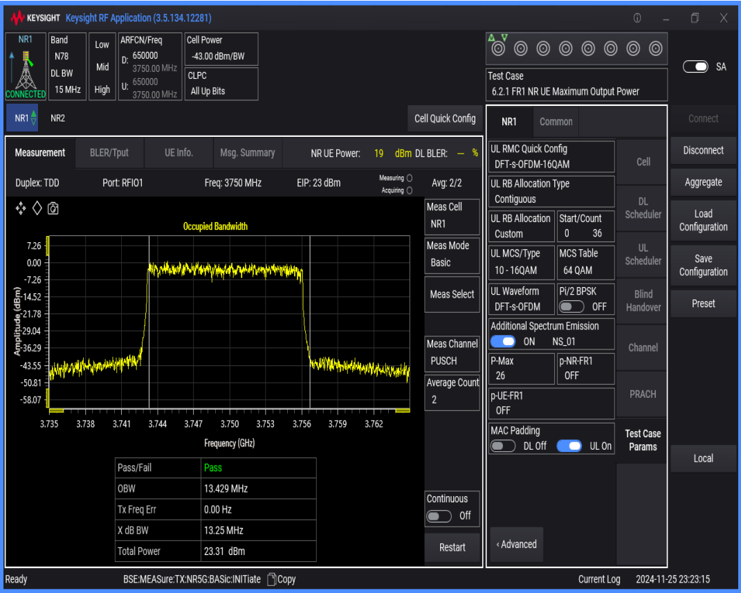
n78(3700-3800) SCS=30kHz DFT_QAM16 BW=40MHz Channel=650000 RB=100@0
