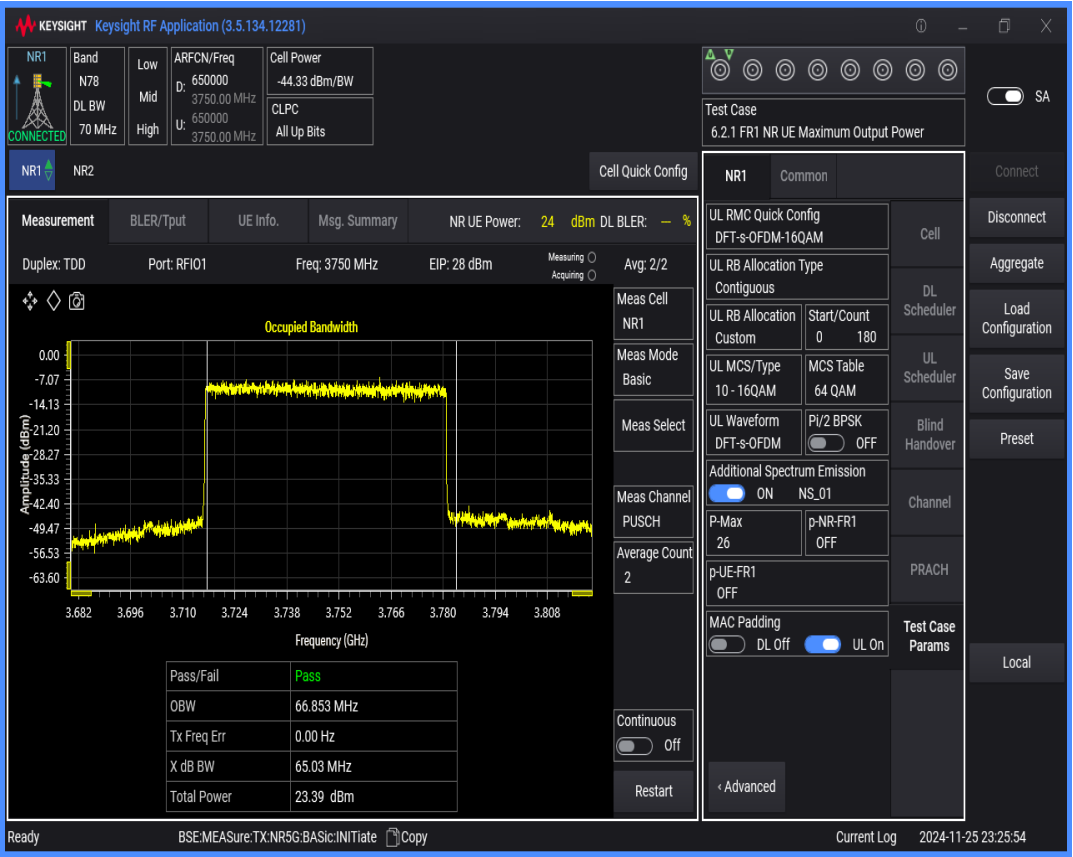
n78(3700-3800) SCS=30kHz DFT_QAM256 BW=100MHz Channel=650000 RB=270@0
