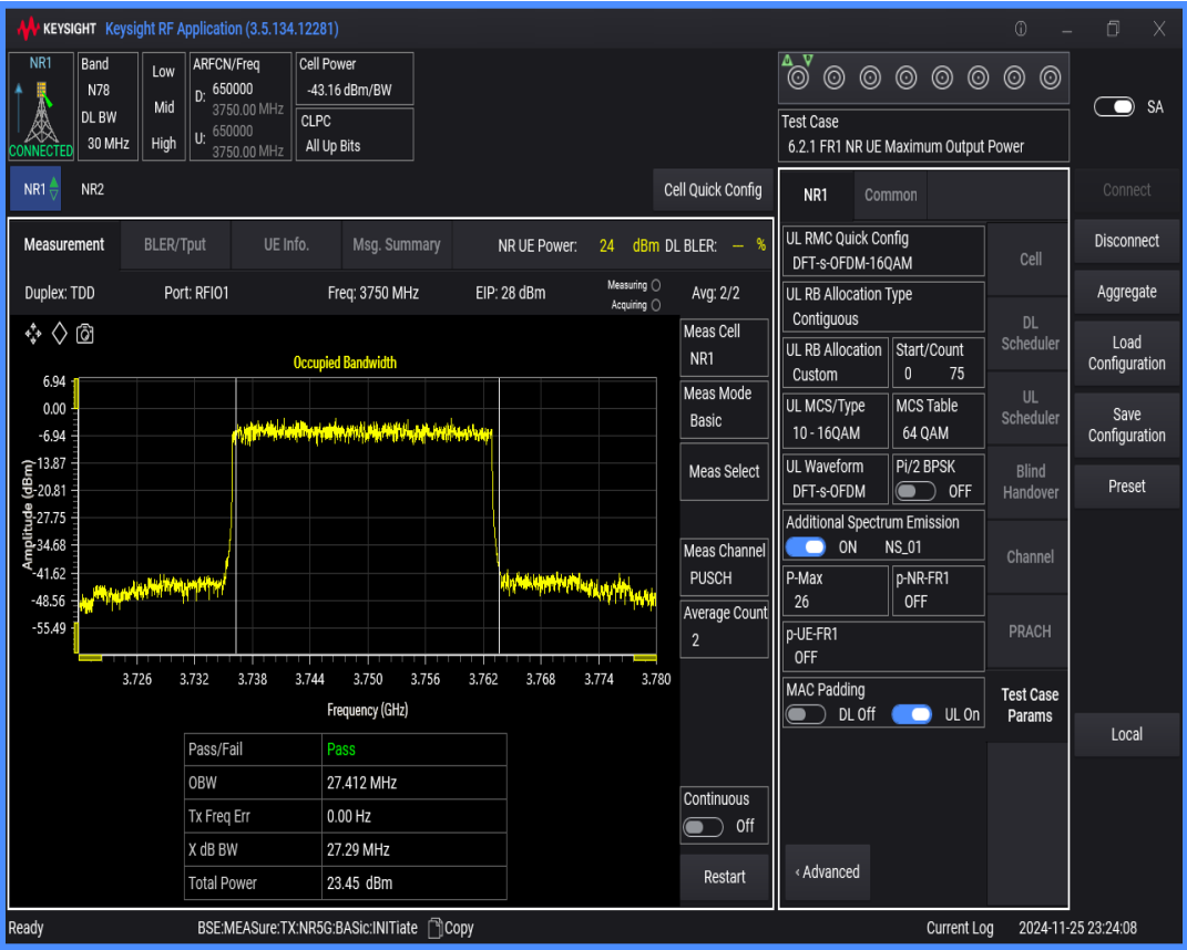
n78(3700-3800) SCS=30kHz DFT_QAM16 BW=60MHz Channel=650000 RB=162@0
