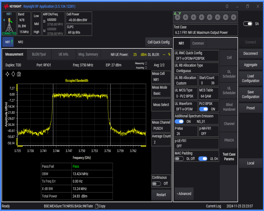
n78(3700-3800) SCS=30kHz DFT_BPSK BW=50MHz Channel=650000 RB=128@0
