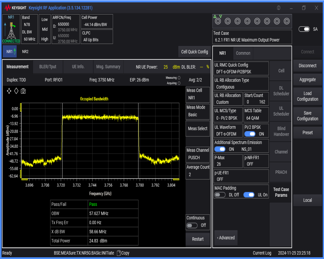
n78(3700-3800) SCS=30kHz DFT_BPSK BW=90MHz Channel=650000 RB=240@0
