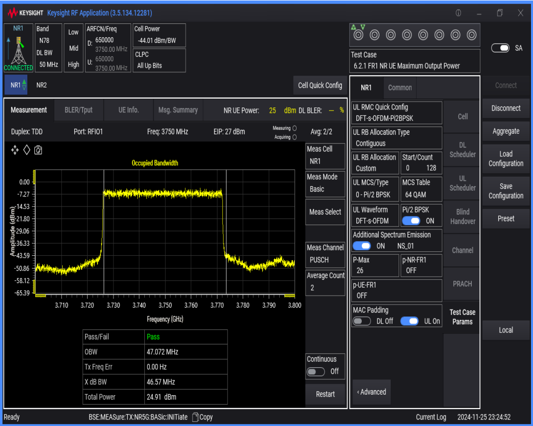
n78(3700-3800) SCS=30kHz DFT_BPSK BW=40MHz Channel=650000 RB=100@0
