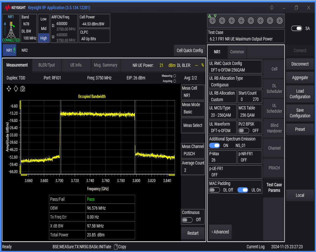
n78(3700-3800) SCS=30kHz DFT_QAM16 BW=90MHz Channel=650000 RB=240@0
