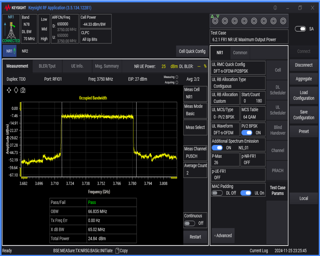
n78(3700-3800) SCS=30kHz DFT_BPSK BW=60MHz Channel=650000 RB=162@0
