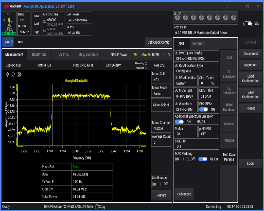
n78(3700-3800) SCS=30kHz DFT_BPSK BW=15MHz Channel=650000 RB=36@0
