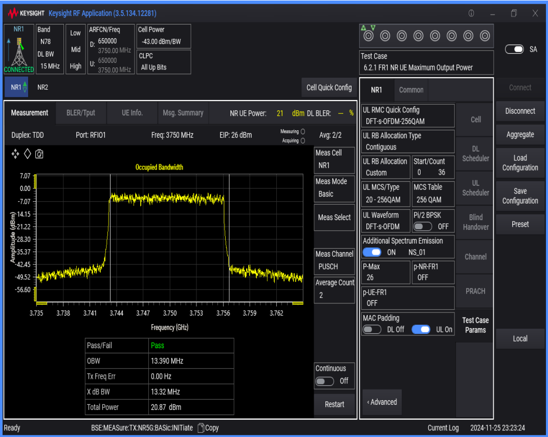
n78(3700-3800) SCS=30kHz DFT_QAM256 BW=10MHz Channel=650000 RB=24@0
