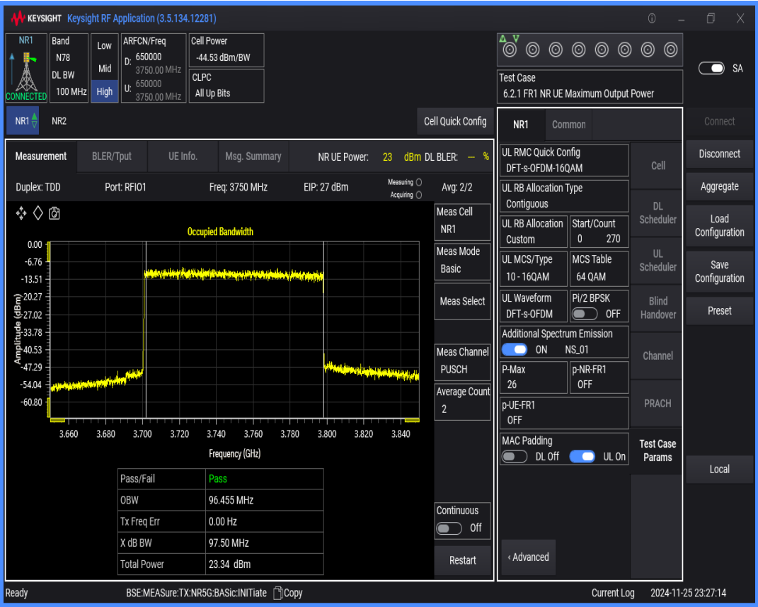
n78(3700-3800) SCS=30kHz DFT_QAM16 BW=20MHz Channel=650000 RB=50@0
