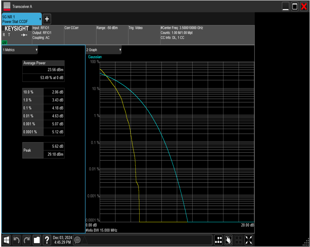
n78(3450-3550) SCS=30kHz DFT_BPSK BW=10MHz Channel=633334 RB=24@0
