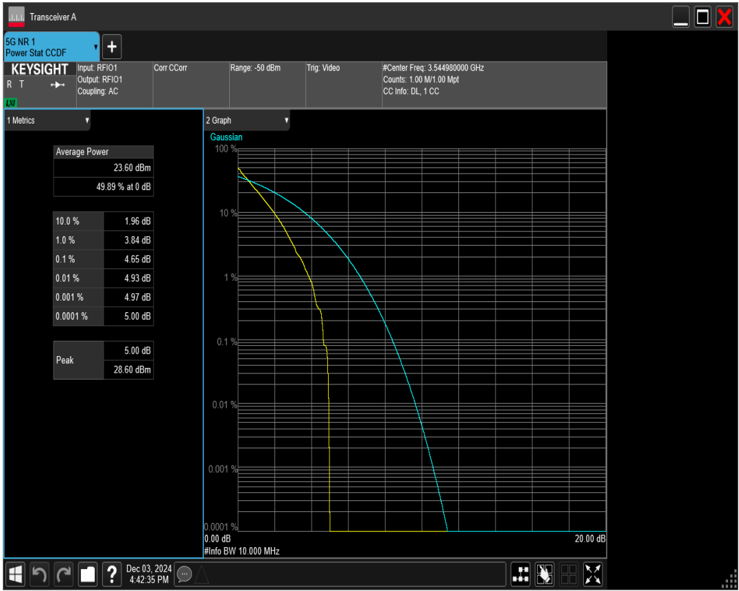
n78(3450-3550) SCS=30kHz DFT_BPSK BW=30MHz Channel=631000 RB=75@0
