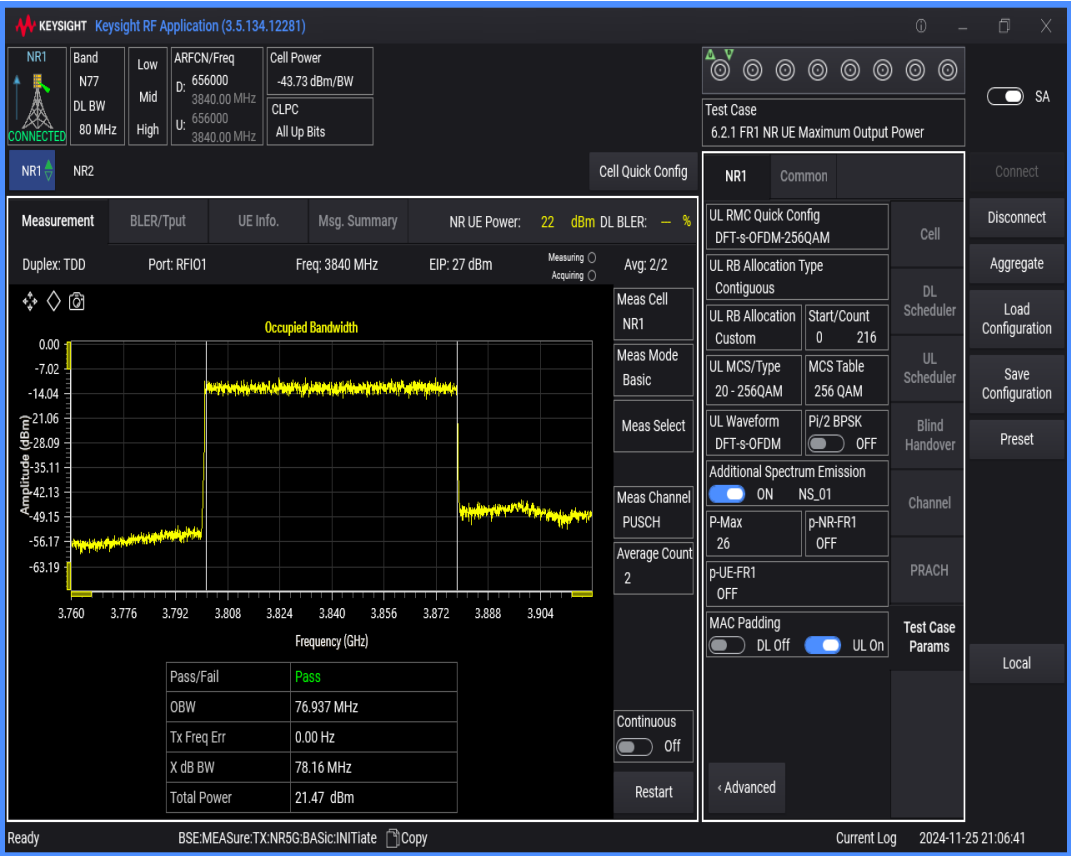
n77(3700-3980) SCS=30kHz DFT_QAM256 BW=60MHz Channel=656000 RB=162@0
