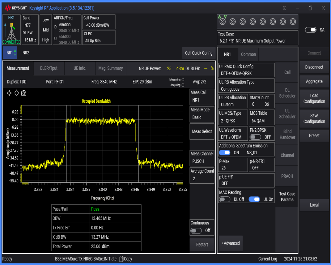
n77(3700-3980) SCS=30kHz DFT_QPSK BW=60MHz Channel=656000 RB=162@0
