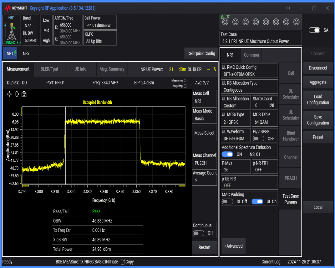
n77(3700-3980) SCS=30kHz DFT_QPSK BW=40MHz Channel=656000 RB=100@0
