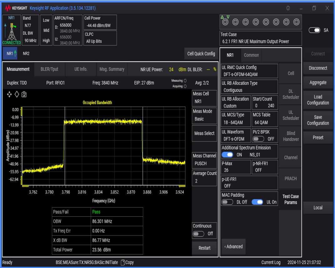
n77(3700-3980) SCS=30kHz DFT_QPSK BW=30MHz Channel=656000 RB=75@0
