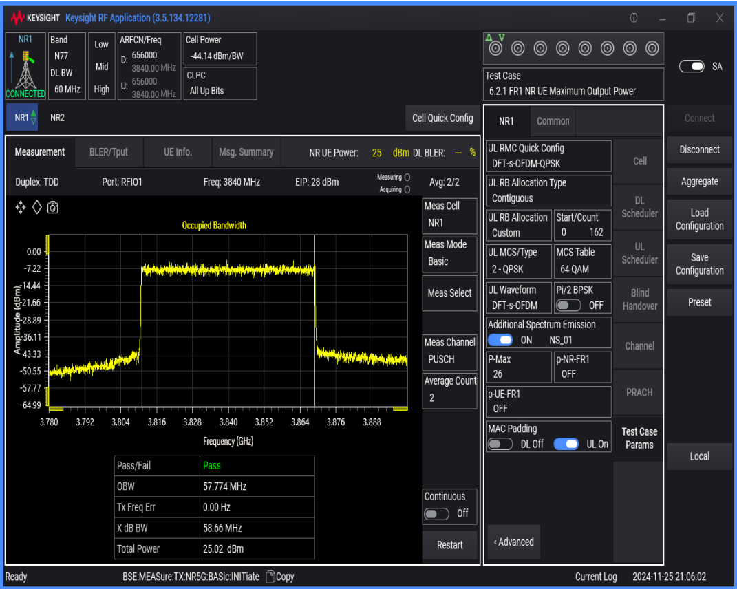
n77(3700-3980) SCS=30kHz DFT_QPSK BW=50MHz Channel=656000 RB=128@0
