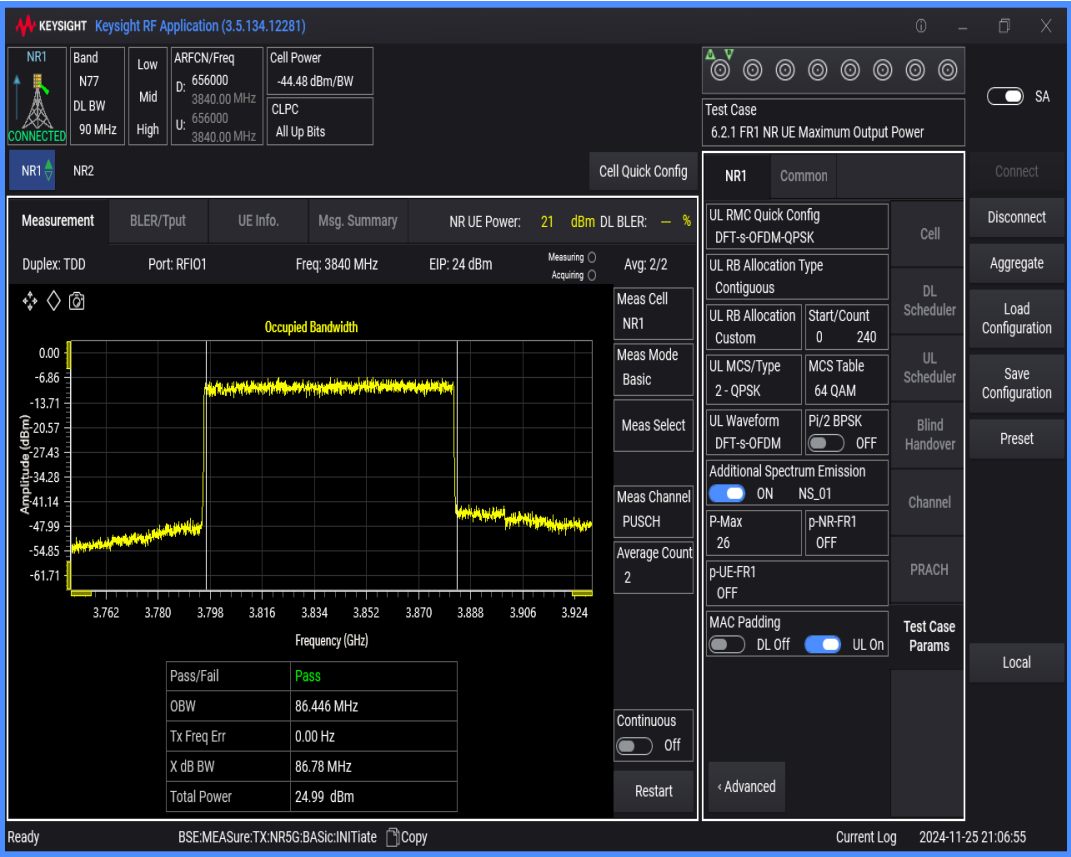
n77(3700-3980) SCS=30kHz DFT_QPSK BW=80MHz Channel=656000 RB=216@0
