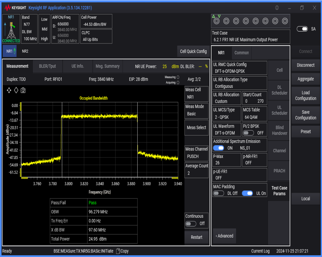
n77(3700-3980) SCS=30kHz DFT_QAM64 BW=90MHz Channel=656000 RB=240@0
