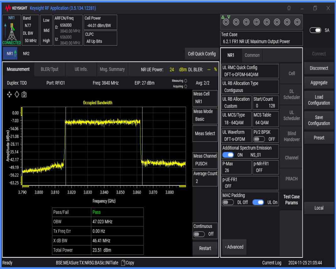
n77(3700-3980) SCS=30kHz DFT_QAM64 BW=30MHz Channel=656000 RB=75@0
