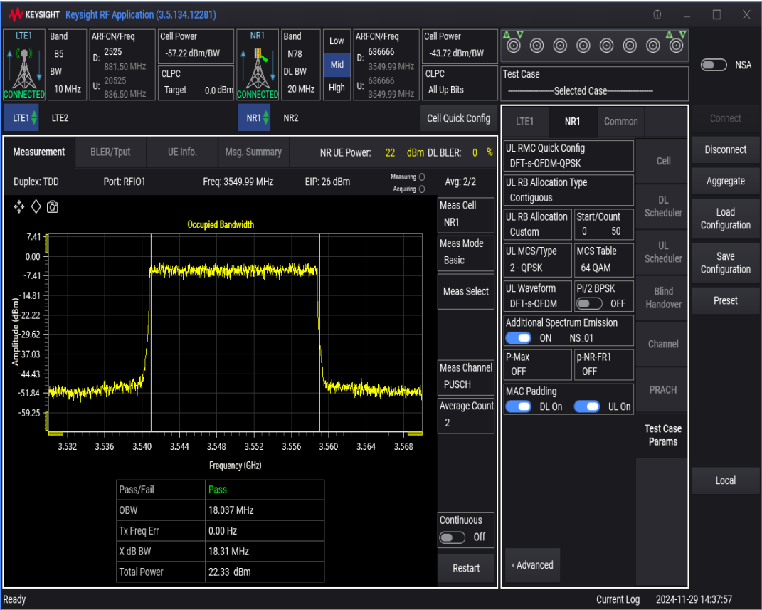
n78 SCS=30kHz DFT_QPSK BW=60MHz Channel=636666 RB=162@0
