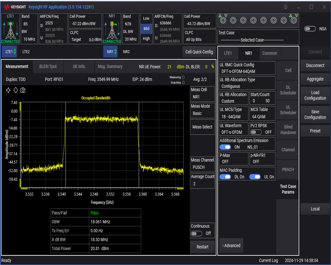
n78 SCS=30kHz DFT_QPSK BW=40MHz Channel=636666 RB=100@0
