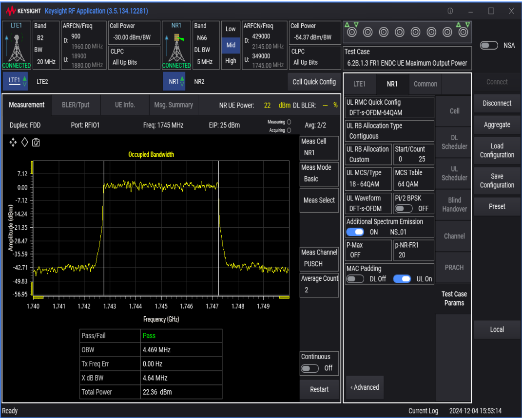
n66 SCS=15kHz DFT_QAM64 BW=40MHz Channel=349000 RB=216@0
