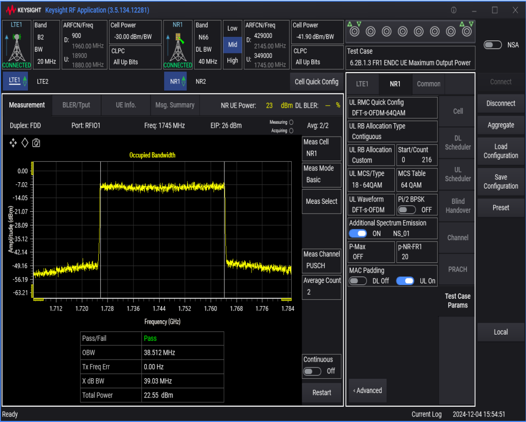
n66 SCS=15kHz DFT_QAM64 BW=20MHz Channel=349000 RB=100@0
