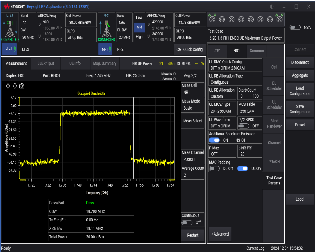
n66 SCS=15kHz DFT_QAM16 BW=5MHz Channel=349000 RB=25@0
