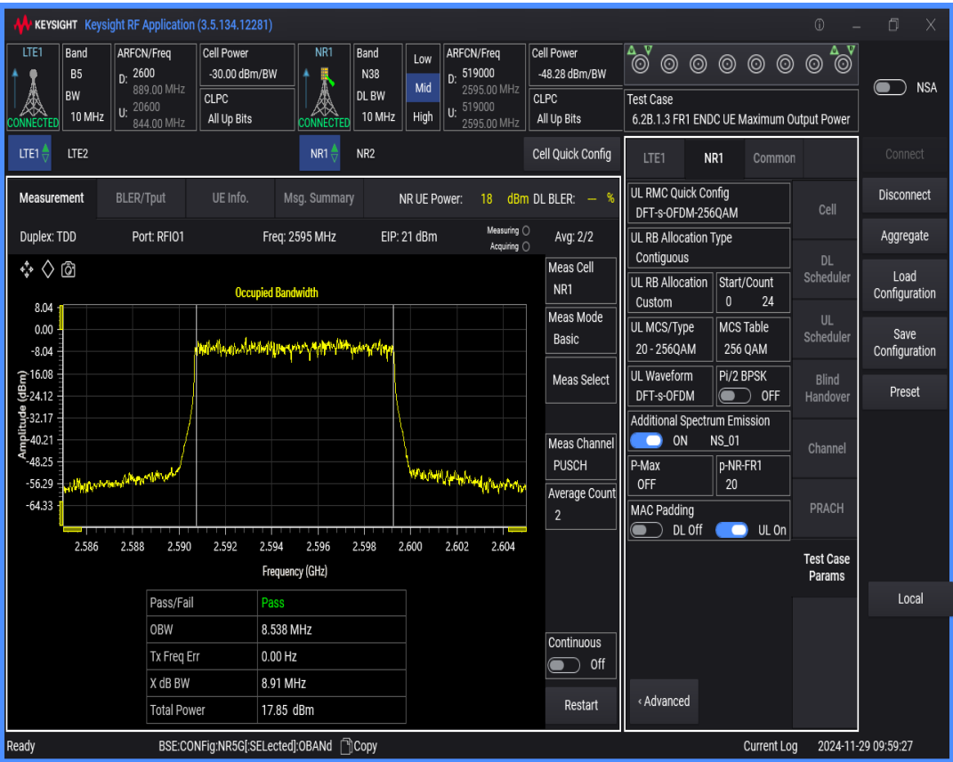
n38 SCS=30kHz DFT_QAM64 BW=10MHz Channel=519000 RB=24@0
