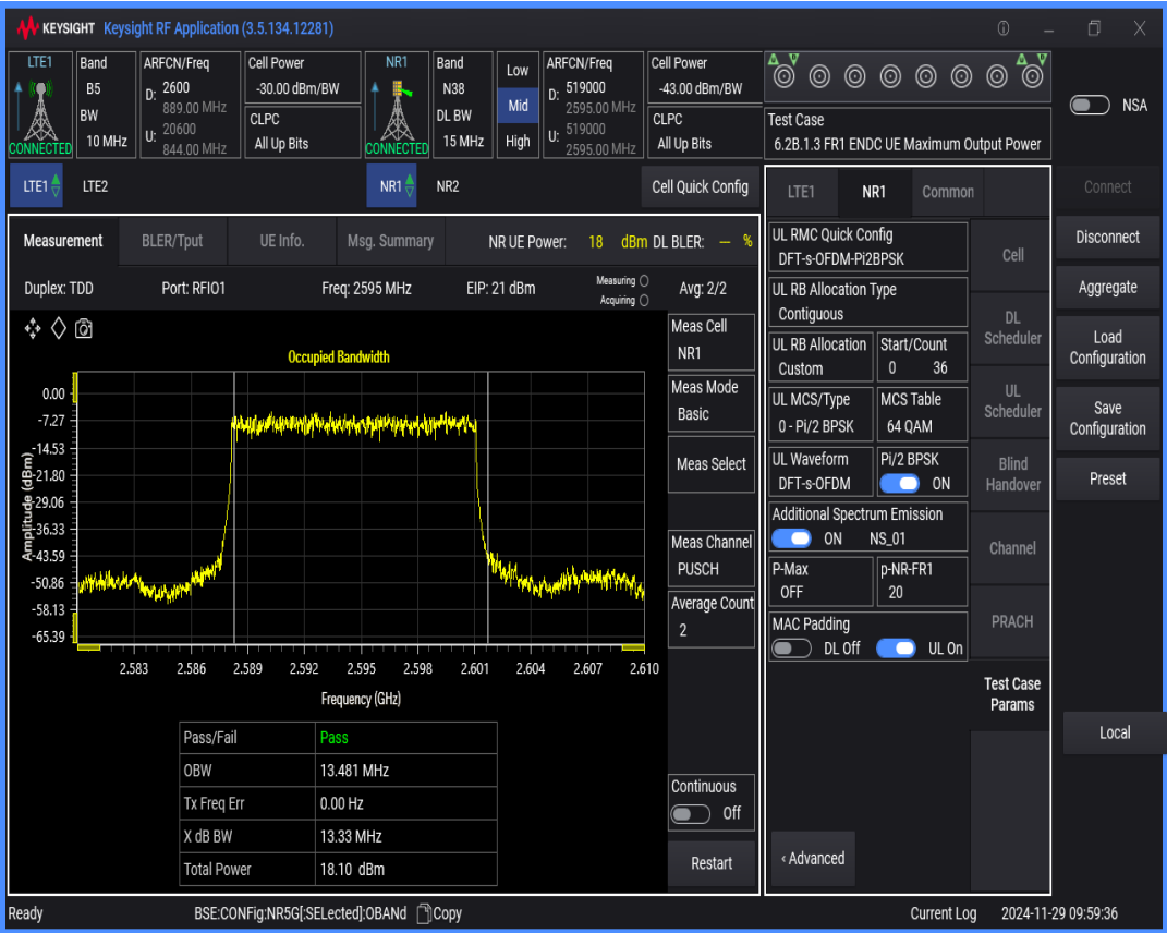
n38 SCS=30kHz DFT_QAM16 BW=15MHz Channel=519000 RB=36@0
