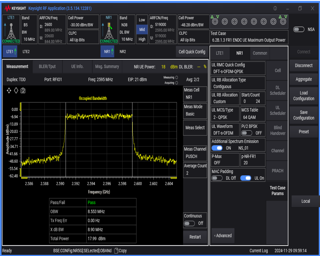
n38 SCS=30kHz DFT_QAM64 BW=15MHz Channel=519000 RB=36@0
