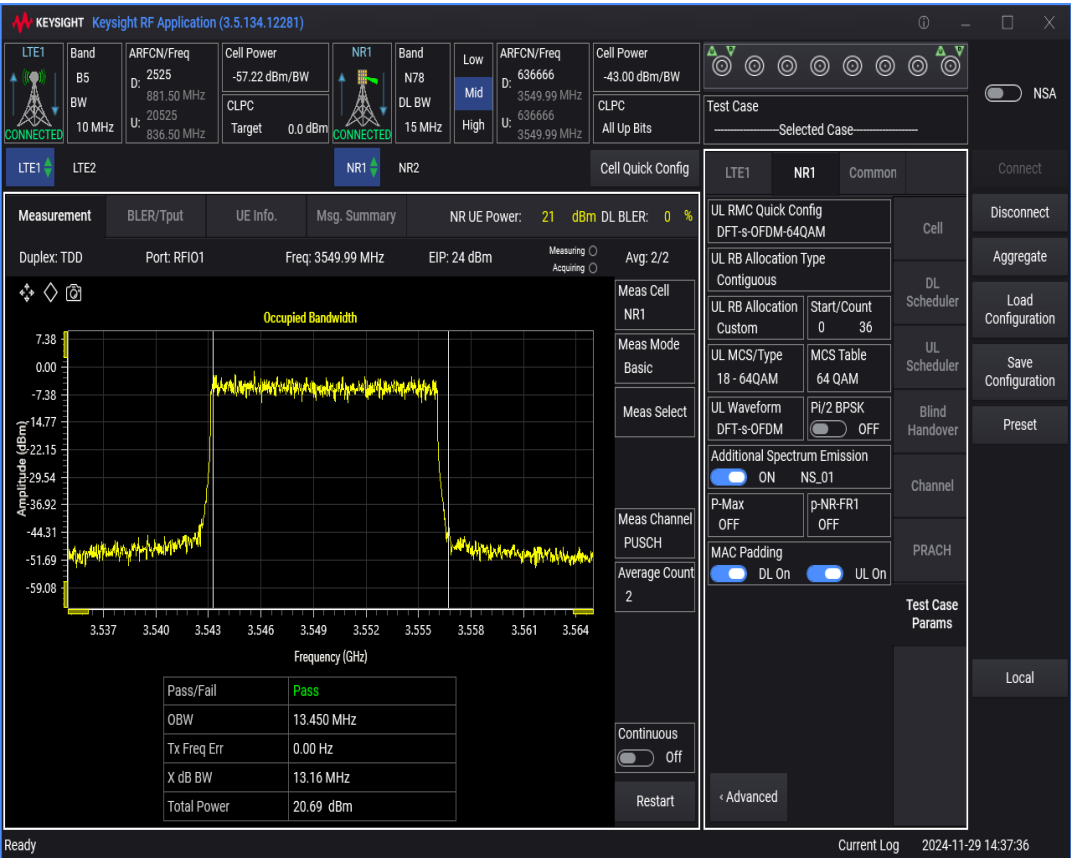
n78 SCS=30kHz DFT_QAM64 BW=10MHz Channel=636666 RB=24@0
