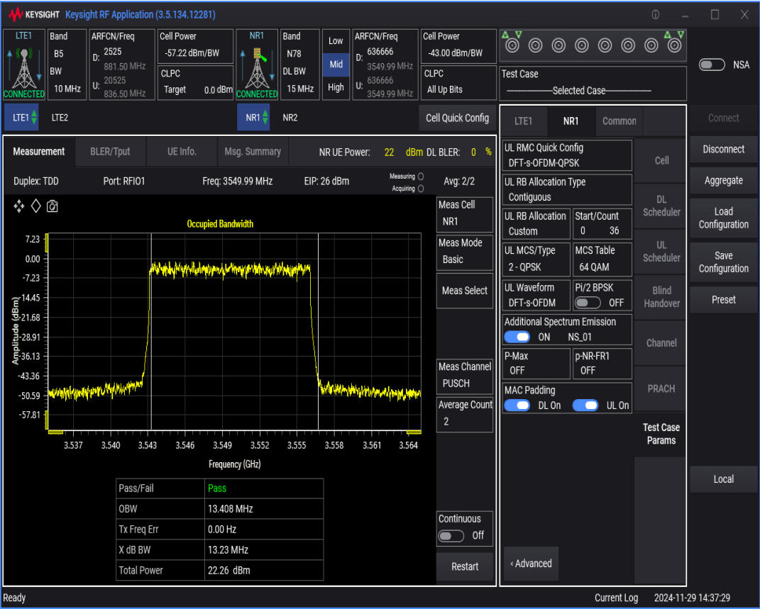
n78 SCS=30kHz DFT_QPSK BW=10MHz Channel=636666 RB=24@0
