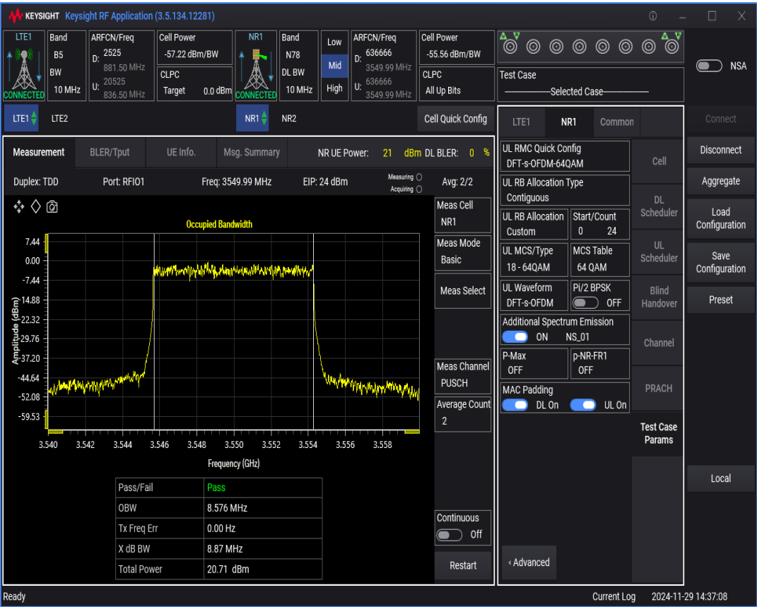
n78 SCS=30kHz DFT_QAM64 BW=40MHz Channel=636666 RB=100@0
