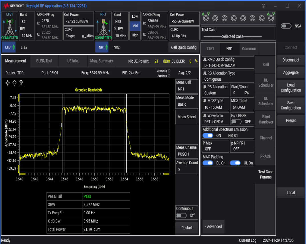
n78 SCS=30kHz DFT_QAM16 BW=100MHz Channel=636666 RB=270@0
