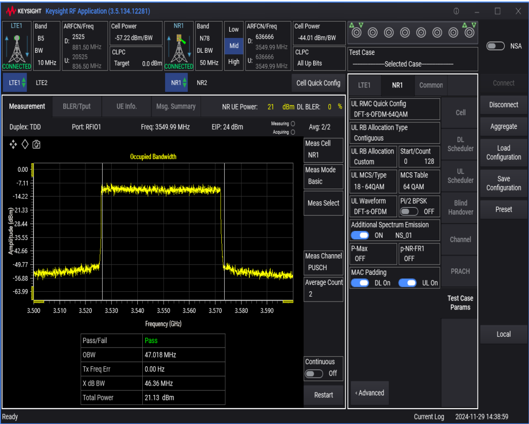
n78 SCS=30kHz DFT_QAM64 BW=15MHz Channel=636666 RB=36@0
