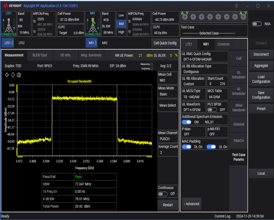
n78 SCS=30kHz DFT_QAM64 BW=60MHz Channel=636666 RB=162@0
