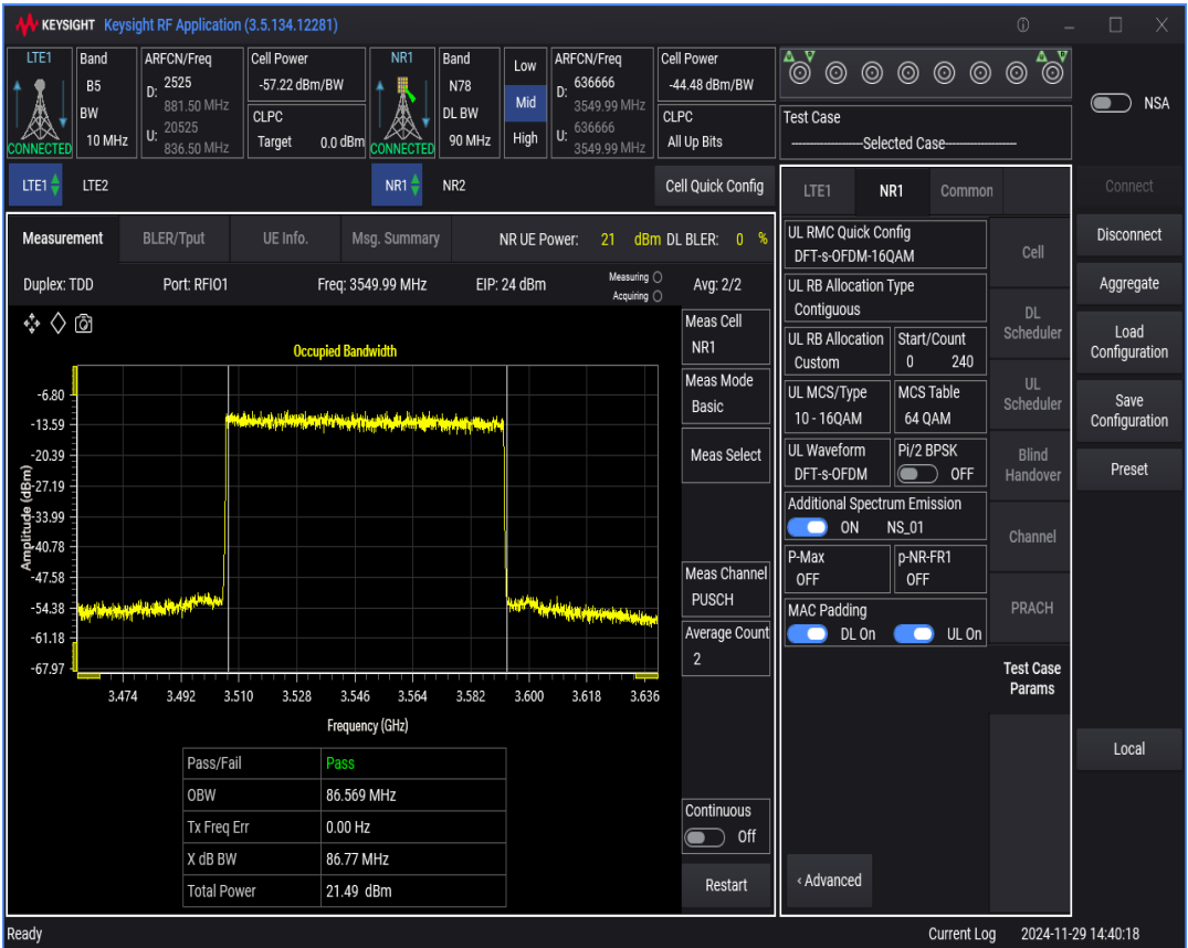
n78 SCS=30kHz DFT_QAM256 BW=10MHz Channel=636666 RB=24@0
