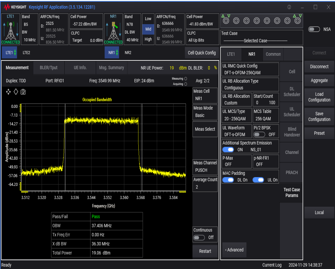
n78 SCS=30kHz DFT_QAM64 BW=80MHz Channel=636666 RB=216@0
