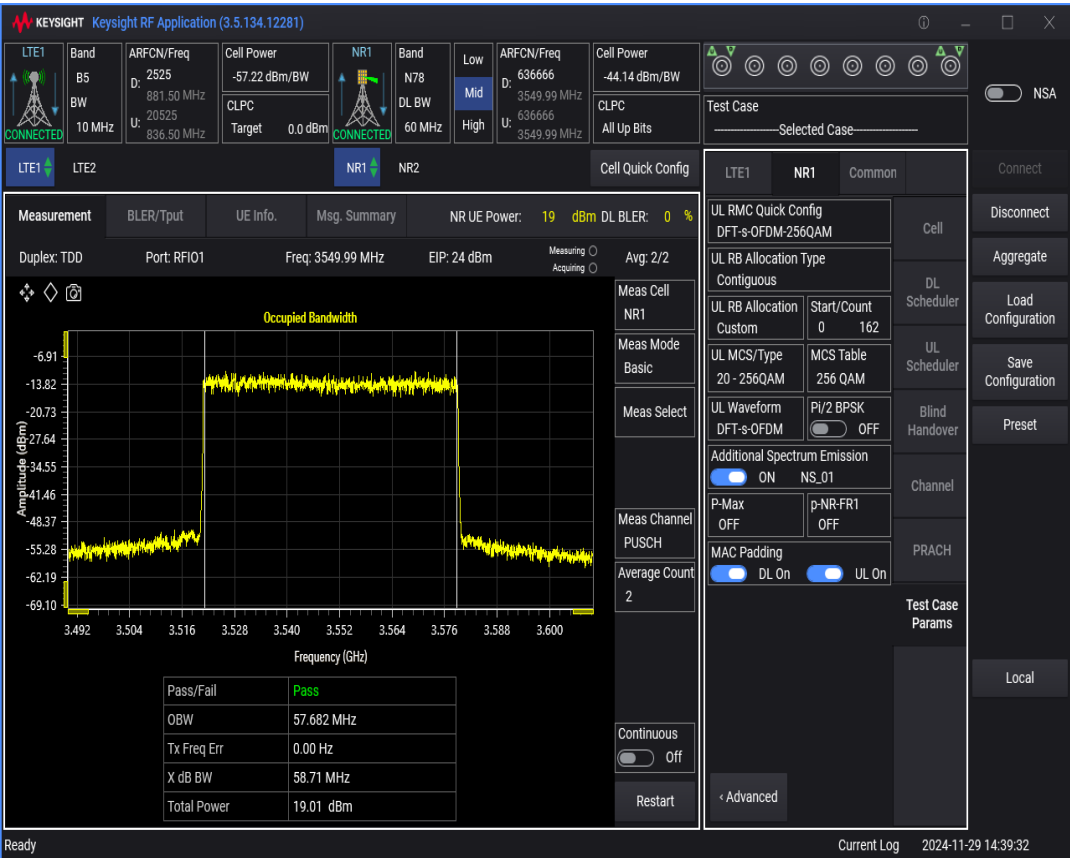
n78 SCS=30kHz DFT_QAM64 BW=100MHz Channel=636666 RB=270@0
