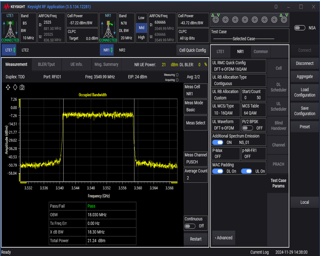
n78 SCS=30kHz DFT_QAM256 BW=80MHz Channel=636666 RB=216@0
