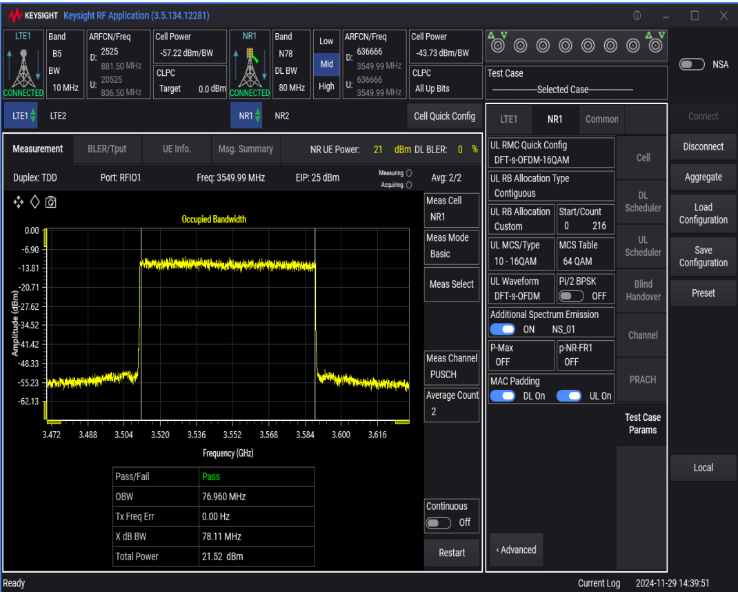
n78 SCS=30kHz DFT_QAM16 BW=60MHz Channel=636666 RB=162@0
