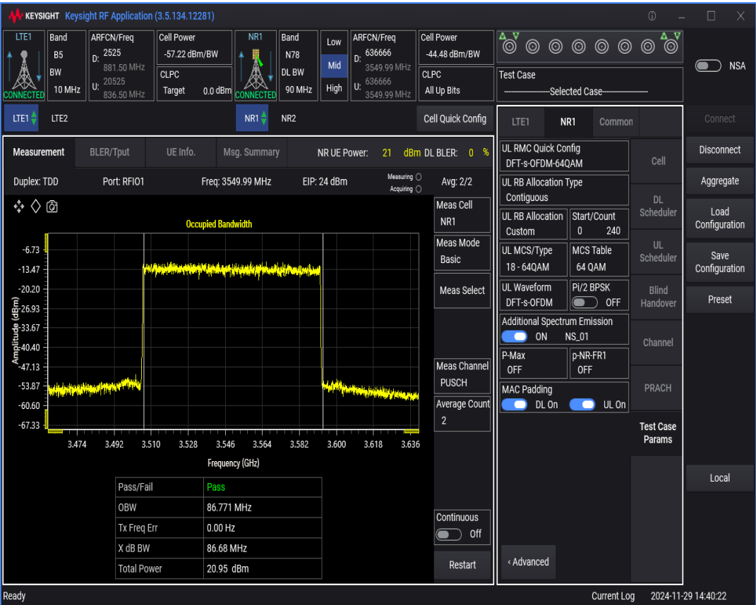
n78 SCS=30kHz DFT_QAM64 BW=50MHz Channel=636666 RB=128@0
