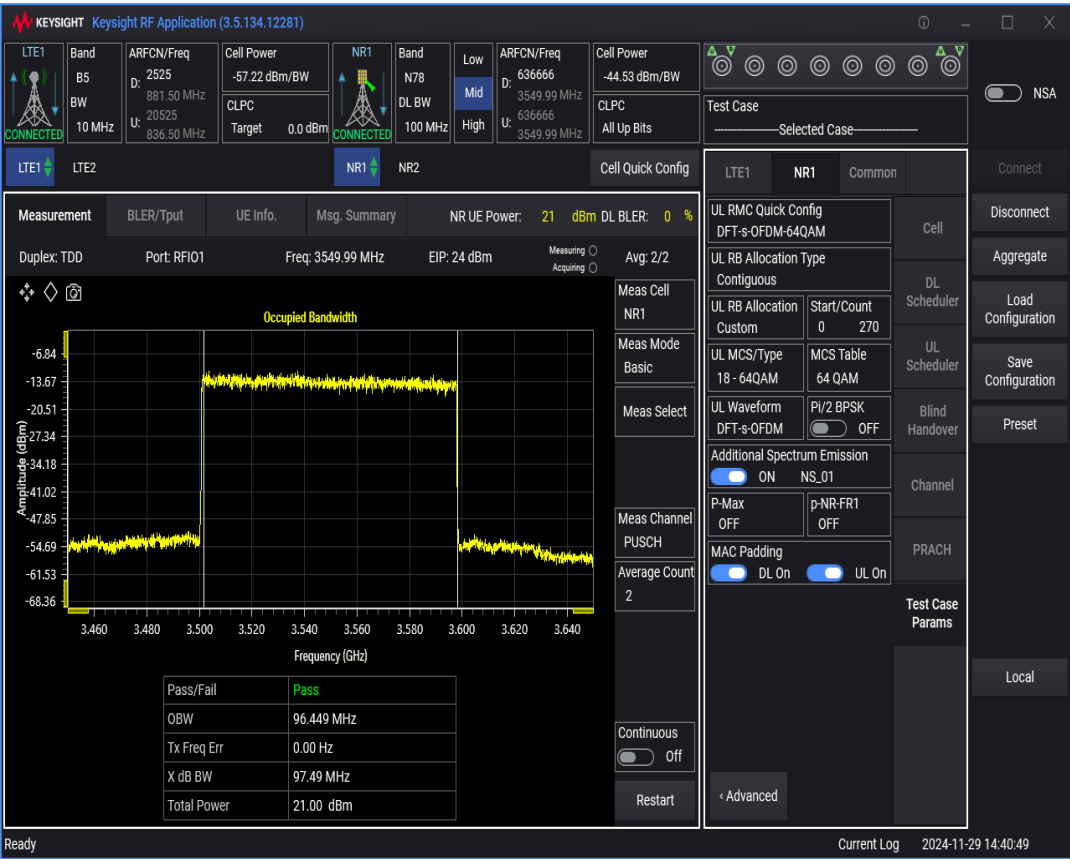
n78 SCS=30kHz DFT_QAM256 BW=90MHz Channel=636666 RB=240@0
