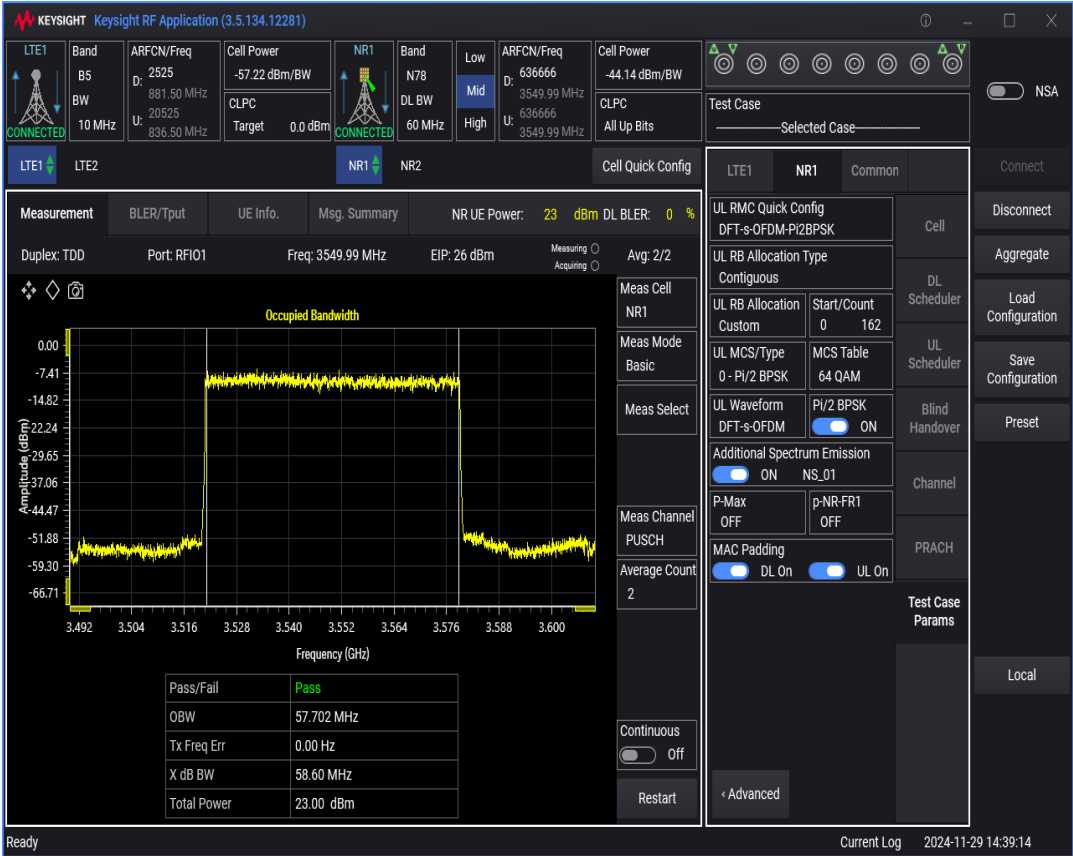
n78 SCS=30kHz DFT_BPSK BW=50MHz Channel=636666 RB=128@0
