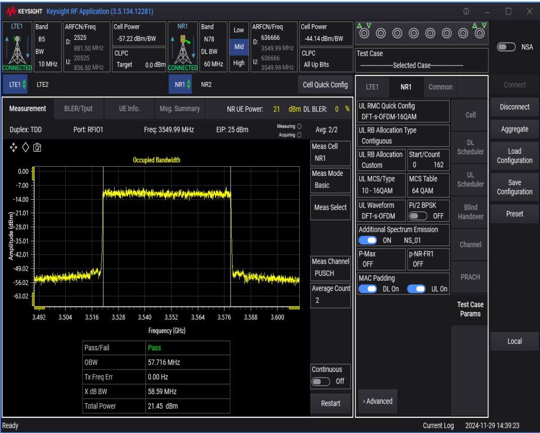
n78 SCS=30kHz DFT_QAM16 BW=90MHz Channel=636666 RB=240@0
