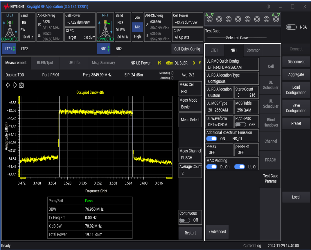
n78 SCS=30kHz DFT_QAM256 BW=60MHz Channel=636666 RB=162@0
