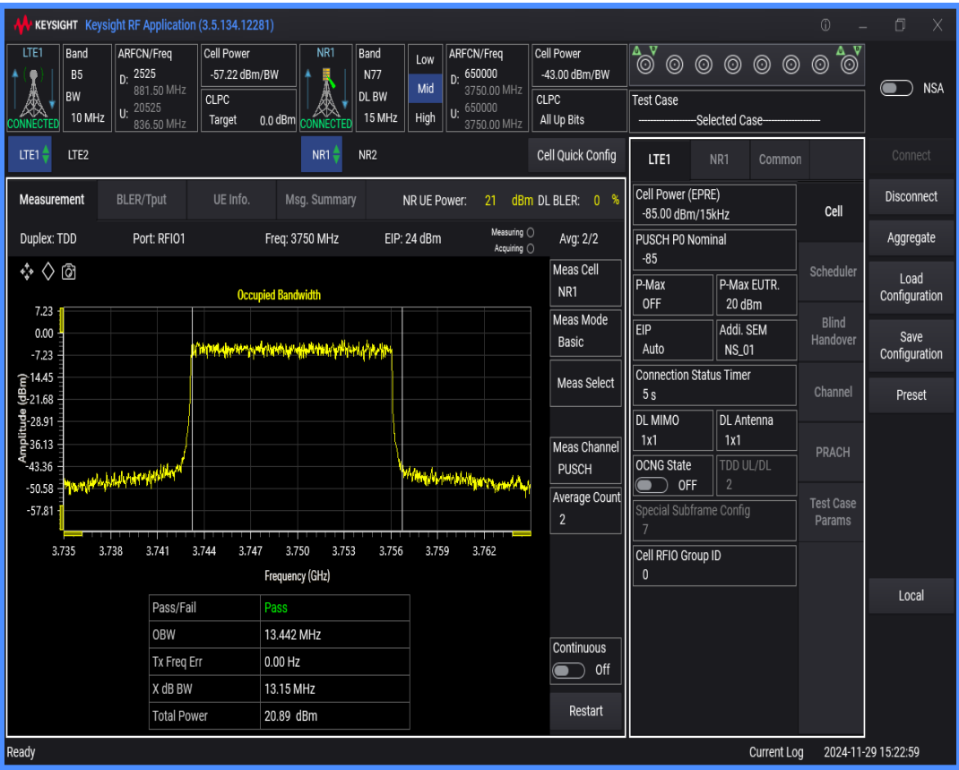
n77 SCS=30kHz DFT_QAM16 BW=20MHz Channel=650000 RB=50@0
