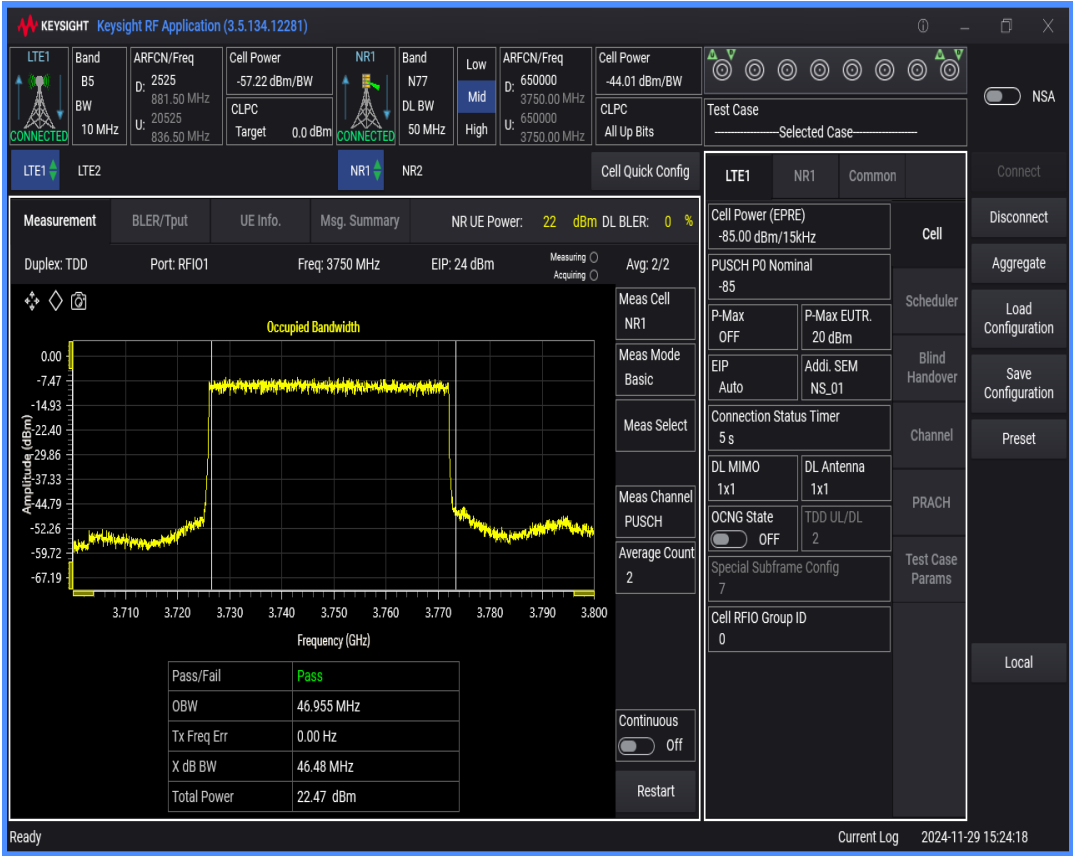
n77 SCS=30kHz DFT_BPSK BW=40MHz Channel=650000 RB=100@0
