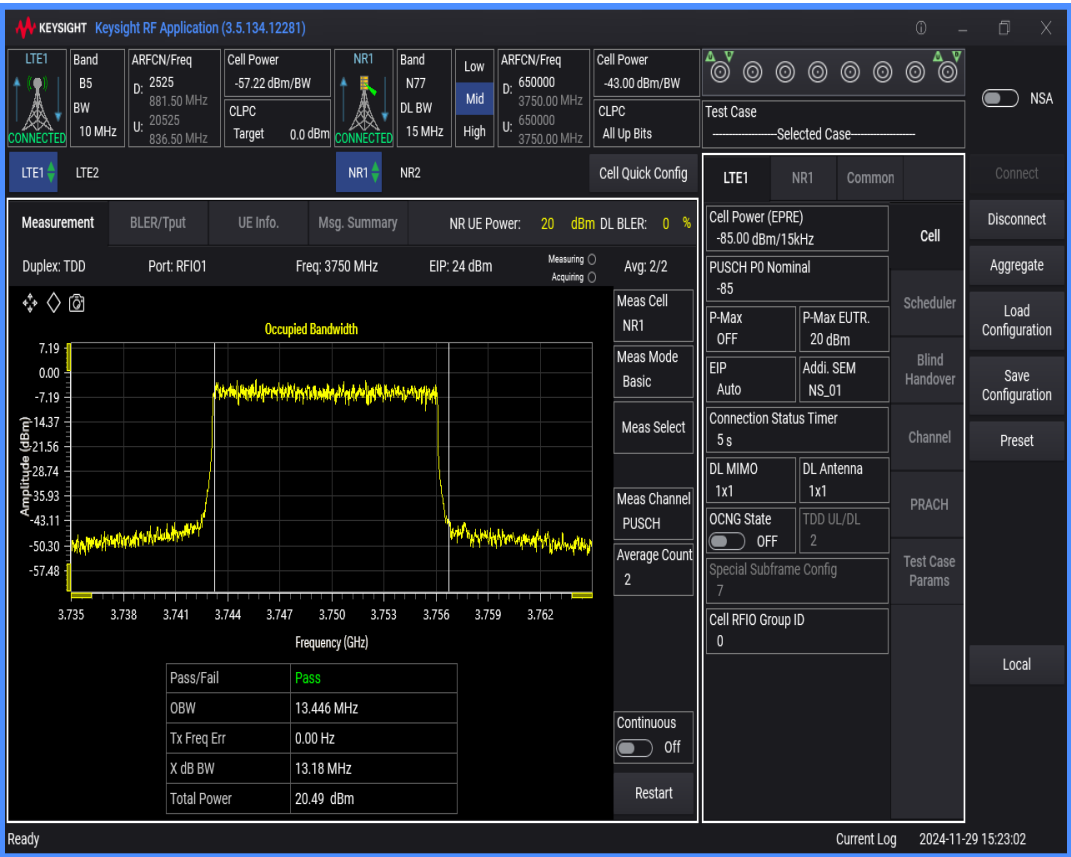
n77 SCS=30kHz DFT_QPSK BW=15MHz Channel=650000 RB=36@0
