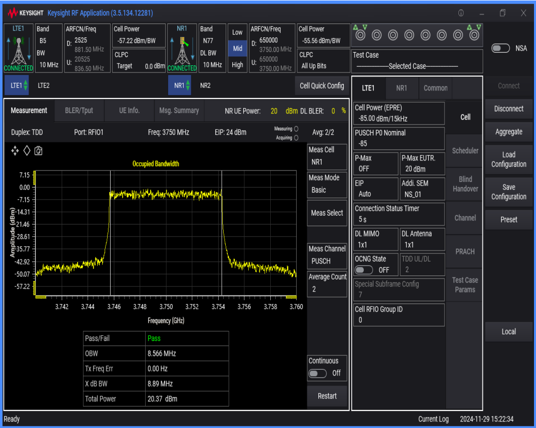
n77 SCS=30kHz DFT_QAM64 BW=15MHz Channel=650000 RB=36@0
