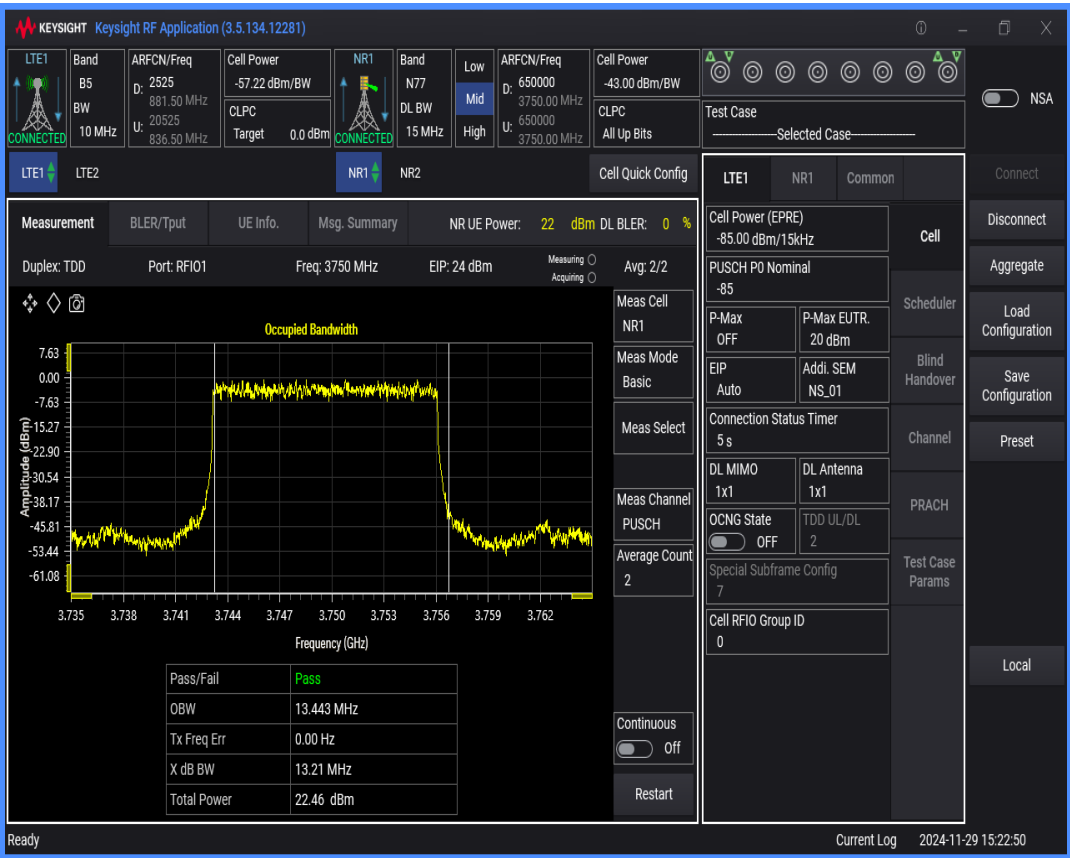
n77 SCS=30kHz DFT_QAM16 BW=15MHz Channel=650000 RB=36@0
