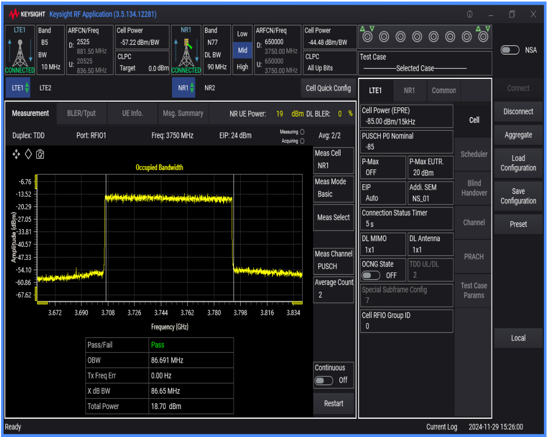
n77 SCS=30kHz DFT_QAM256 BW=50MHz Channel=650000 RB=128@0
