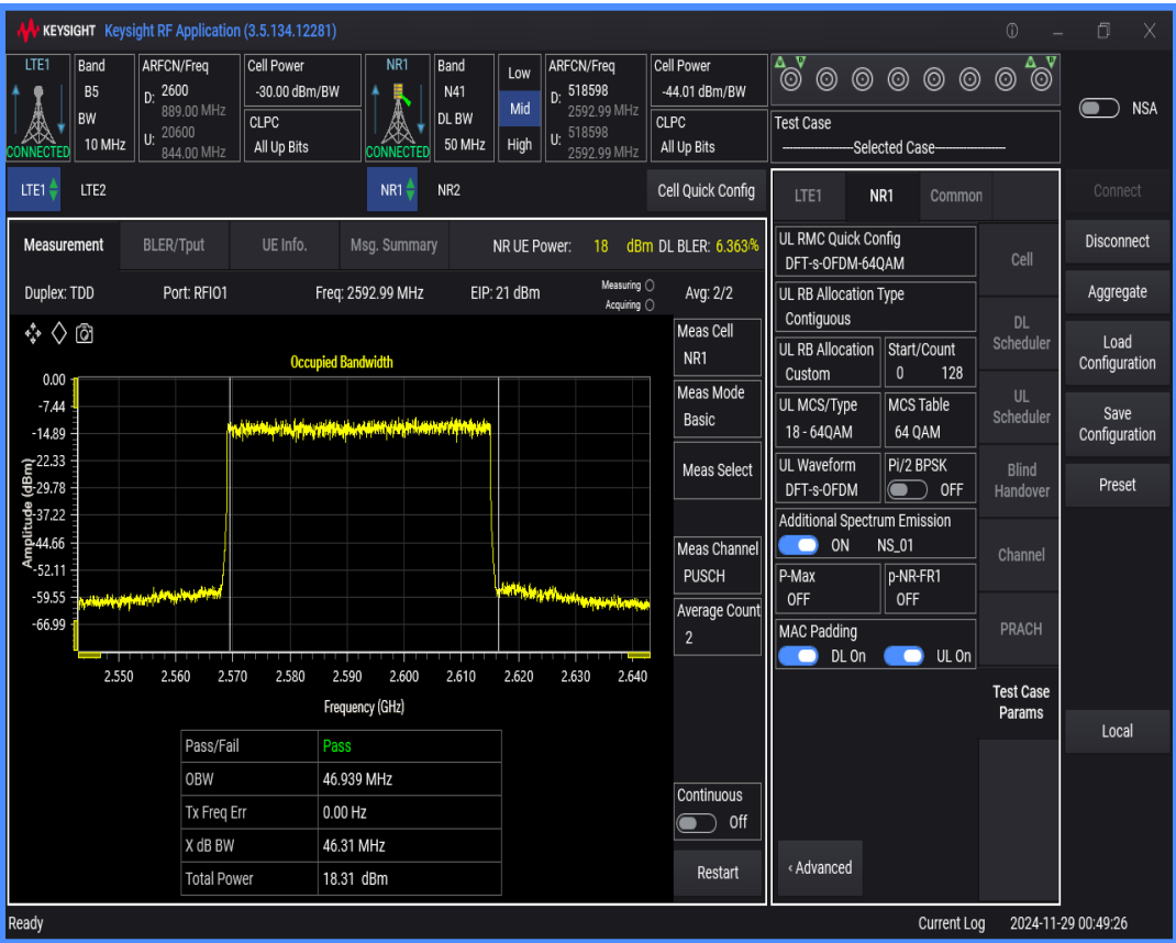
n41 SCS=30kHz DFT_QAM64 BW=40MHz Channel=518598 RB=100@0
