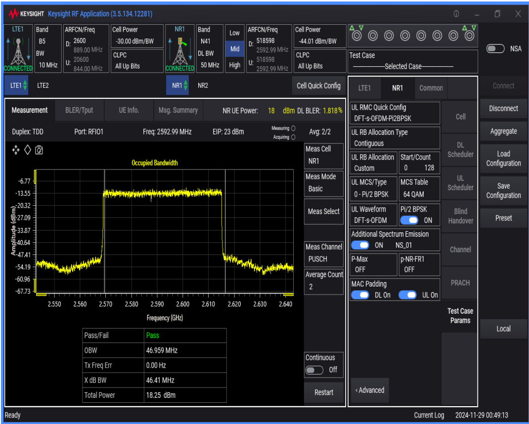
n41 SCS=30kHz DFT_QAM16 BW=60MHz Channel=518598 RB=162@0
