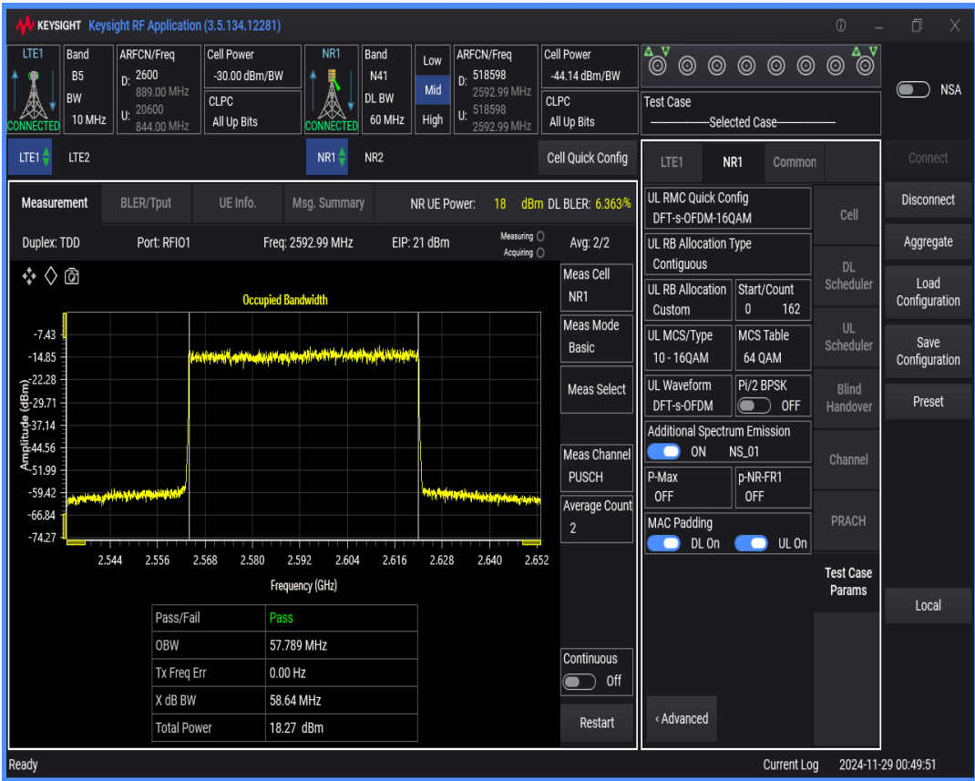
n41 SCS=30kHz DFT_QAM16 BW=50MHz Channel=518598 RB=128@0
