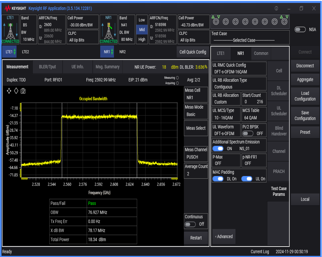
n41 SCS=30kHz DFT_QAM16 BW=90MHz Channel=518598 RB=240@0
