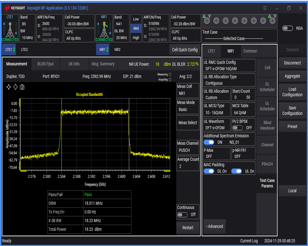
n41 SCS=30kHz DFT_QAM16 BW=100MHz Channel=518598 RB=270@0
