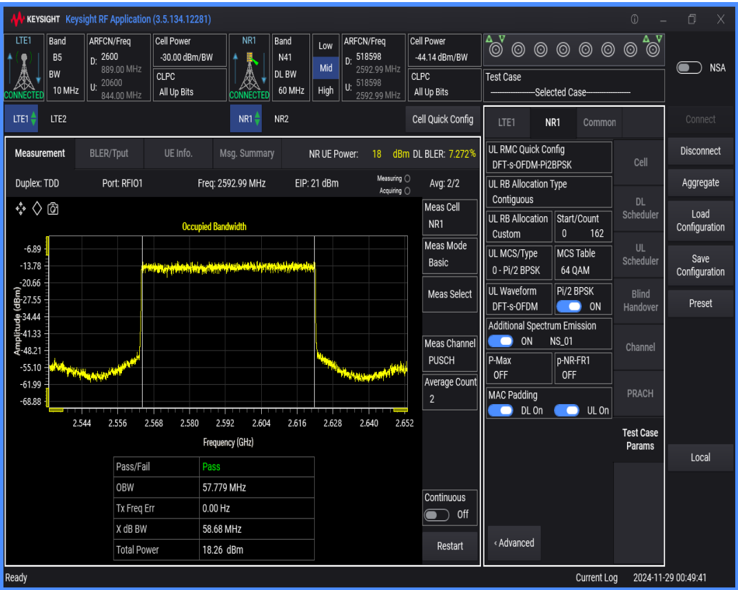
n41 SCS=30kHz DFT_BPSK BW=50MHz Channel=518598 RB=128@0
