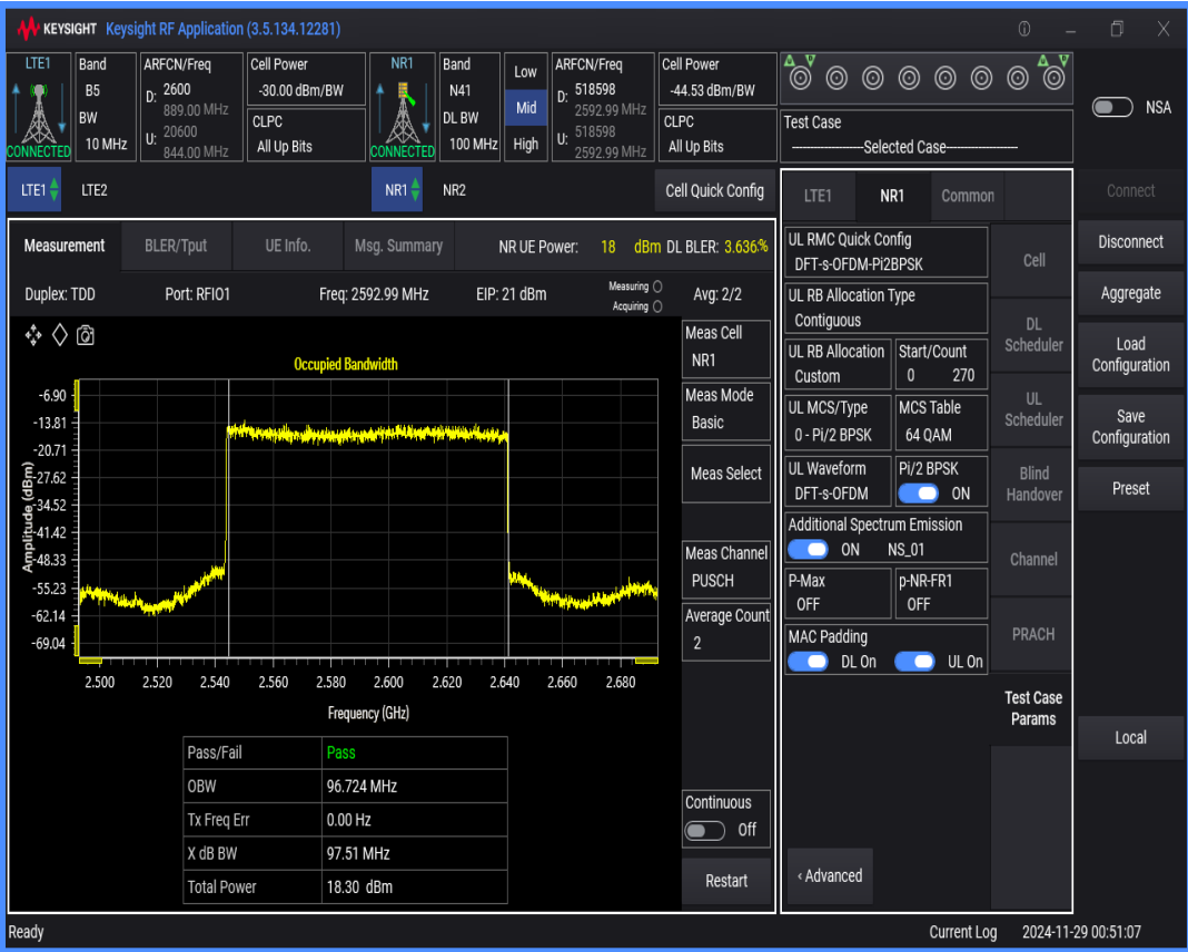
n41 SCS=30kHz DFT_BPSK BW=90MHz Channel=518598 RB=240@0
