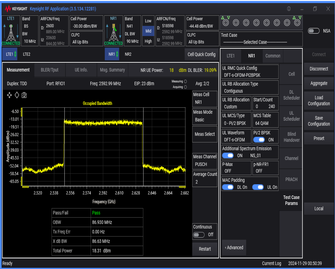
n41 SCS=30kHz DFT_BPSK BW=80MHz Channel=518598 RB=216@0
