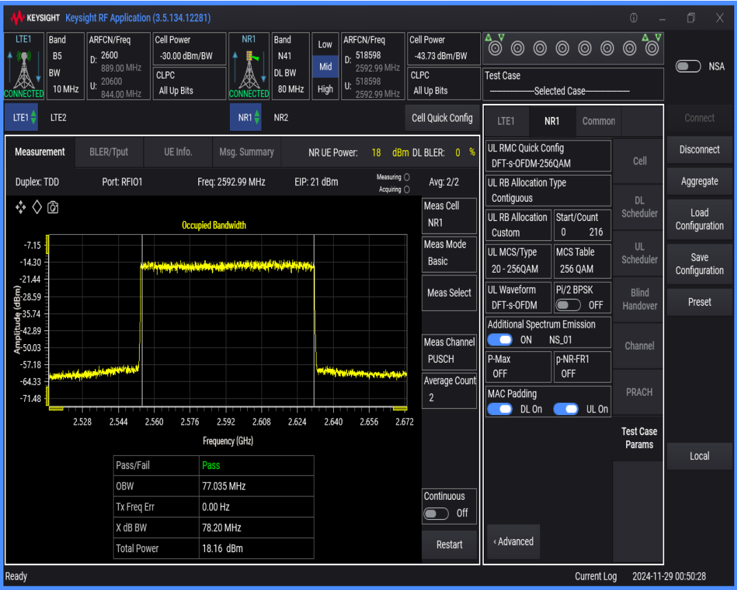
n41 SCS=30kHz DFT_QAM256 BW=60MHz Channel=518598 RB=162@0
