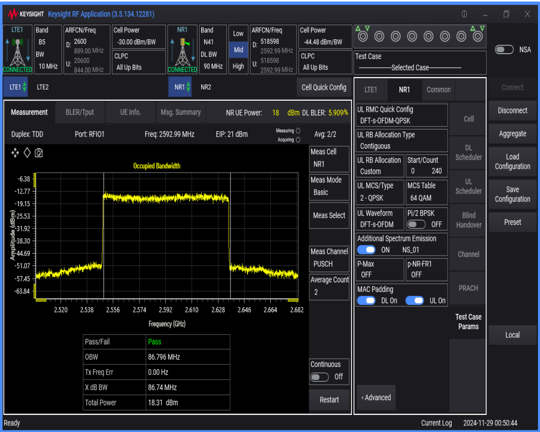
n41 SCS=30kHz DFT_QPSK BW=80MHz Channel=518598 RB=216@0
