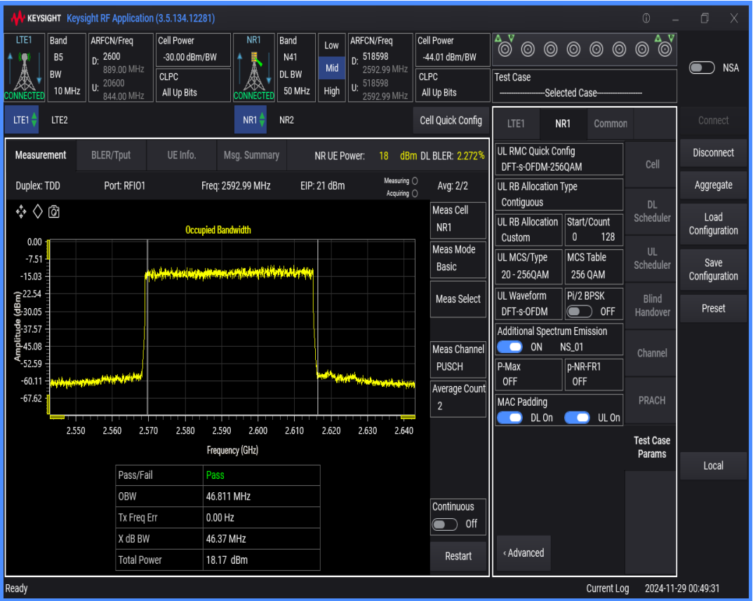
n41 SCS=30kHz DFT_QAM16 BW=80MHz Channel=518598 RB=216@0
