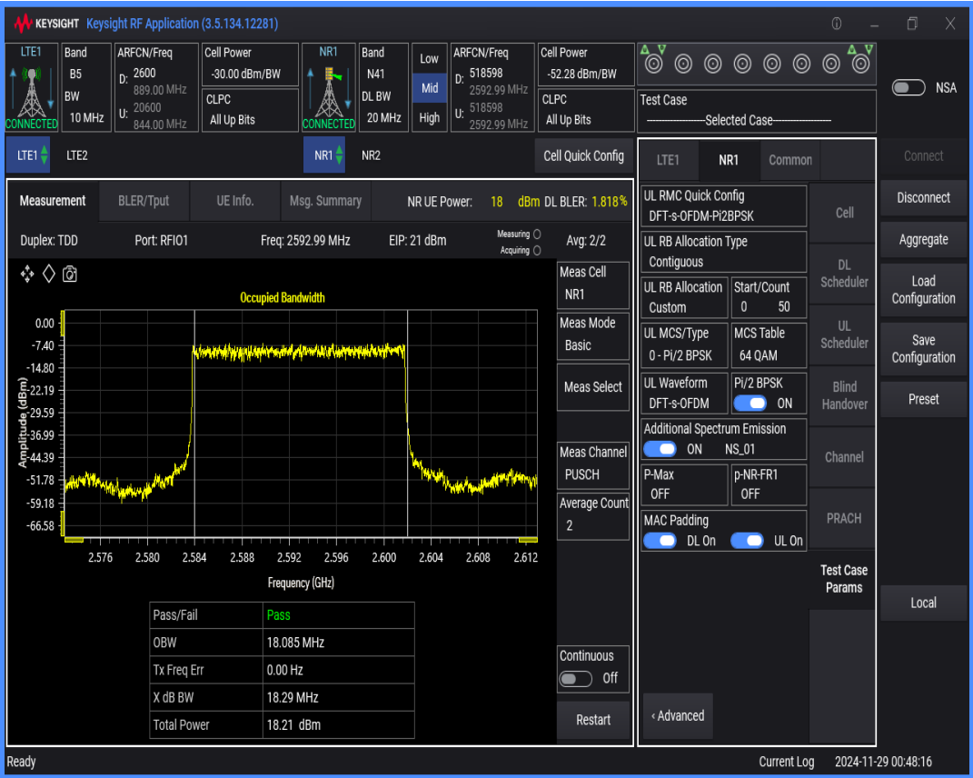
n41 SCS=30kHz DFT_BPSK BW=60MHz Channel=518598 RB=162@0
