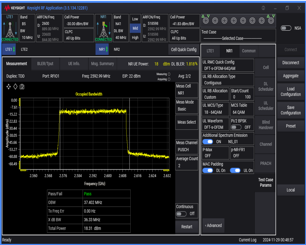
n41 SCS=30kHz DFT_QAM64 BW=80MHz Channel=518598 RB=216@0
