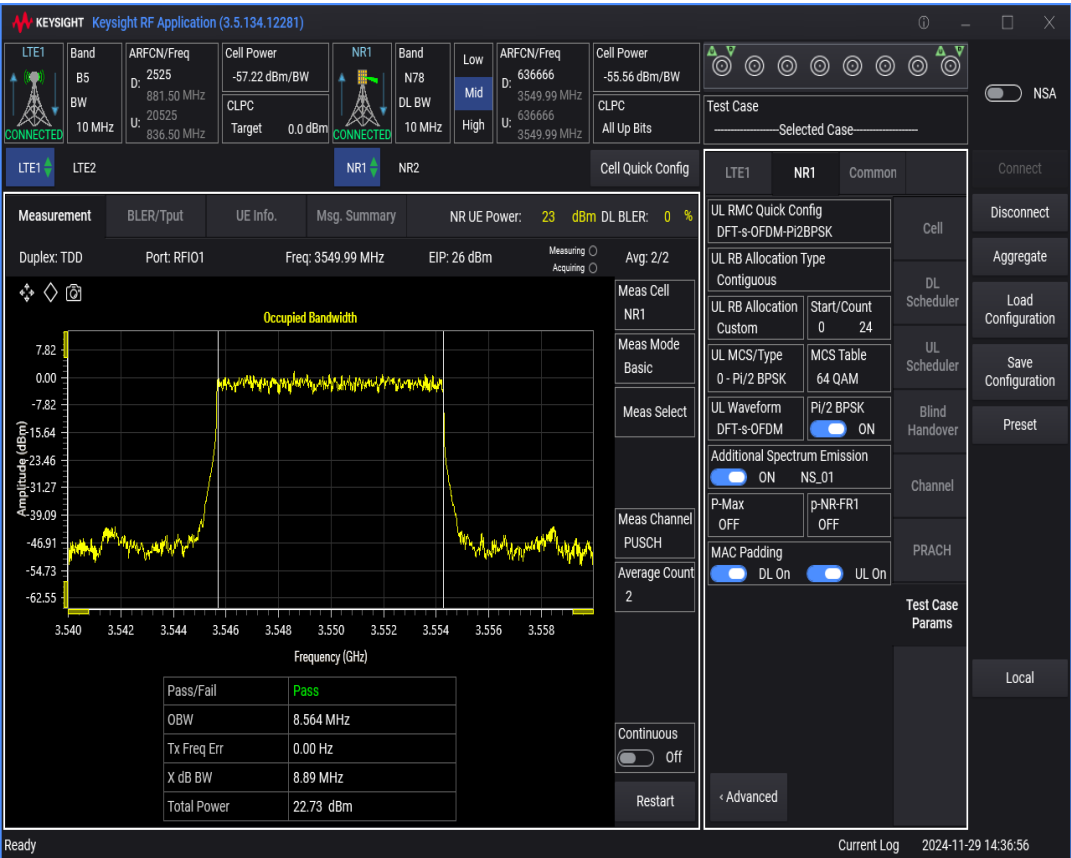
n78 SCS=30kHz DFT_QAM16 BW=10MHz Channel=636666 RB=24@0
