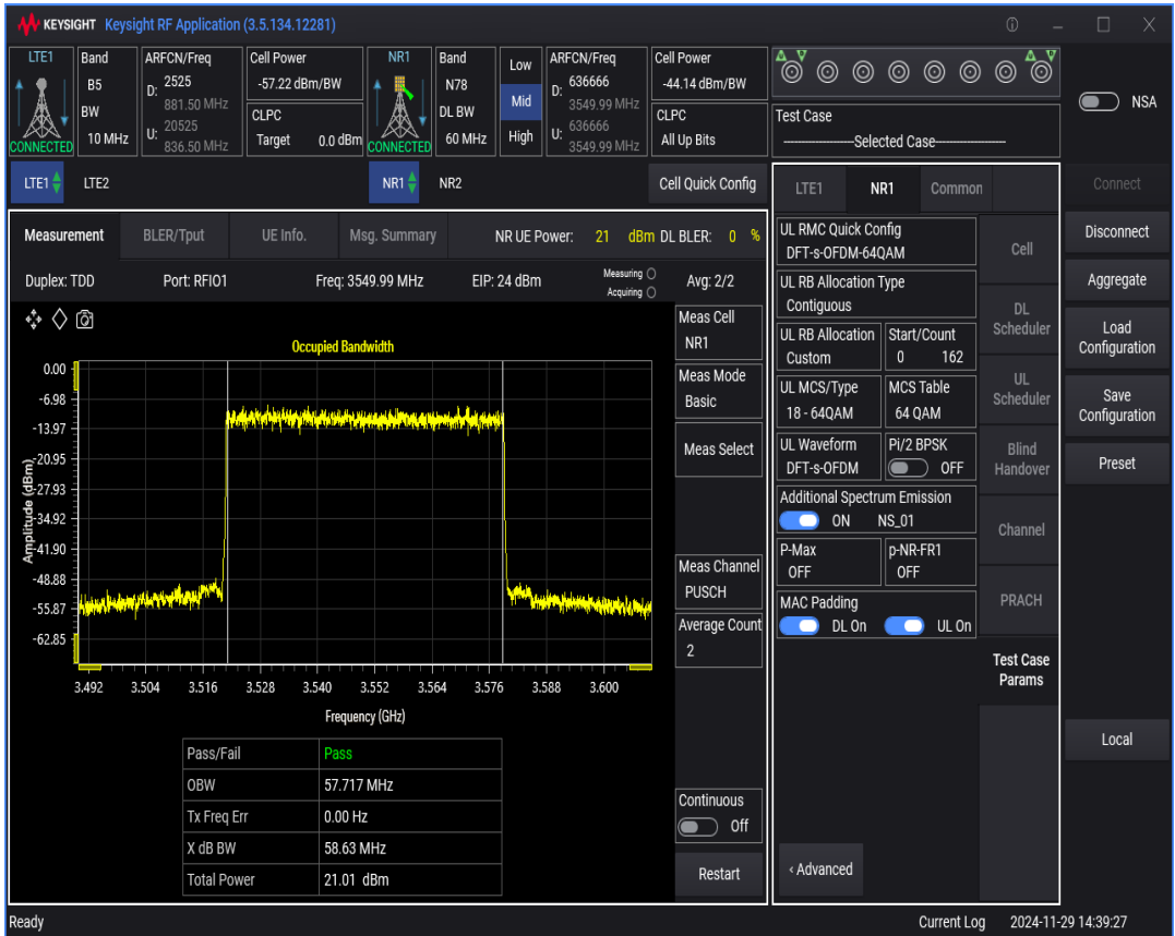
n78 SCS=30kHz DFT_QAM256 BW=90MHz Channel=636666 RB=240@0
