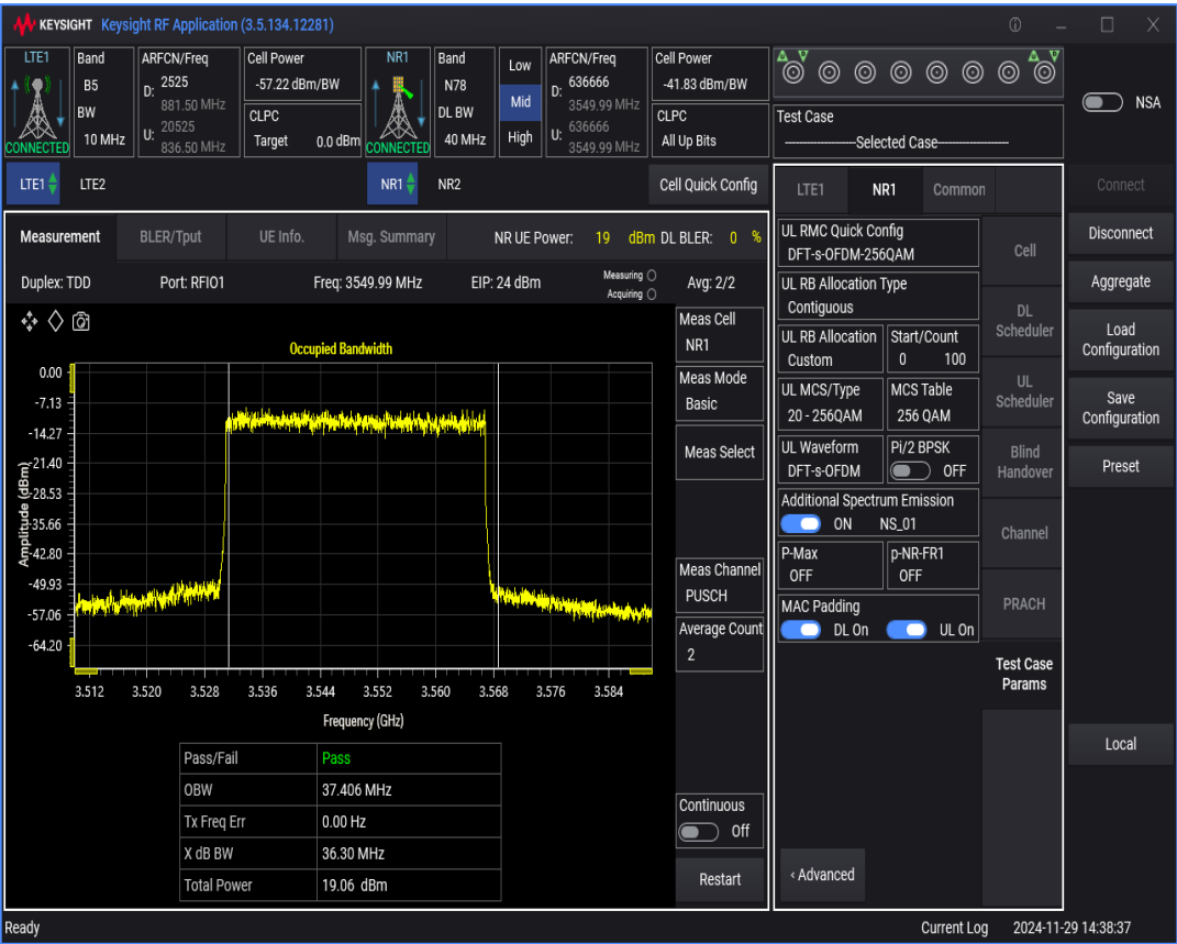
n78 SCS=30kHz DFT_QAM256 BW=15MHz Channel=636666 RB=36@0
