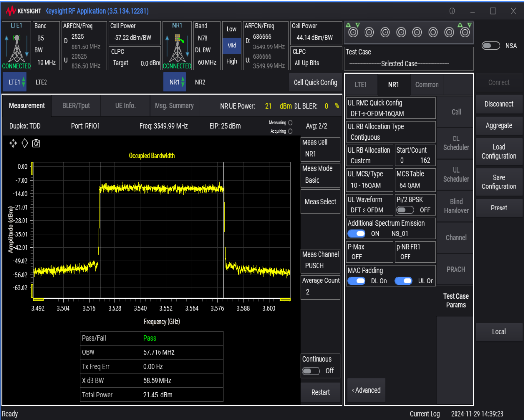
n78 SCS=30kHz DFT_QAM256 BW=50MHz Channel=636666 RB=128@0
