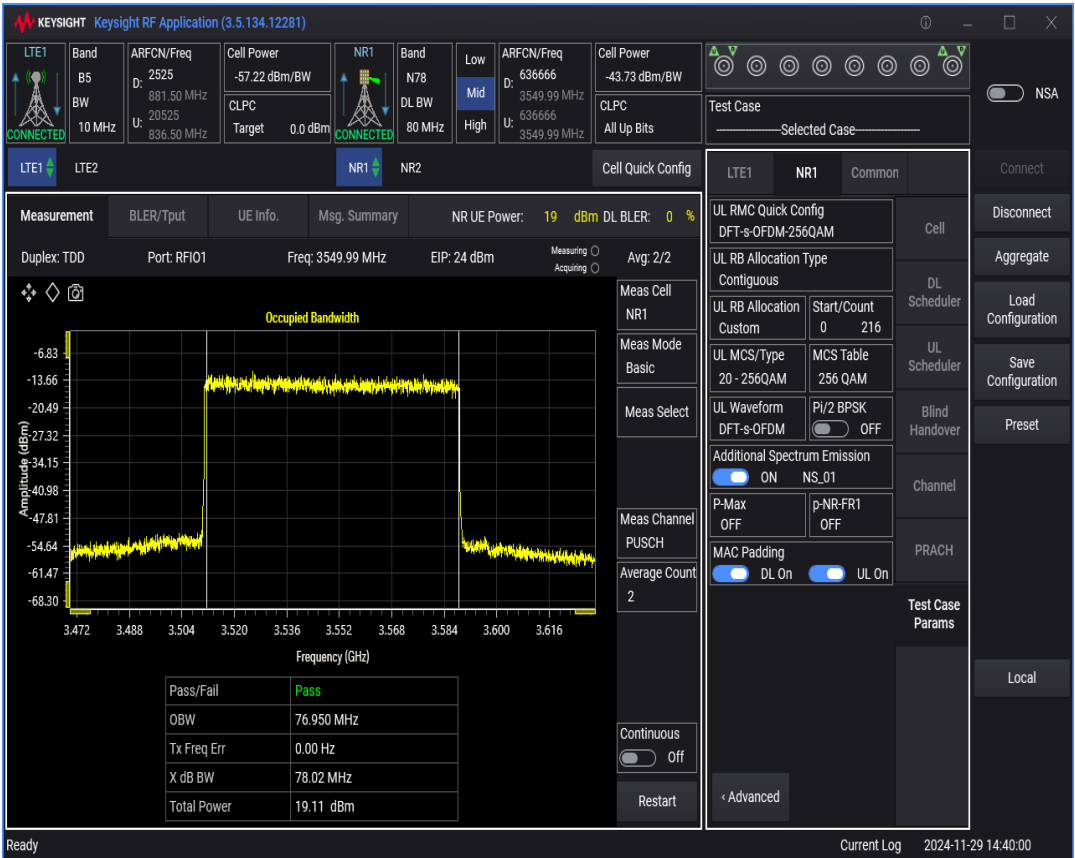
n78 SCS=30kHz DFT_QAM64 BW=100MHz Channel=636666 RB=270@0
