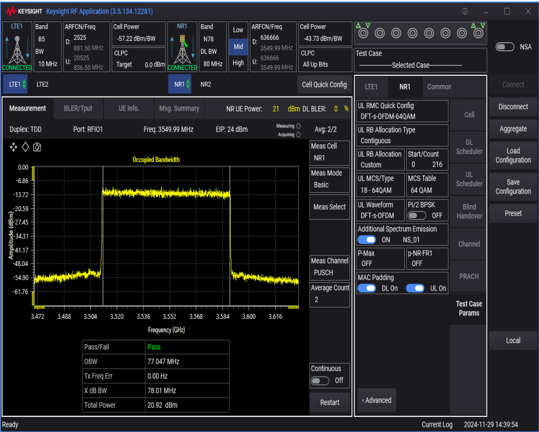
n78 SCS=30kHz DFT_QAM64 BW=60MHz Channel=636666 RB=162@0
