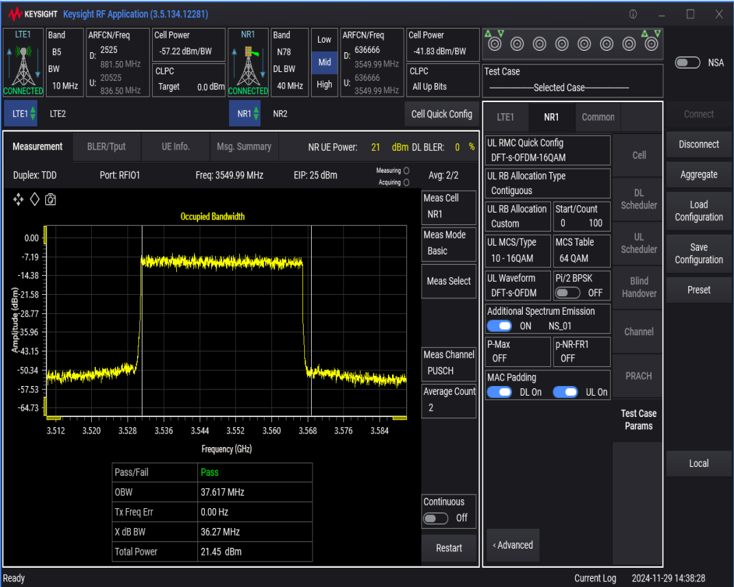
n78 SCS=30kHz DFT_QAM16 BW=50MHz Channel=636666 RB=128@0
