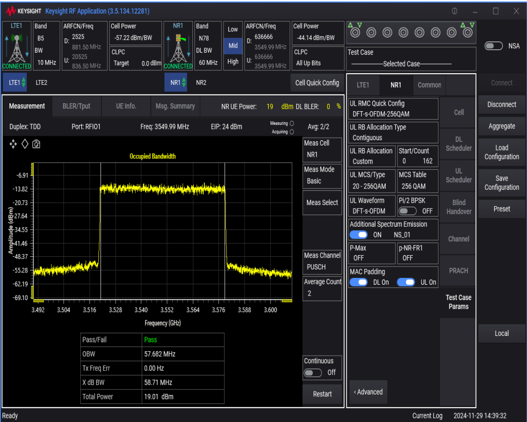
n78 SCS=30kHz DFT_QAM256 BW=40MHz Channel=636666 RB=100@0
