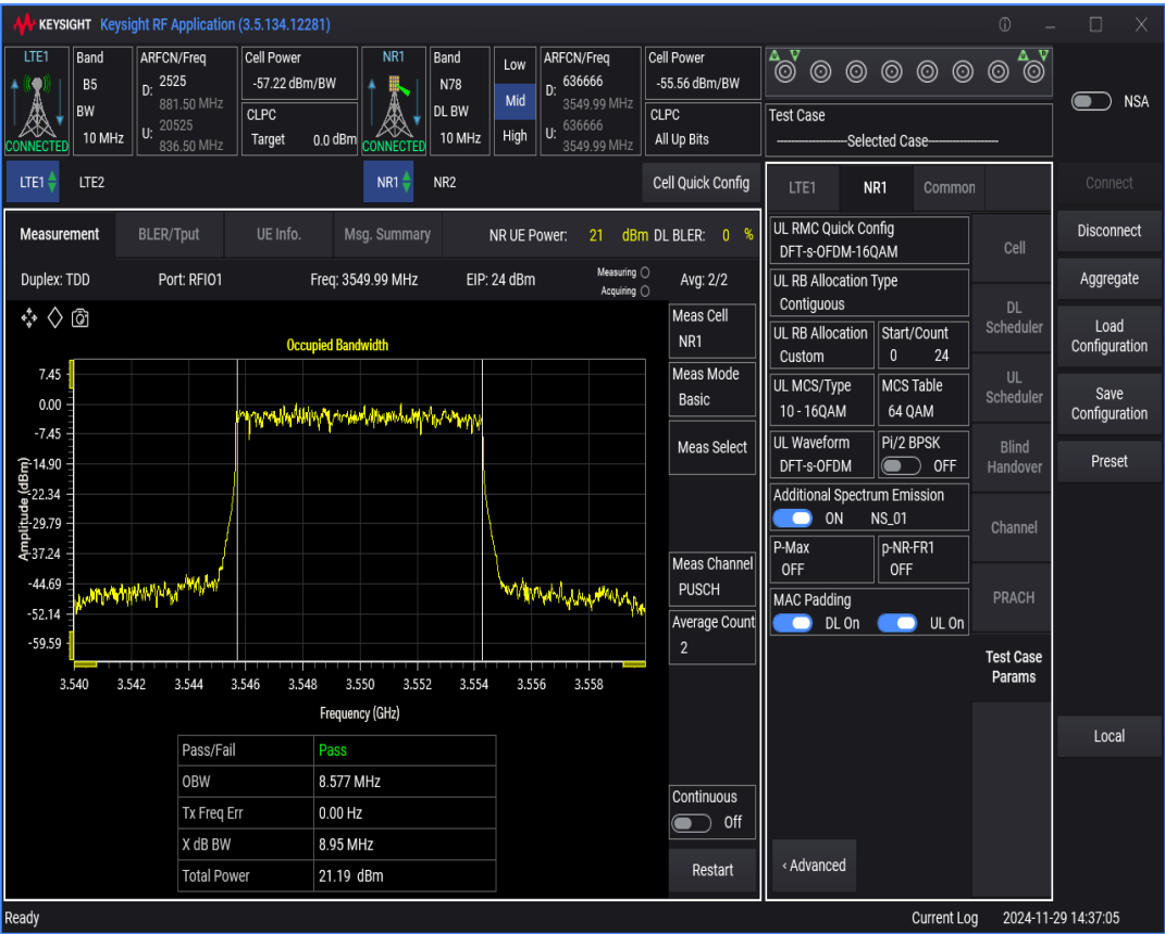
n78 SCS=30kHz DFT_QAM16 BW=100MHz Channel=636666 RB=270@0
