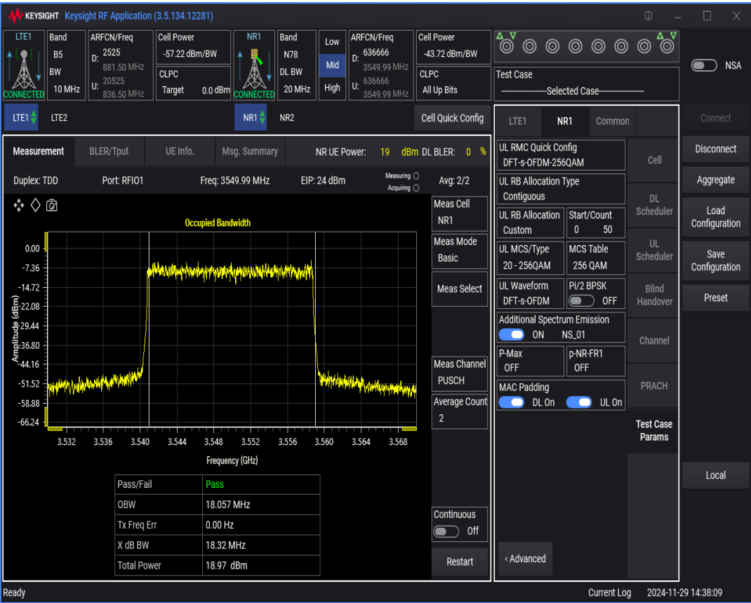
n78 SCS=30kHz DFT_QAM64 BW=40MHz Channel=636666 RB=100@0
