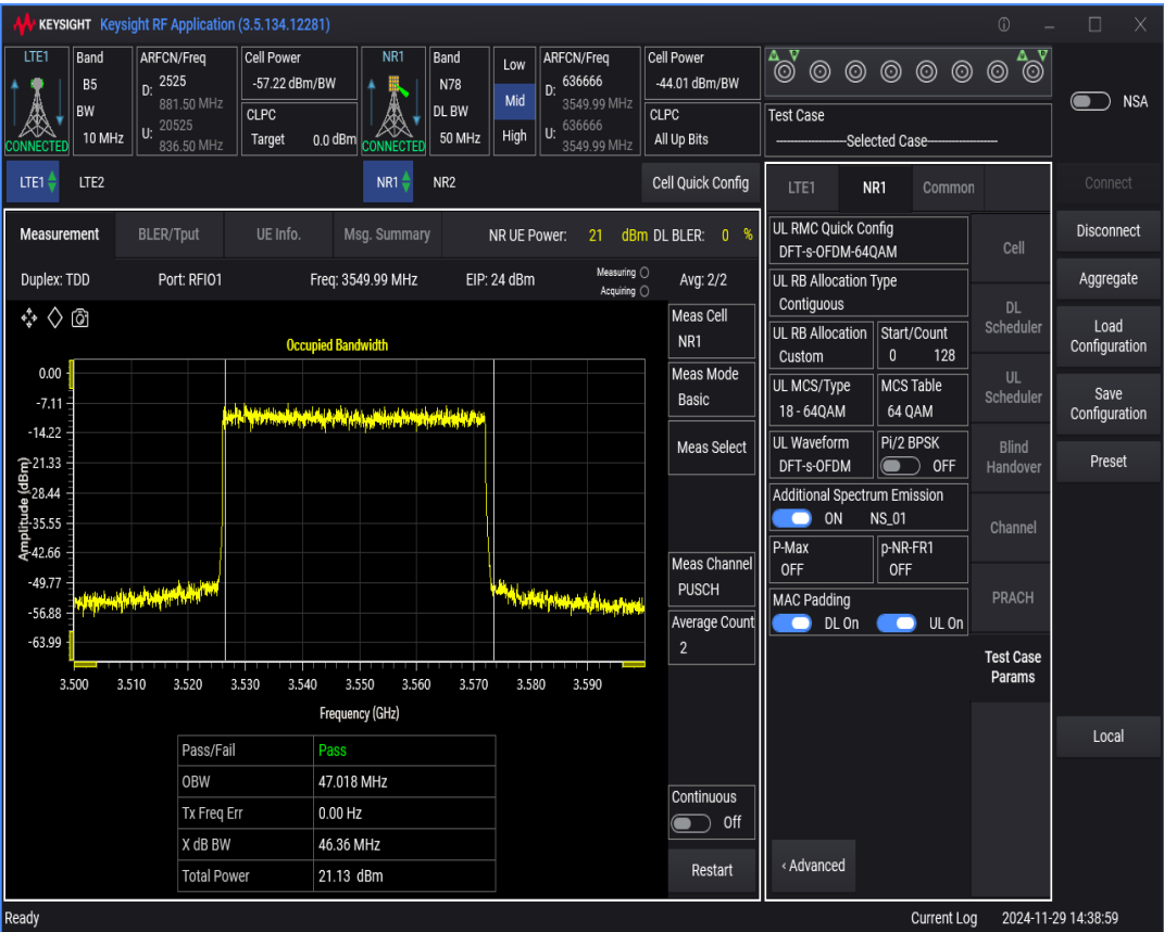
n78 SCS=30kHz DFT_QAM64 BW=80MHz Channel=636666 RB=216@0
