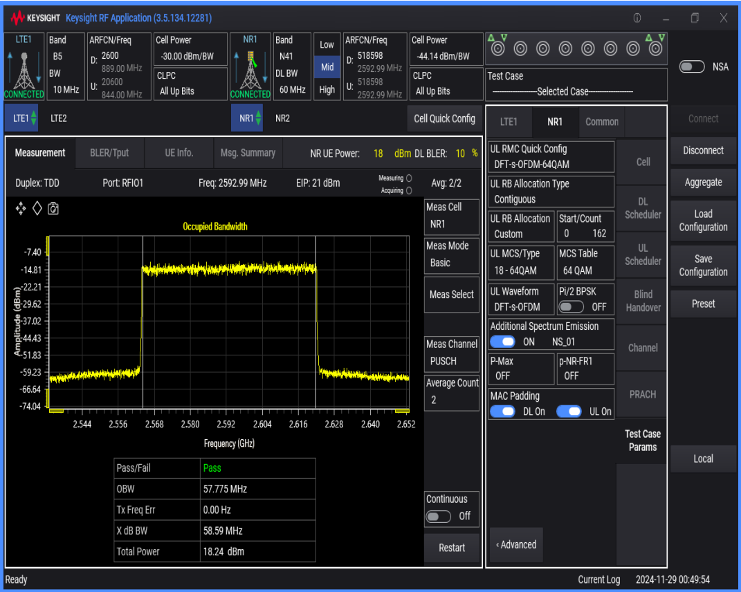
n41 SCS=30kHz DFT_QAM64 BW=40MHz Channel=518598 RB=100@0
