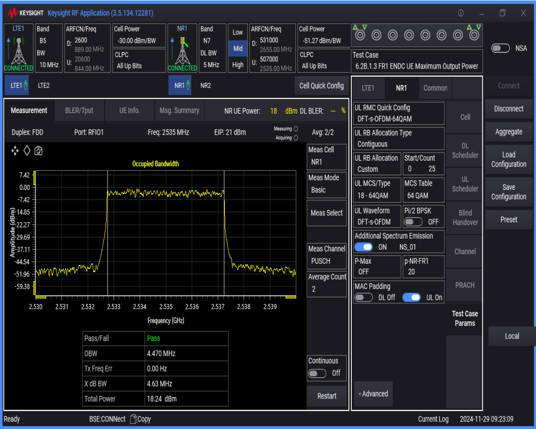
n7 SCS=15kHz DFT_QAM64 BW=20MHz Channel=507000 RB=100@0
