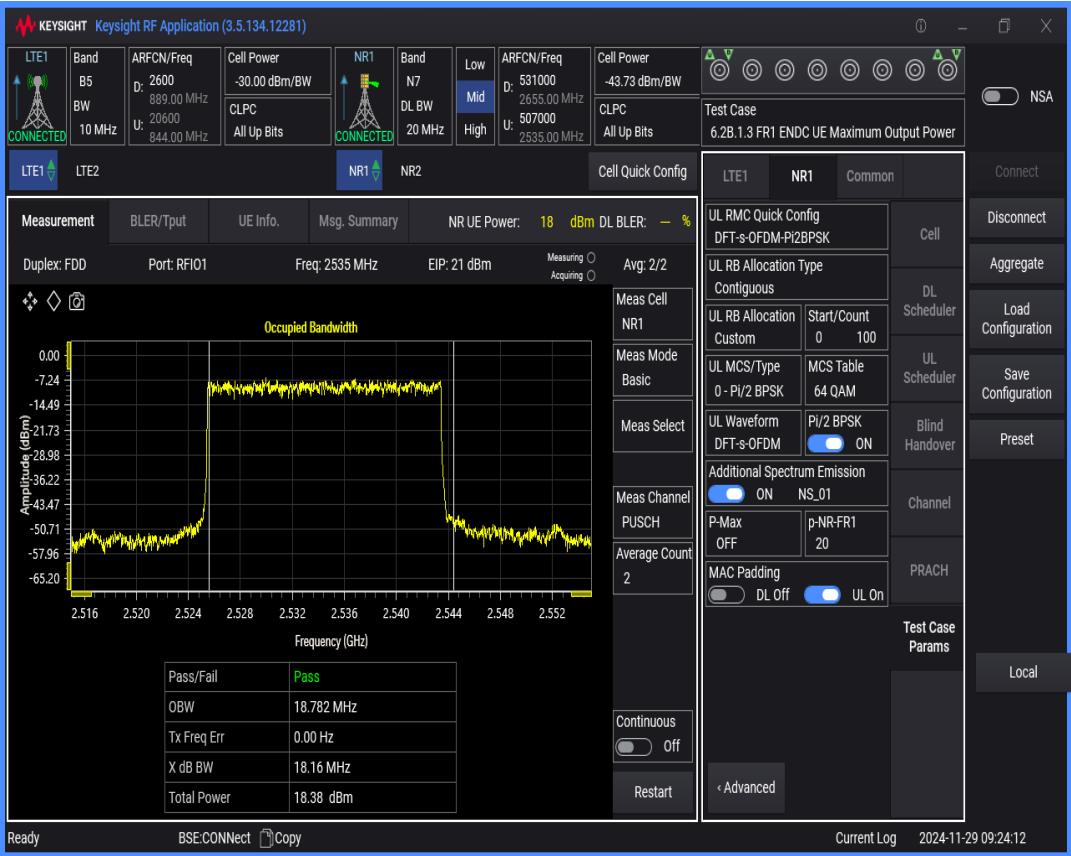
n7 SCS=15kHz DFT_QAM64 BW=5MHz Channel=507000 RB=25@0
