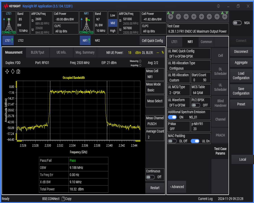
n7 SCS=15kHz DFT_QAM64 BW=15MHz Channel=507000 RB=75@0
