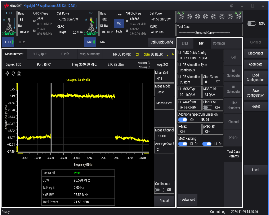
n78 SCS=30kHz DFT_BPSK BW=60MHz Channel=636666 RB=162@0
