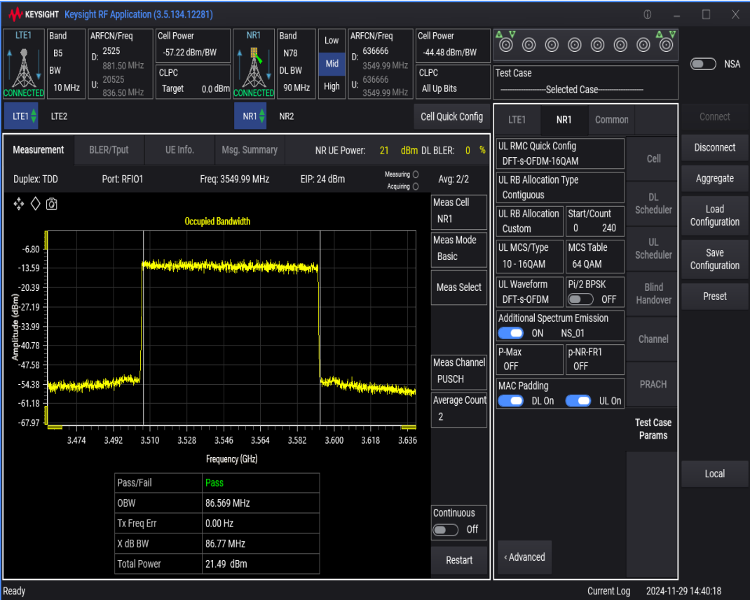
n78 SCS=30kHz DFT_QAM16 BW=80MHz Channel=636666 RB=216@0
