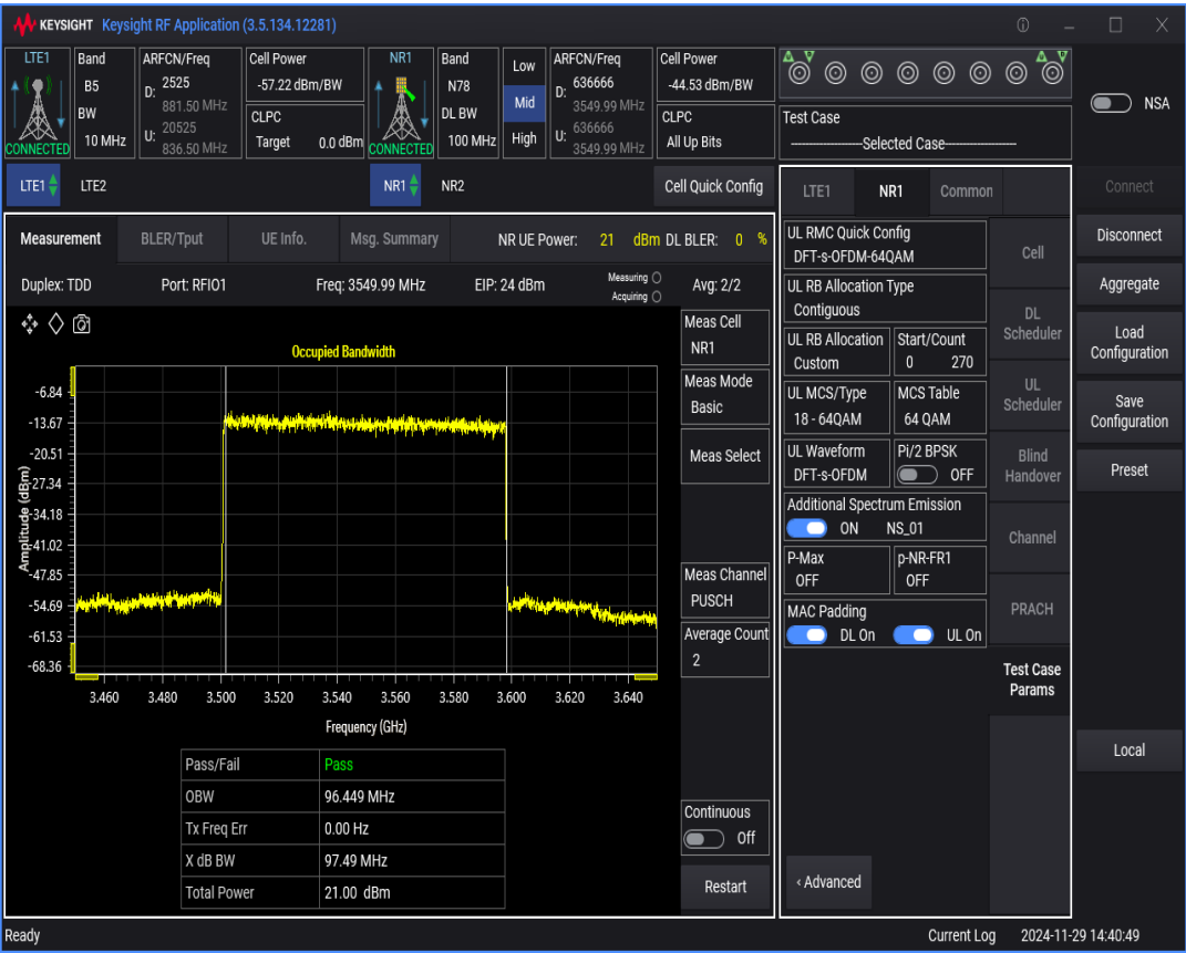
n78 SCS=30kHz DFT_QAM256 BW=60MHz Channel=636666 RB=162@0
