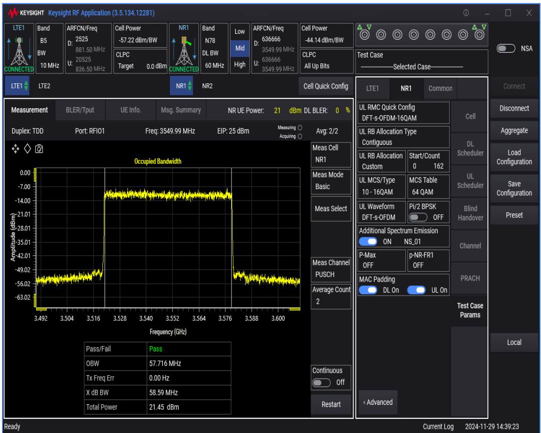
n78 SCS=30kHz DFT_QAM16 BW=50MHz Channel=636666 RB=128@0
