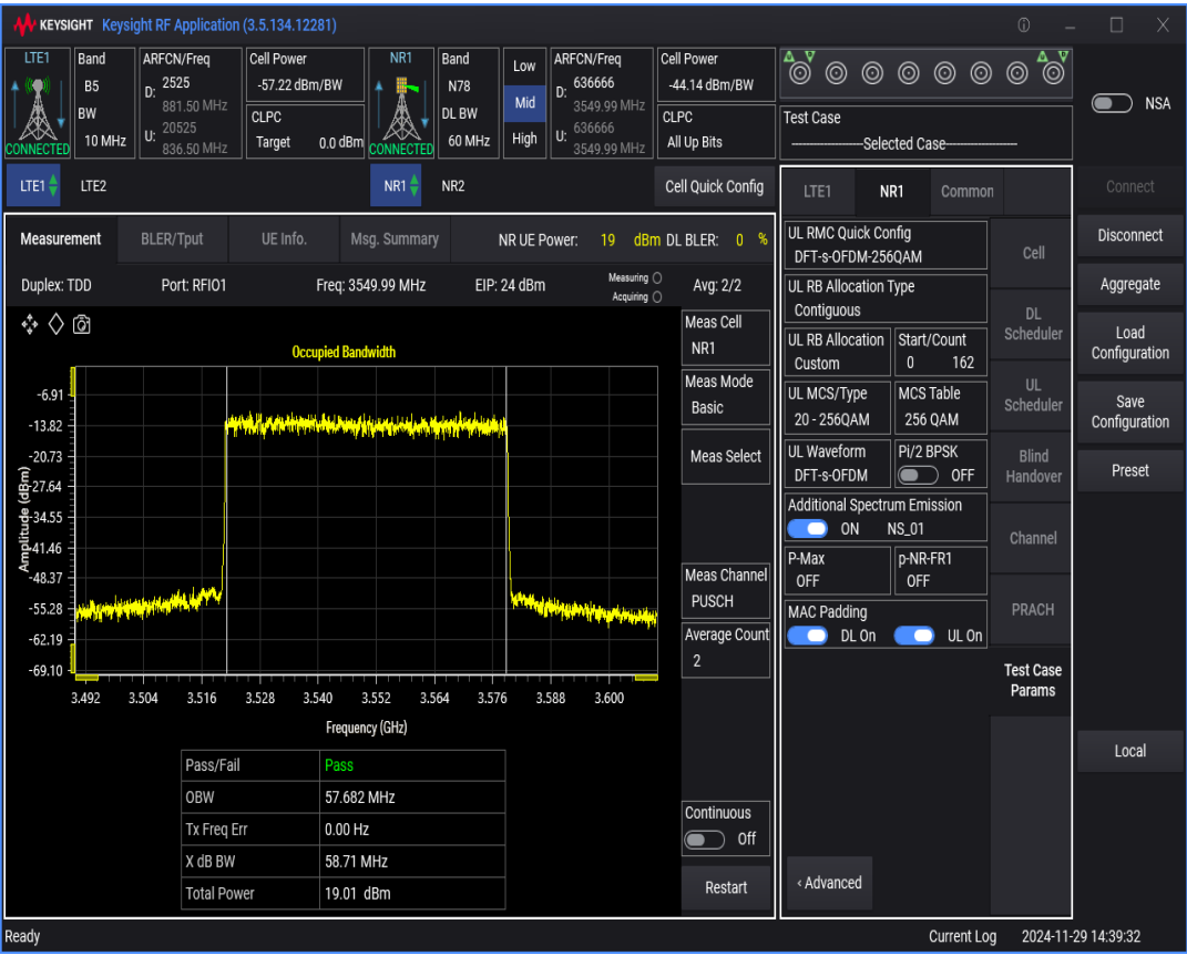
n78 SCS=30kHz DFT_QAM256 BW=50MHz Channel=636666 RB=128@0
