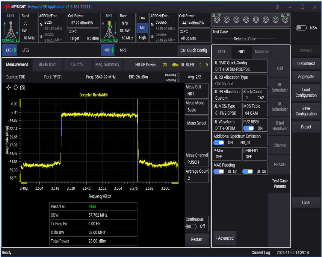
n78 SCS=30kHz DFT_BPSK BW=50MHz Channel=636666 RB=128@0
