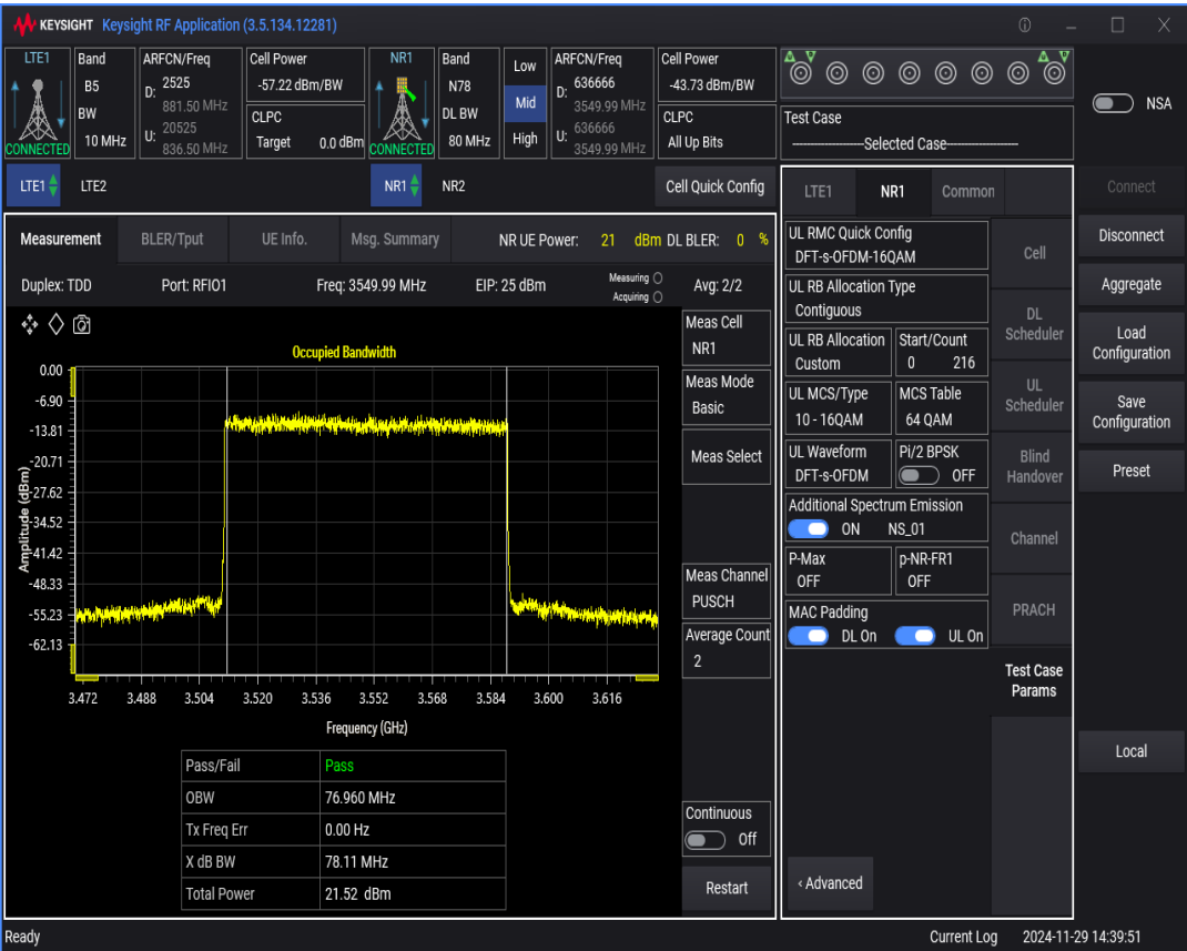
n78 SCS=30kHz DFT_QAM64 BW=15MHz Channel=636666 RB=36@0
