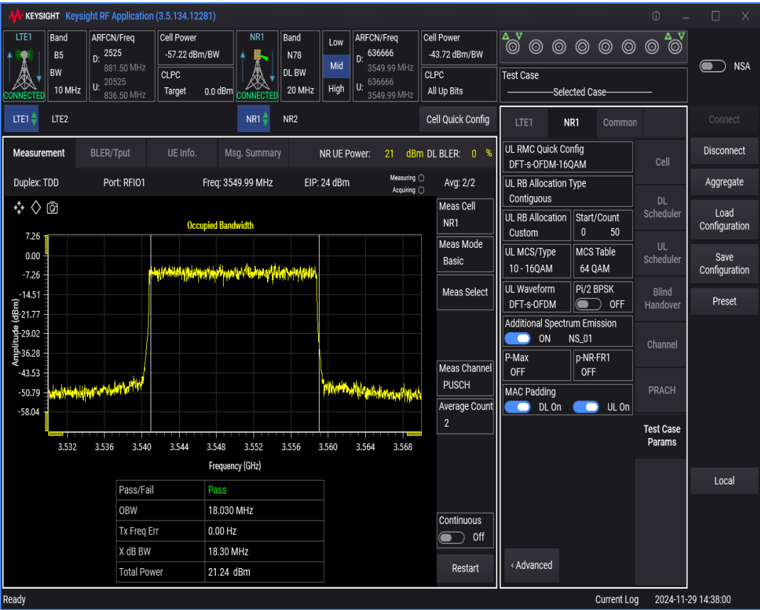
n78 SCS=30kHz DFT_QAM16 BW=100MHz Channel=636666 RB=270@0
