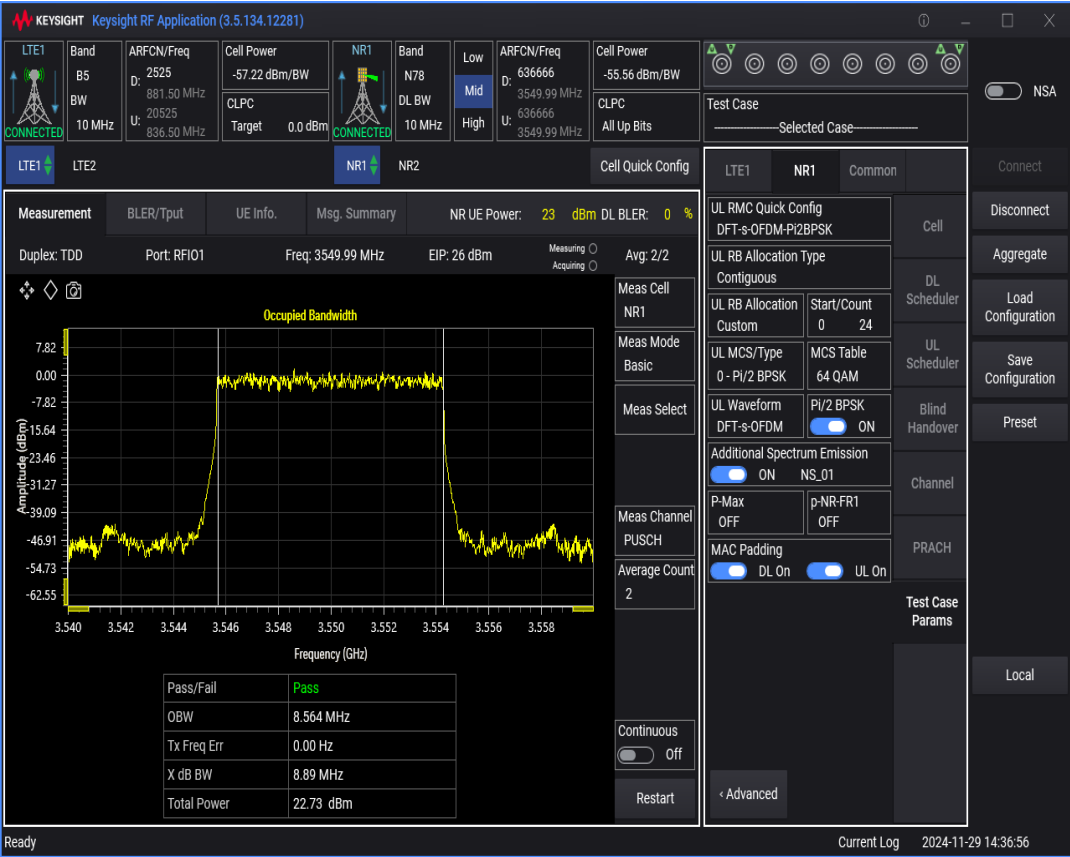
n78 SCS=30kHz DFT_QAM16 BW=15MHz Channel=636666 RB=36@0
