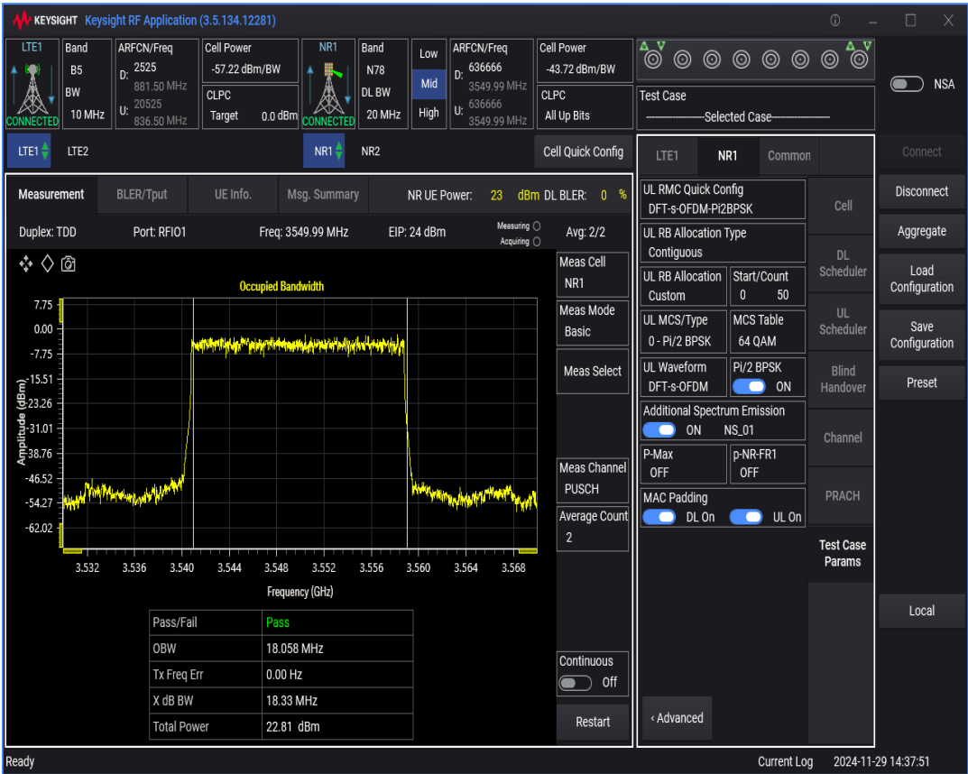
n78 SCS=30kHz DFT_BPSK BW=40MHz Channel=636666 RB=100@0
