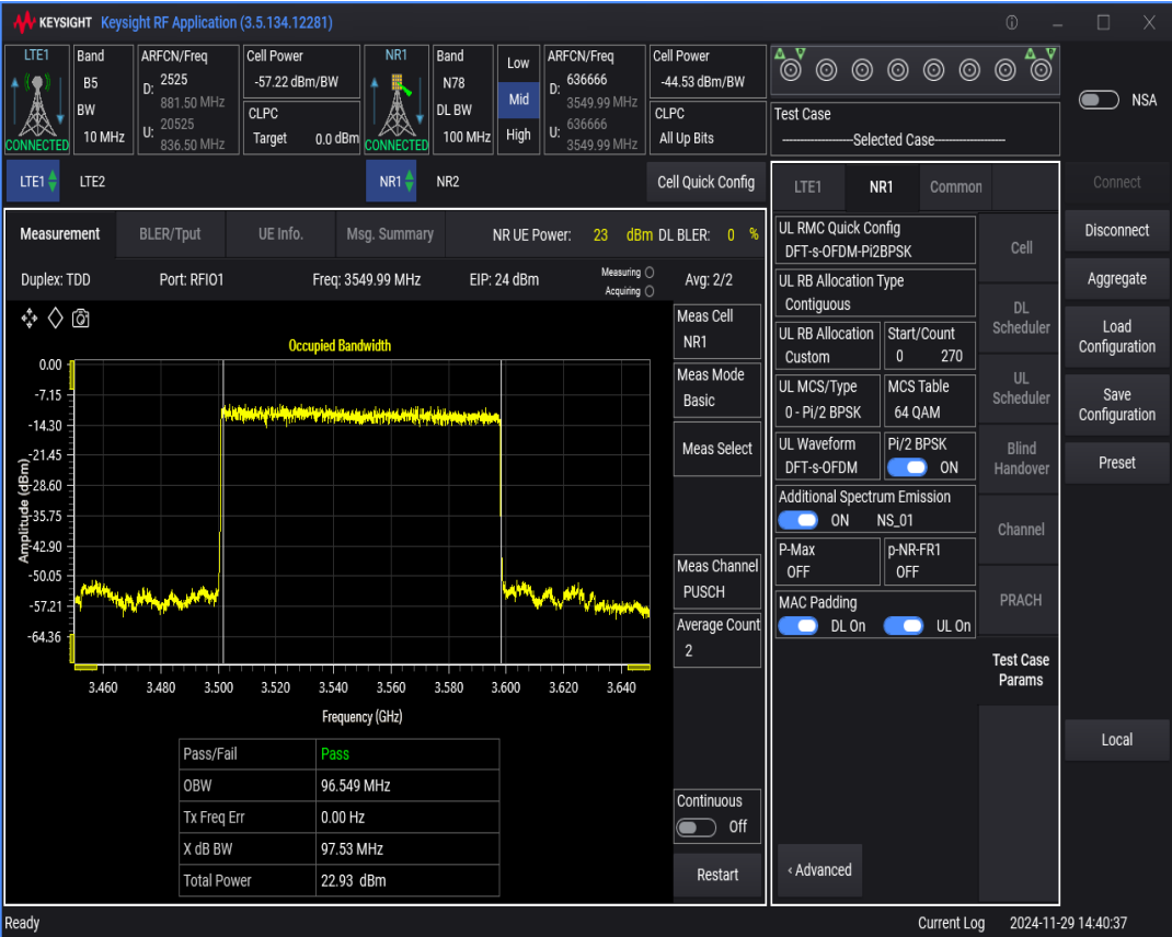
n78 SCS=30kHz DFT_BPSK BW=10MHz Channel=636666 RB=24@0
