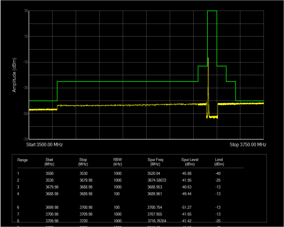
n78(3550-3700) SCS=30kHz CP_QPSK BW=10MHz Channel=646332 RB=24@0
