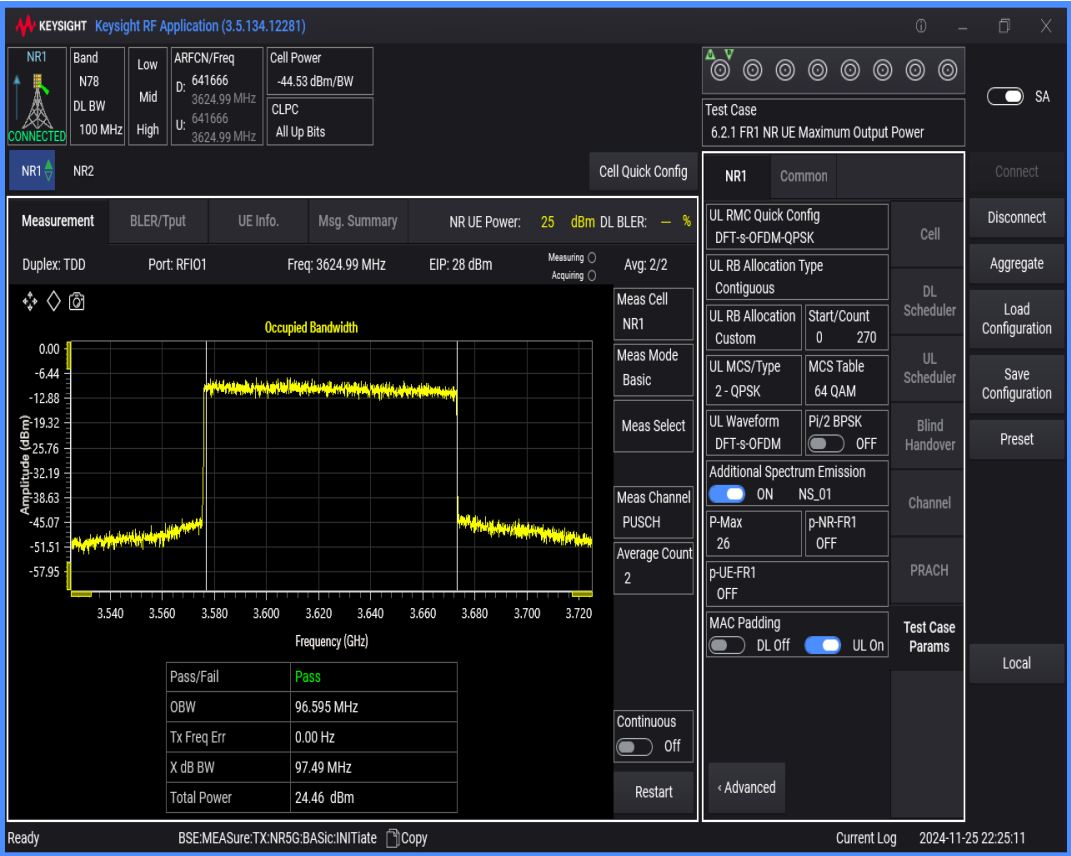
n78(3550-3700) SCS=30kHz DFT_QAM64 BW=80MHz Channel=641666 RB=216@0
