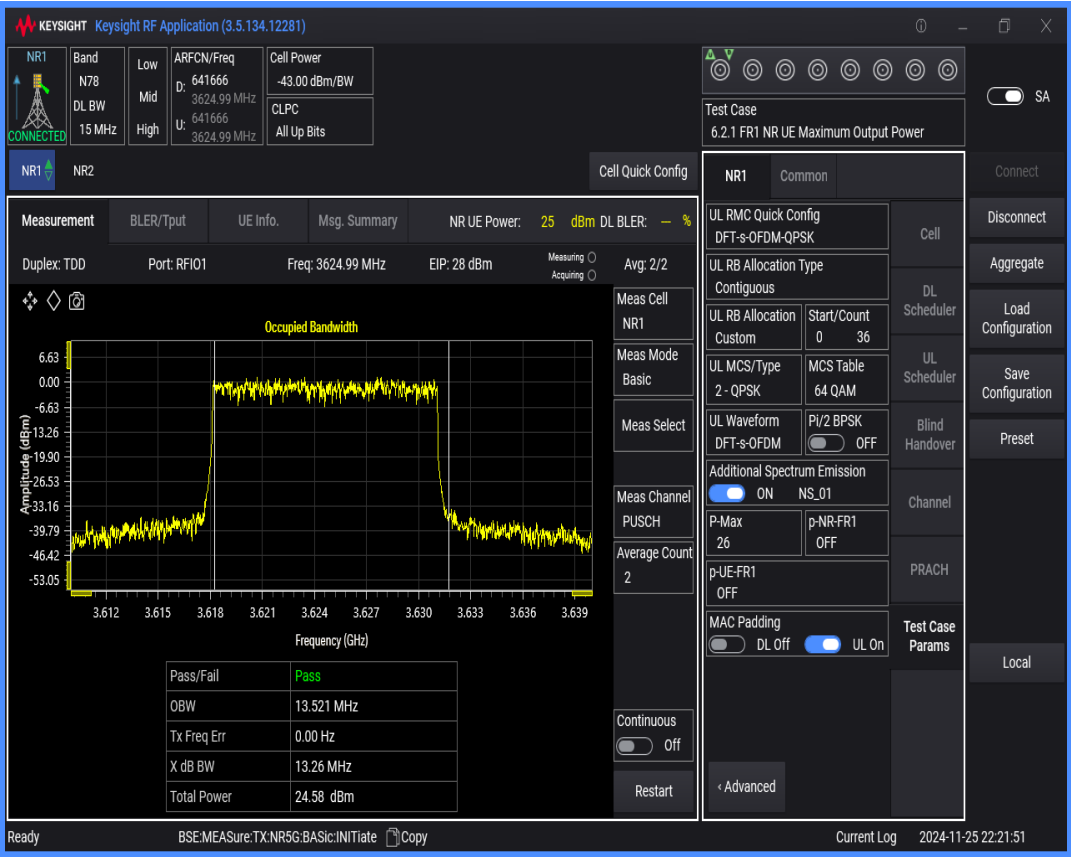
n78(3550-3700) SCS=30kHz DFT_QPSK BW=10MHz Channel=641666 RB=24@0
