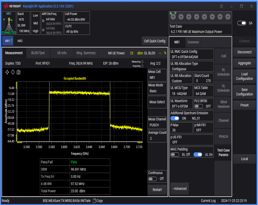
n78(3550-3700) SCS=30kHz DFT_QAM256 BW=80MHz Channel=641666 RB=216@0
