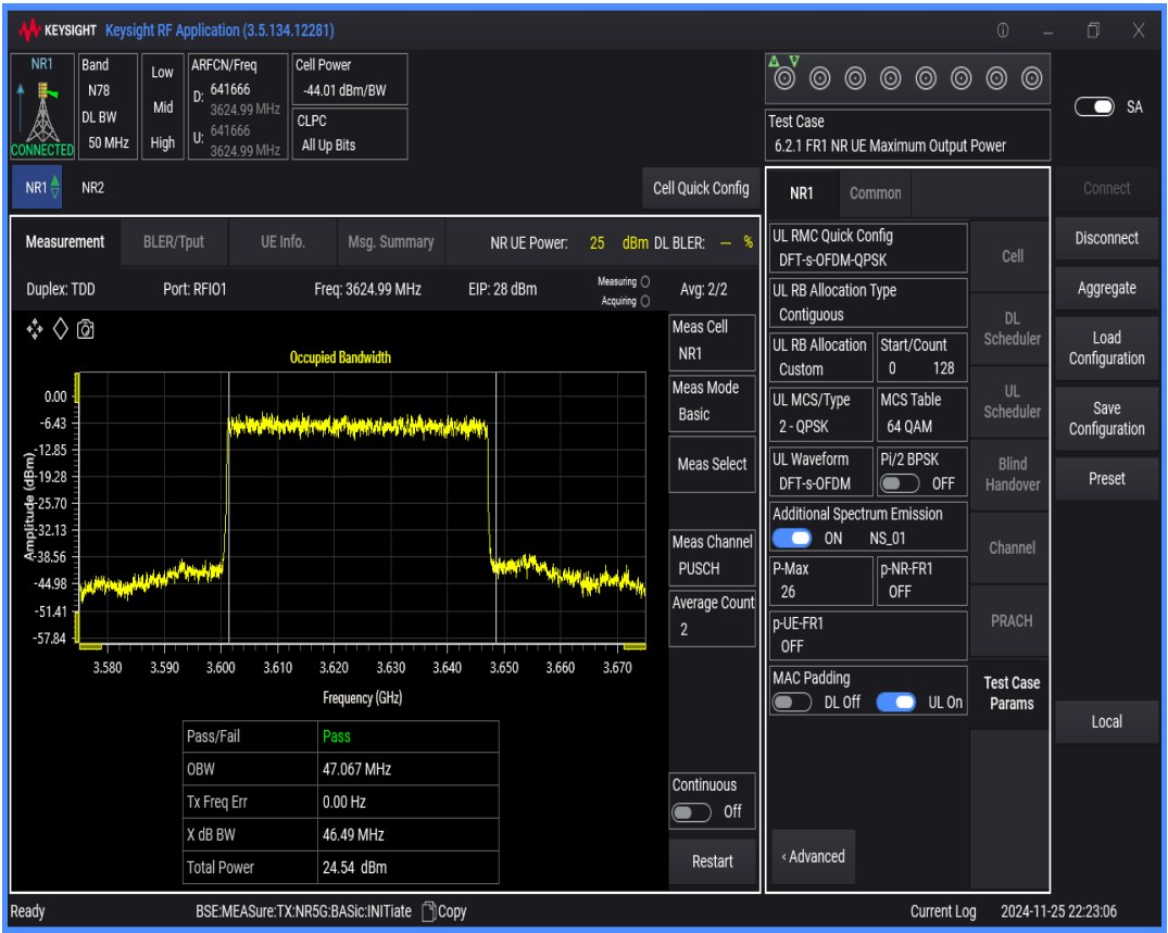
n78(3550-3700) SCS=30kHz DFT_QPSK BW=80MHz Channel=641666 RB=216@0
