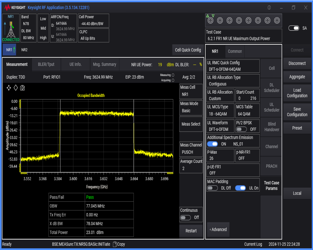
n78(3550-3700) SCS=30kHz DFT_QAM64 BW=60MHz Channel=641666 RB=162@0
