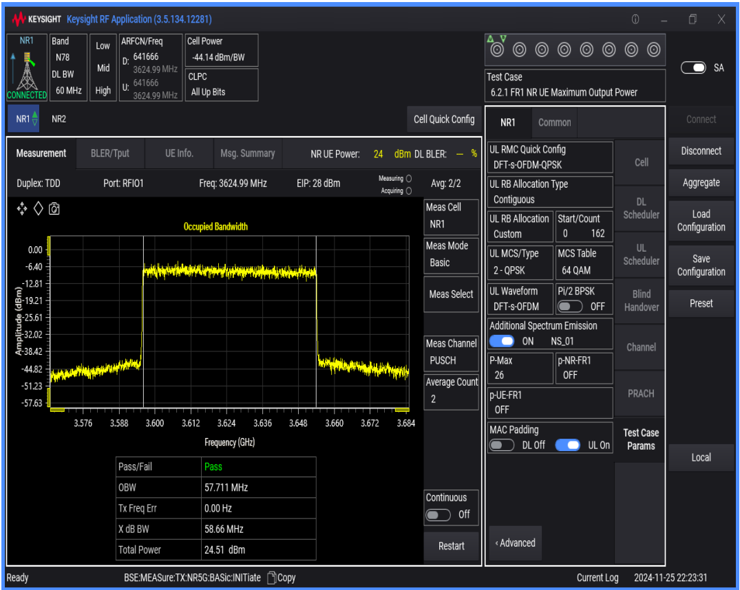
n78(3550-3700) SCS=30kHz DFT_QPSK BW=50MHz Channel=641666 RB=128@0
