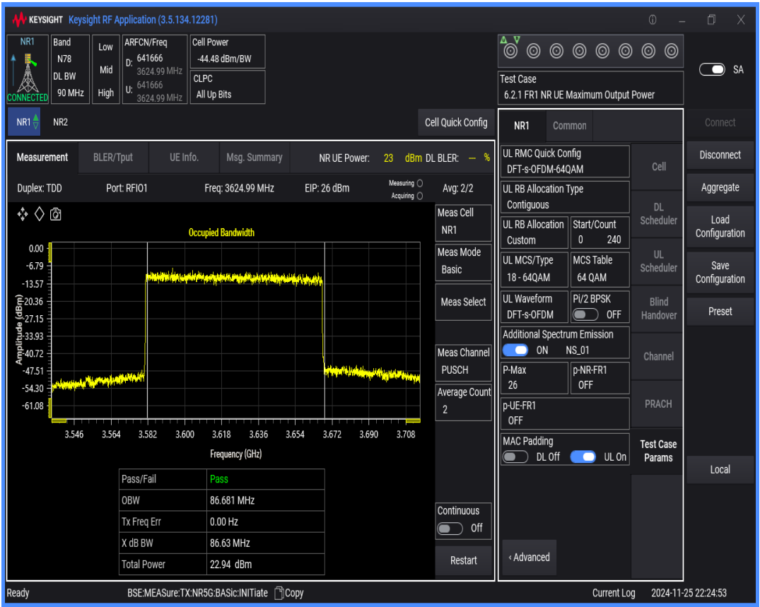
n78(3550-3700) SCS=30kHz DFT_QPSK BW=100MHz Channel=641666 RB=270@0
