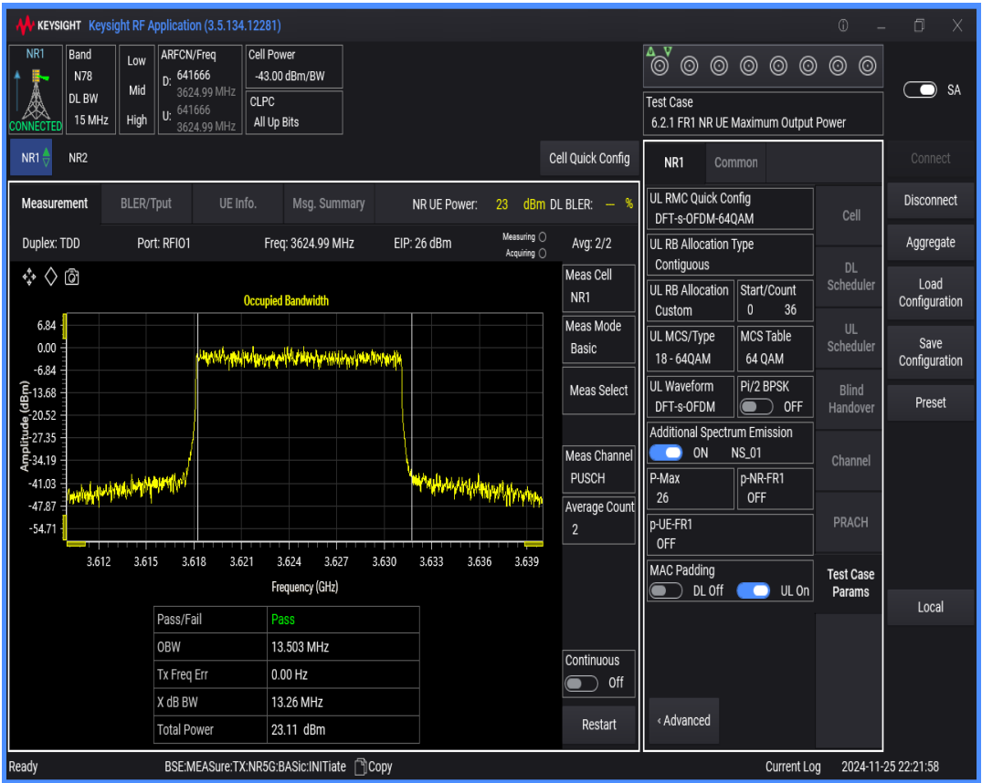
n78(3550-3700) SCS=30kHz DFT_QAM64 BW=90MHz Channel=641666 RB=240@0
