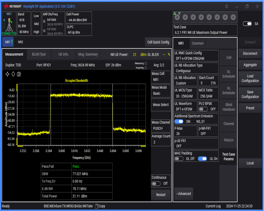
n78(3550-3700) SCS=30kHz DFT_QAM256 BW=60MHz Channel=641666 RB=162@0
