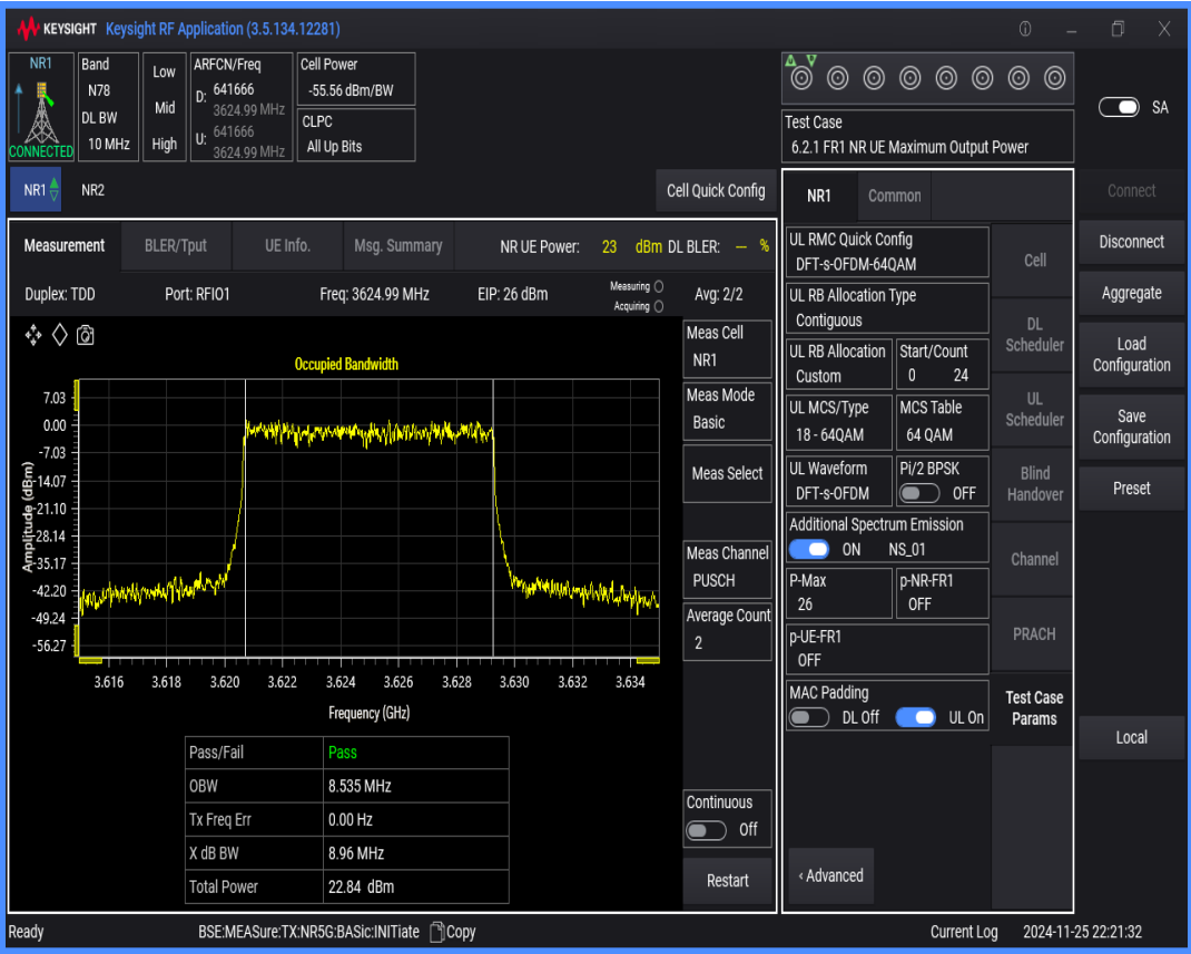
n78(3550-3700) SCS=30kHz DFT_QAM64 BW=15MHz Channel=641666 RB=36@0
