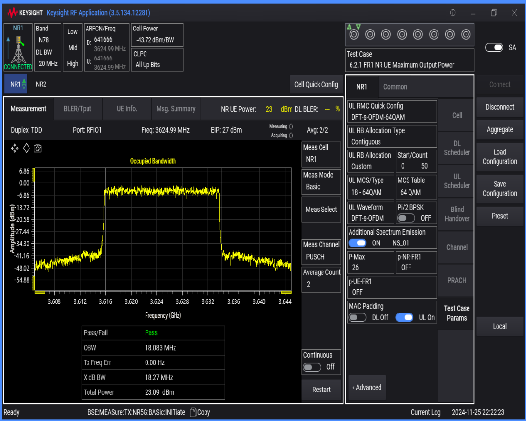
n78(3550-3700) SCS=30kHz DFT_QAM64 BW=10MHz Channel=641666 RB=24@0
