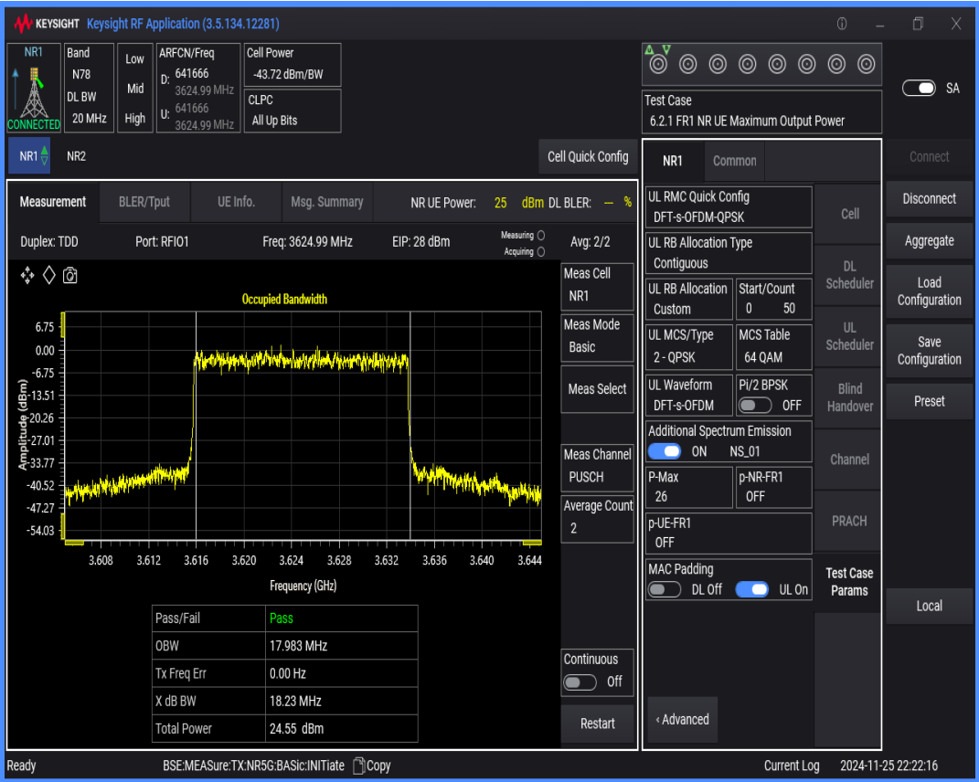
n78(3550-3700) SCS=30kHz DFT_QPSK BW=15MHz Channel=641666 RB=36@0
