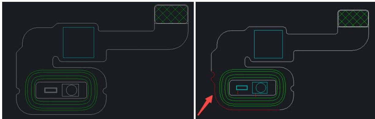
3. NFC Antenna: change material. (The material is changed from ferrite to absorber material, which does not affect NFC performance)
