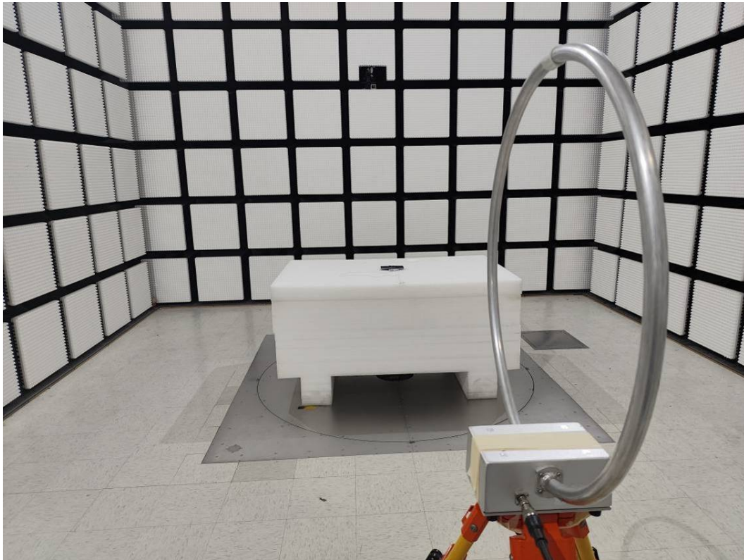
Radiated Emission Below 30MHz View Ground-parallel-2CII-6
