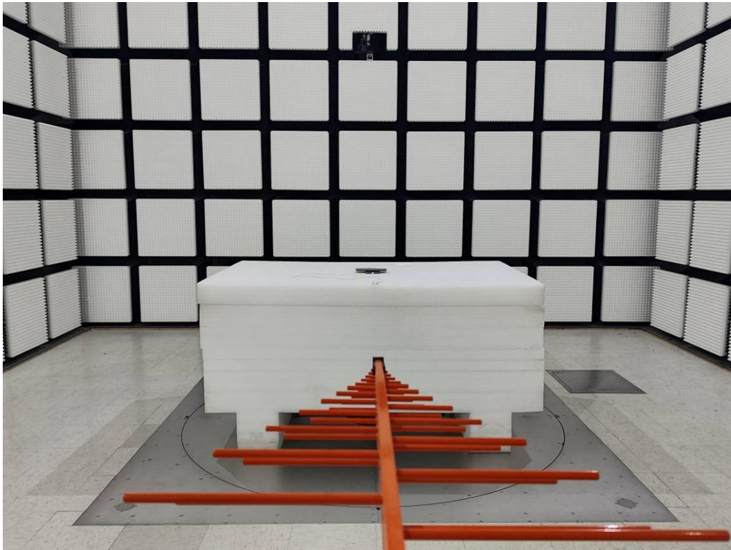
Radiated Emission Below 30MHz View Parallel-2CII-5
