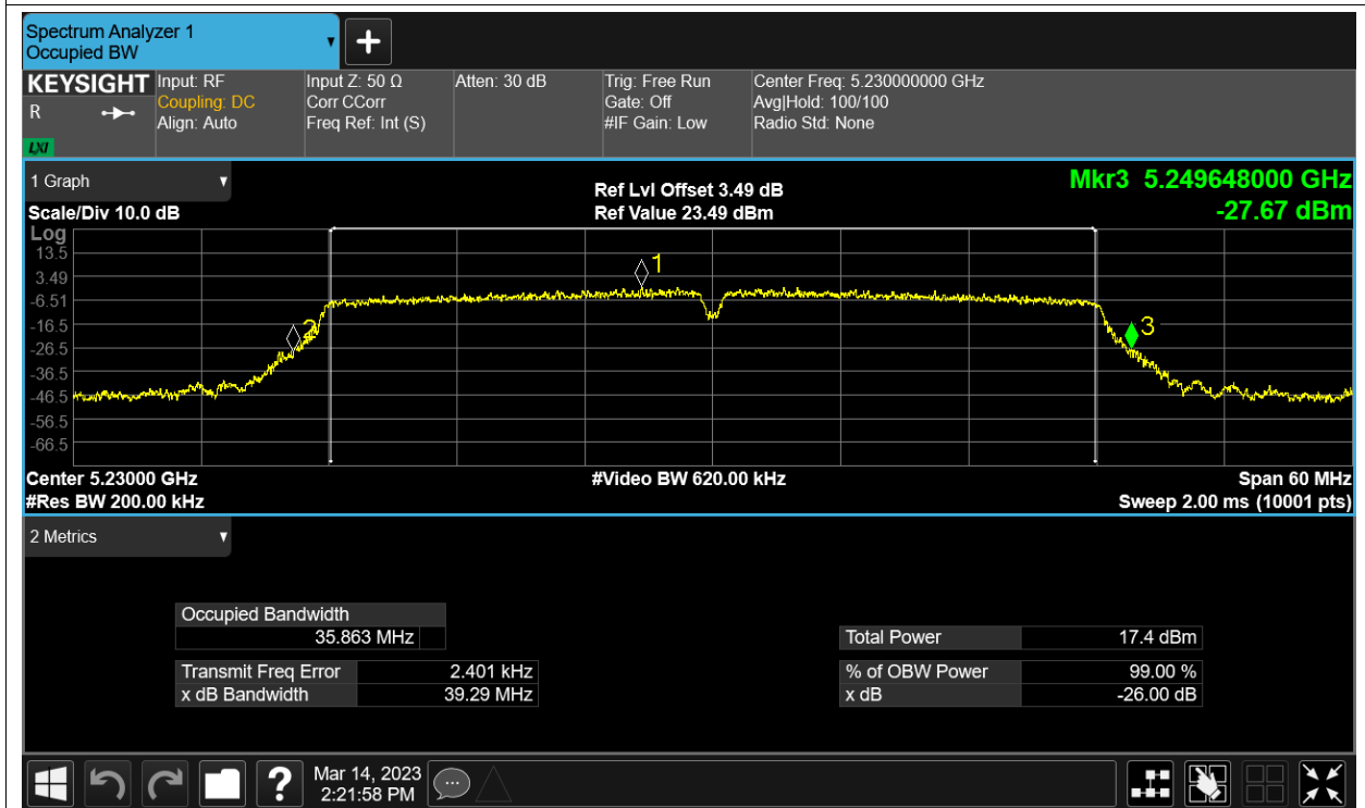
-26dB Bandwidth NVNT ac80 5210MHz Ant6
