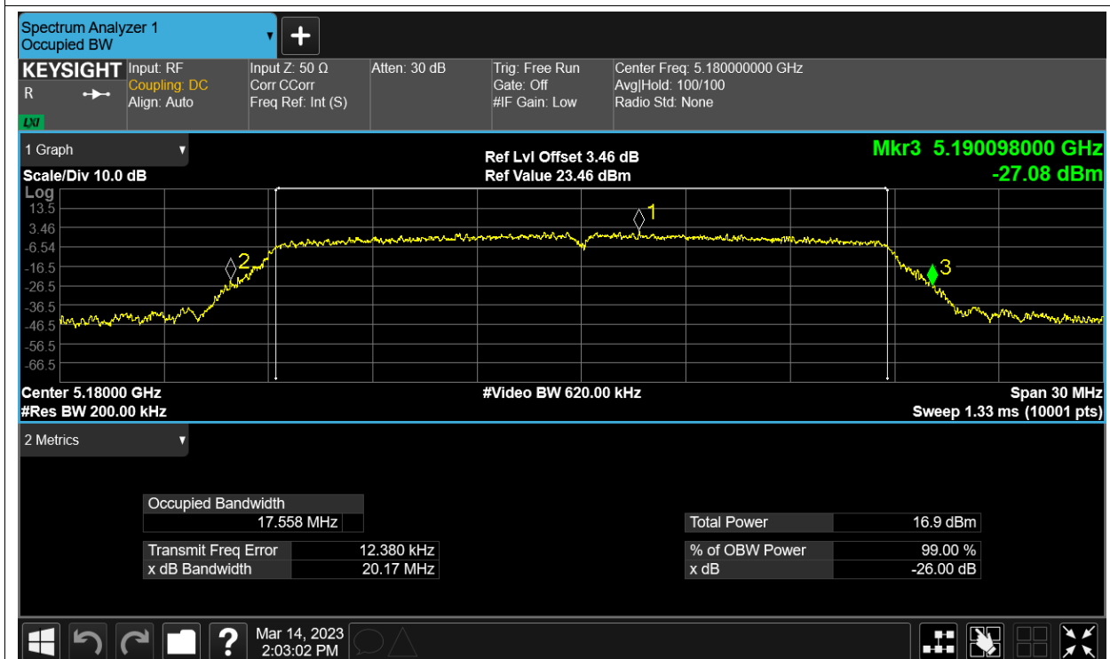
-26dB Bandwidth NVNT ac20 5200MHz Ant6
