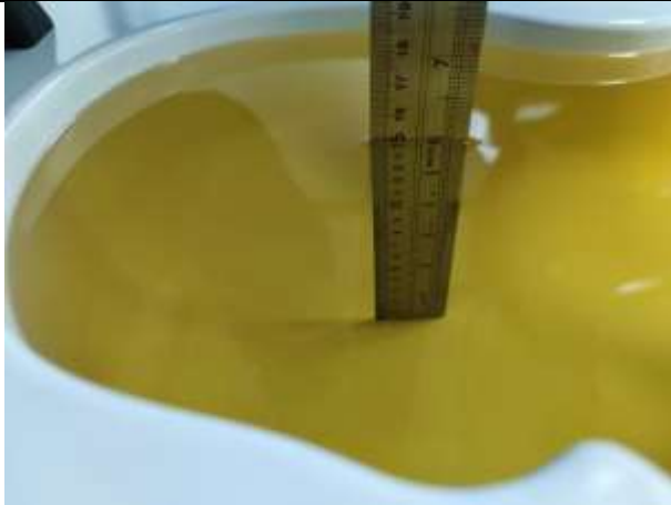
Fig. 9.1 Photo of Liquid Height for Head SAR (depth>15cm)
