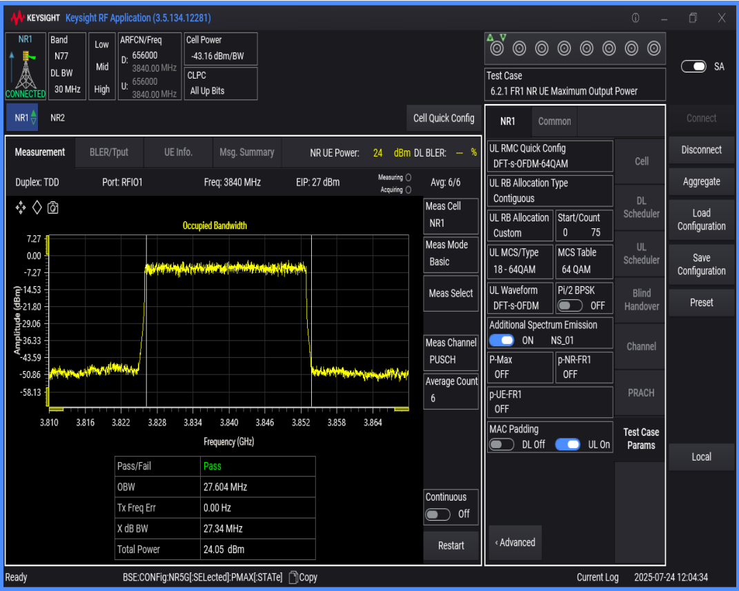
n77(3700-3980) SCS=30kHz DFT_QAM64 BW=40MHz Channel=656000 RB=100@0
