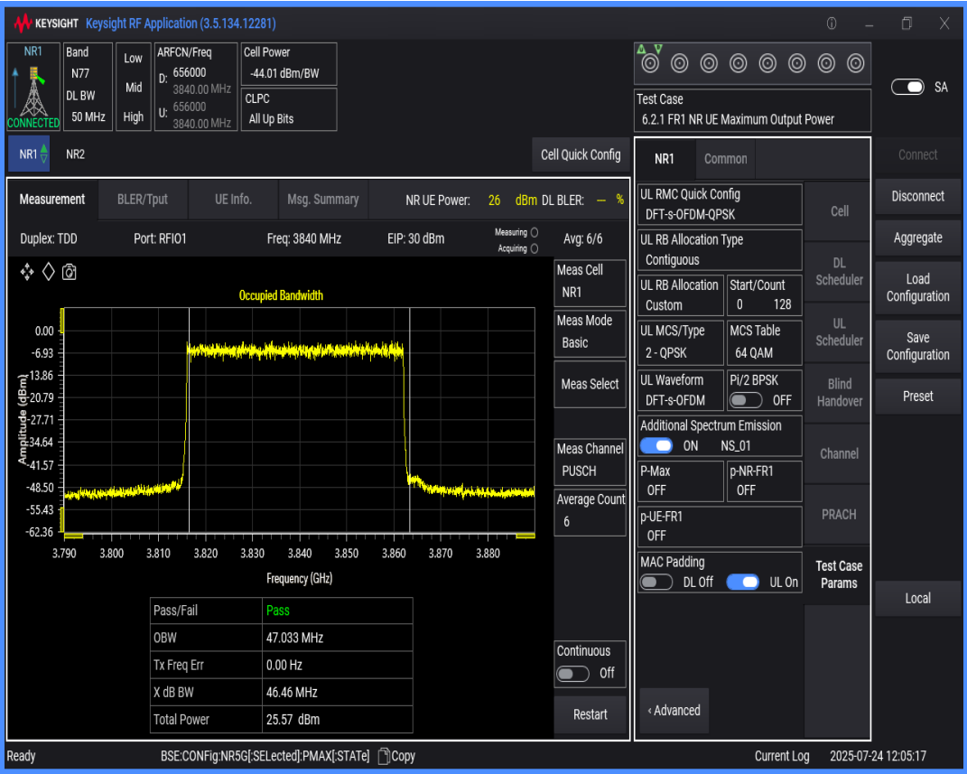
n77(3700-3980) SCS=30kHz DFT_QPSK BW=90MHz Channel=656000 RB=240@0
