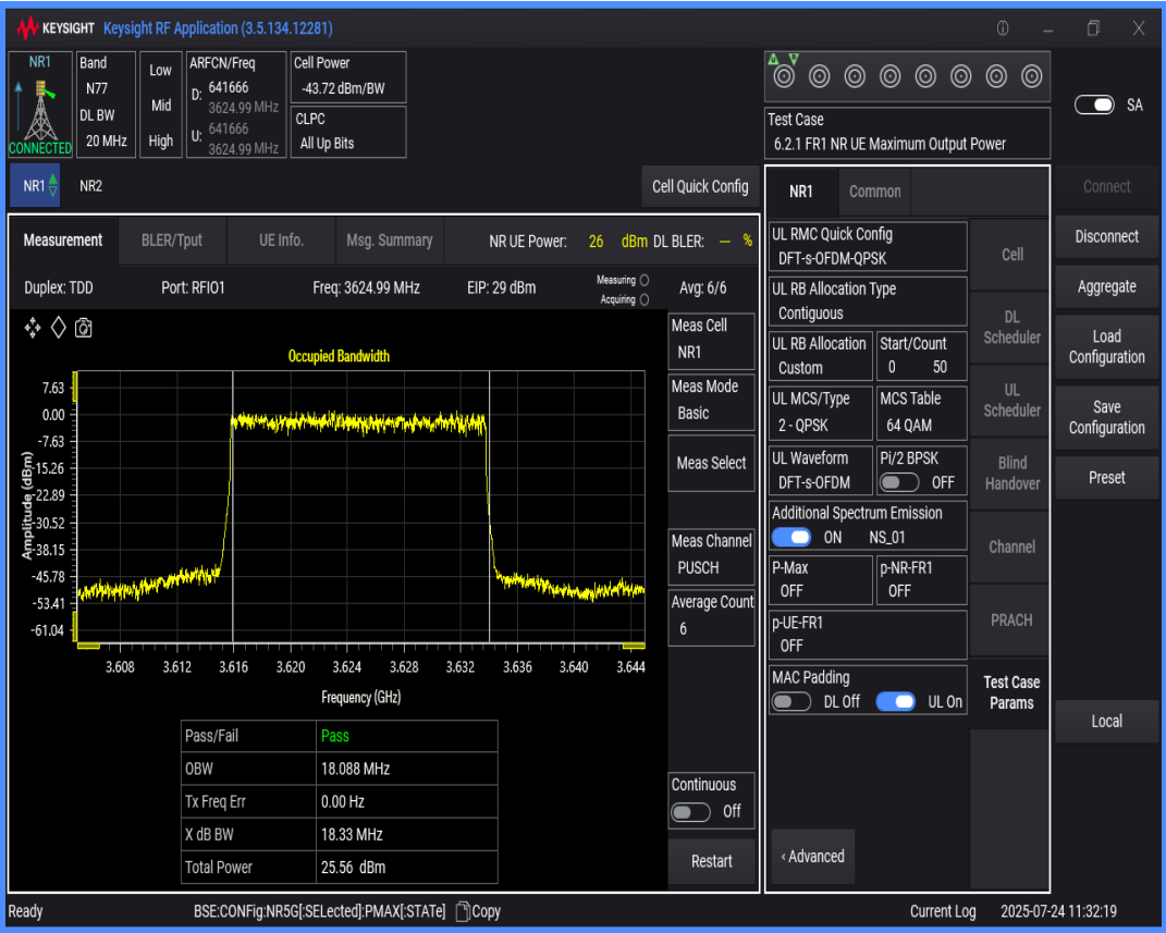
n77(3550-3700) SCS=30kHz DFT_QPSK BW=10MHz Channel=641666 RB=24@0
