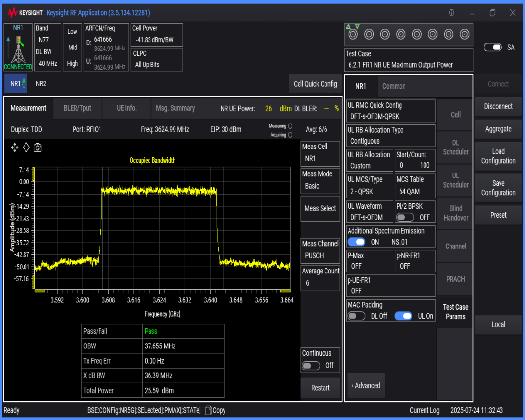
n77(3550-3700) SCS=30kHz DFT_QPSK BW=50MHz Channel=641666 RB=128@0
