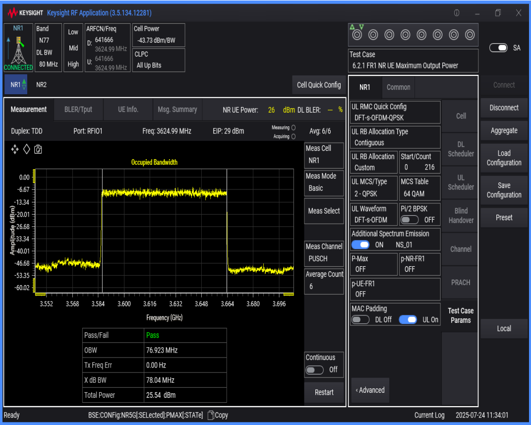
n77(3550-3700) SCS=30kHz DFT_QPSK BW=60MHz Channel=641666 RB=162@0
