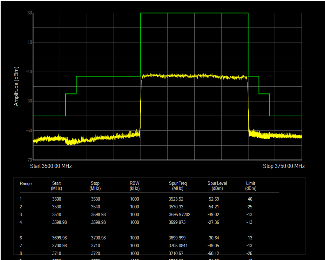
n77(3550-3700) SCS=30kHz CP_QPSK BW=10MHz Channel=637000 RB=24@0
