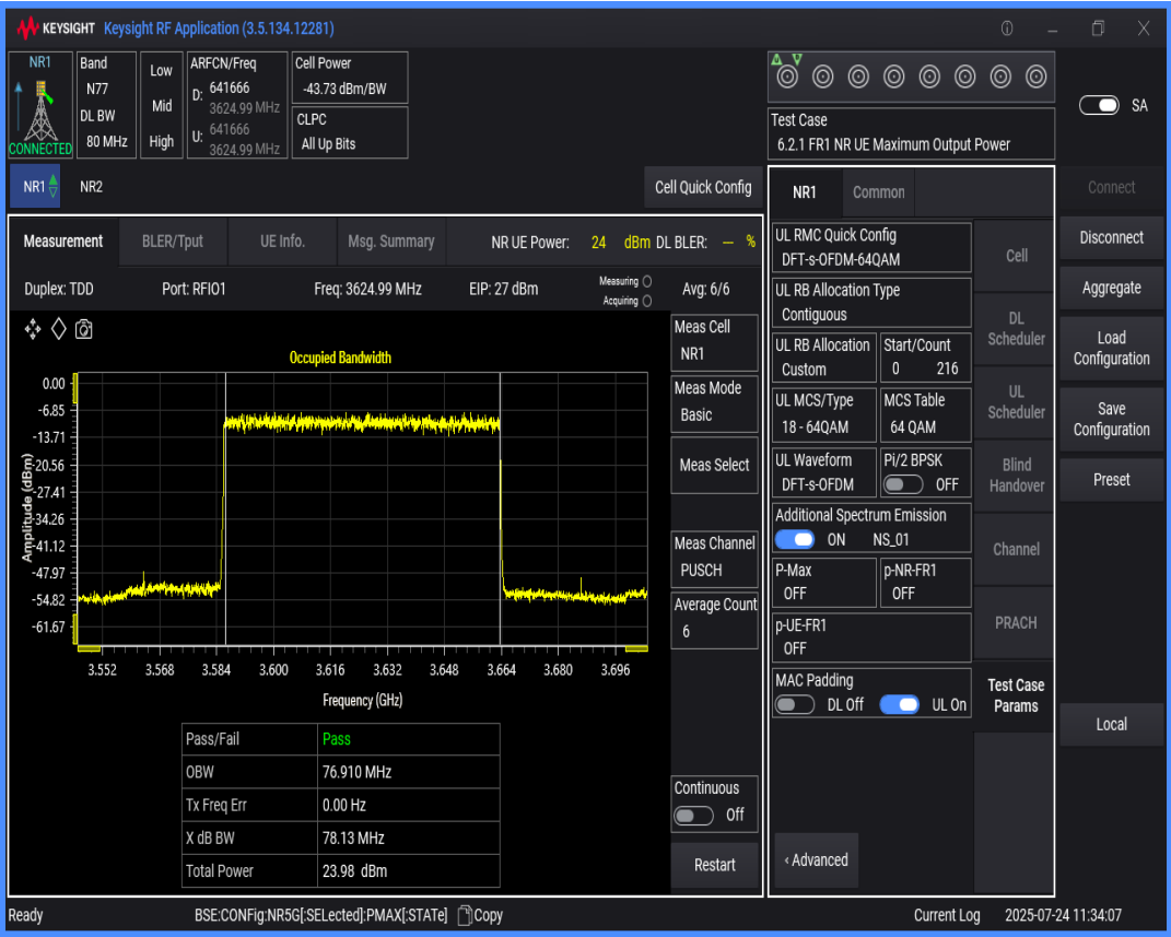
n77(3550-3700) SCS=30kHz DFT_QAM64 BW=60MHz Channel=641666 RB=162@0
