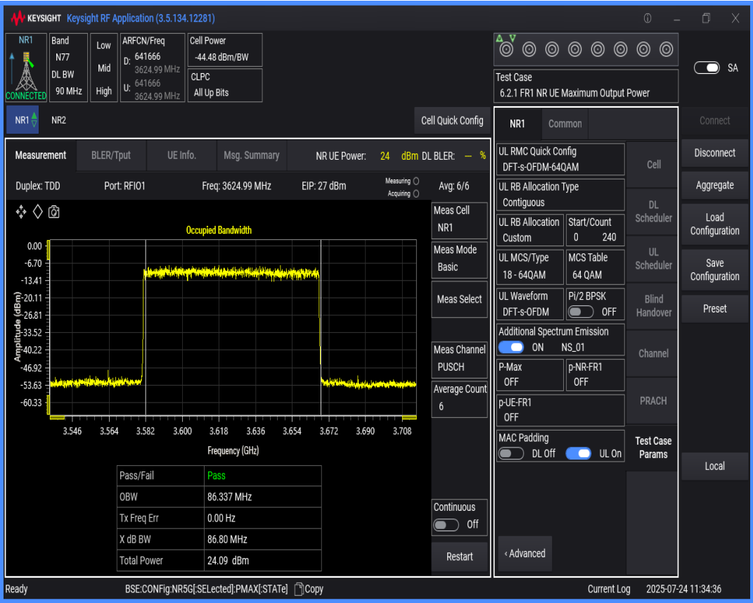
n77(3550-3700) SCS=30kHz DFT_QPSK BW=100MHz Channel=641666 RB=270@0
