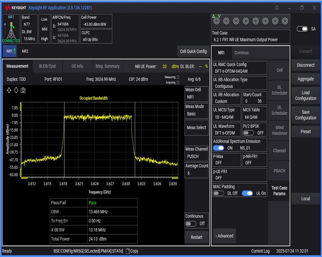
n77(3550-3700) SCS=30kHz DFT_QAM64 BW=40MHz Channel=641666 RB=100@0
