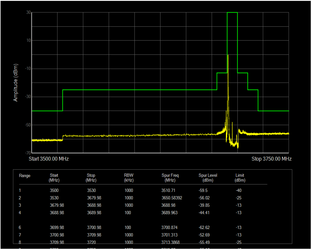
n77(3550-3700) SCS=30kHz CP_QPSK BW=50MHz Channel=638334 RB=133@0
