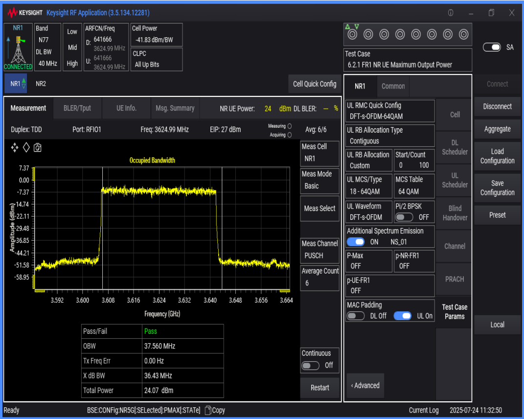
n77(3550-3700) SCS=30kHz DFT_QAM64 BW=80MHz Channel=641666 RB=216@0
