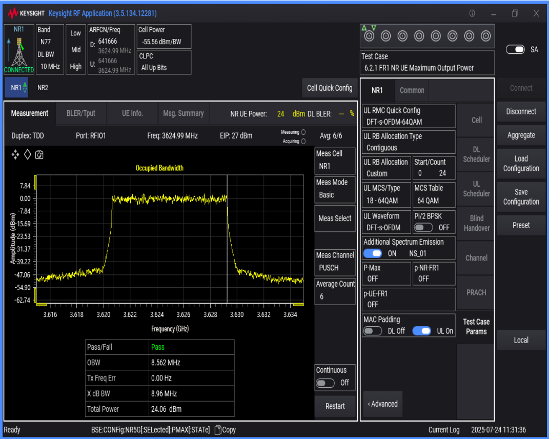
n77(3550-3700) SCS=30kHz DFT_QAM64 BW=100MHz Channel=641666 RB=270@0
