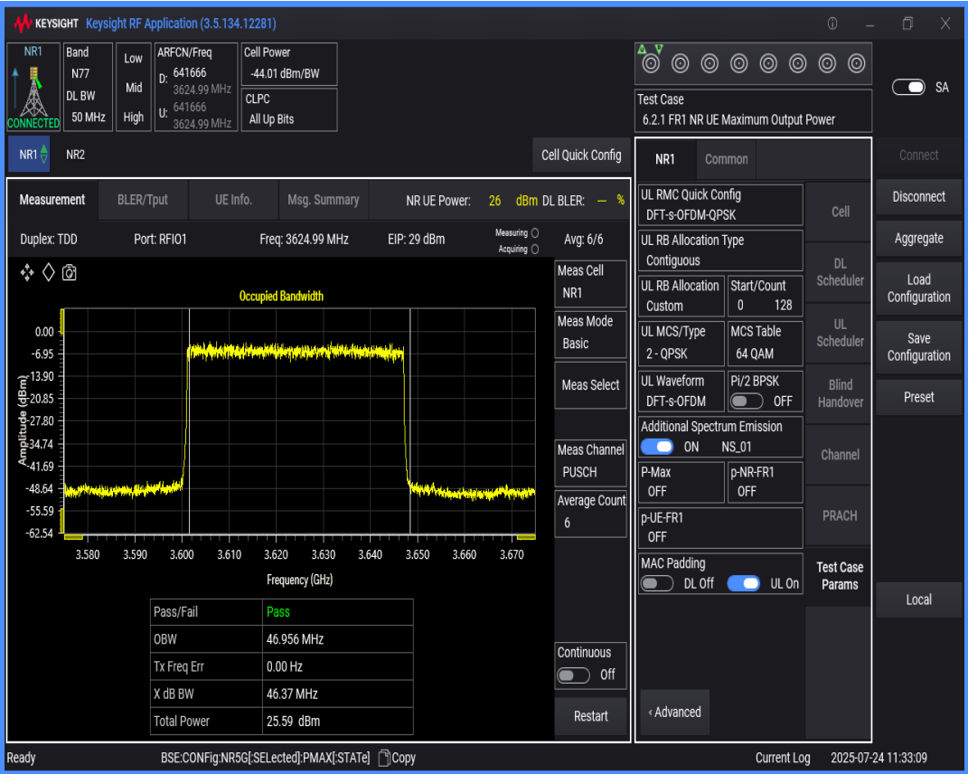
n77(3550-3700) SCS=30kHz DFT_QPSK BW=80MHz Channel=641666 RB=216@0
