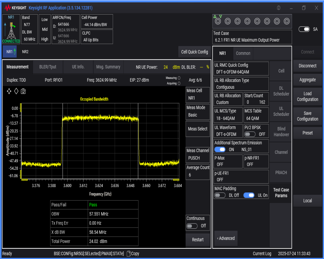
n77(3550-3700) SCS=30kHz DFT_QAM64 BW=50MHz Channel=641666 RB=128@0
