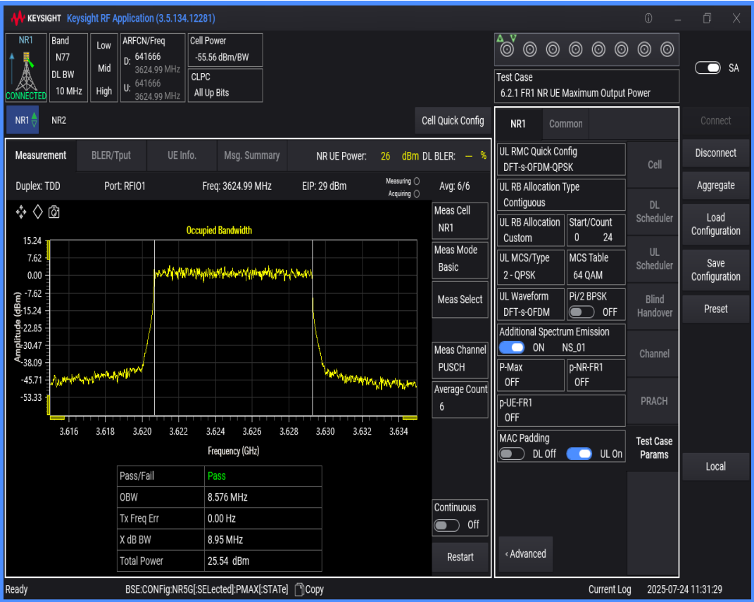
n77(3550-3700) SCS=30kHz DFT_QAM64 BW=90MHz Channel=641666 RB=240@0
