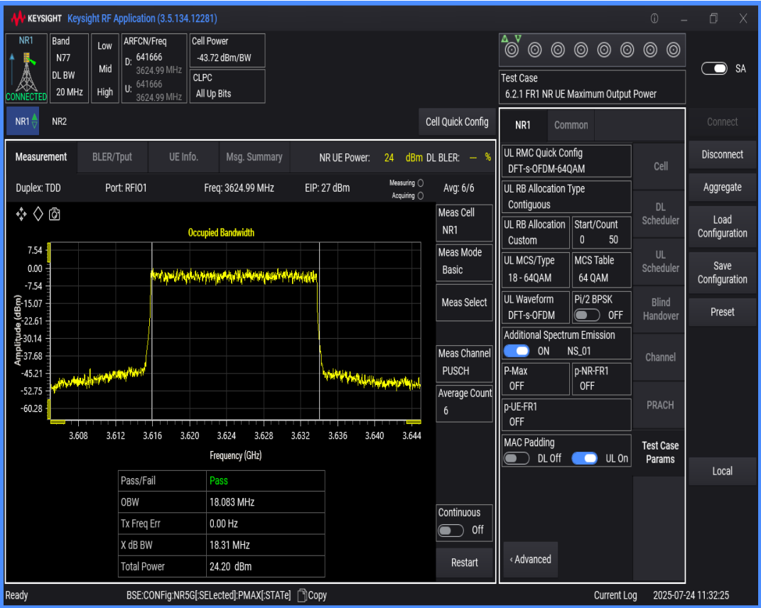
n77(3550-3700) SCS=30kHz DFT_QAM64 BW=15MHz Channel=641666 RB=36@0
