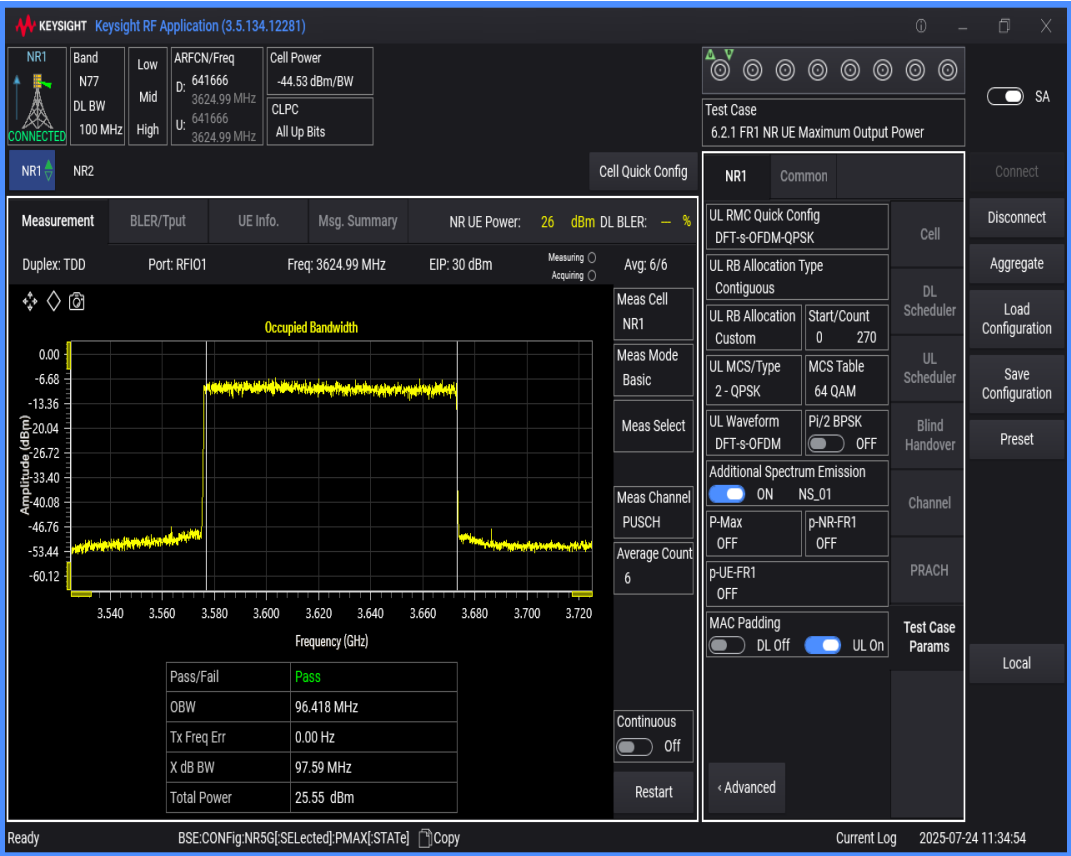
n77(3550-3700) SCS=30kHz DFT_QPSK BW=40MHz Channel=641666 RB=100@0
