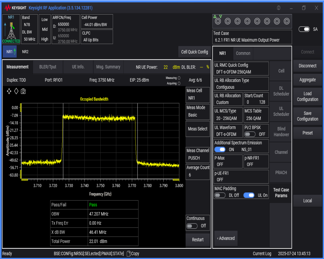
n78(3700-3800) SCS=30kHz DFT_QAM256 BW=60MHz Channel=650000 RB=162@0
