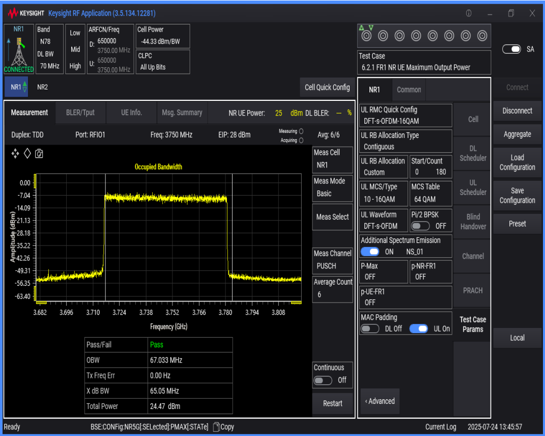
n78(3700-3800) SCS=30kHz DFT_QAM16 BW=90MHz Channel=650000 RB=240@0
