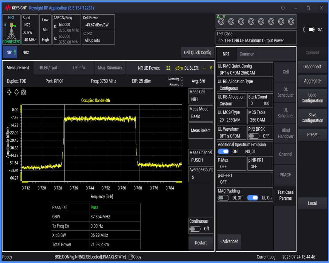
n78(3700-3800) SCS=30kHz DFT_QAM256 BW=30MHz Channel=650000 RB=75@0
