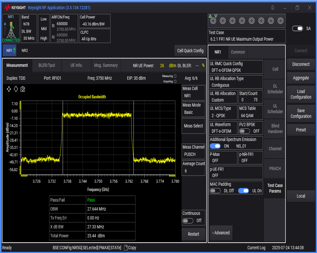
n78(3700-3800) SCS=30kHz DFT_QPSK BW=40MHz Channel=650000 RB=100@0
