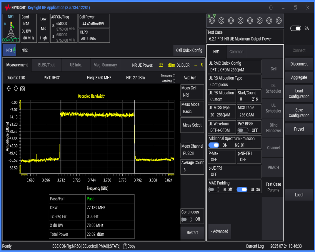
n78(3700-3800) SCS=30kHz DFT_QAM256 BW=90MHz Channel=650000 RB=240@0
