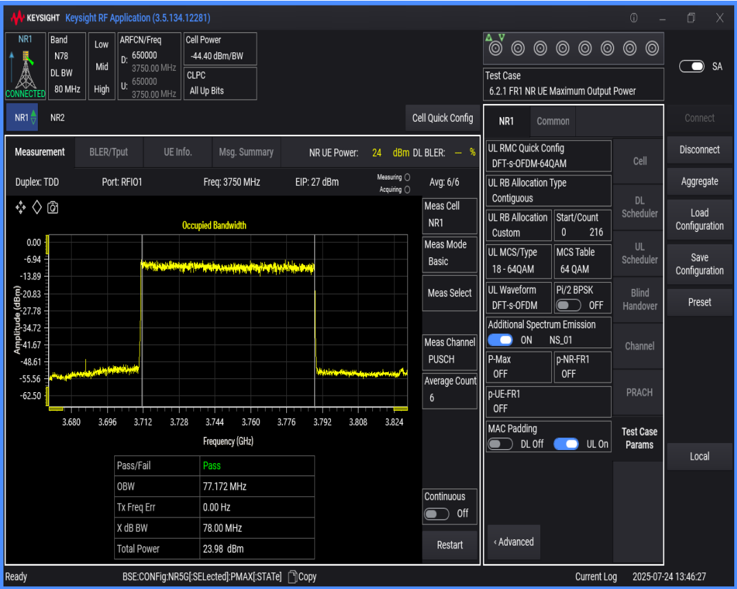
n78(3700-3800) SCS=30kHz DFT_QAM64 BW=60MHz Channel=650000 RB=162@0
