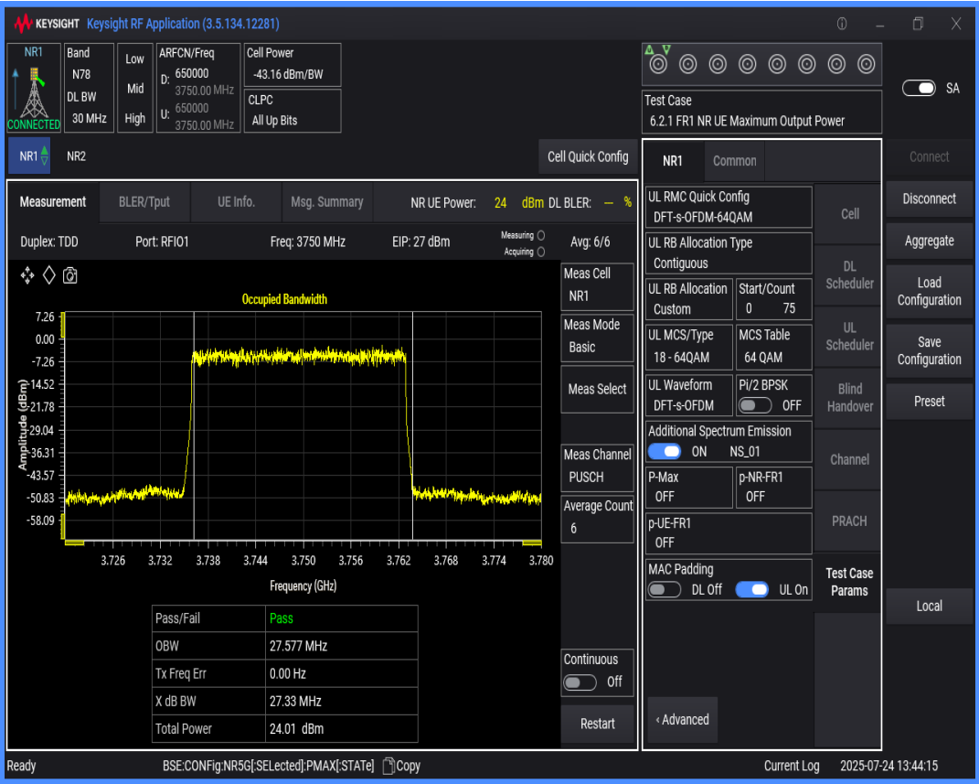
n78(3700-3800) SCS=30kHz DFT_QAM64 BW=15MHz Channel=650000 RB=36@0
