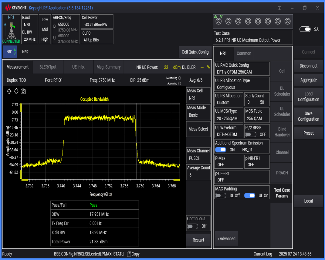
n78(3700-3800) SCS=30kHz DFT_QAM256 BW=15MHz Channel=650000 RB=36@0
