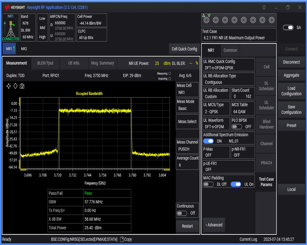
n78(3700-3800) SCS=30kHz DFT_QPSK BW=70MHz Channel=650000 RB=180@0
