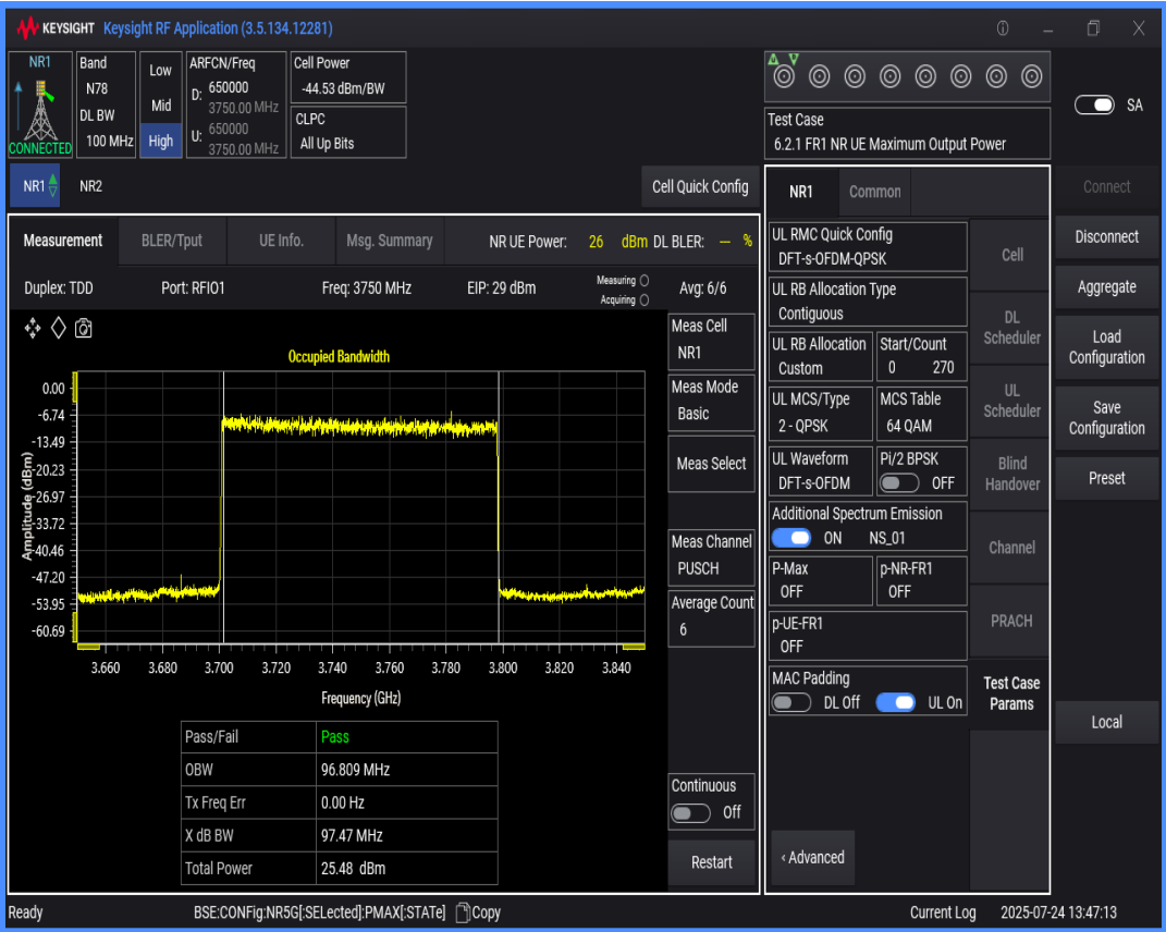
n78(3700-3800) SCS=30kHz DFT_QPSK BW=60MHz Channel=650000 RB=162@0
