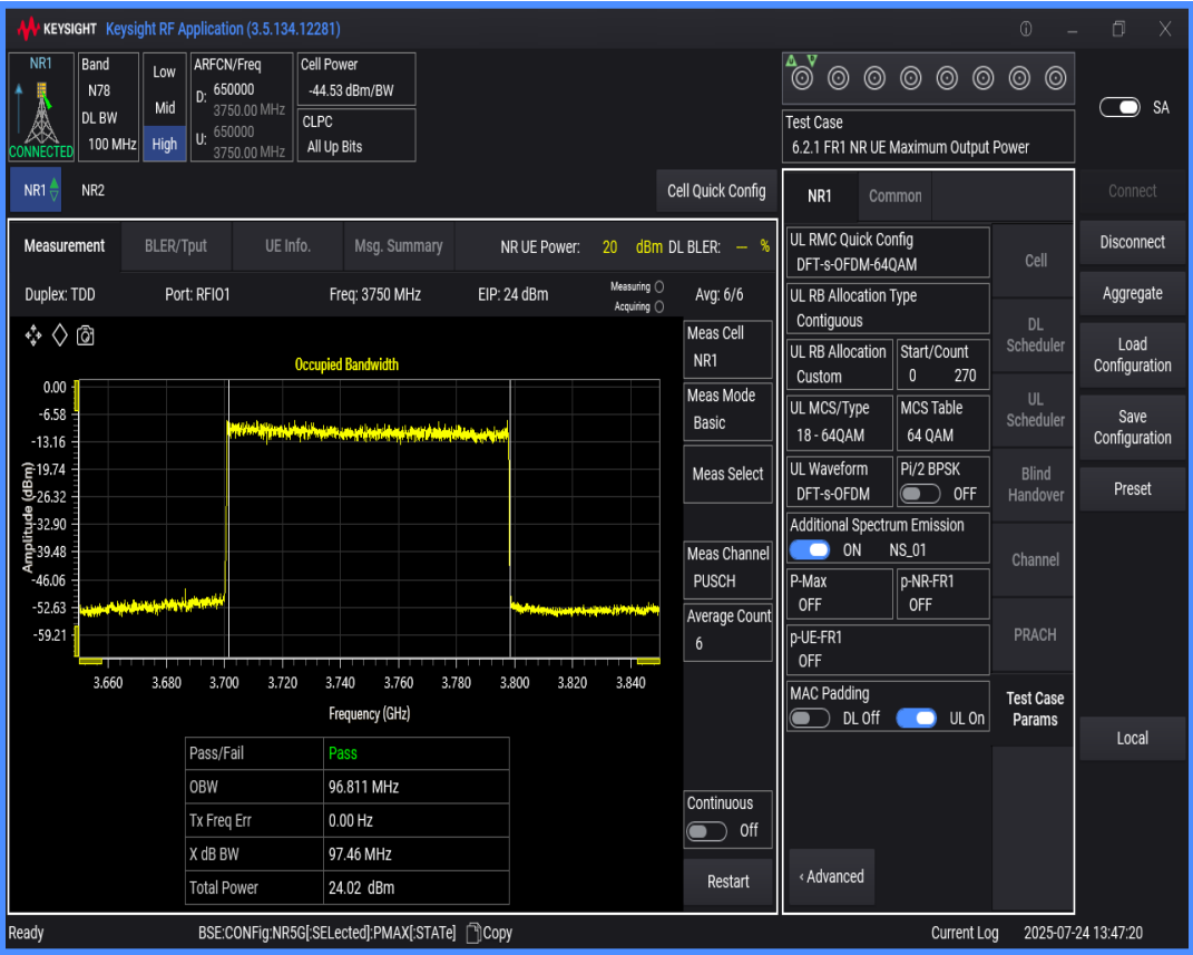
n78(3700-3800) SCS=30kHz DFT_QAM64 BW=10MHz Channel=650000 RB=24@0
