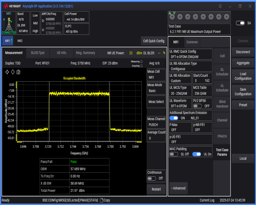
n78(3700-3800) SCS=30kHz DFT_QAM64 BW=20MHz Channel=650000 RB=50@0
