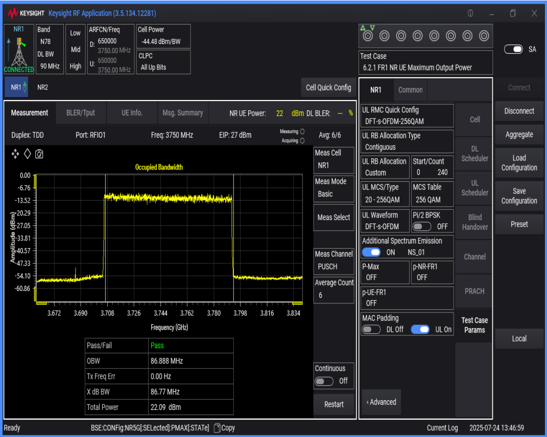
n78(3700-3800) SCS=30kHz DFT_QAM256 BW=70MHz Channel=650000 RB=180@0
