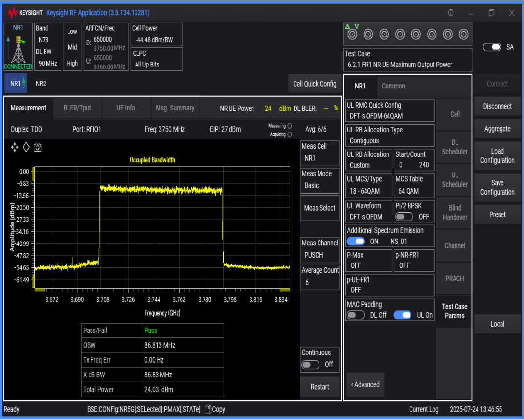
n78(3700-3800) SCS=30kHz DFT_QPSK BW=100MHz Channel=650000 RB=270@0
