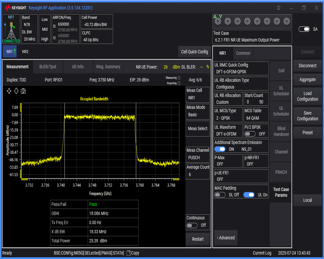
n78(3700-3800) SCS=30kHz DFT_QPSK BW=10MHz Channel=650000 RB=24@0
