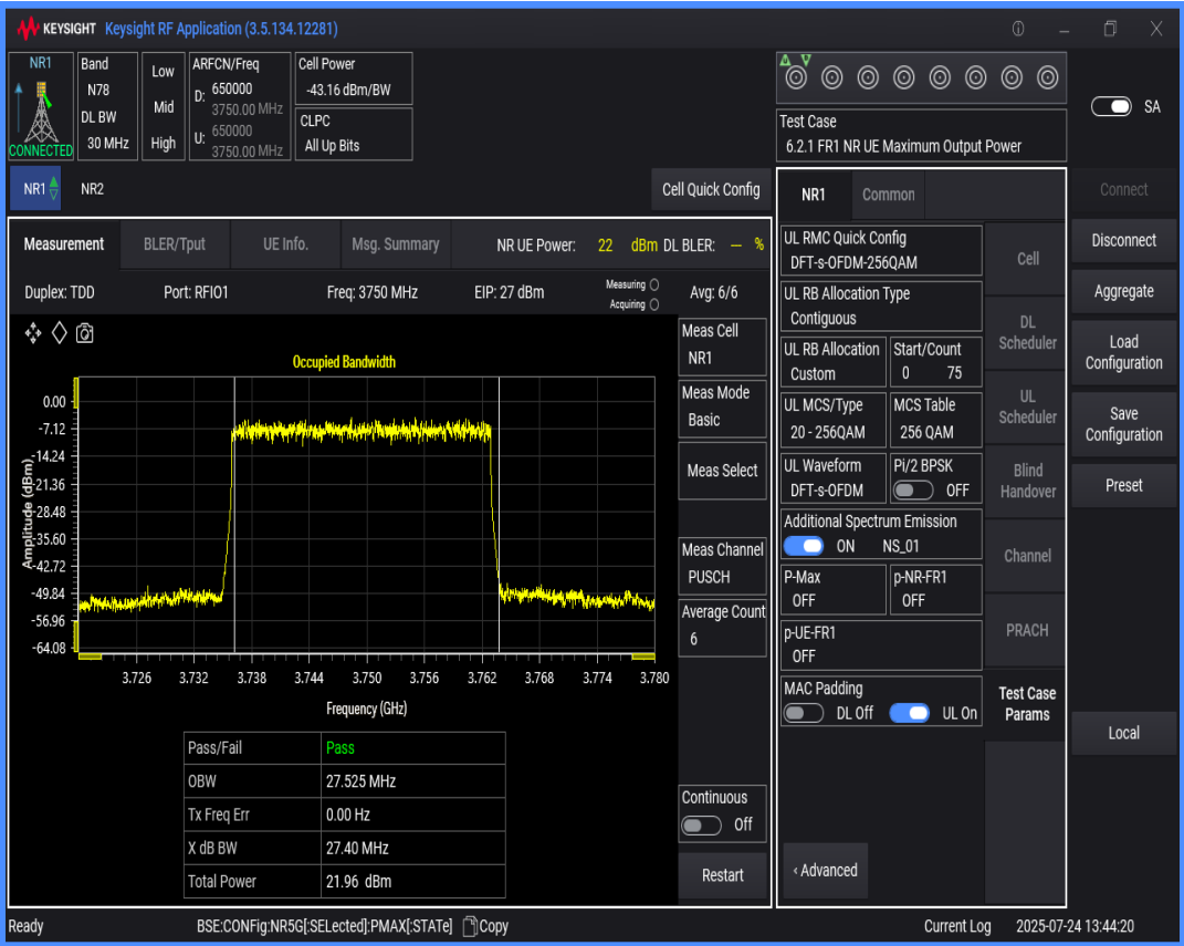
n78(3700-3800) SCS=30kHz DFT_QAM256 BW=80MHz Channel=650000 RB=216@0
