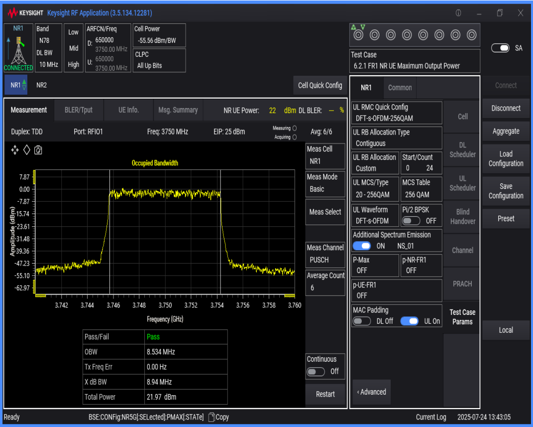
n78(3700-3800) SCS=30kHz DFT_QAM256 BW=100MHz Channel=650000 RB=270@0
