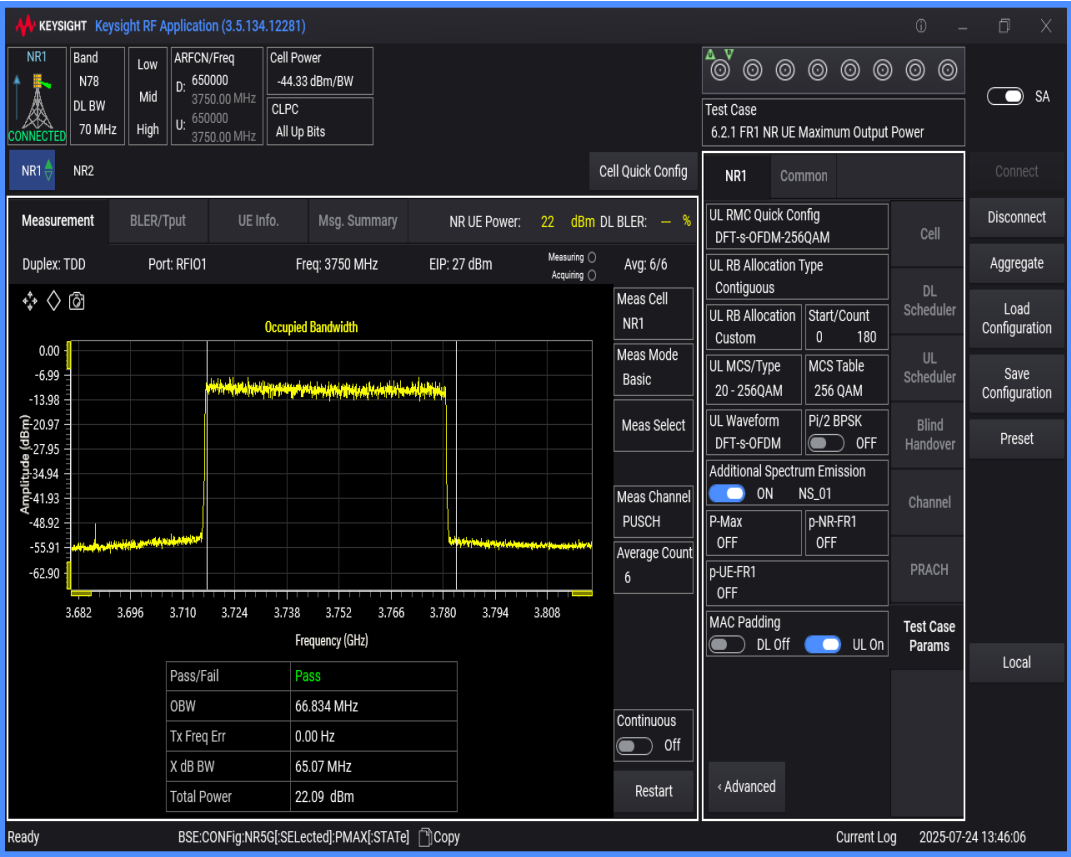
n78(3700-3800) SCS=30kHz DFT_QAM256 BW=50MHz Channel=650000 RB=128@0
