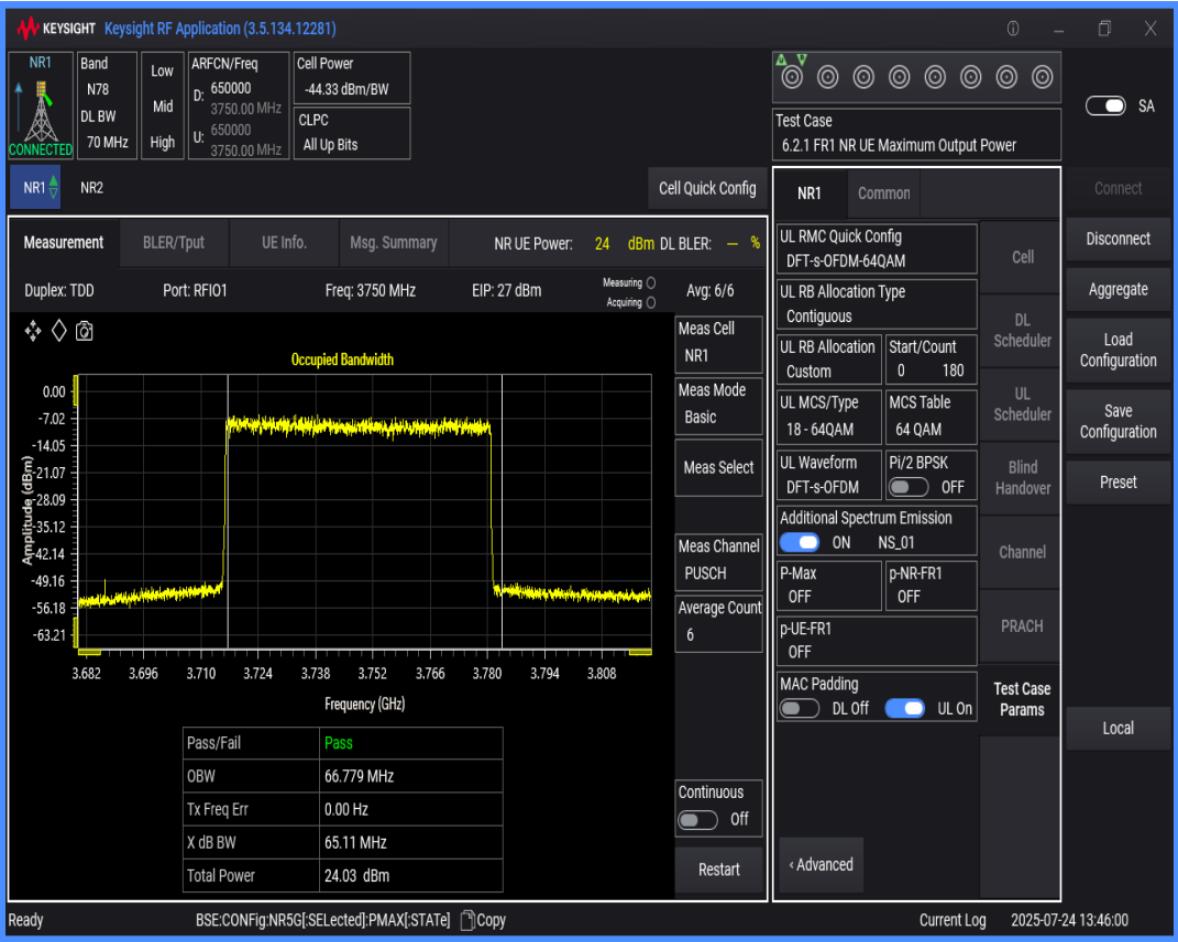
n78(3700-3800) SCS=30kHz DFT_QAM64 BW=80MHz Channel=650000 RB=216@0
