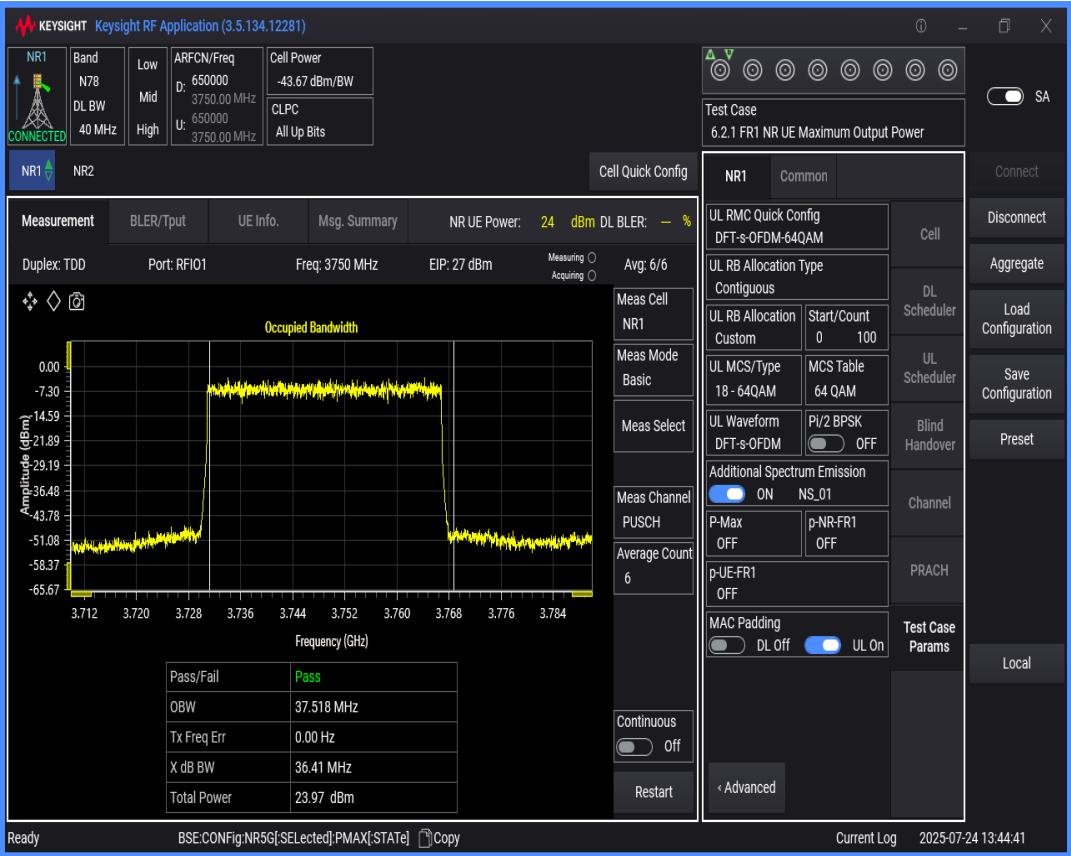
n78(3700-3800) SCS=30kHz DFT_QAM64 BW=50MHz Channel=650000 RB=128@0
