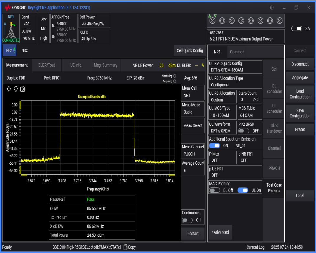
n78(3700-3800) SCS=30kHz DFT_QAM16 BW=80MHz Channel=650000 RB=216@0
