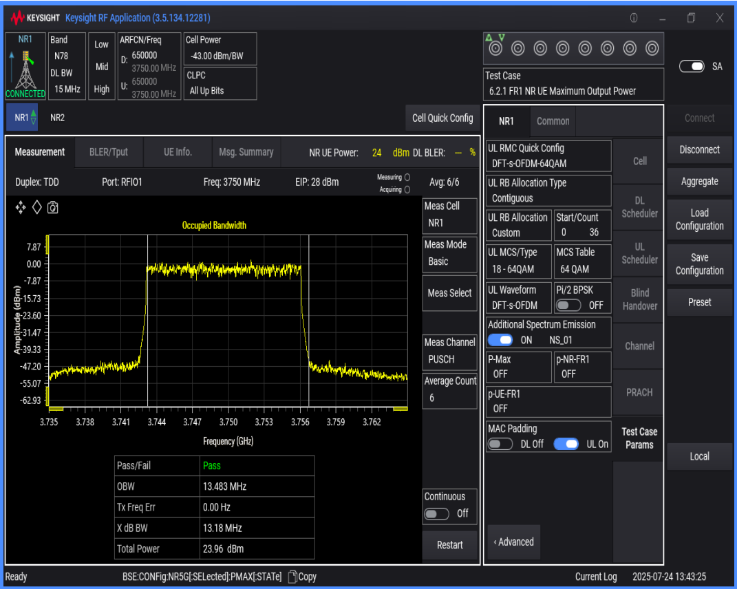
n78(3700-3800) SCS=30kHz DFT_QAM64 BW=100MHz Channel=650000 RB=270@0
