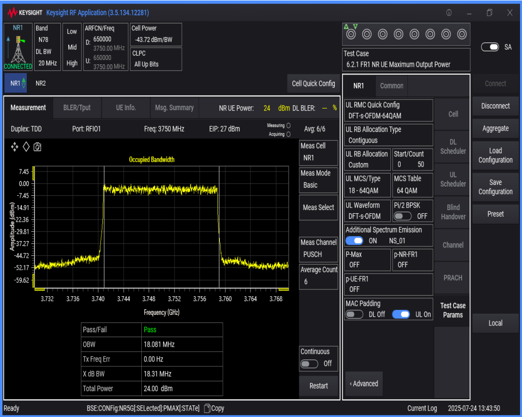
n78(3700-3800) SCS=30kHz DFT_QAM64 BW=30MHz Channel=650000 RB=75@0
