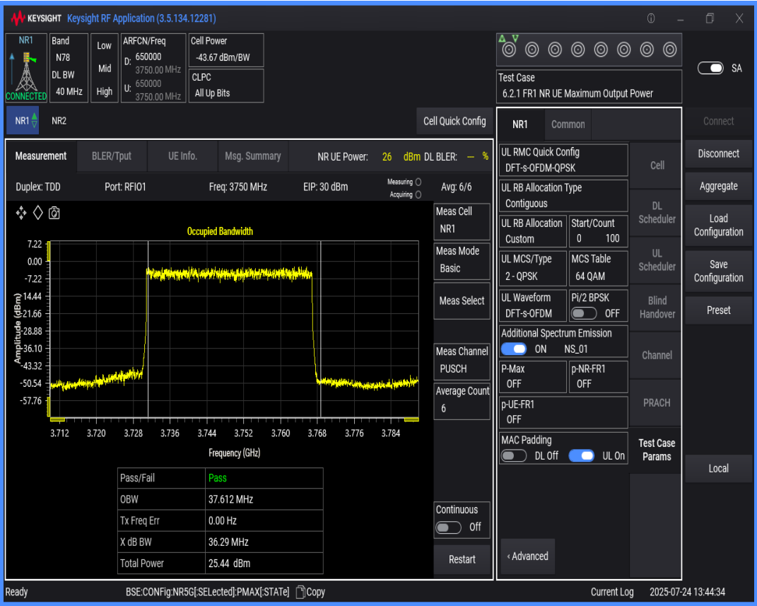
n78(3700-3800) SCS=30kHz DFT_QPSK BW=50MHz Channel=650000 RB=128@0
