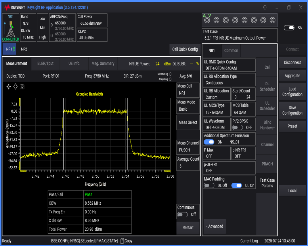
n78(3700-3800) SCS=30kHz DFT_QAM64 BW=70MHz Channel=650000 RB=180@0
