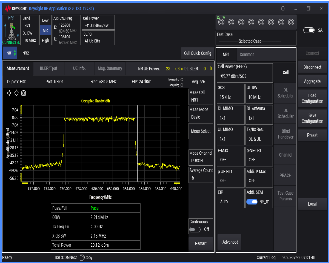
n71 SCS=15kHz DFT_QAM16 BW=20MHz Channel=136100 RB=100@0
