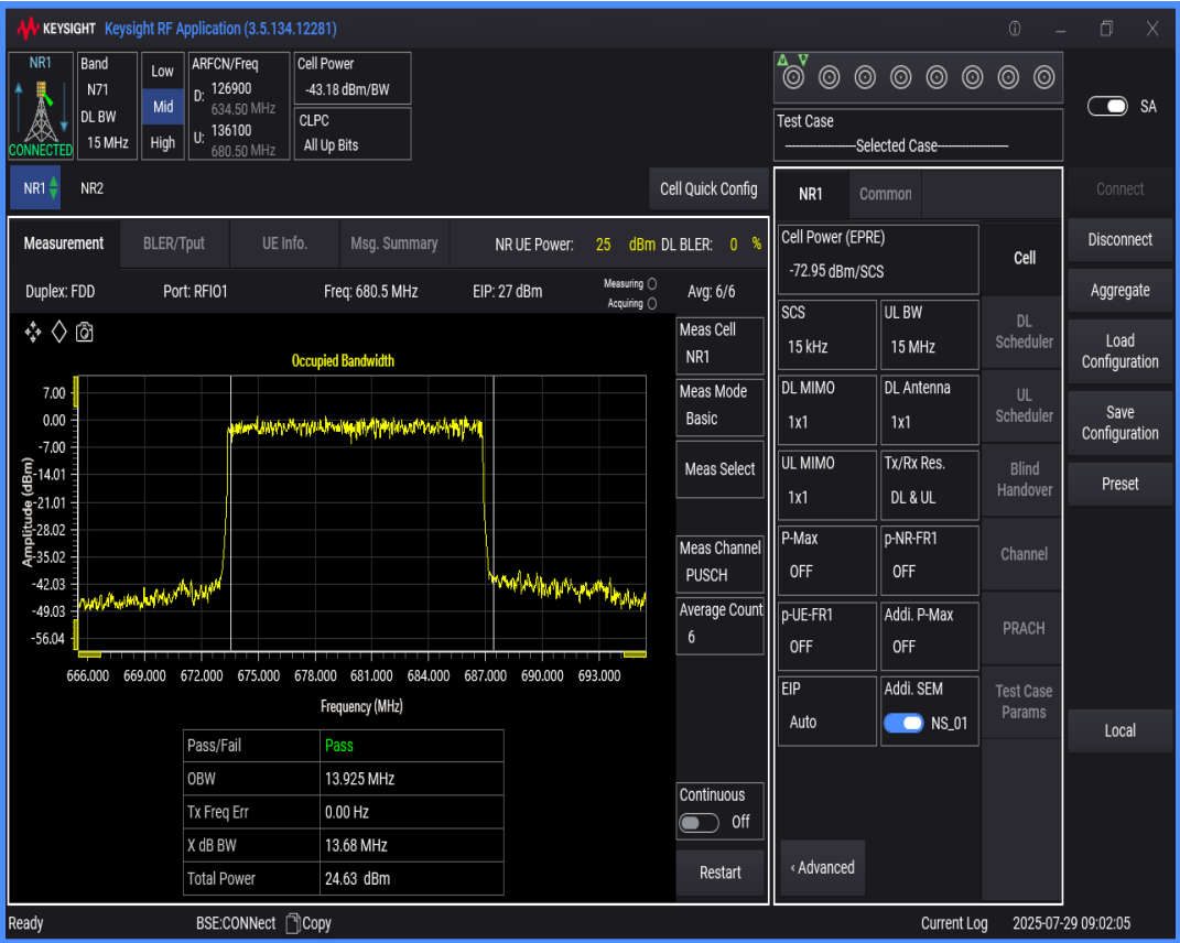
n71 SCS=15kHz DFT_BPSK BW=5MHz Channel=136100 RB=25@0
