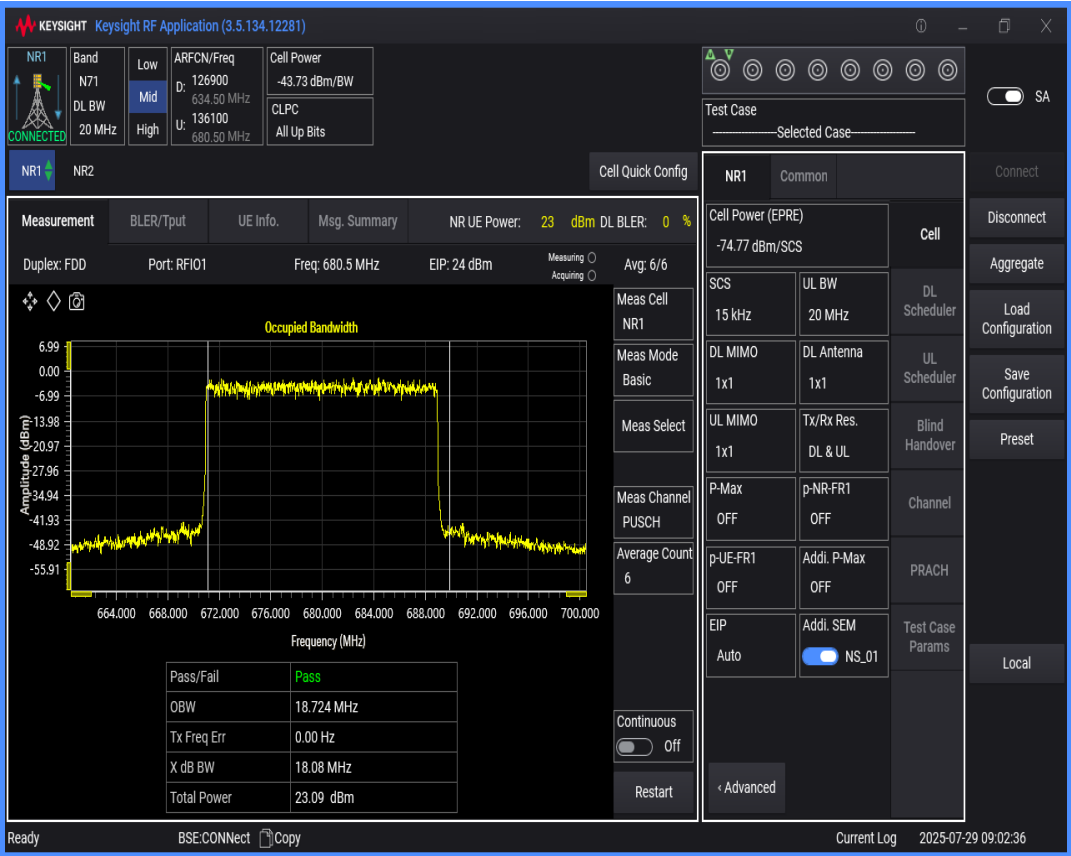
n71 SCS=15kHz DFT_QAM256 BW=20MHz Channel=136100 RB=100@0
