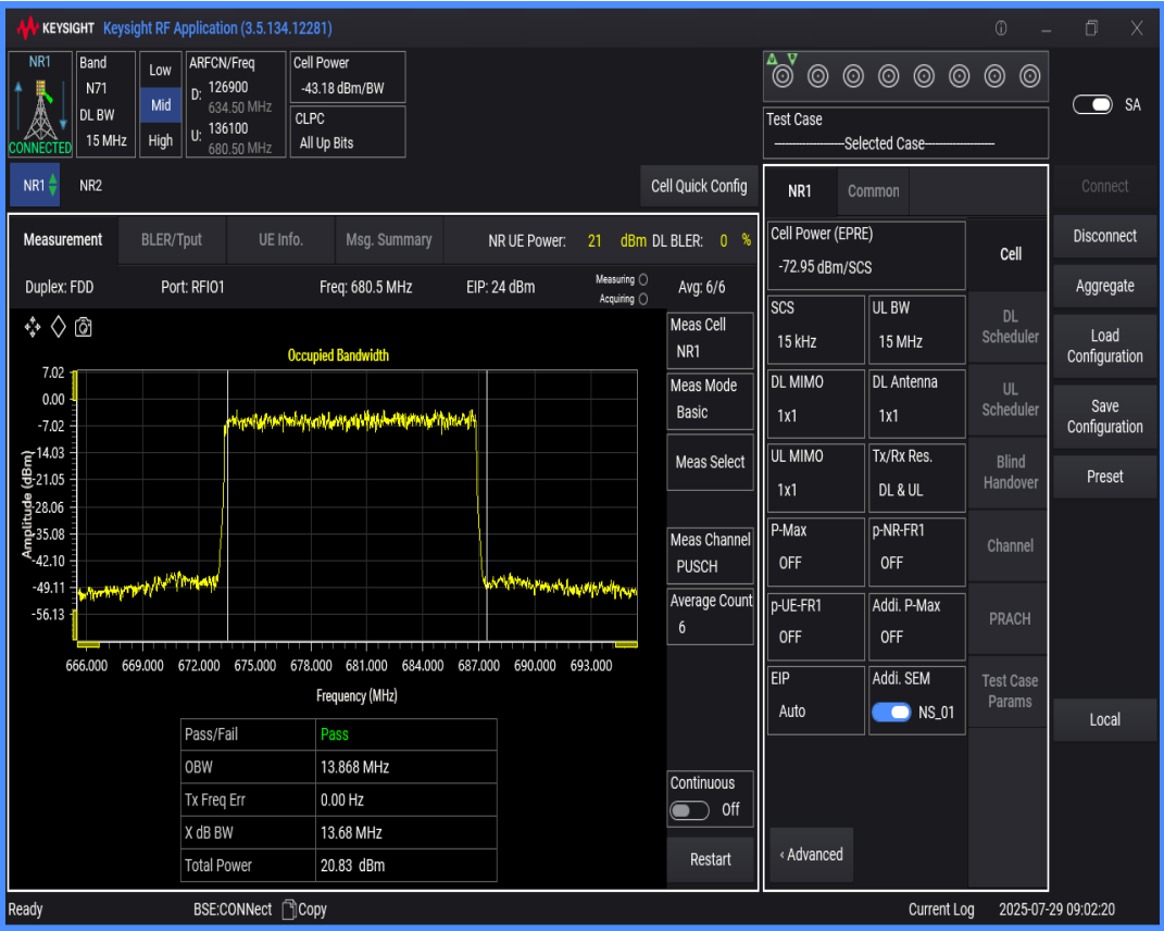
n71 SCS=15kHz DFT_QAM16 BW=5MHz Channel=136100 RB=25@0
