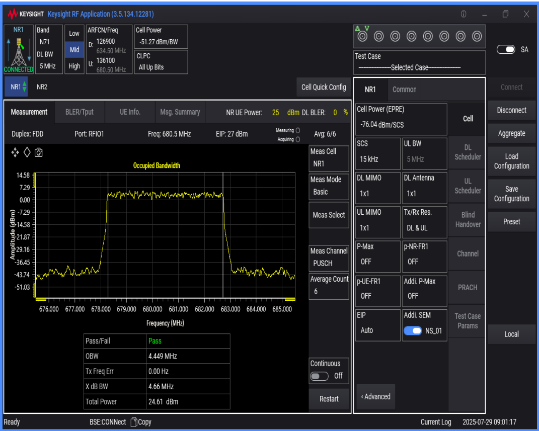
n71 SCS=15kHz DFT_QAM16 BW=15MHz Channel=136100 RB=75@0
