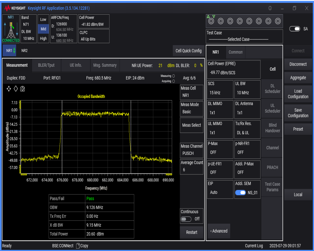
n71 SCS=15kHz DFT_QAM64 BW=20MHz Channel=136100 RB=100@0
