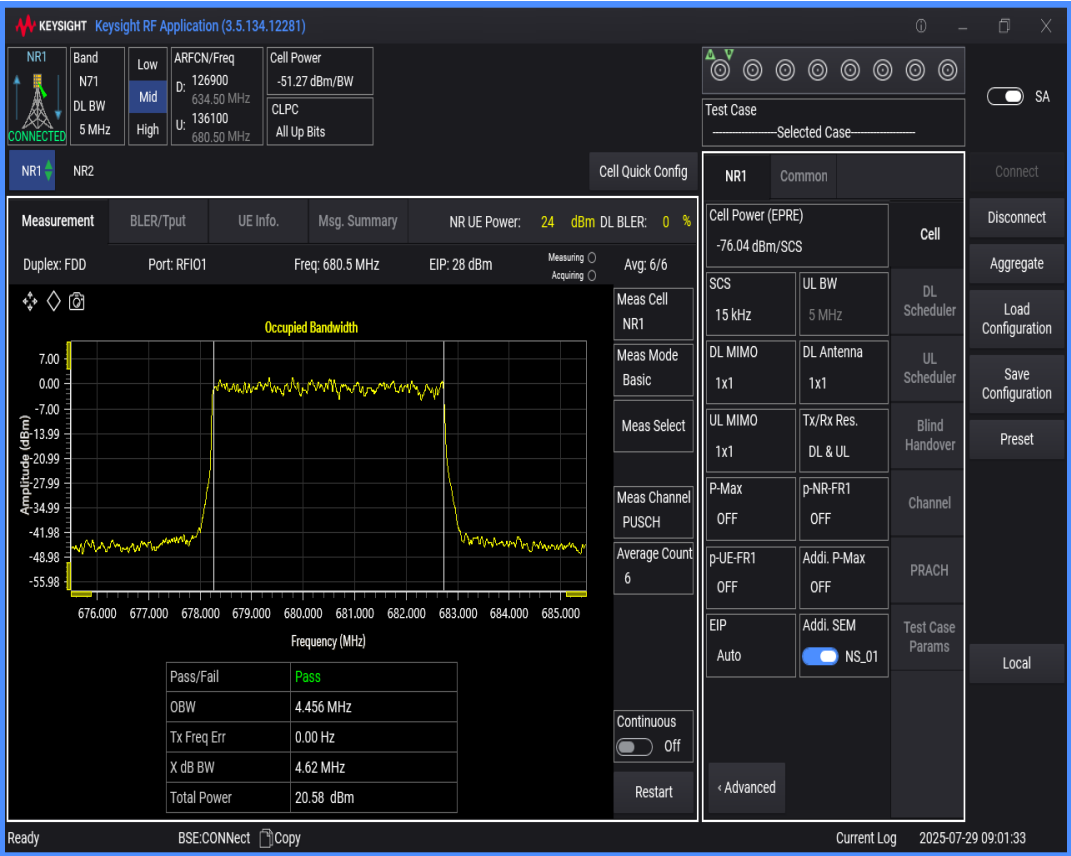
n71 SCS=15kHz DFT_QAM256 BW=15MHz Channel=136100 RB=75@0
