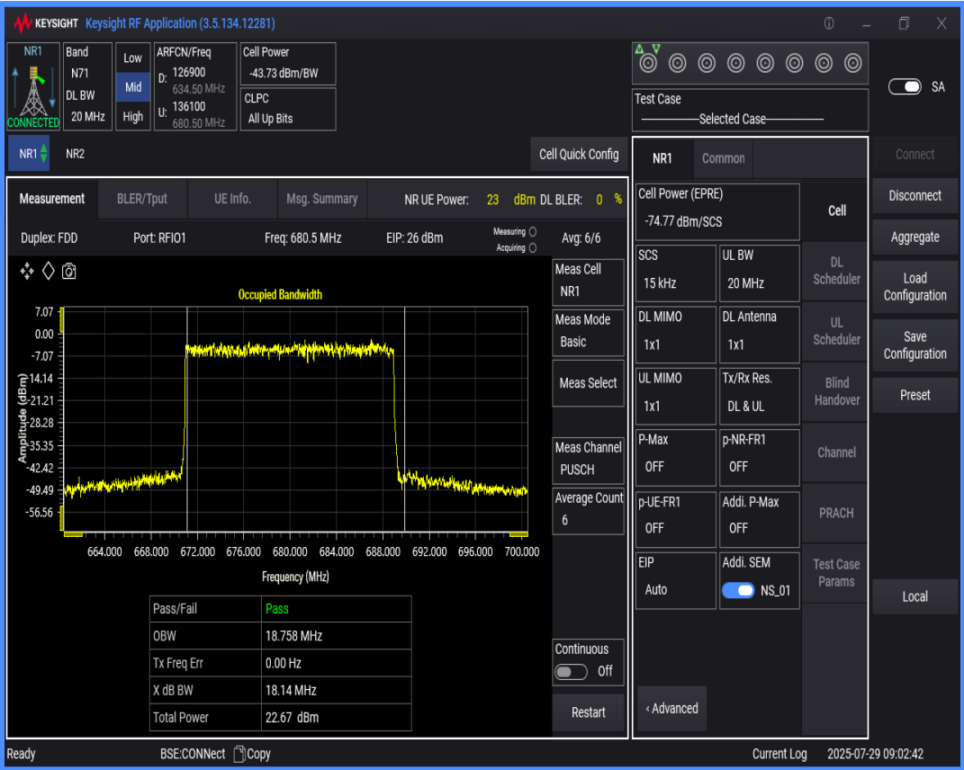
n71 SCS=15kHz DFT_QAM64 BW=15MHz Channel=136100 RB=75@0
