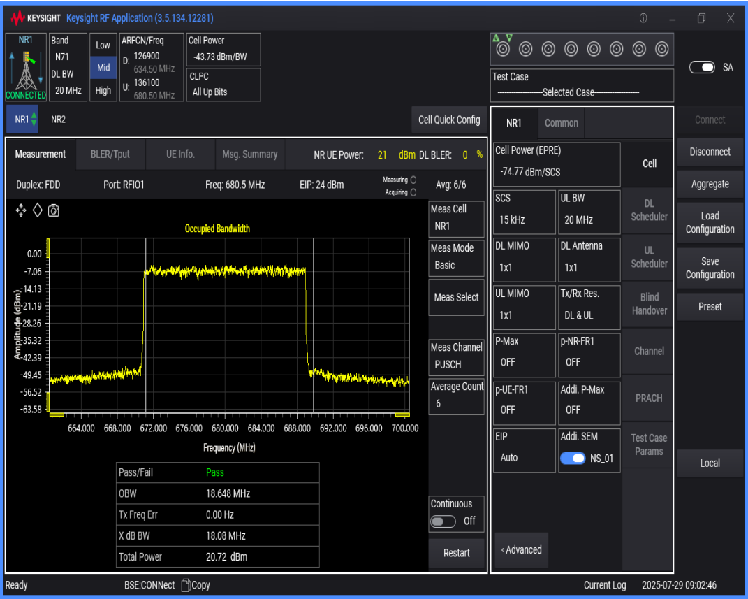
n71 SCS=15kHz DFT_QAM256 BW=5MHz Channel=136100 RB=25@0
