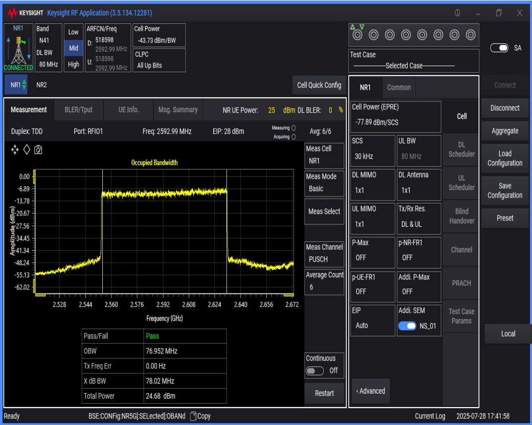
n41 SCS=30kHz DFT_QAM16 BW=100MHz Channel=518598 RB=270@0
