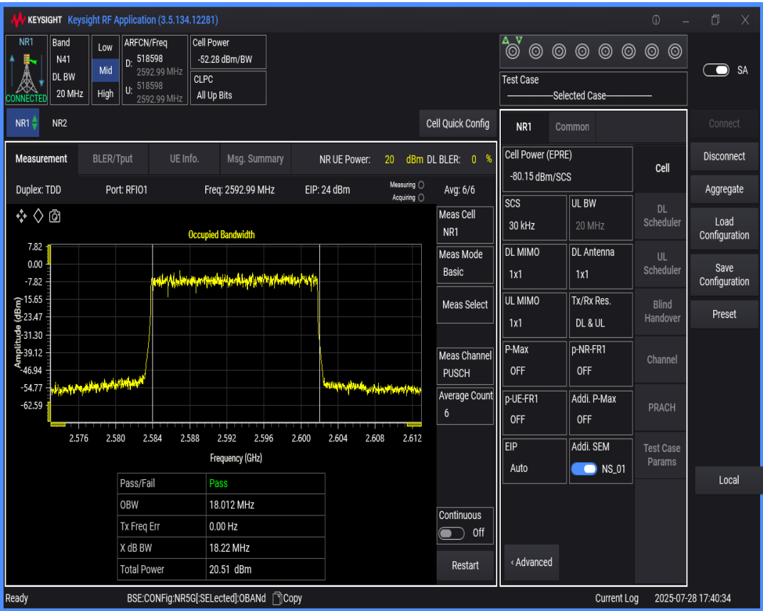
n41 SCS=30kHz DFT_QAM256 BW=80MHz Channel=518598 RB=216@0
