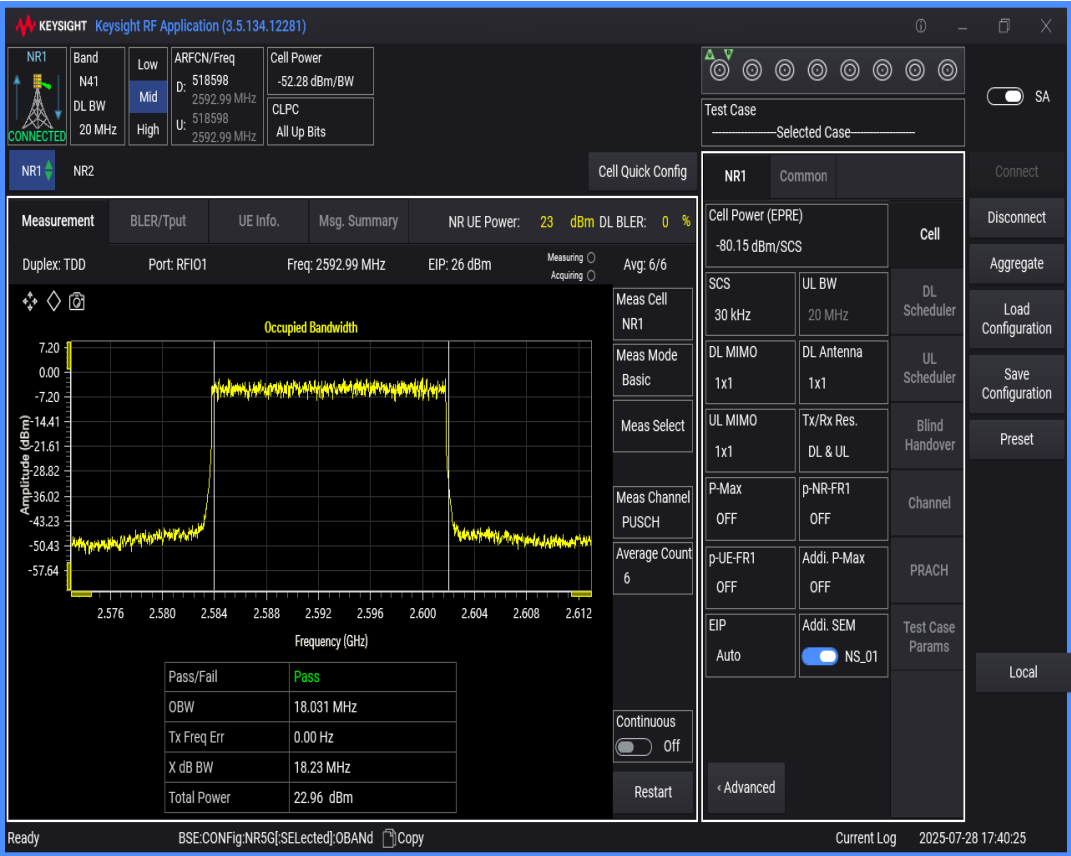
n41 SCS=30kHz DFT_QAM16 BW=40MHz Channel=518598 RB=100@0
