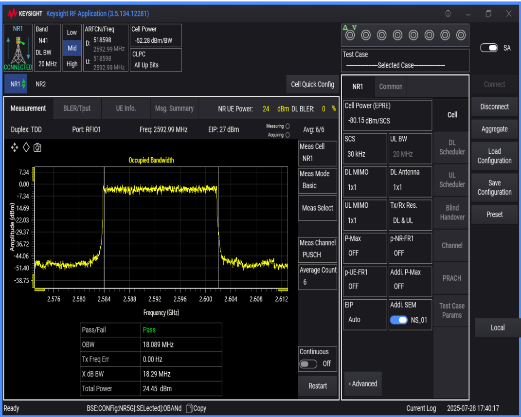
n41 SCS=30kHz DFT_BPSK BW=50MHz Channel=518598 RB=128@0
