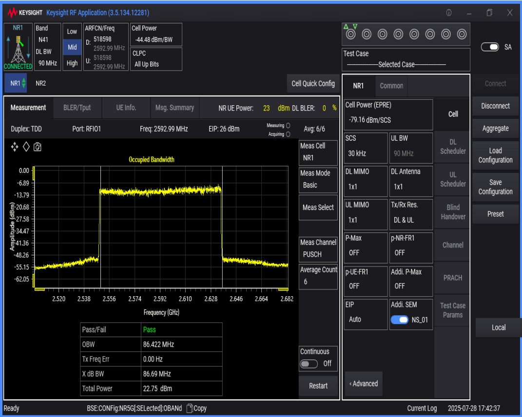
n41 SCS=30kHz DFT_QPSK BW=100MHz Channel=518598 RB=270@0
