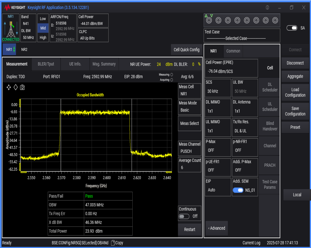
n41 SCS=30kHz DFT_QAM64 BW=80MHz Channel=518598 RB=216@0
