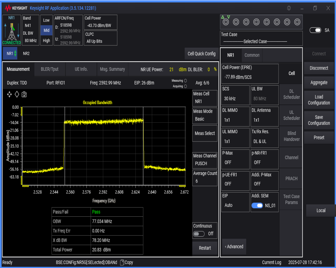
n41 SCS=30kHz DFT_QAM256 BW=90MHz Channel=518598 RB=240@0
