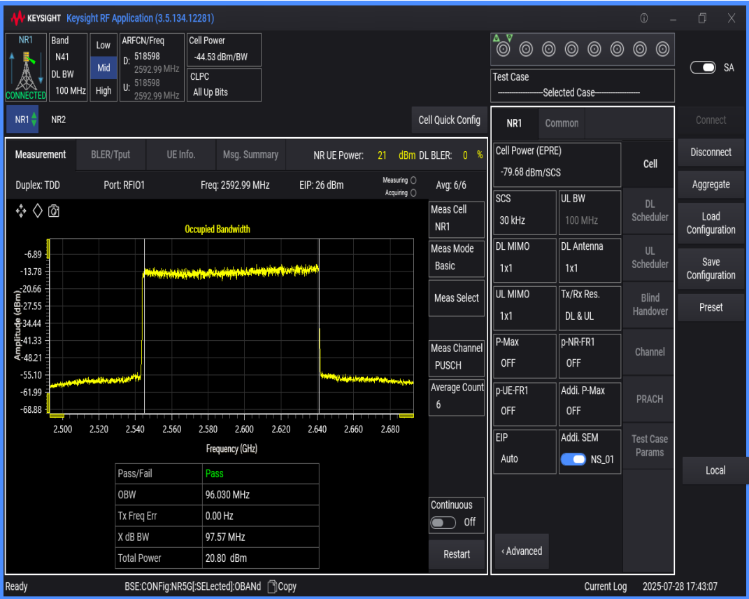
n41 SCS=30kHz DFT_QAM16 BW=90MHz Channel=518598 RB=240@0
