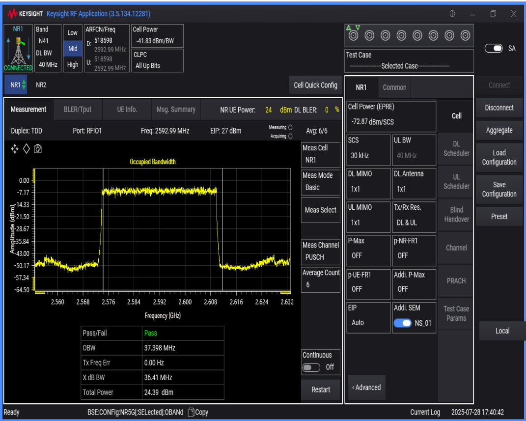
n41 SCS=30kHz DFT_BPSK BW=60MHz Channel=518598 RB=162@0
