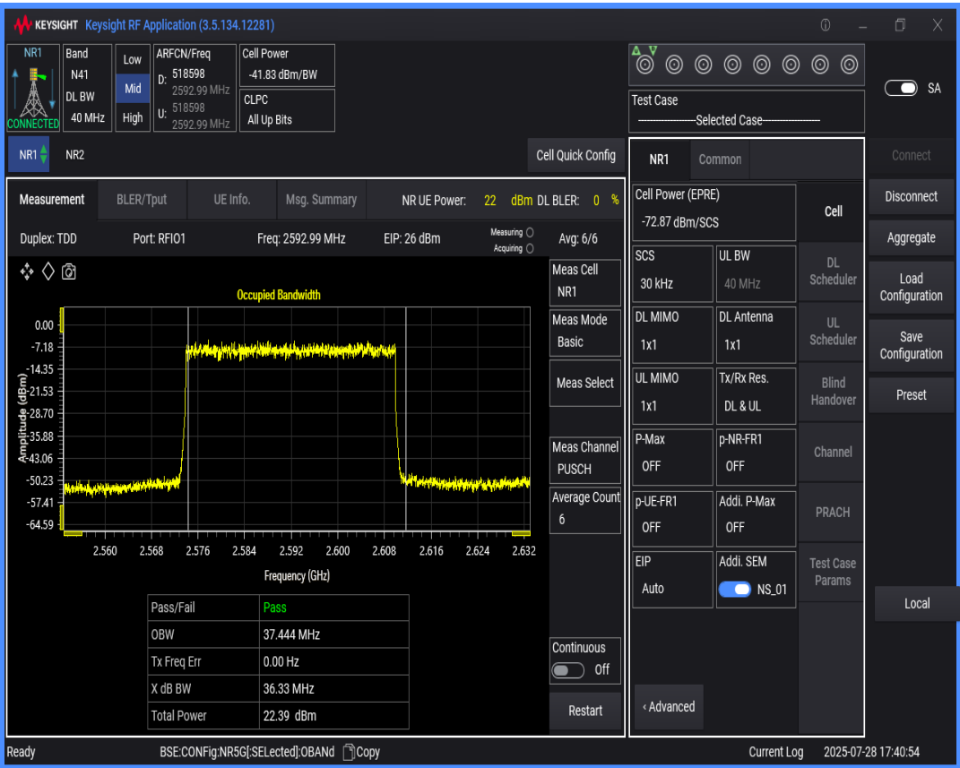
n41 SCS=30kHz DFT_QAM64 BW=100MHz Channel=518598 RB=270@0
