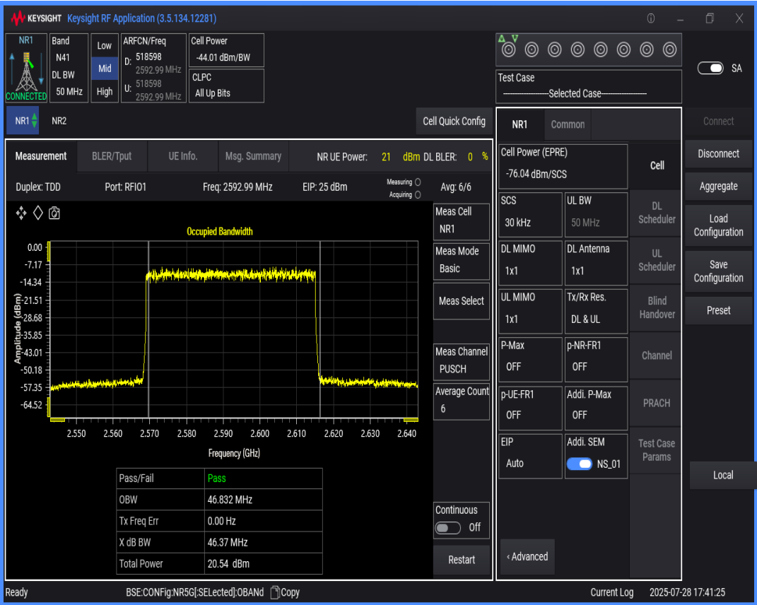
n41 SCS=30kHz DFT_QAM64 BW=50MHz Channel=518598 RB=128@0
