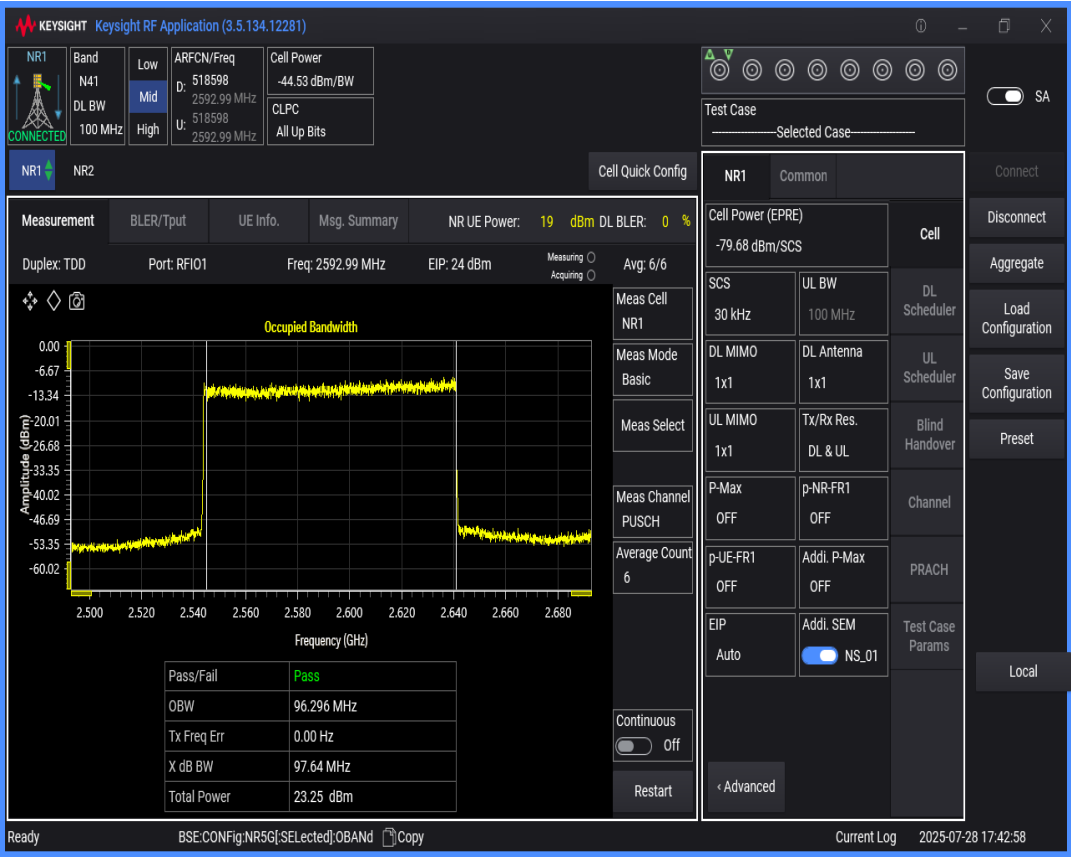
n41 SCS=30kHz DFT_QAM16 BW=50MHz Channel=518598 RB=128@0
