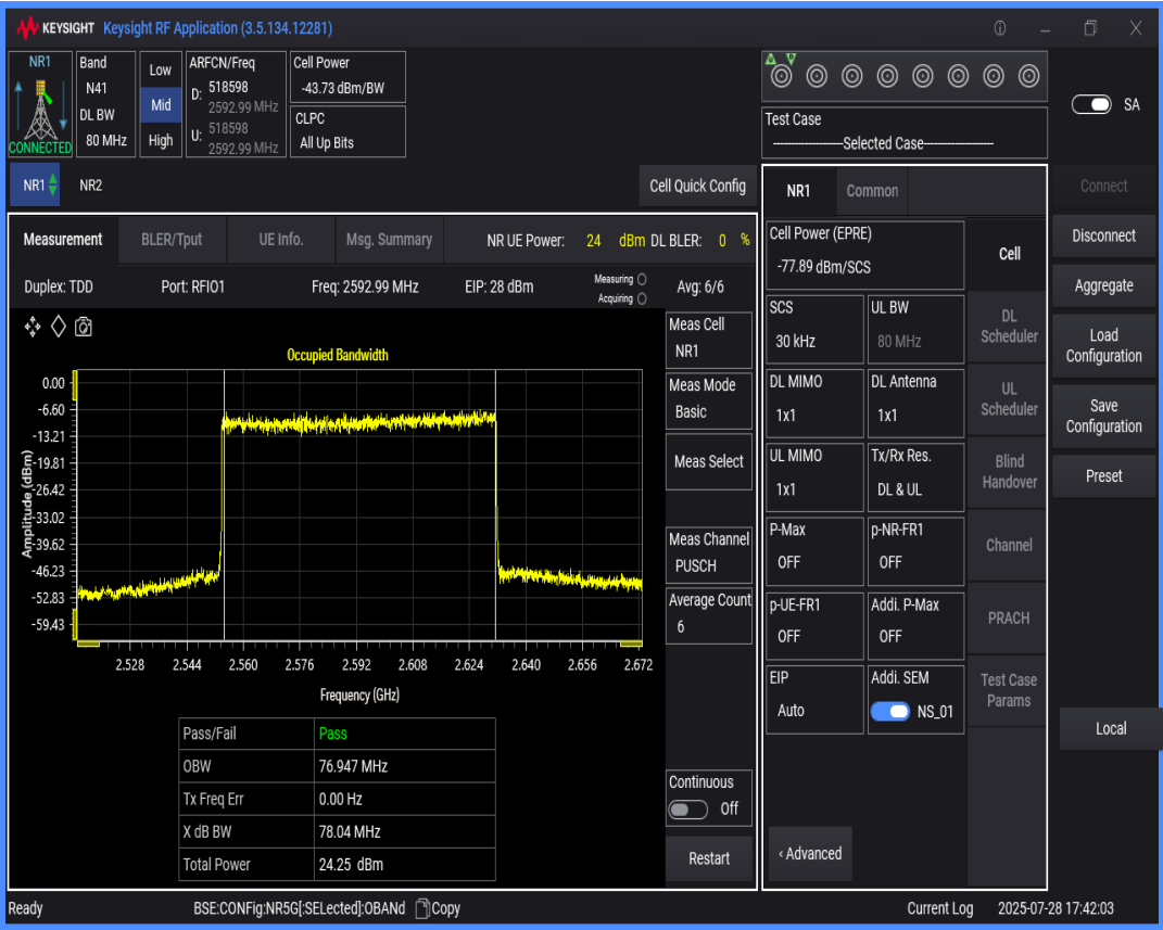
n41 SCS=30kHz DFT_QPSK BW=60MHz Channel=518598 RB=162@0
