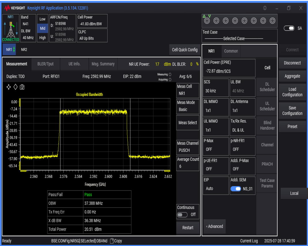
n41 SCS=30kHz DFT_QAM256 BW=50MHz Channel=518598 RB=128@0
