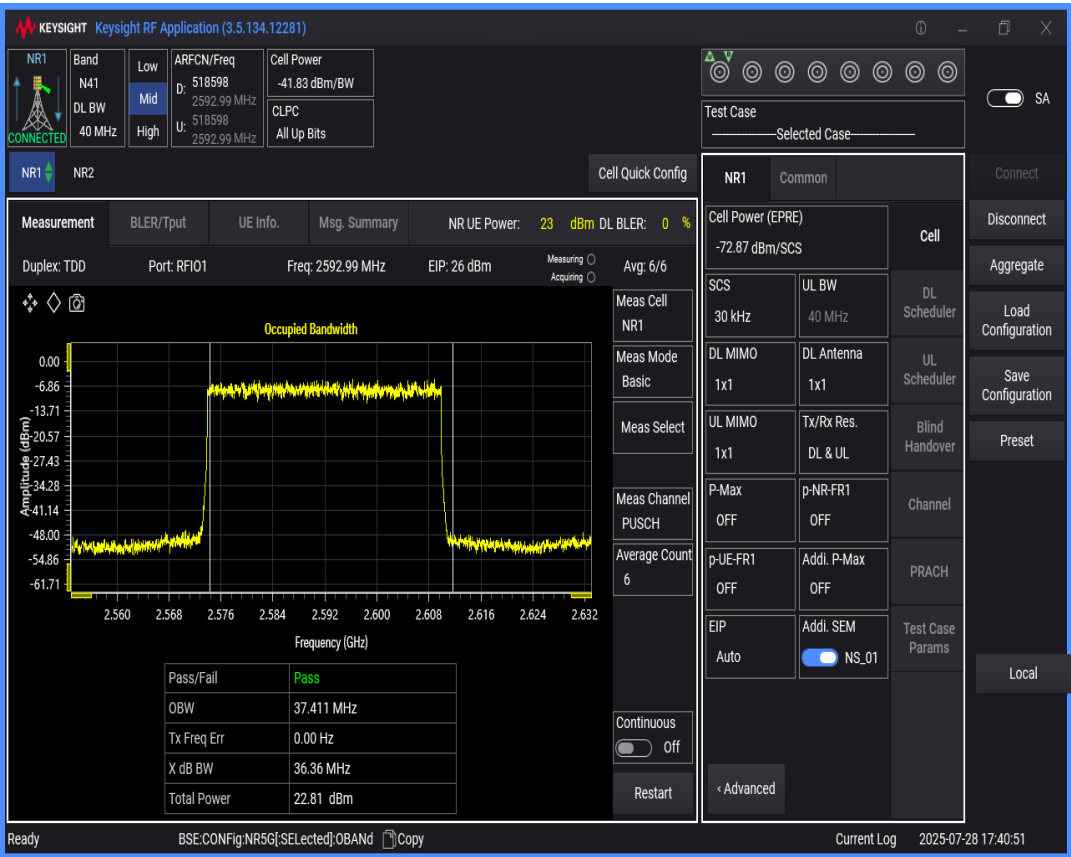
n41 SCS=30kHz DFT_QAM256 BW=100MHz Channel=518598 RB=270@0
