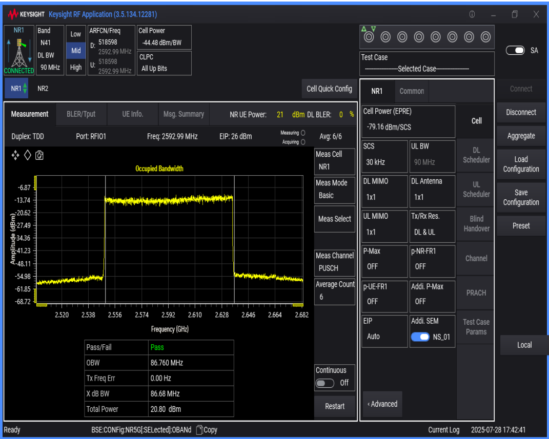
n41 SCS=30kHz DFT_QAM256 BW=60MHz Channel=518598 RB=162@0
