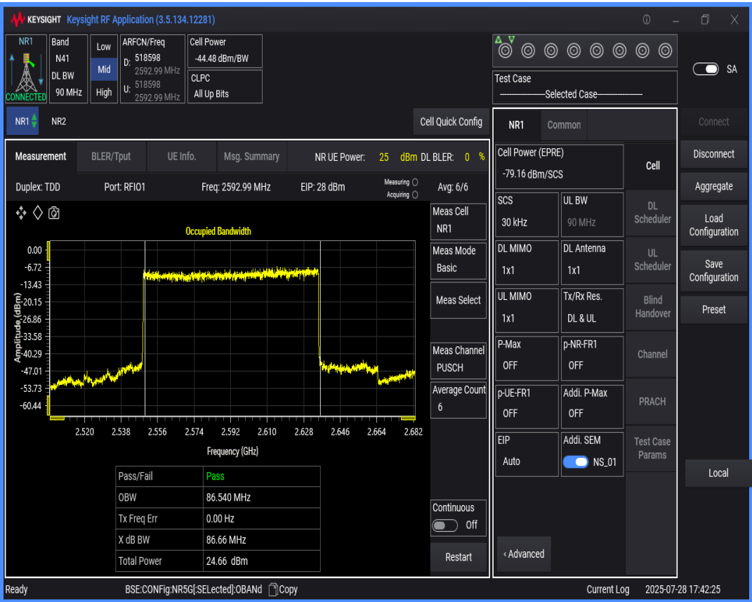
n41 SCS=30kHz DFT_BPSK BW=80MHz Channel=518598 RB=216@0
