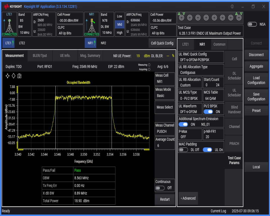
n78 SCS=30kHz DFT_QAM16 BW=100MHz Channel=636666 RB=270@0
