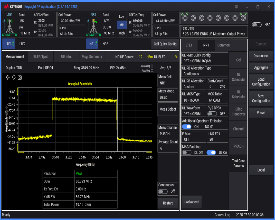
n78 SCS=30kHz DFT_QAM16 BW=80MHz Channel=636666 RB=216@0
