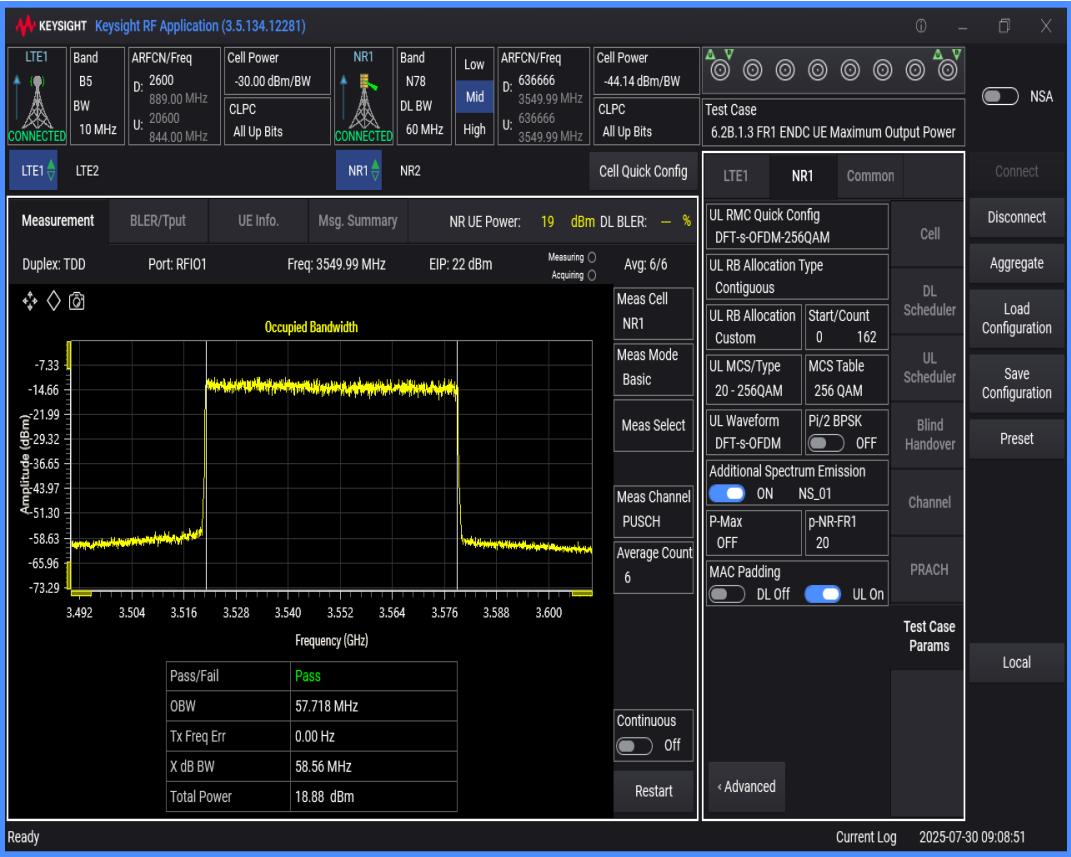
n78 SCS=30kHz DFT_QAM256 BW=80MHz Channel=636666 RB=216@0
