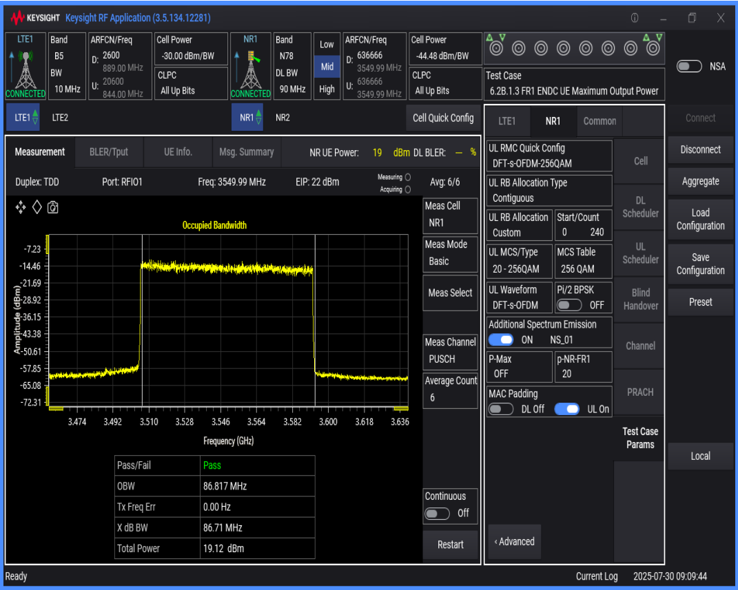
n78 SCS=30kHz DFT_QAM256 BW=50MHz Channel=636666 RB=128@0
