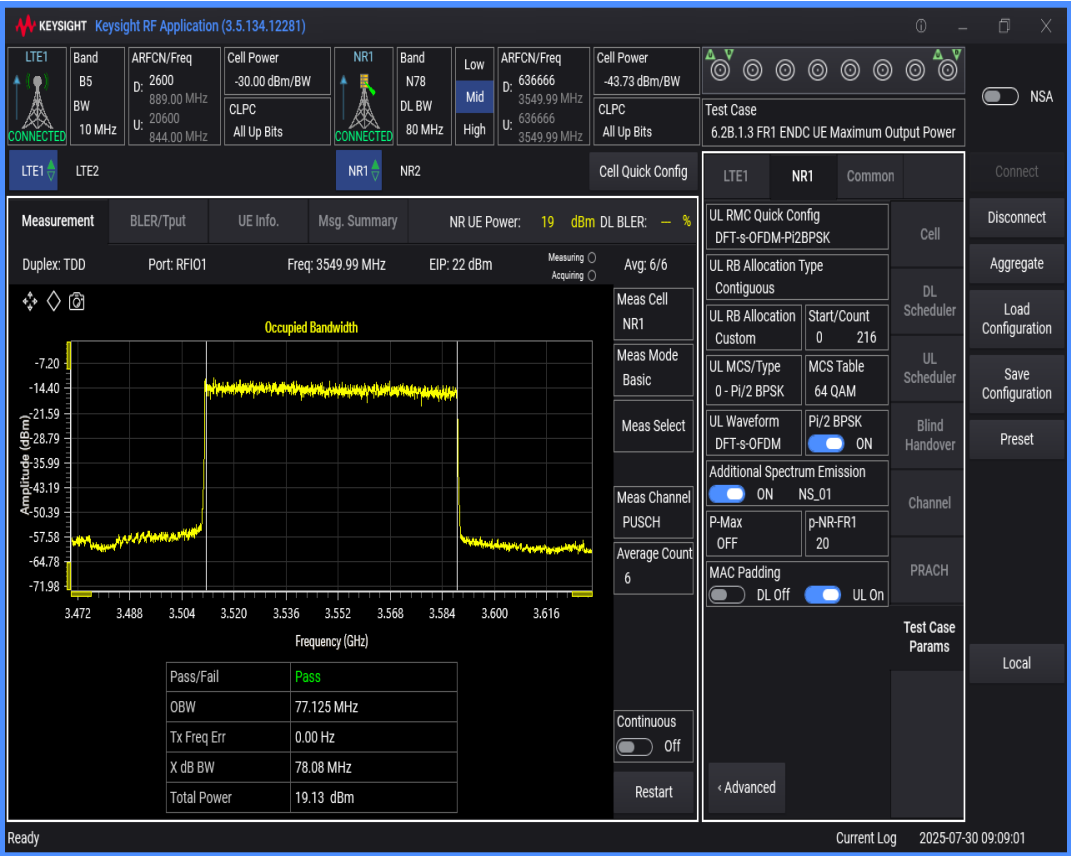
n78 SCS=30kHz DFT_QAM16 BW=90MHz Channel=636666 RB=240@0
