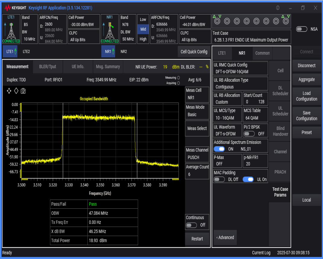
n78 SCS=30kHz DFT_QAM256 BW=60MHz Channel=636666 RB=162@0
