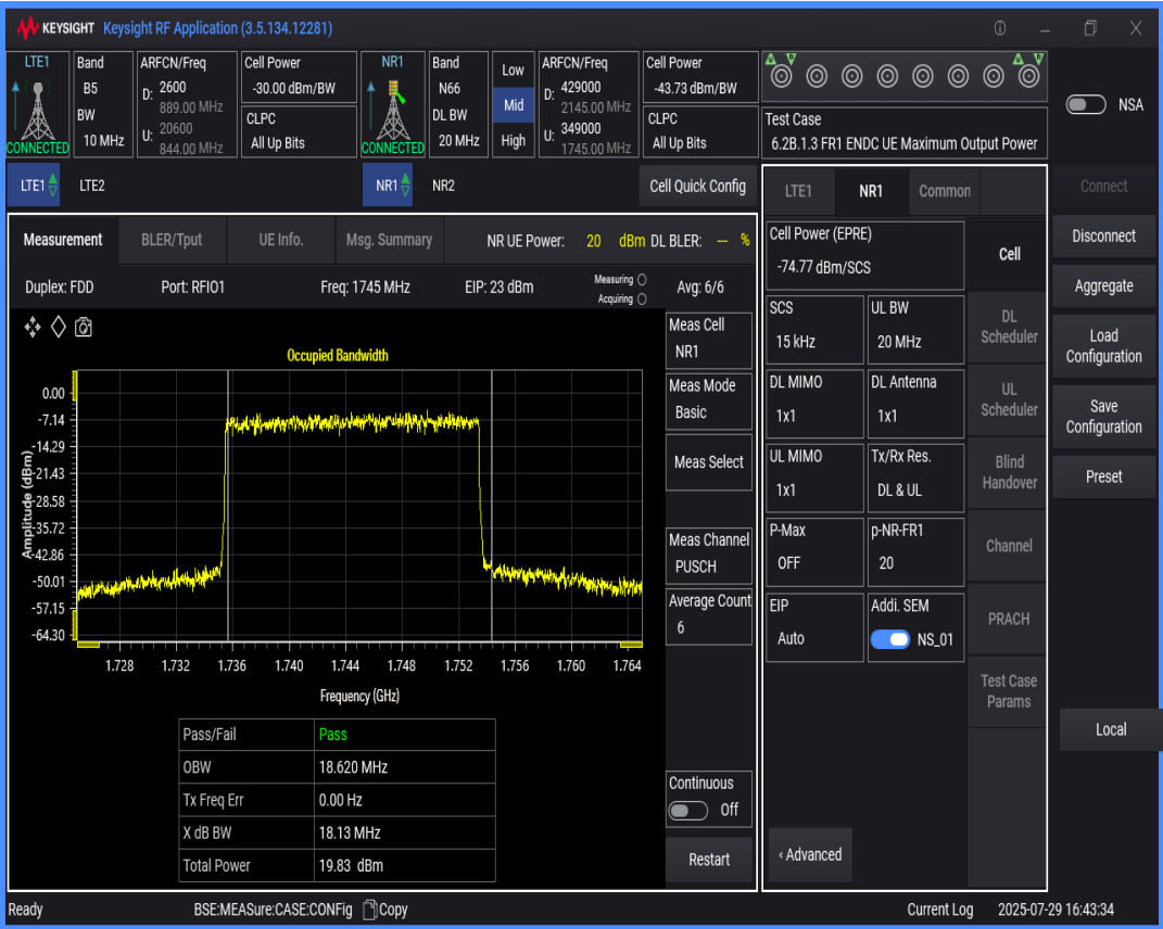
n66 SCS=15kHz DFT_QAM16 BW=15MHz Channel=349000 RB=75@0
