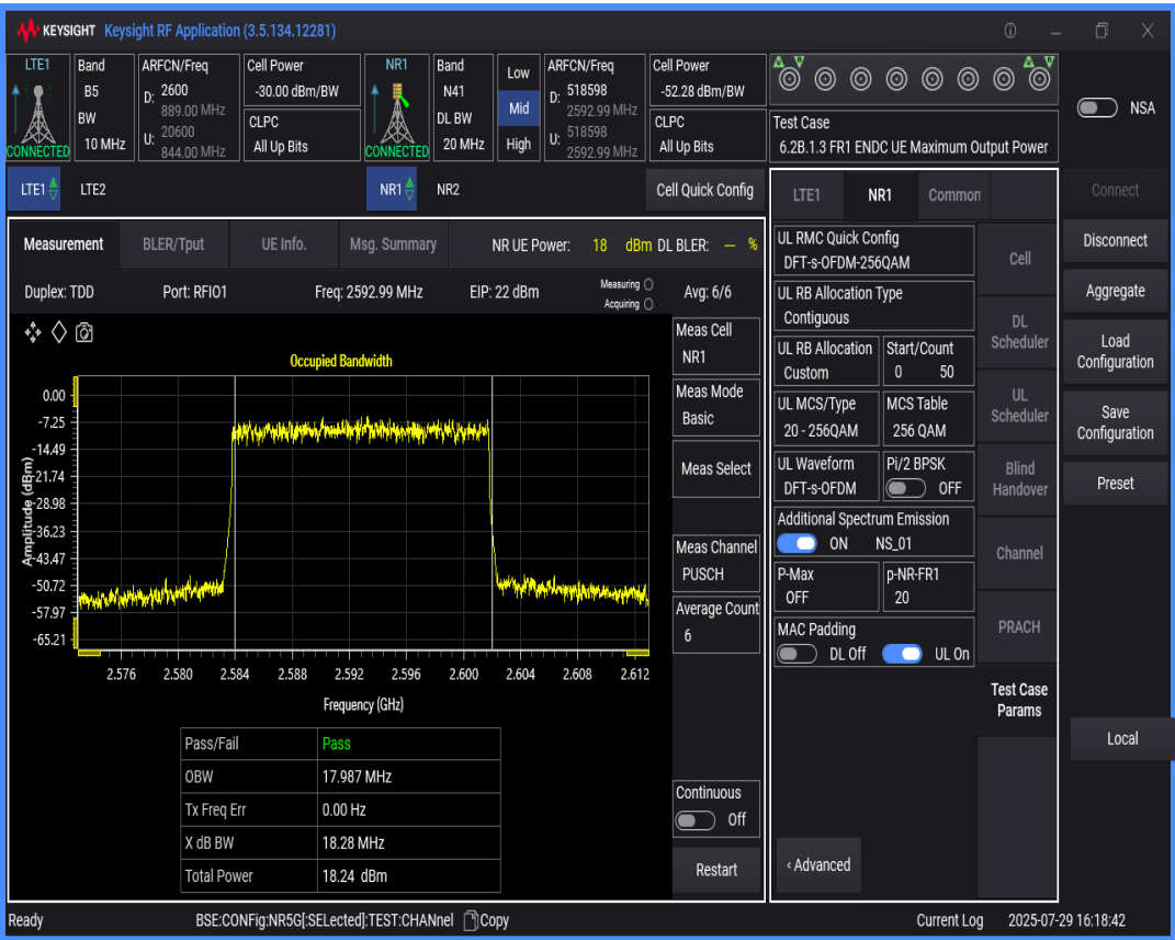
n41 SCS=30kHz DFT_QAM16 BW=80MHz Channel=518598 RB=216@0
