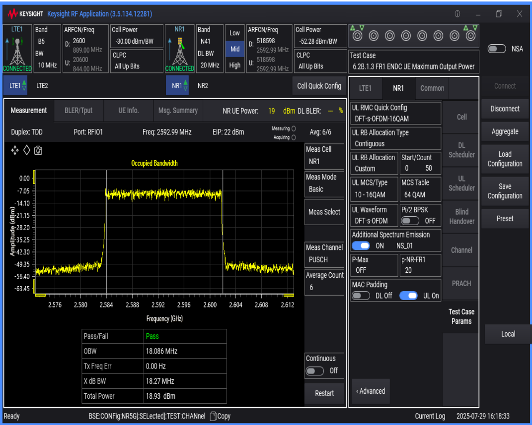
n41 SCS=30kHz DFT_BPSK BW=50MHz Channel=518598 RB=128@0
