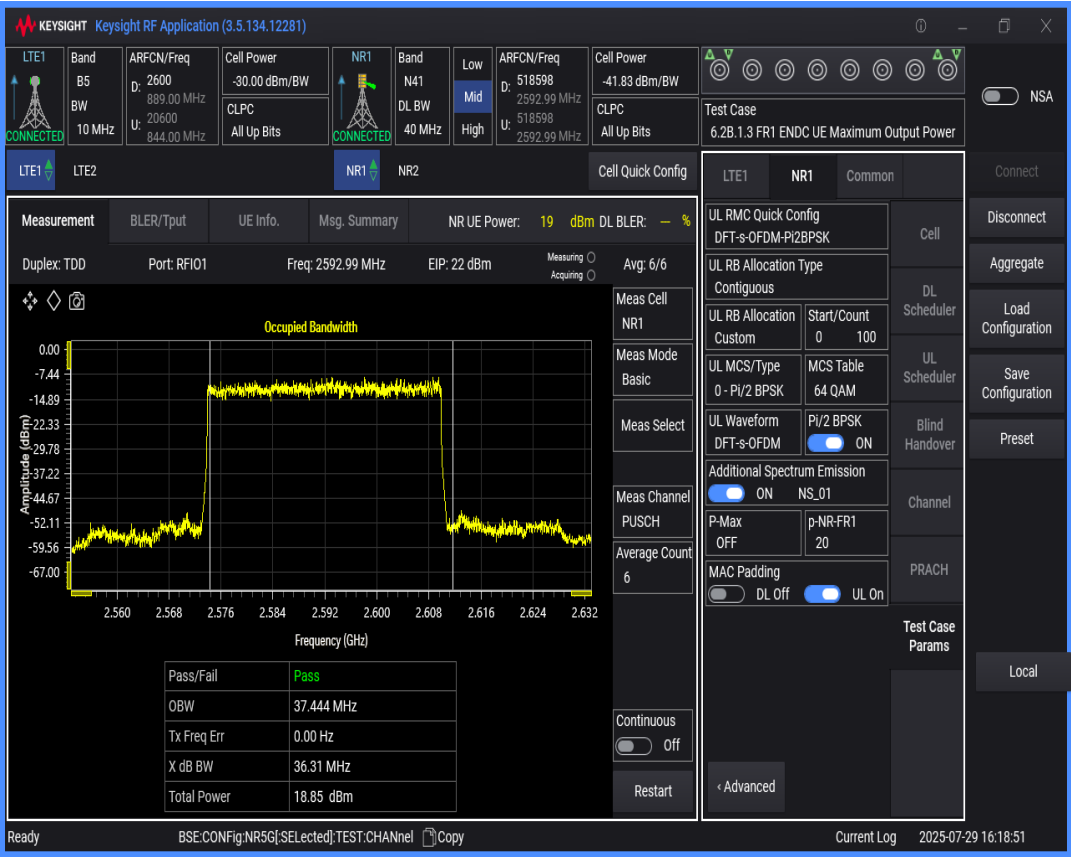
n41 SCS=30kHz DFT_BPSK BW=80MHz Channel=518598 RB=216@0
