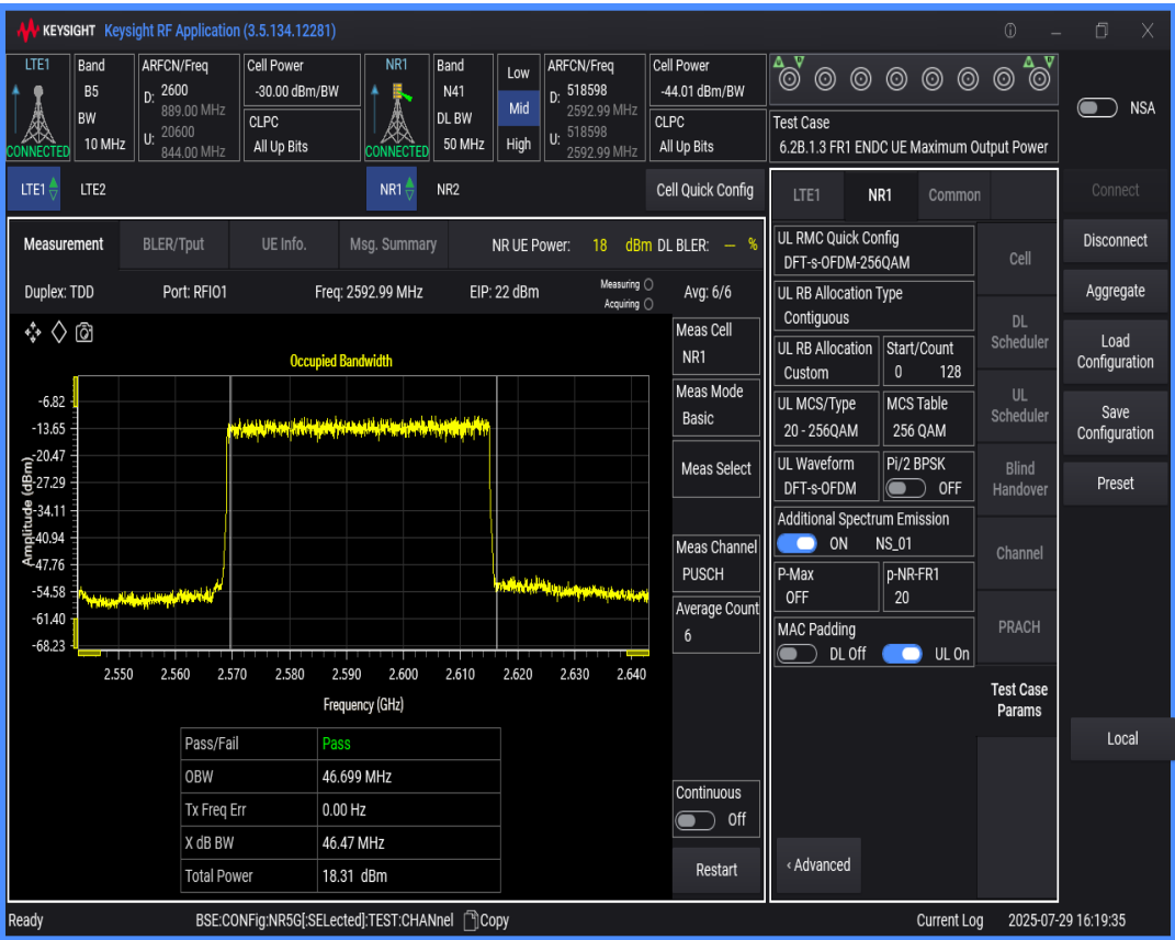
n41 SCS=30kHz DFT_QAM256 BW=60MHz Channel=518598 RB=162@0
