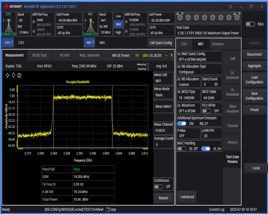
n41 SCS=30kHz DFT_QAM256 BW=80MHz Channel=518598 RB=216@0
