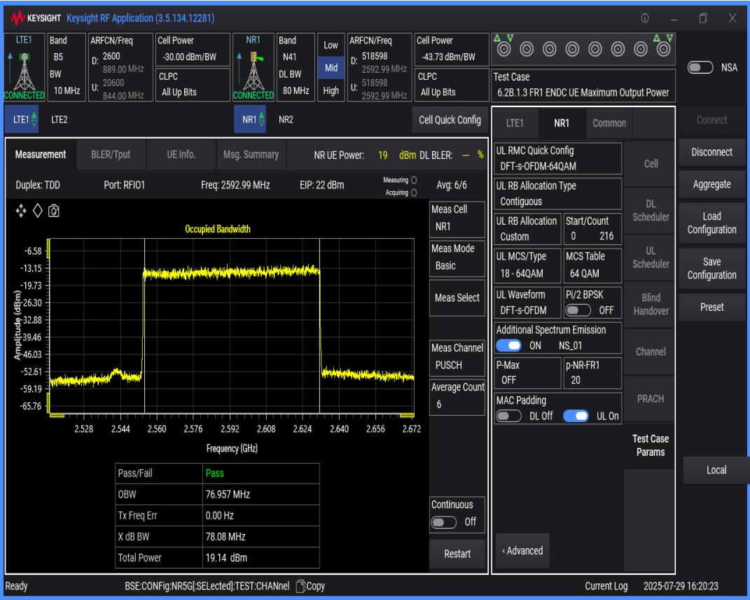
n41 SCS=30kHz DFT_QAM64 BW=90MHz Channel=518598 RB=240@0
