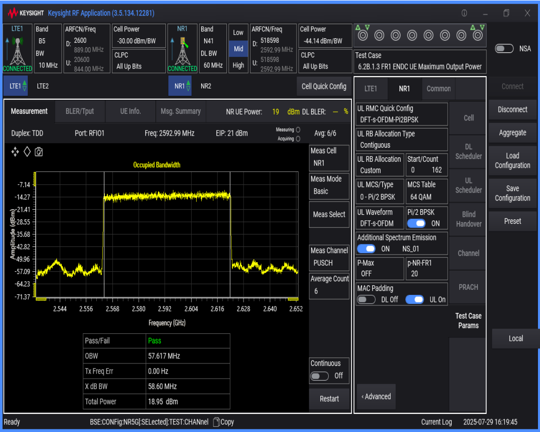
n41 SCS=30kHz DFT_QAM16 BW=60MHz Channel=518598 RB=162@0
