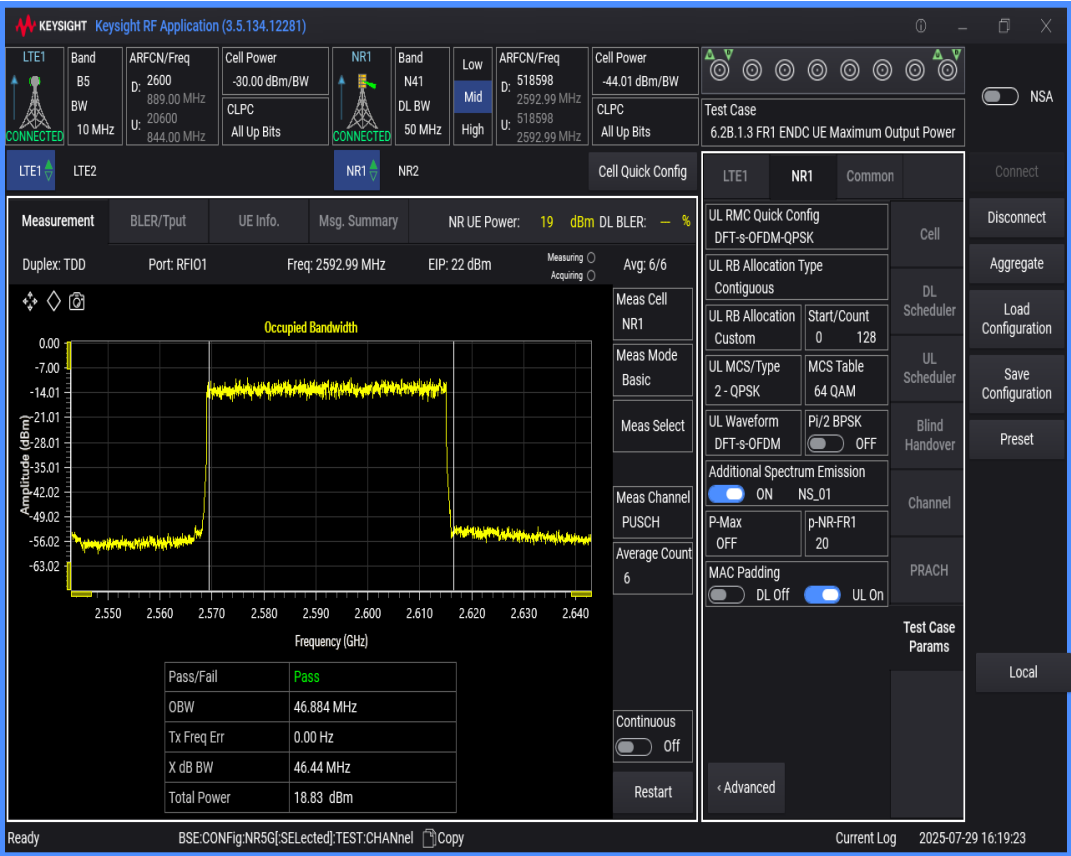
n41 SCS=30kHz DFT_QAM64 BW=80MHz Channel=518598 RB=216@0
