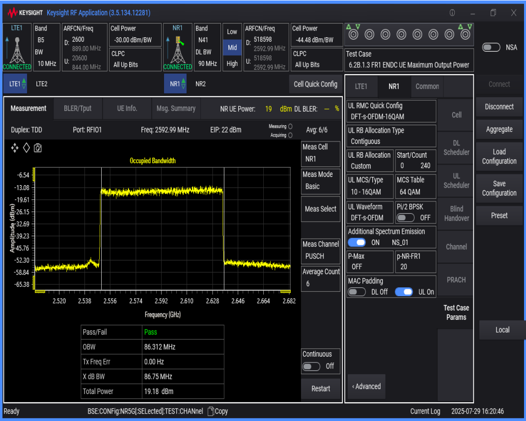
n41 SCS=30kHz DFT_QAM256 BW=90MHz Channel=518598 RB=240@0
