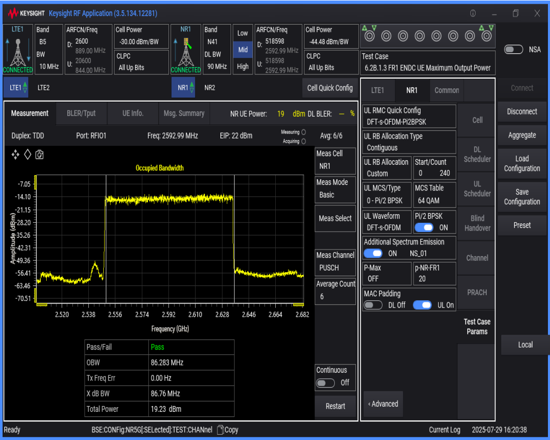
n41 SCS=30kHz DFT_QAM16 BW=40MHz Channel=518598 RB=100@0
