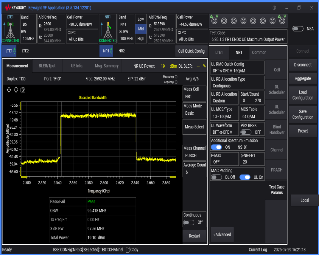
n41 SCS=30kHz DFT_BPSK BW=90MHz Channel=518598 RB=240@0
