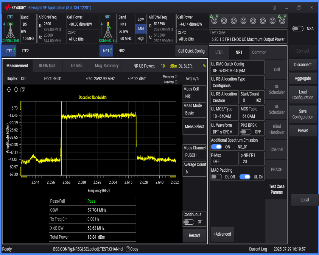
n41 SCS=30kHz DFT_QAM64 BW=50MHz Channel=518598 RB=128@0
