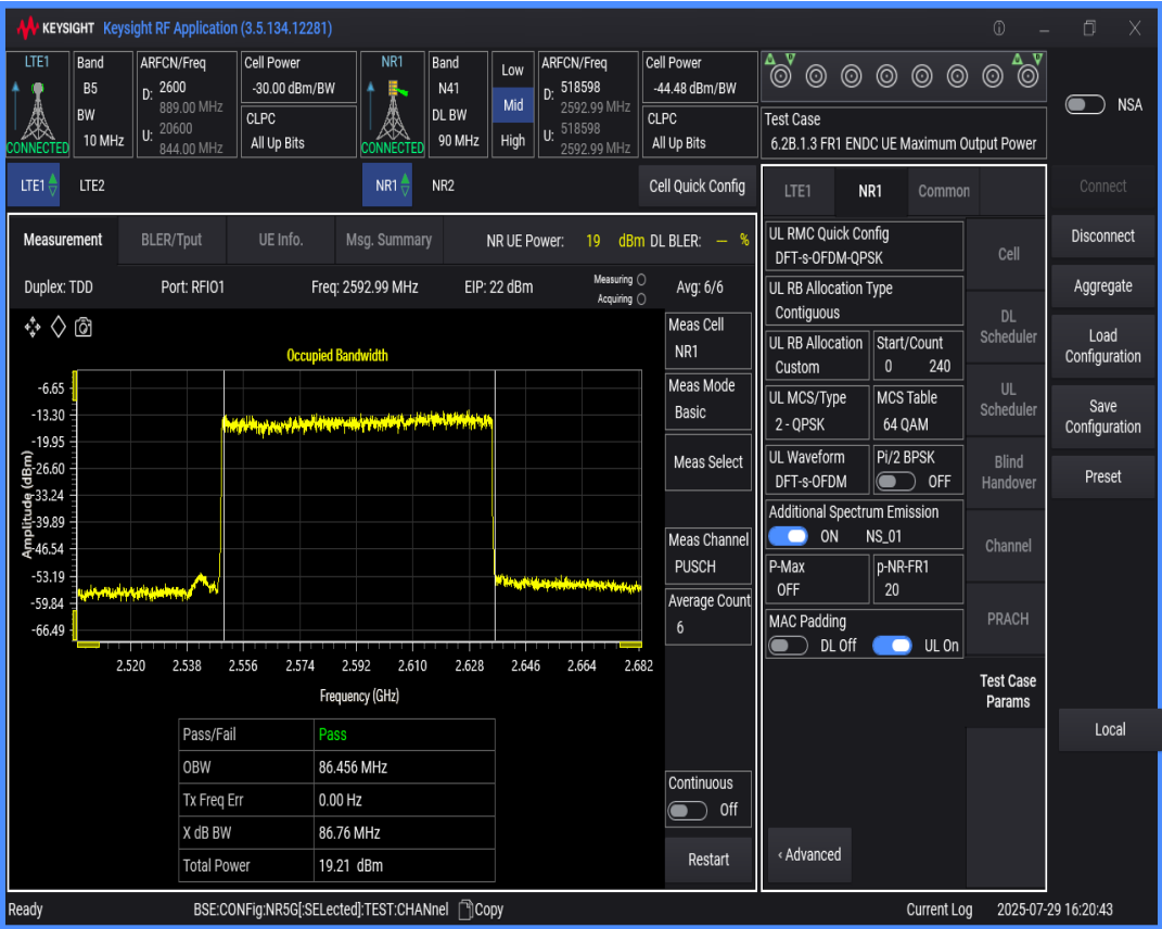
n41 SCS=30kHz DFT_QPSK BW=80MHz Channel=518598 RB=216@0
