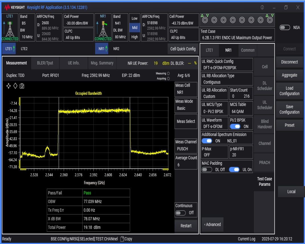
n41 SCS=30kHz DFT_BPSK BW=60MHz Channel=518598 RB=162@0
