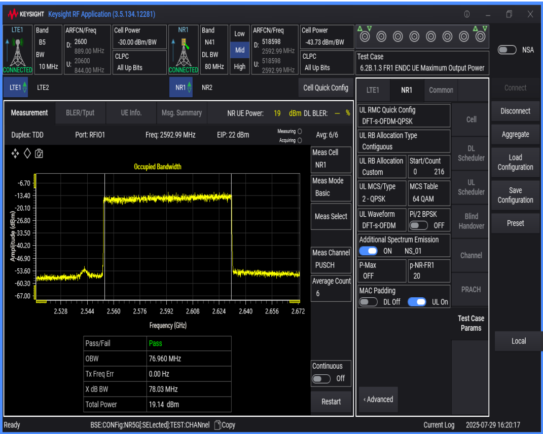
n41 SCS=30kHz DFT_QPSK BW=60MHz Channel=518598 RB=162@0
