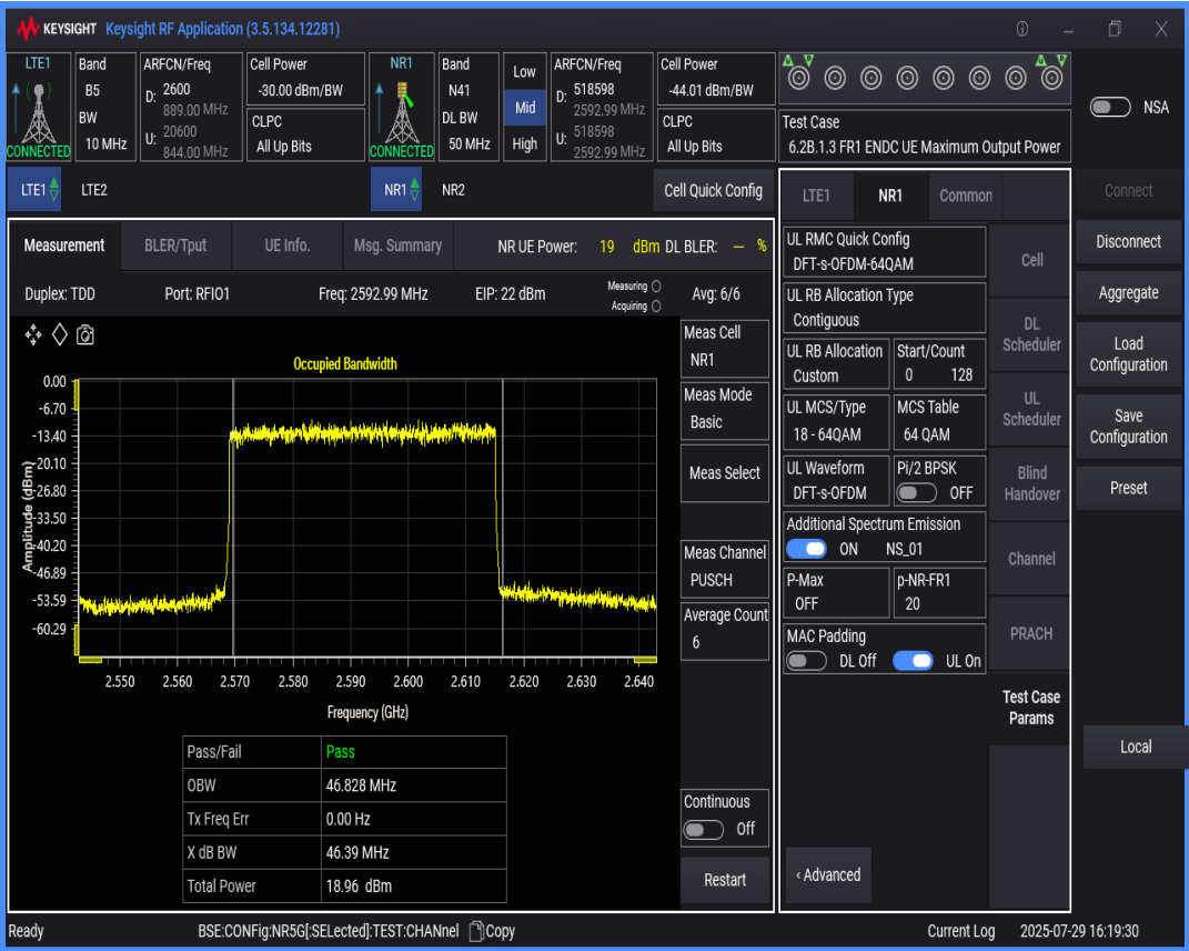
n41 SCS=30kHz DFT_QAM64 BW=40MHz Channel=518598 RB=100@0
