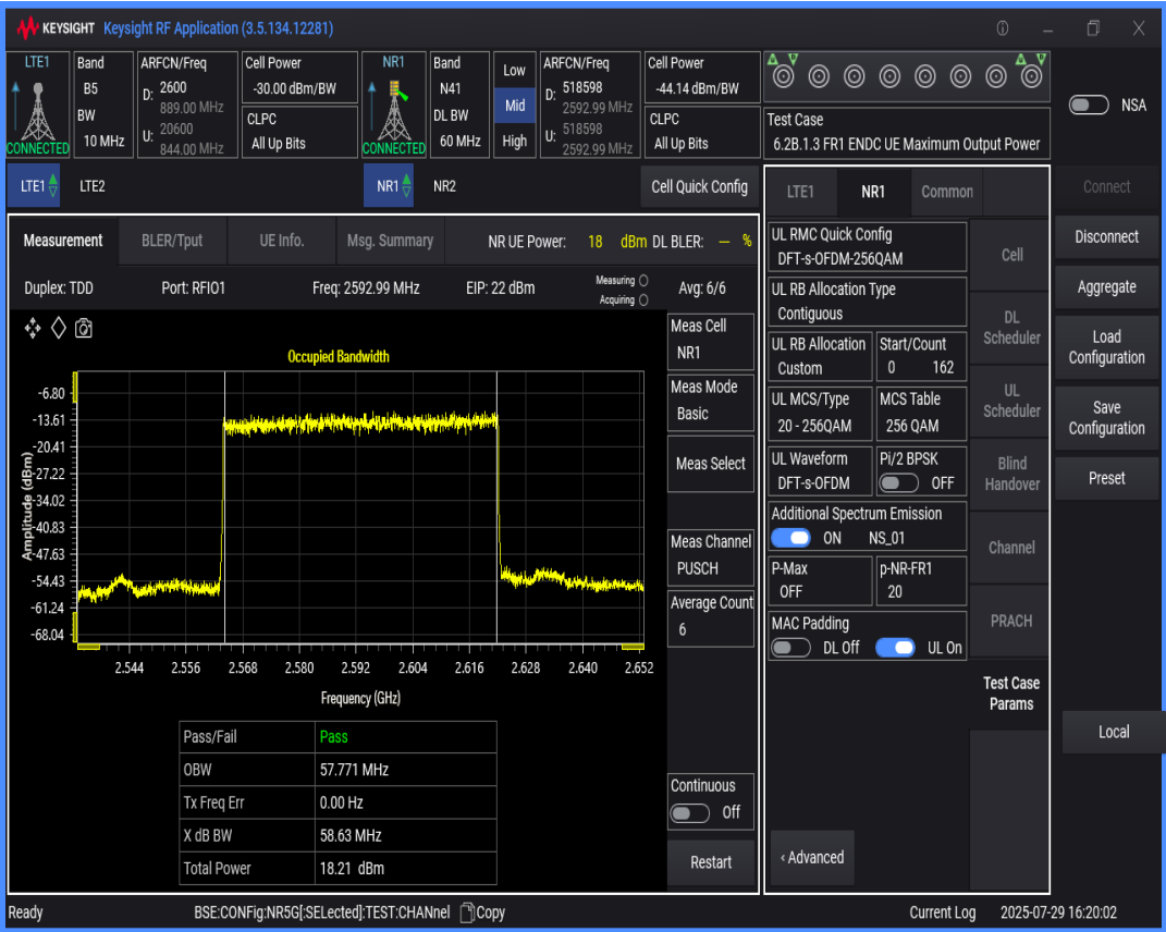
n41 SCS=30kHz DFT_QAM64 BW=60MHz Channel=518598 RB=162@0
