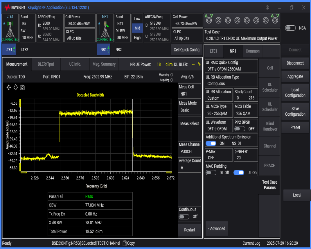
n41 SCS=30kHz DFT_QAM256 BW=40MHz Channel=518598 RB=100@0
