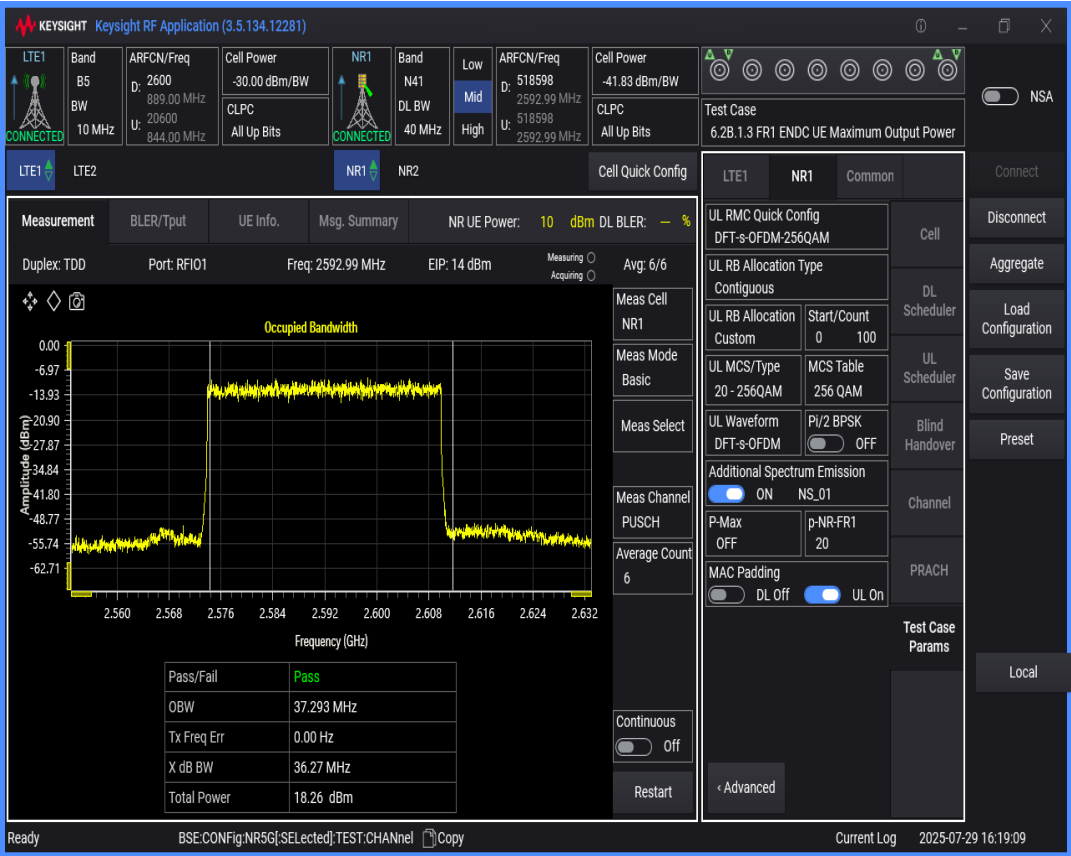
n41 SCS=30kHz DFT_QAM256 BW=50MHz Channel=518598 RB=128@0
