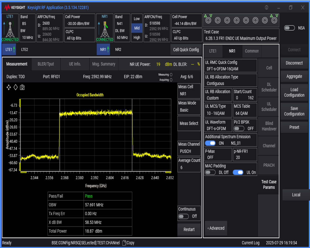
n41 SCS=30kHz DFT_QAM16 BW=50MHz Channel=518598 RB=128@0
