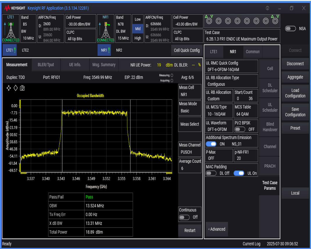
n78 SCS=30kHz DFT_QAM16 BW=90MHz Channel=636666 RB=240@0
