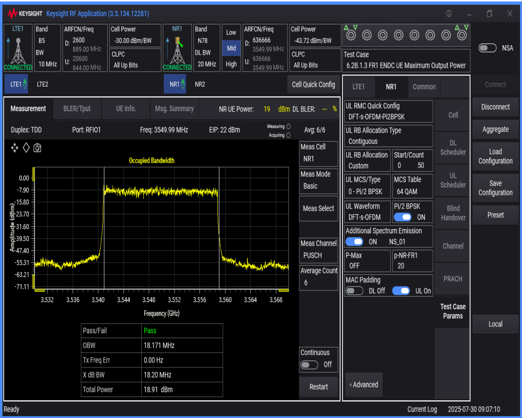
n78 SCS=30kHz DFT_BPSK BW=100MHz Channel=636666 RB=270@0
