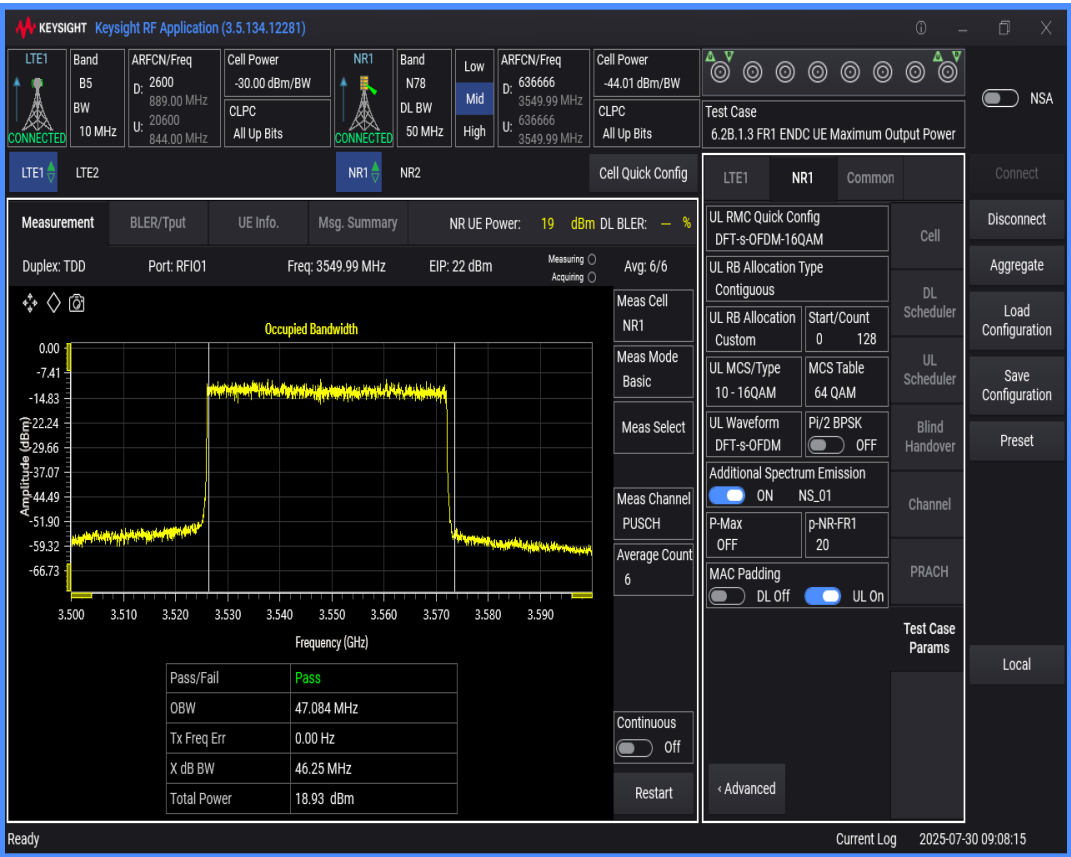
n78 SCS=30kHz DFT_QAM16 BW=60MHz Channel=636666 RB=162@0
