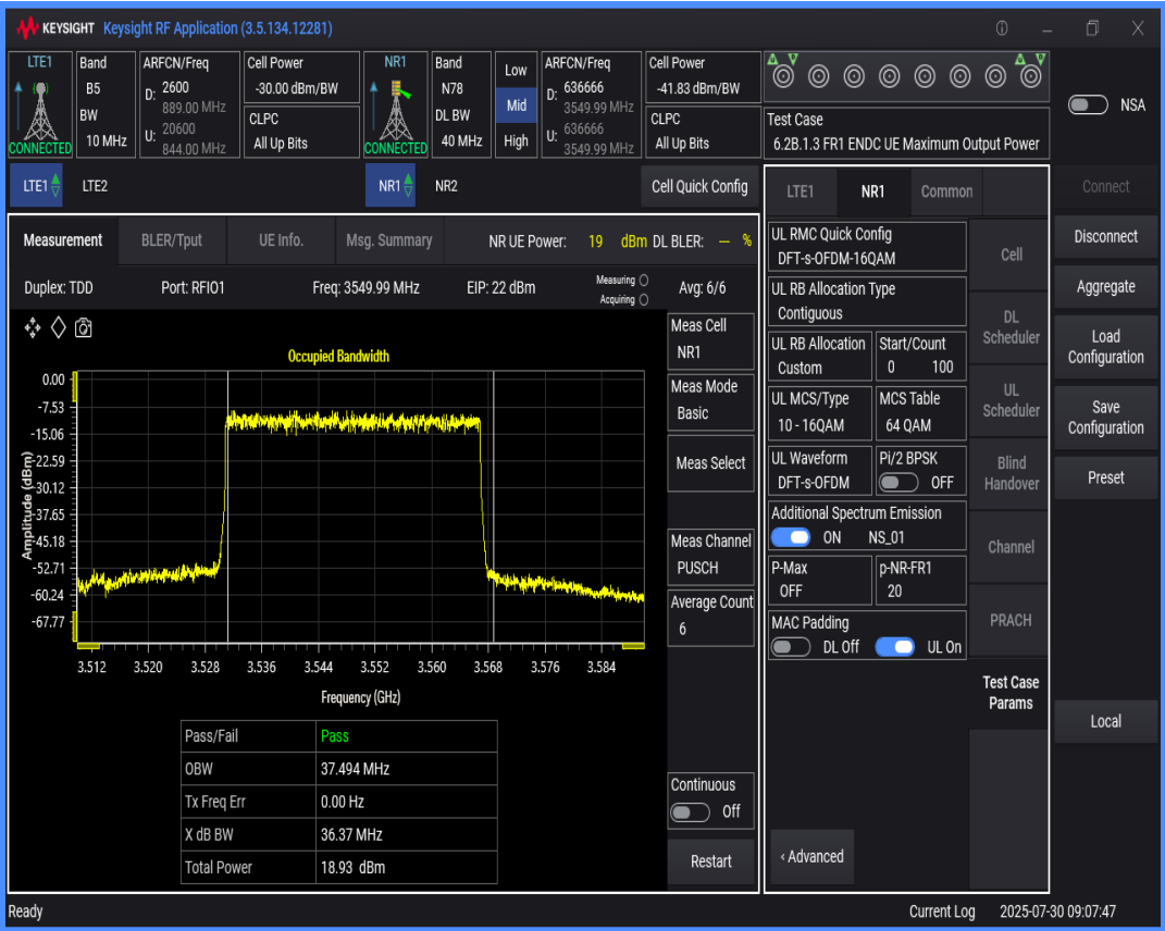
n78 SCS=30kHz DFT_QAM16 BW=50MHz Channel=636666 RB=128@0
