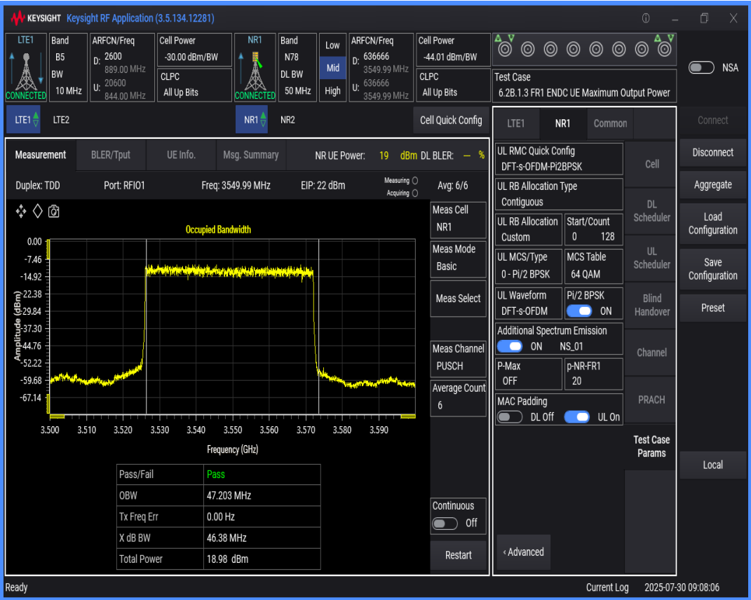
n78 SCS=30kHz DFT_BPSK BW=60MHz Channel=636666 RB=162@0
