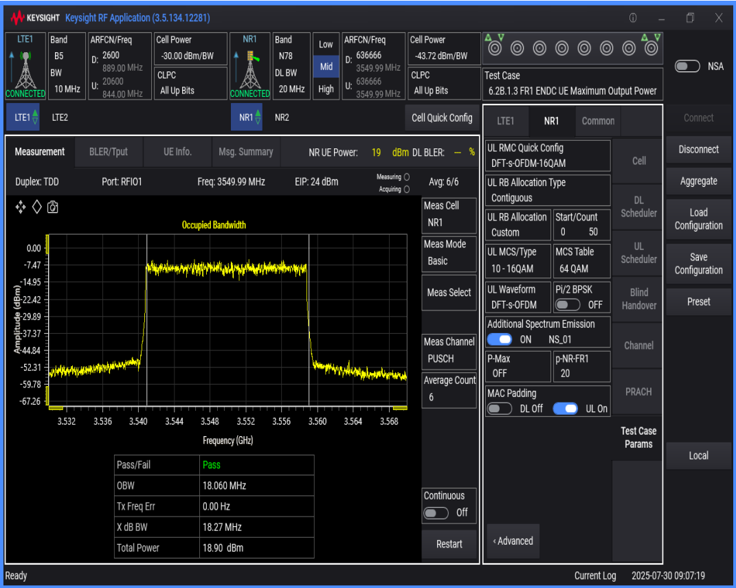
n78 SCS=30kHz DFT_QAM16 BW=15MHz Channel=636666 RB=36@0
