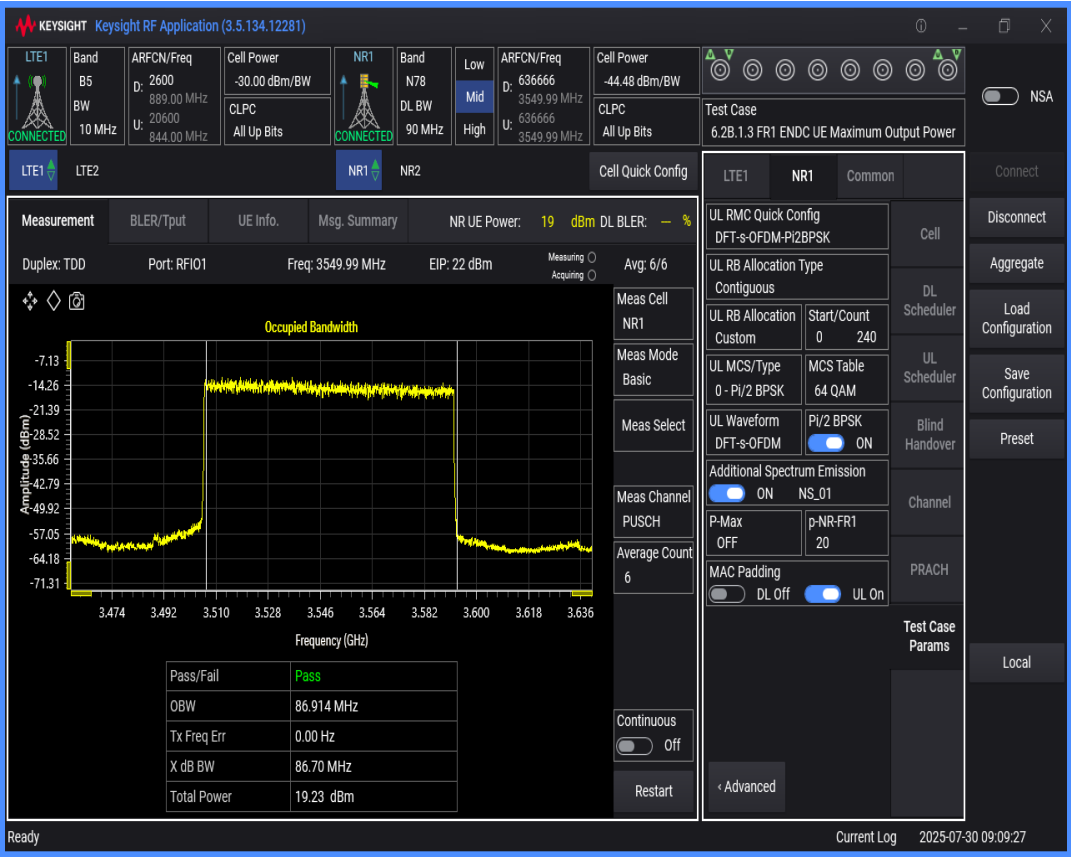
n78 SCS=30kHz DFT_QAM16 BW=100MHz Channel=636666 RB=270@0
