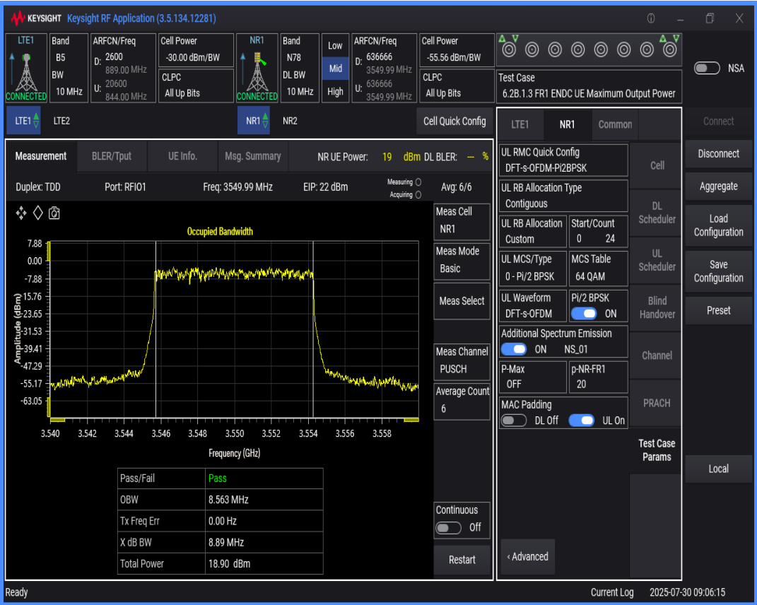
n78 SCS=30kHz DFT_BPSK BW=90MHz Channel=636666 RB=240@0
