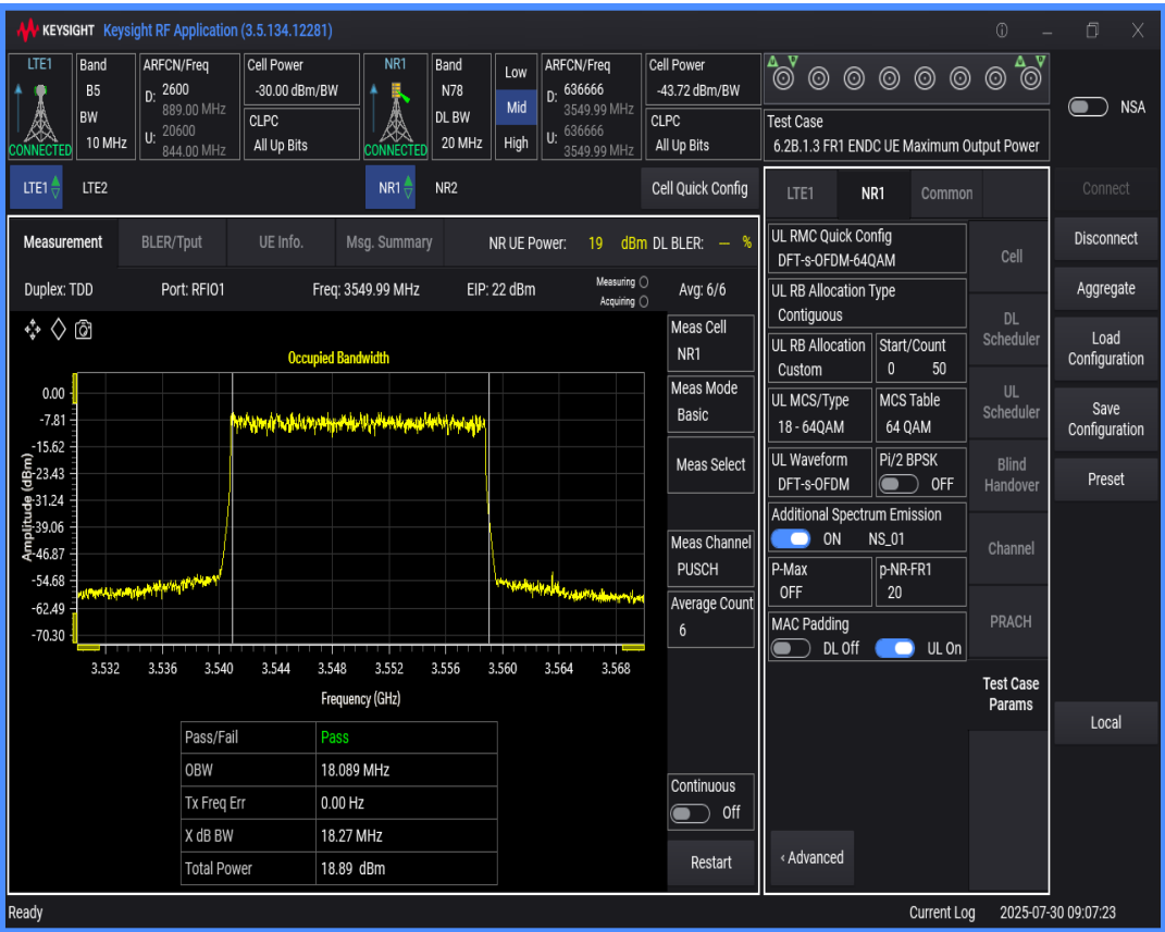
n78 SCS=30kHz DFT_QAM64 BW=90MHz Channel=636666 RB=240@0
