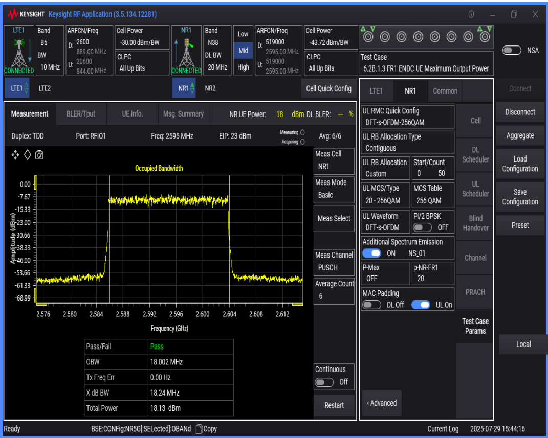
n38 SCS=30kHz DFT_QAM64 BW=10MHz Channel=519000 RB=24@0
