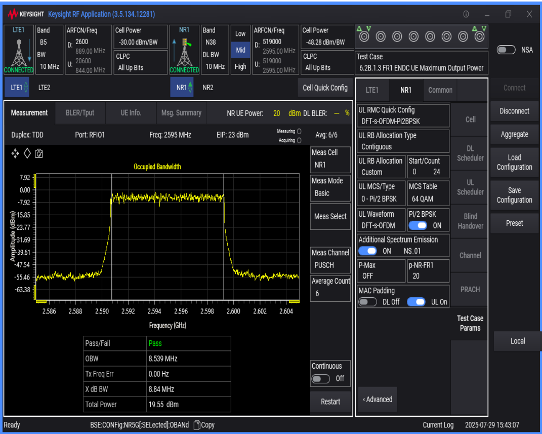
n38 SCS=30kHz DFT_QAM256 BW=15MHz Channel=519000 RB=36@0
