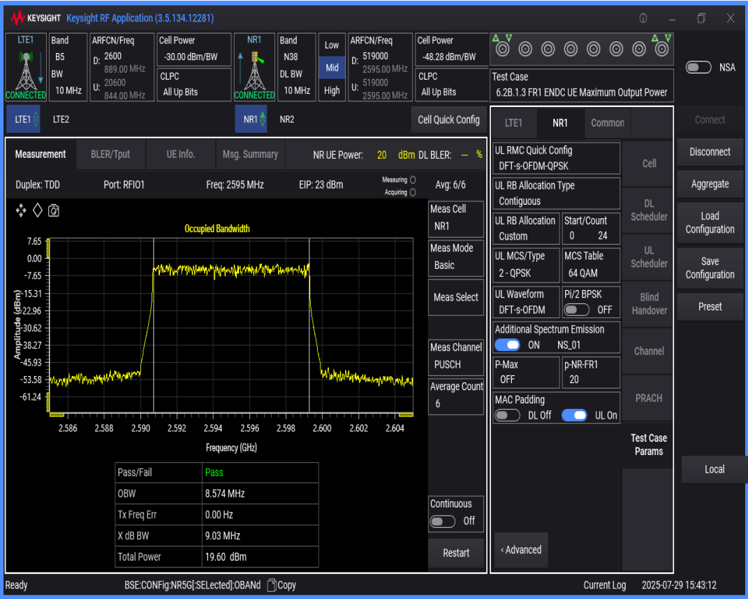
n38 SCS=30kHz DFT_QAM64 BW=15MHz Channel=519000 RB=36@0
