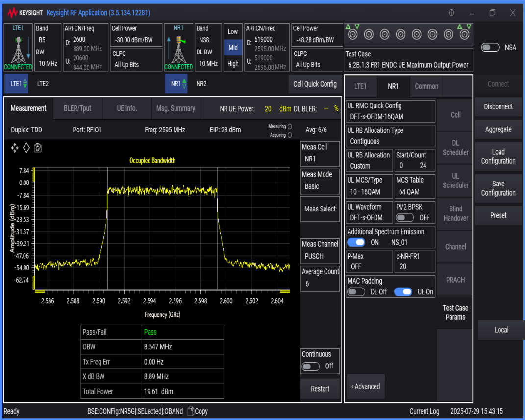
n38 SCS=30kHz DFT_QAM16 BW=15MHz Channel=519000 RB=36@0
