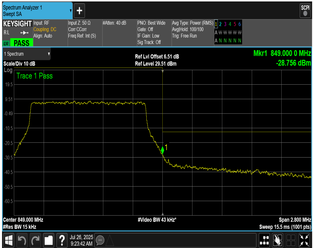
Band5 QAM16 BW=1.4MHz Channel=20407 RB Size=6 Position=#0
