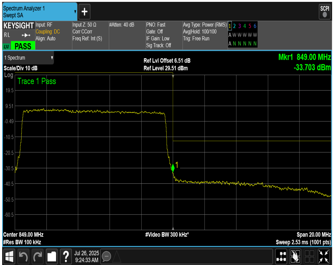
Band5 QAM16 BW=3MHz Channel=20415 RB Size=15 Position=#0
