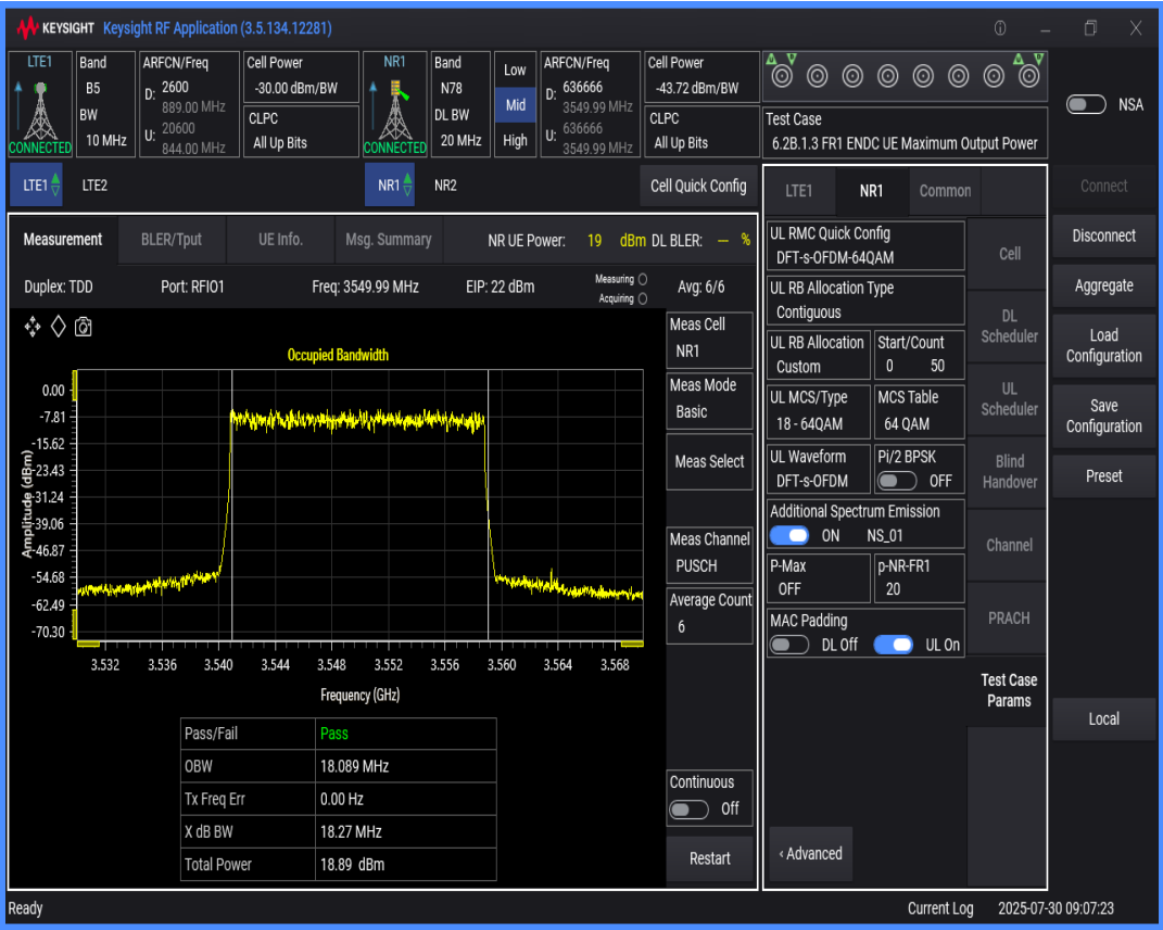
n78 SCS=30kHz DFT_QAM64 BW=40MHz Channel=636666 RB=100@0
