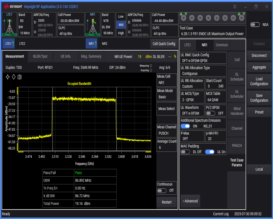
n78 SCS=30kHz DFT_QPSK BW=80MHz Channel=636666 RB=216@0
