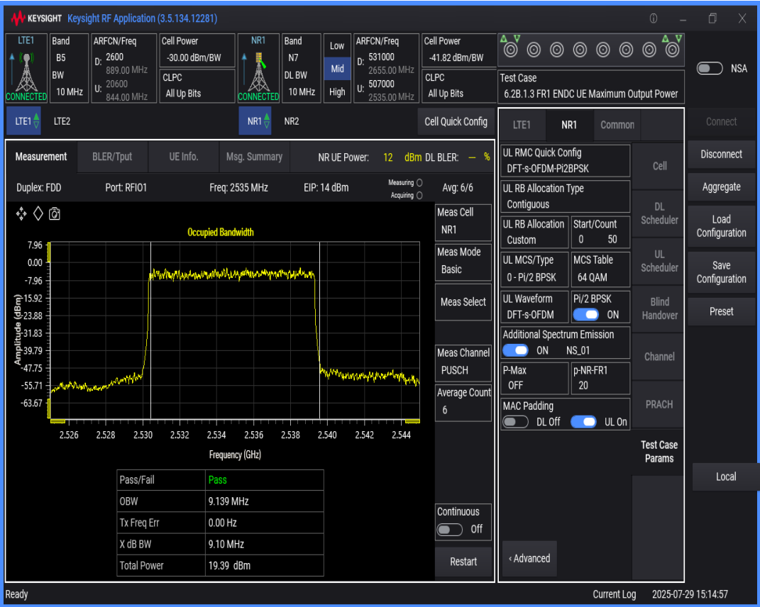
n7 SCS=15kHz DFT_BPSK BW=15MHz Channel=507000 RB=75@0
