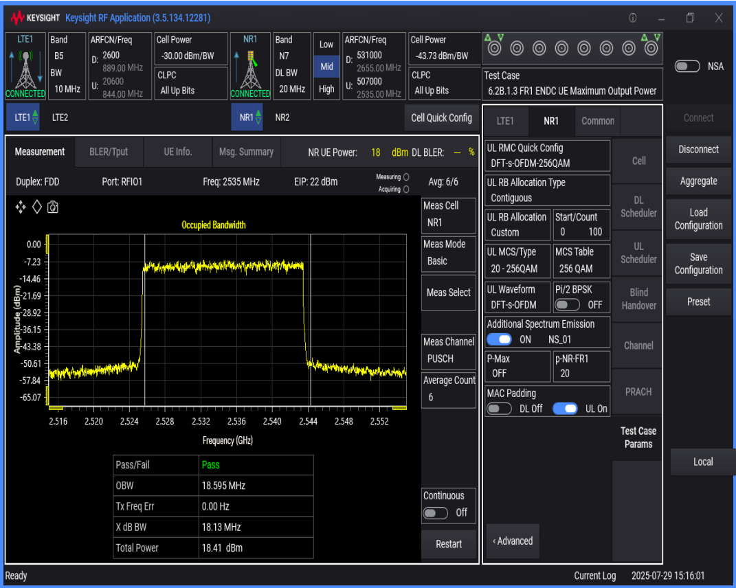
n7 SCS=15kHz DFT_QAM16 BW=5MHz Channel=507000 RB=25@0
