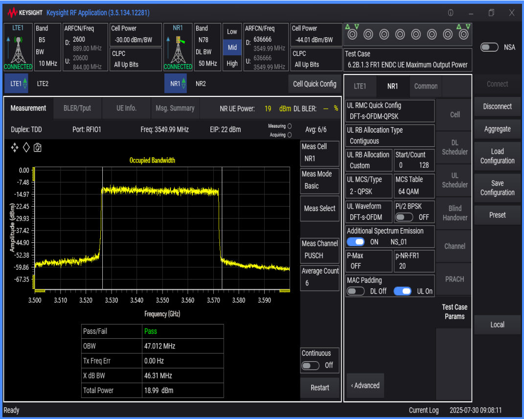
n78 SCS=30kHz DFT_QPSK BW=80MHz Channel=636666 RB=216@0
