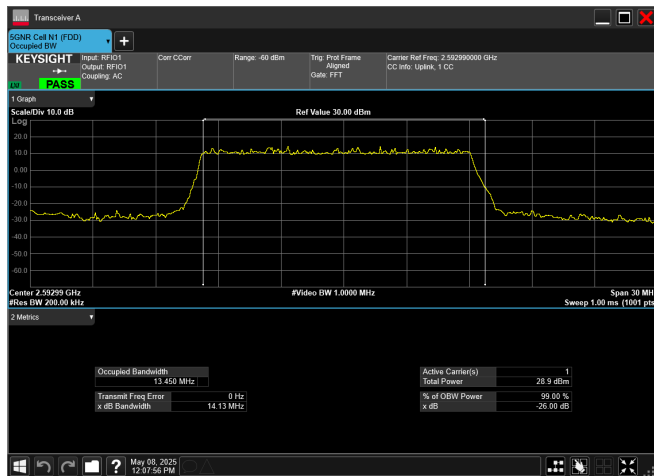
n41_15MHz_30kHz_2592.99MHz_CP-OFDM QPSK_RB38@0
