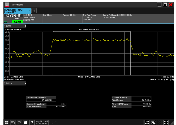
n41_50MHz_30kHz_2592.99MHz_DFT-s-OFDM \pi/2 BPSK_RB128@0
