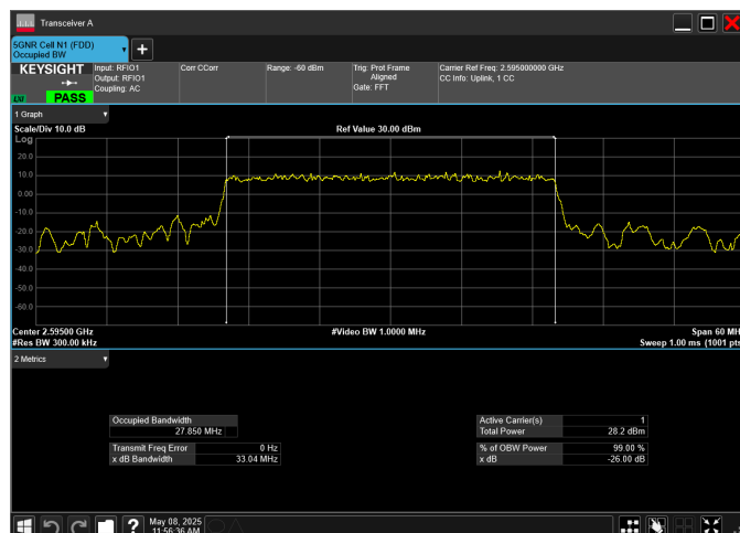
n38_40MHz_30kHz_2595MHz_DFT-s-OFDM \pi/2 BPSK_RB100@0
